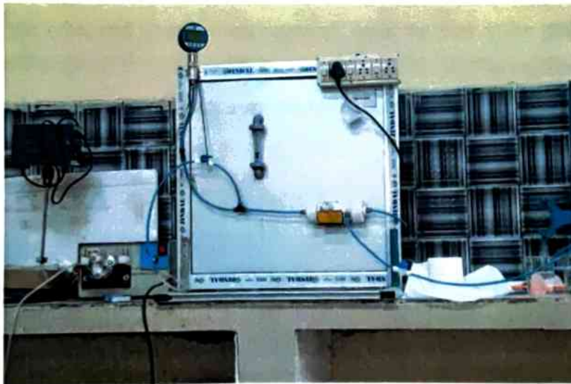
Fig 3.8: Crossflow set up For Water Flux Test
