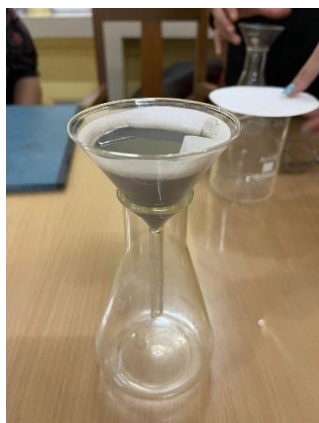
Fig.3.4: Filtration of reacted NaOH + RHA
