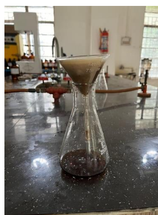
Fig.3.7: Filtration of the alkaline solution
