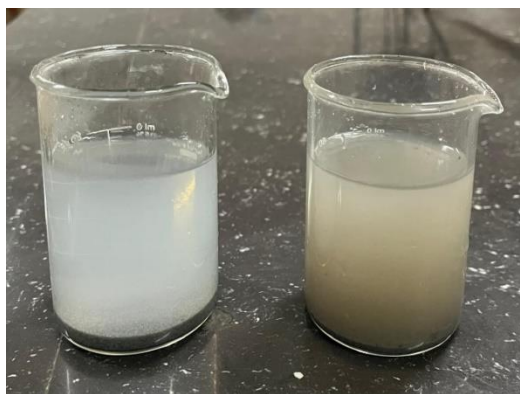
Fig.4.3: Solubility test of sodium silicate
