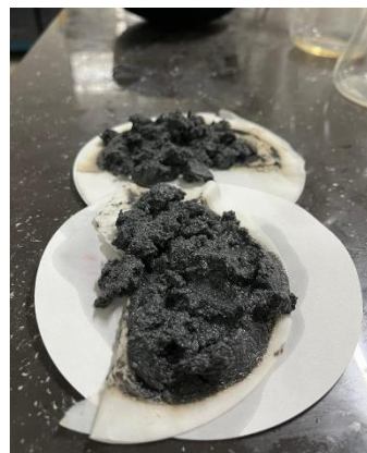
Fig.3.5: Filtered and dried \text{Na}_2\text{SiO}_3
