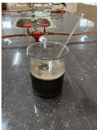
Fig.3.6: Mixing of banana stem ash and water
