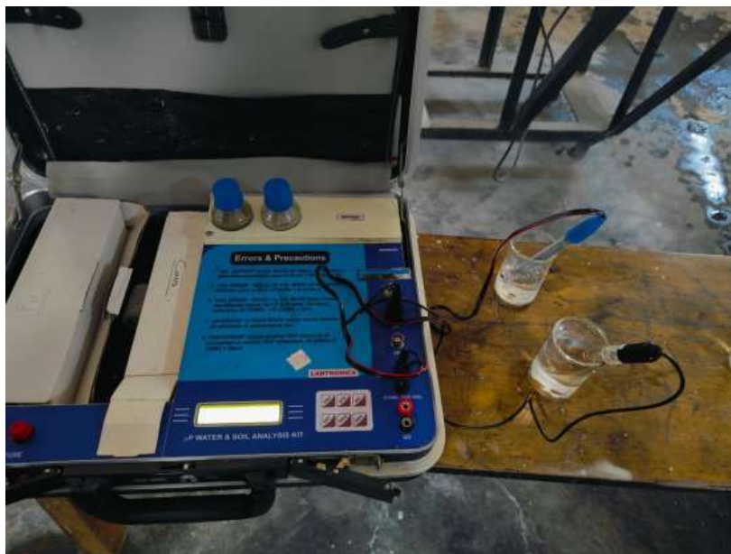
Fig 5- Measuring TDS with Water Analysis Kit.
