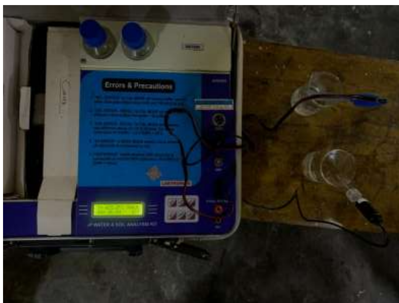
Fig 4- Measuring pH with Water Analysis Kit.
