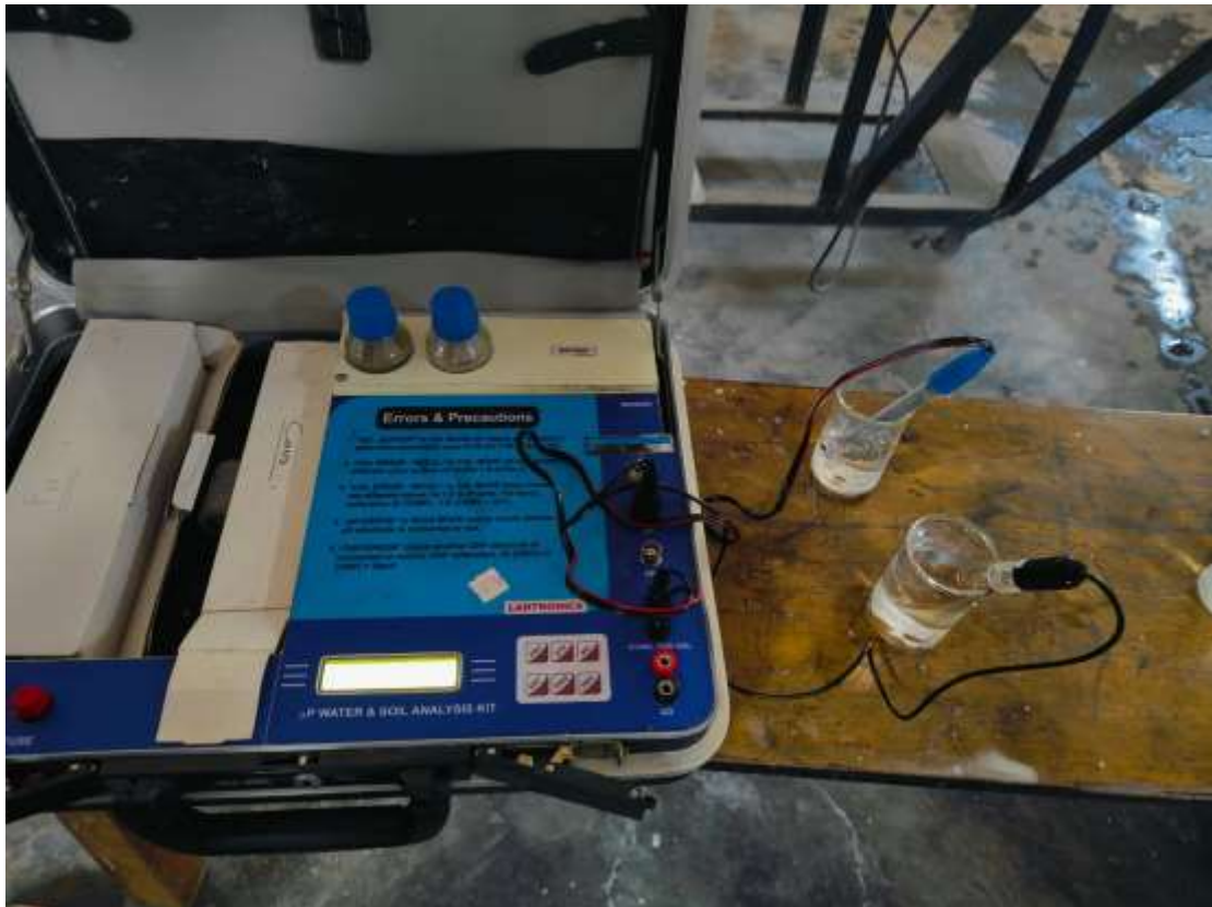
Fig 7- Measuring Salinity with Water Analysis Kit.
