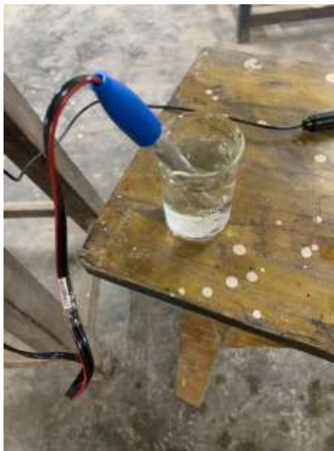
Fig 6- Measuring Conductivity with Water Analysis Kit.
