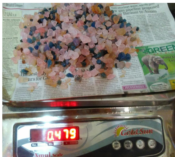
Figure 6.12: Silica gel started reducing in weight (479gm)
