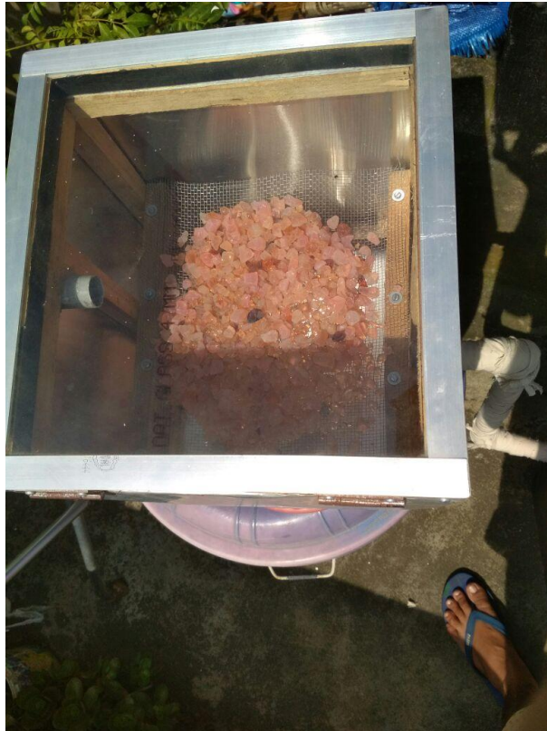
Figure 6.7: Saturated silica gel placed at the regenerating chamber
