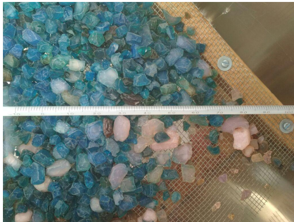
Figure 6.9: Silica gel dried completely with thermometer showing 67°C
