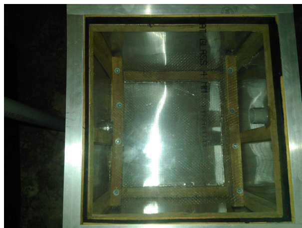
Figure 4.3: Reactivation chamber of first hardware model
