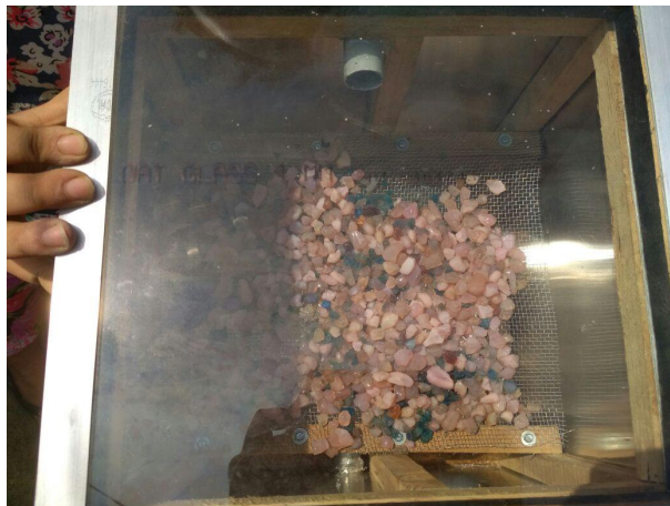
Figure 6.8: Silica gel started srying in the reactivation chamber
