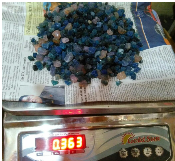
Figure 6.15: Silica gel dried completely (363gm)
