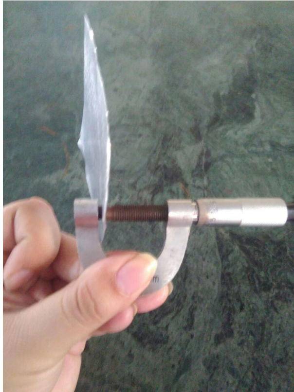
Figure 6.5: measurement of thickness of the aluminium sheet with a screw gauge at the physics laboratory of Assam Engineering College
