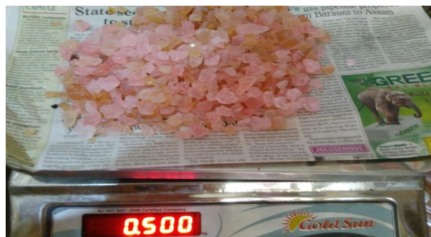
Figure 6.10: Saturated silica gel of 500gm
