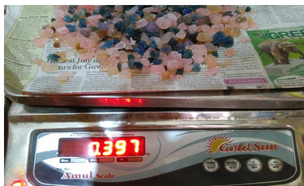
Figure 6.13: Silica gel started reducing in weight (397gm)
