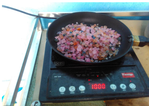
Figure 6.16: Drying of silica gel in an induction plate (electric heating)
