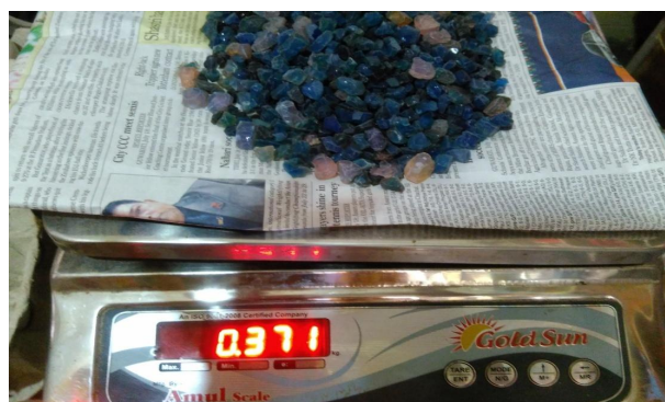
Figure 6.14: Silica gel started reducing in weight (371gm)
