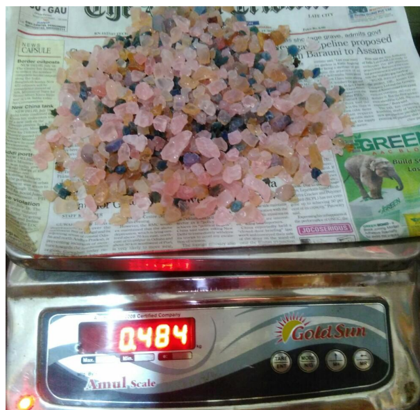
Figure 6.11: Silica gel started reducing in weight (484gm)
