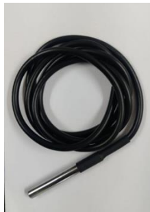
Fig 2.17: DS18B20 Temperature Sensor
