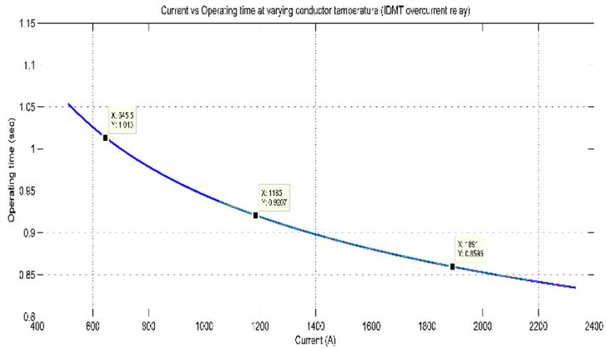
Fig. 5.2: Current Vs Operating time at varying conductor temperature for IDMT overcurrent relay
