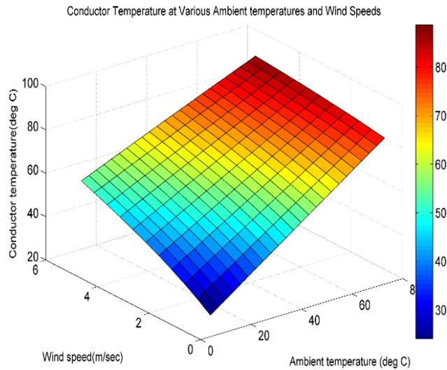
Figure 5.1: Conductor temperature under varying ambient conditions for fixed static rating
