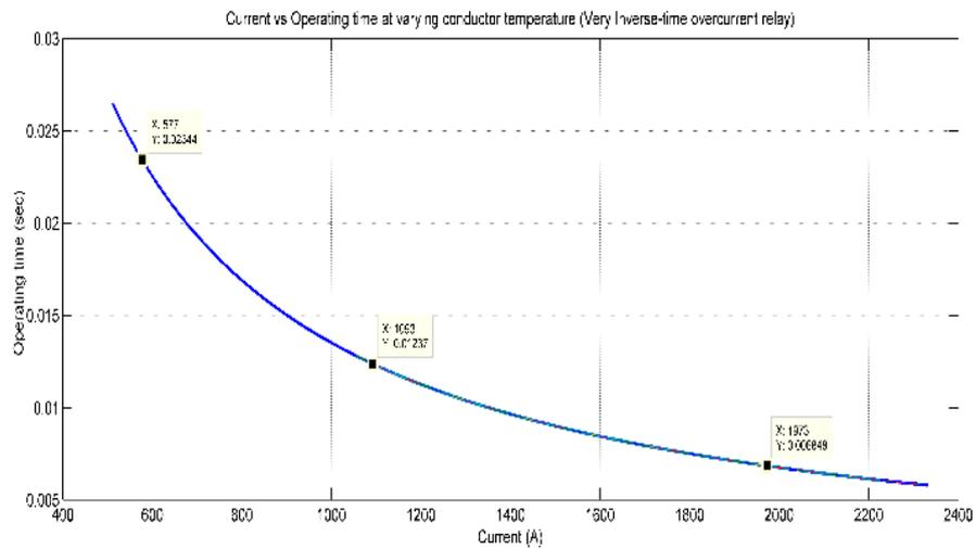
Figure 5.3: Current Vs Operating time at varying conductor temperature for Very inverse overcurrent relay
