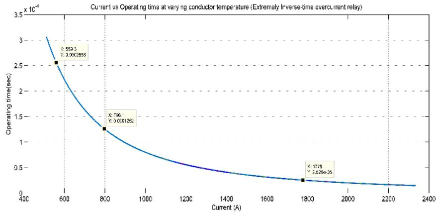
Figure 5.4: Current Vs Operating time at varying conductor temperature for Extremely inverse overcurrent relay
