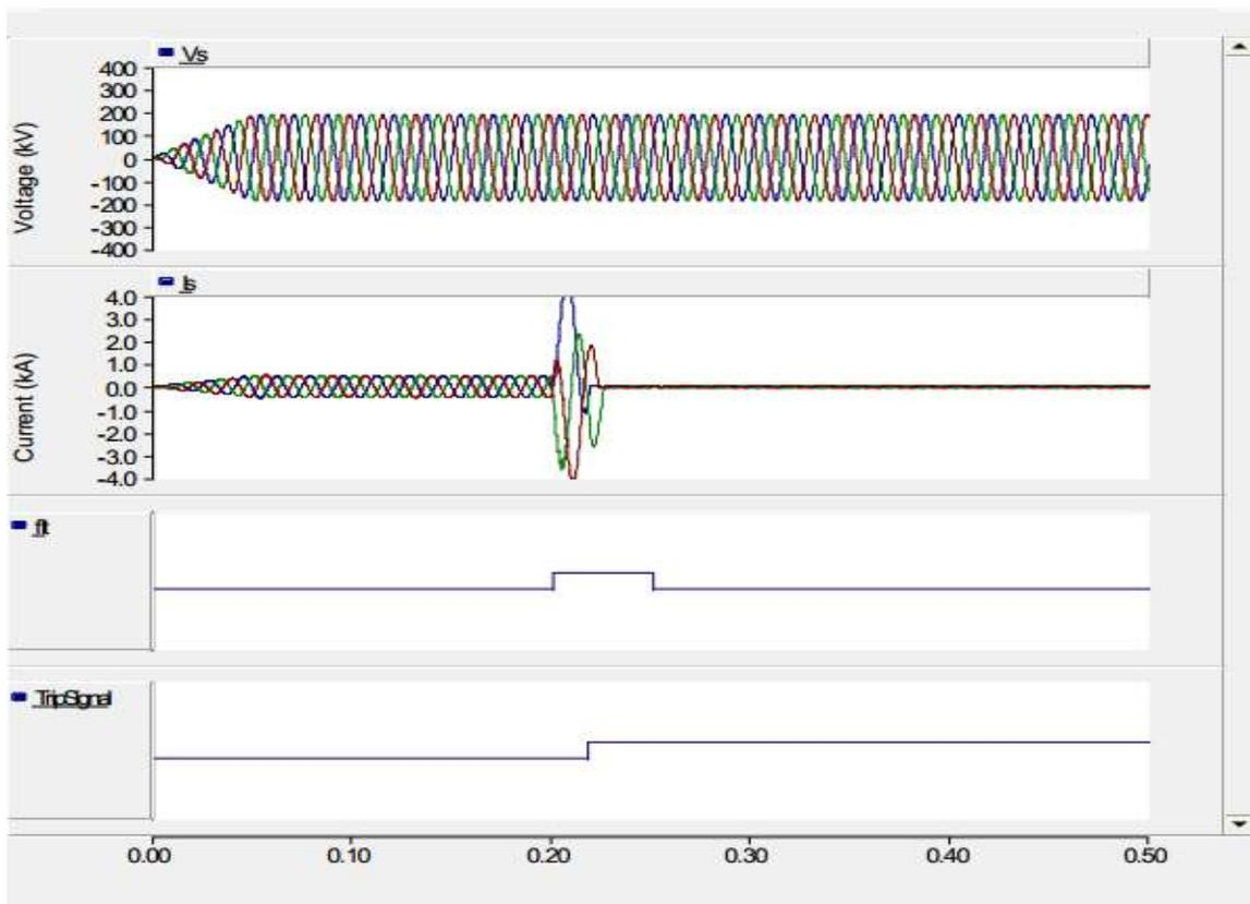
*Fig. 2.23: Variation of Voltage, Current and Trip signal result for STATCOM having LLL fault.*
