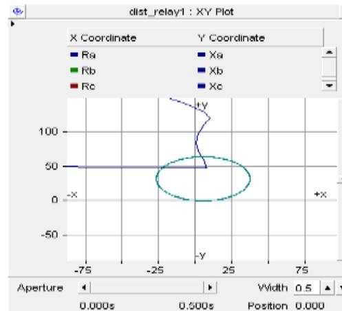
*Fig. 3.2: Result of Distance Relay Operating without mid-point UPFC*
