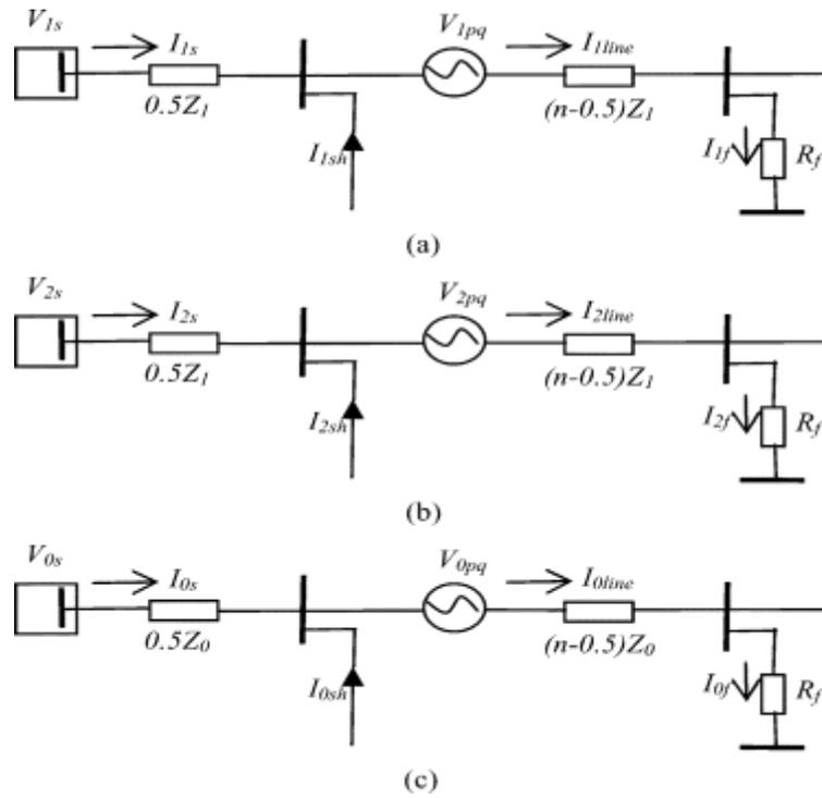
**Fig.3.3: Sequence networks of the system from the relay location to fault. (a) Positive sequence network. (b) Negative sequence network. (c) Zero sequence network.**
