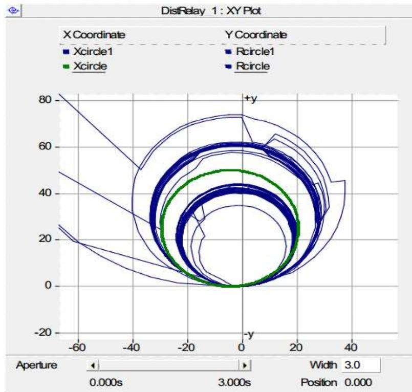
**Fig. 4.6 Adaptive mho relay second zone characteristics with SVC supplying inductive reactive power of 100 MVAR into the system with reverse power flow.**
