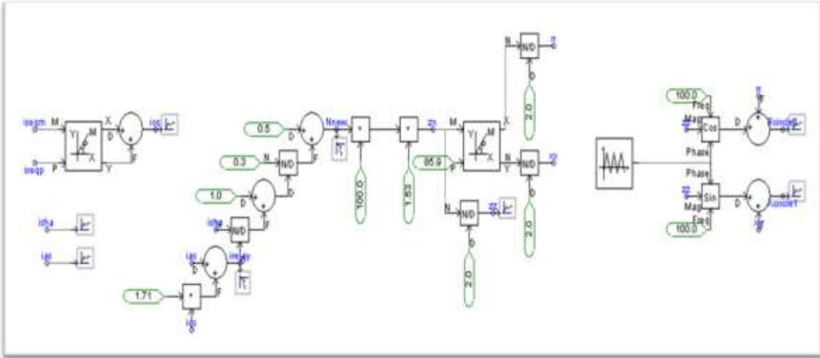
*Figure: Modelling of Adaptive Distance Protection in PSCAD*
