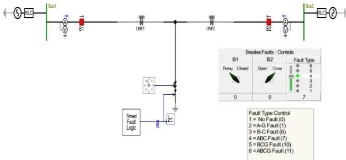
Figure 1.2: A Simple Distance Protection of two bus system with fault timer logic.
