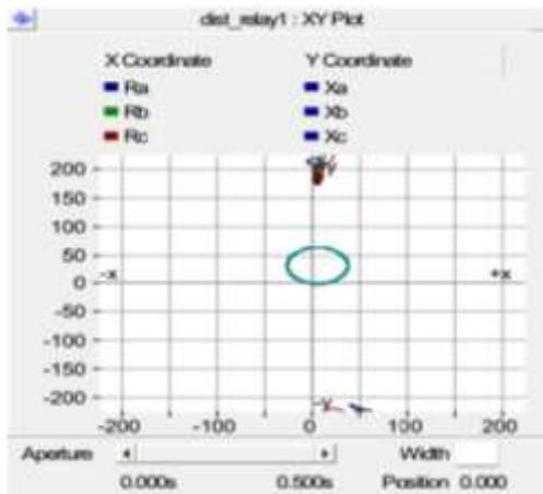
*Fig. 3.1: Result of Distance Relay Operating with mid-point UPFC*
