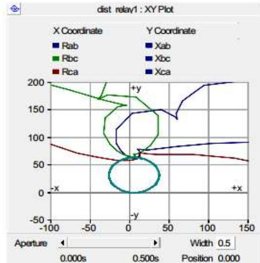
Fig. 2.20: L-L fault for the System having mid-point STATCOM
