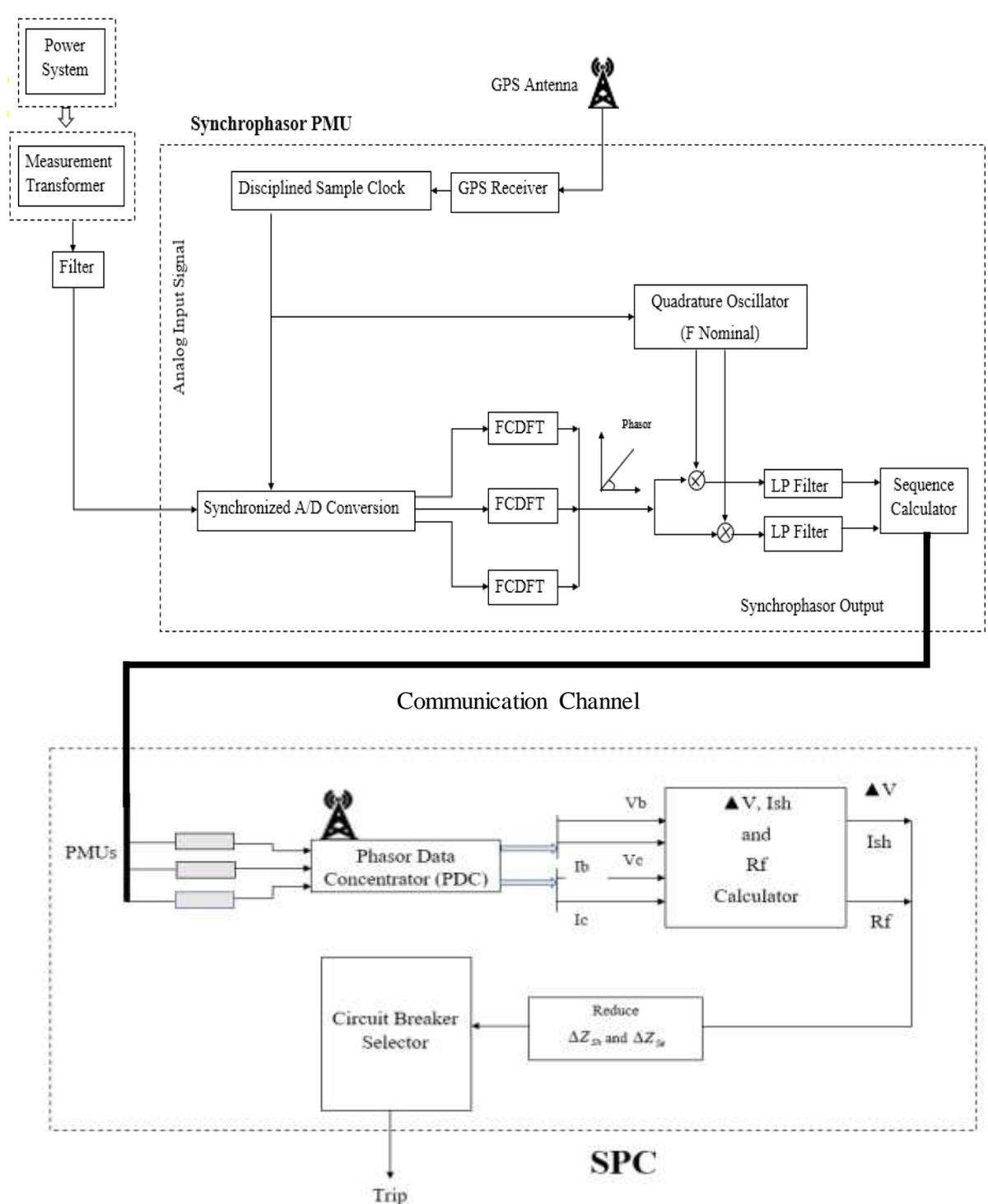
Fig.4.13: The main parts of the new modified method for distance relay
