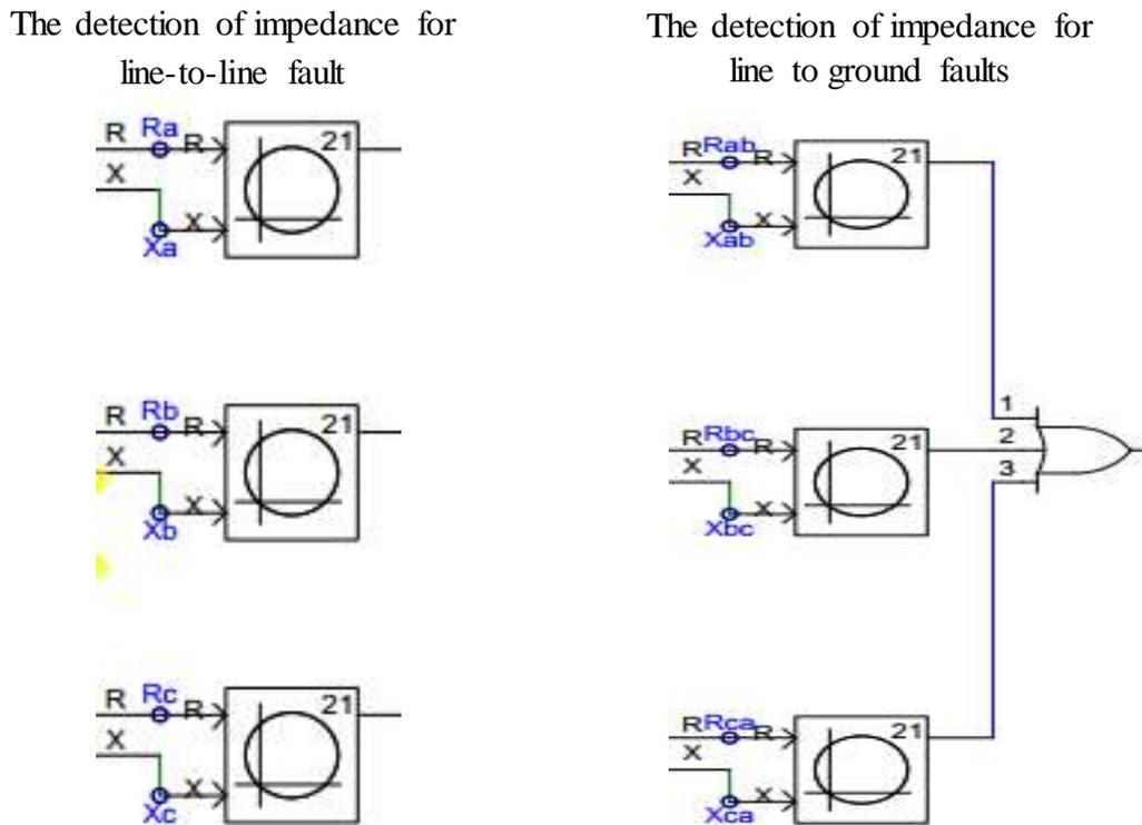
*Figure 1.7: Mho characteristics of distance relay*
