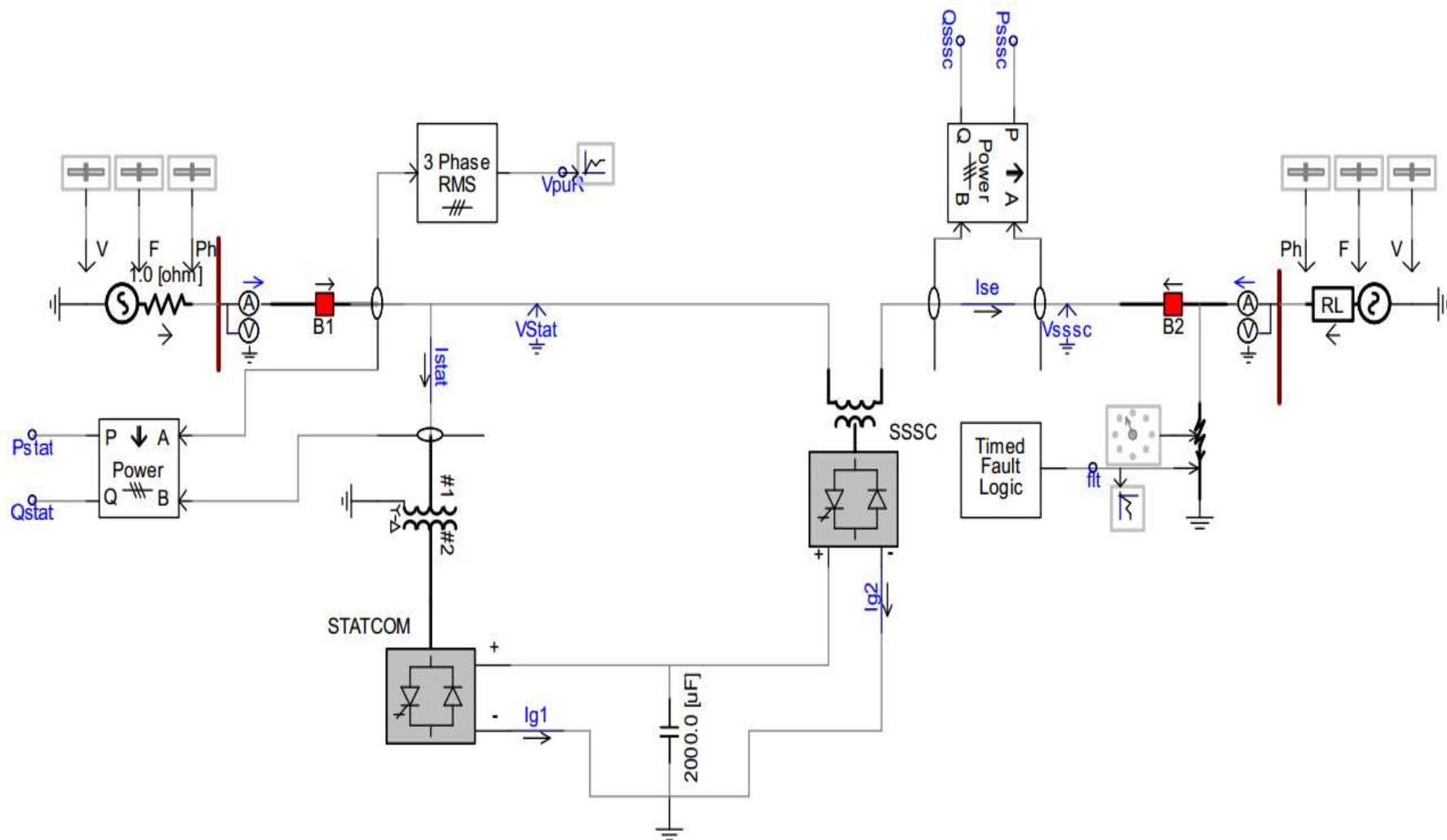
*Fig. 3.4: Distance protection setting in presence of mid-point UPFC*
