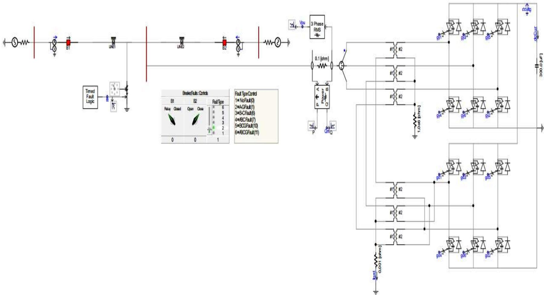
Fig. 2.6: Distance protection setting in presence of mid-point STATCOM
