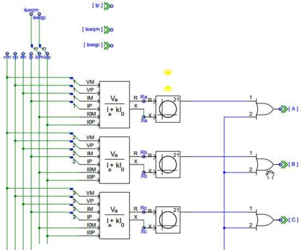
Figure 1.5: Calculation for line-to-line Impedance block
