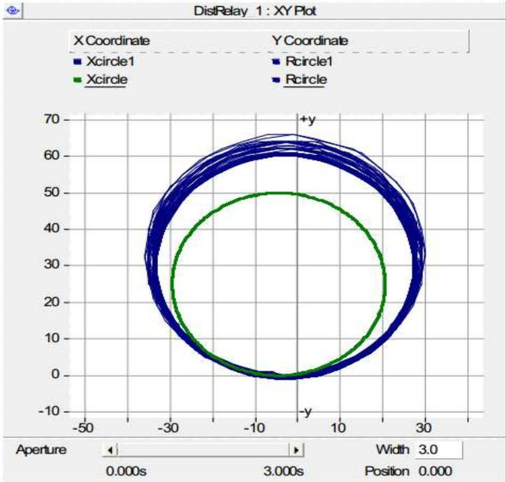
Fig.4.8: Adaptive distance protection mho relay characteristics with STATCOM supplying inductive reactive power of 100 MVAR into the system with forward power flow from A to B.
