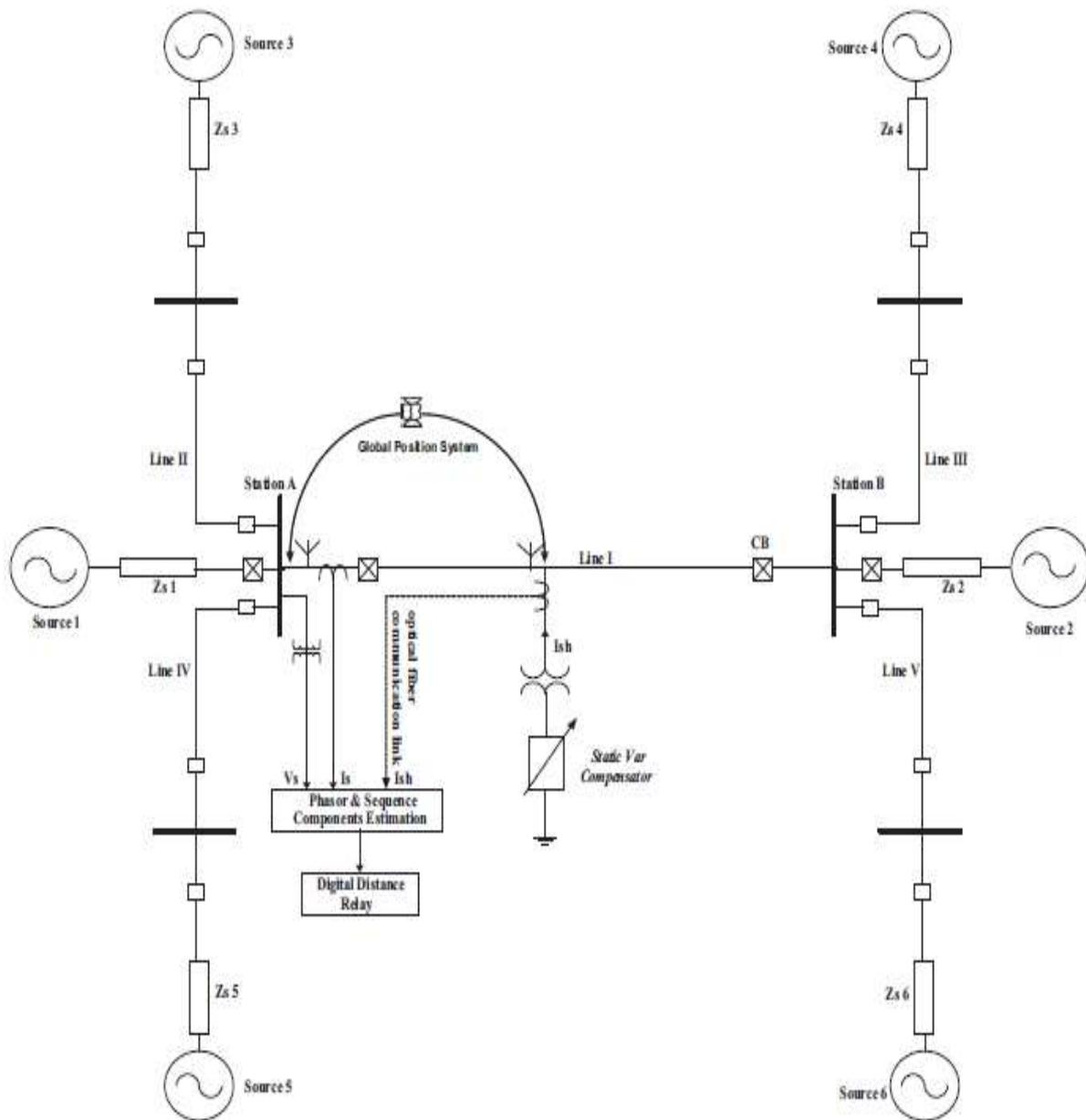
*Fig. 4.1. Single line diagram of study system model with mid-point SVC*
