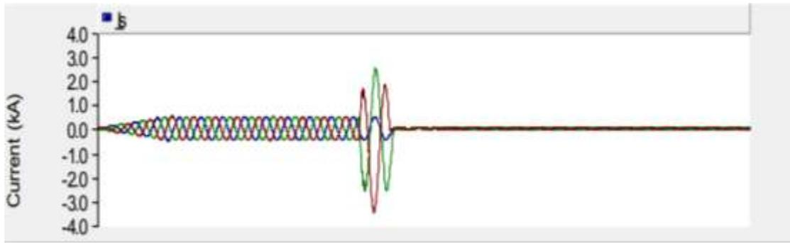
*Fig. 2.26: Variation of current for STATCOM having L-L fault.*
