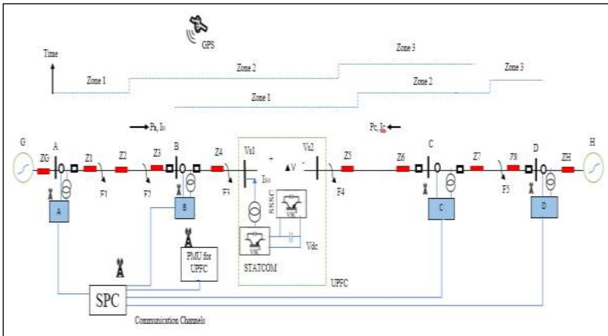
*Fig.4.12: Single-line diagram of multi-line system with UPFC*
