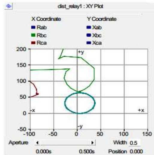
Fig. 2.22: LL-G fault for the System having mid-point STATCOM
