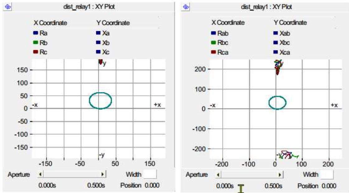
*Fig. 3.5: The apparent impedance seen by the distance relay during a L-G phase fault*
