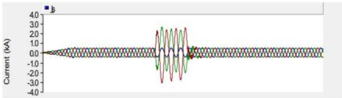
*Fig. 2.24: Variation of current for STATCOM having L-L-G fault.*
