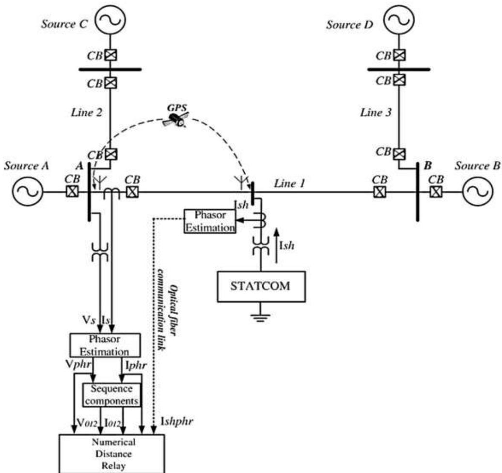
Fig. 4.7: Single line diagram of study system model
