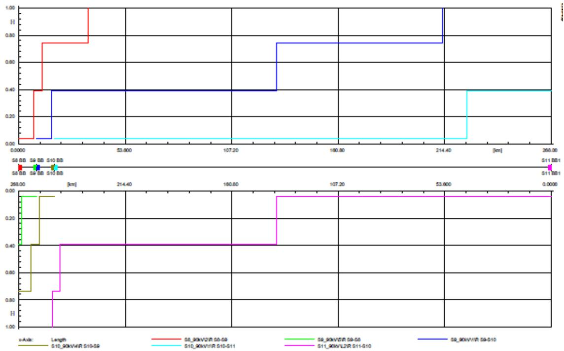
**Figure: Result of Distance Relay Operation for Three Zone Protection, Zone 1 = 80km (red), Zone 2 =120km (blue), Zone 3= 180km(violet) in DIGSILENT PowerFactory Software.**
