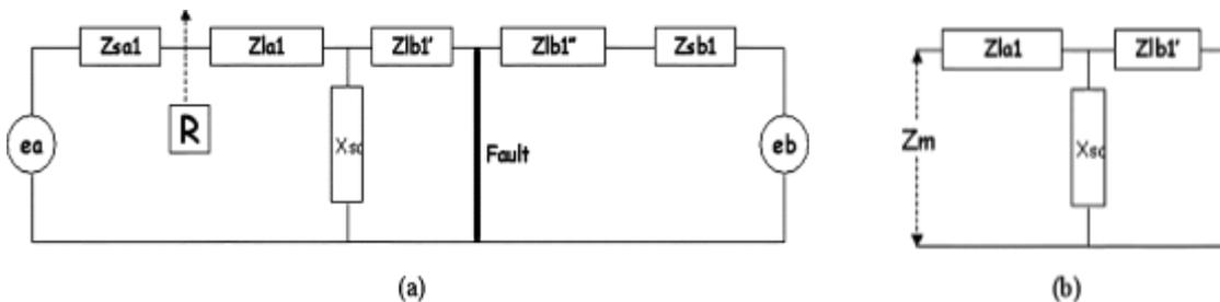
Fig.2. 3: (a) Equivalent circuit for 3 phase faults; (b) reduced equivalent circuit.
