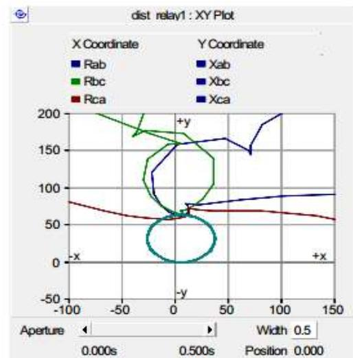
Fig. 2.21: LLL-G fault for the System having mid-point STATCOM
