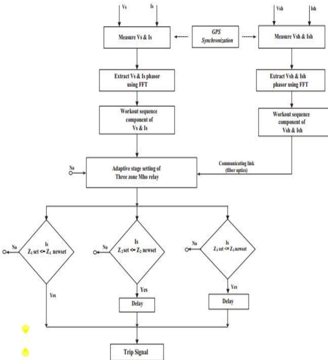
Fig. 4.2. Flow Chart of three zones adaptive distance with mid-point SVC
