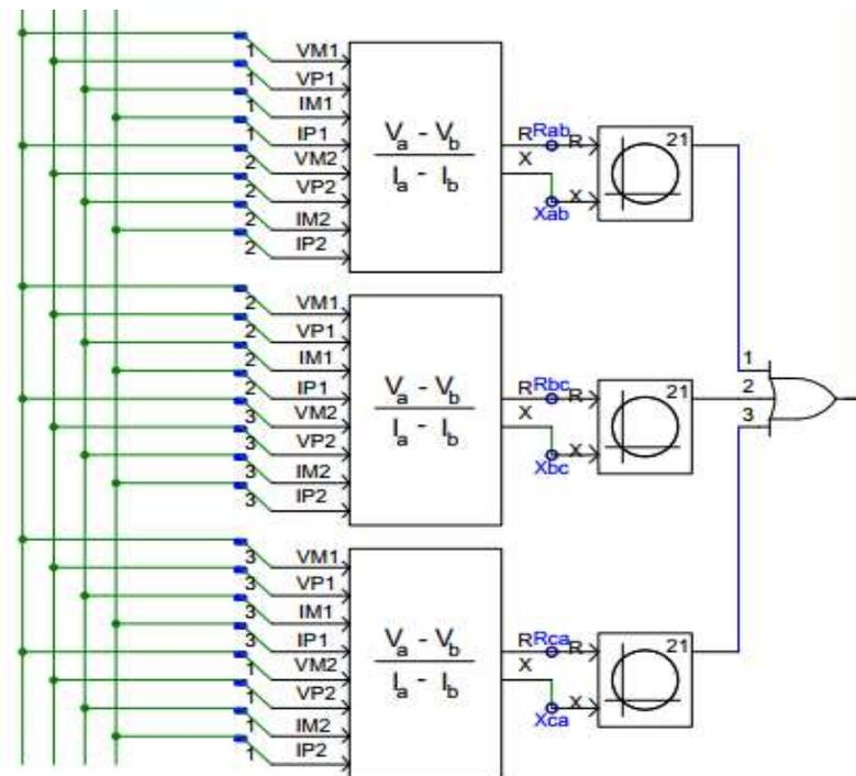
Figure 1.6: Calculation for line to ground impedance block
