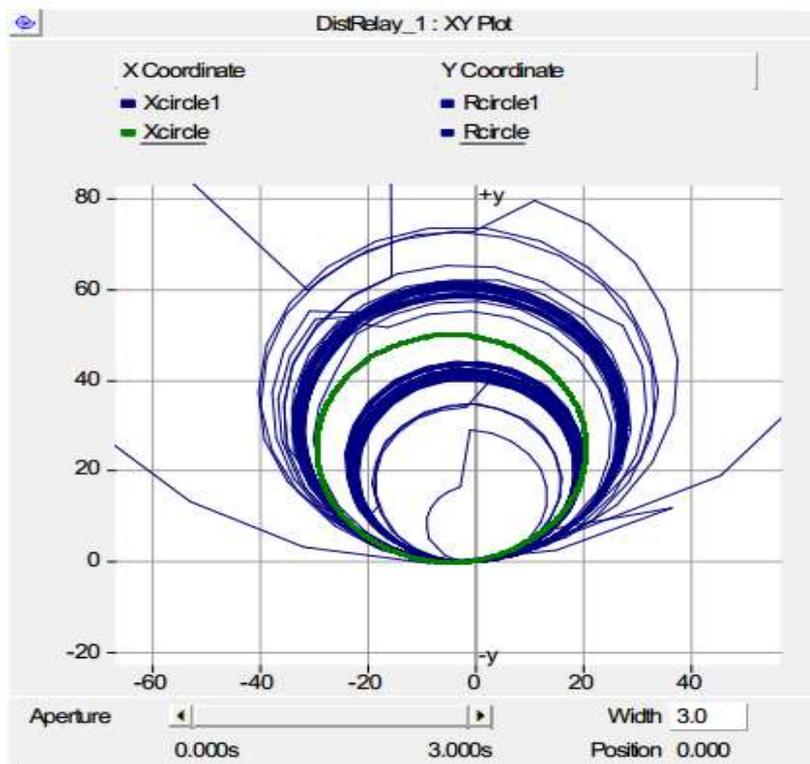
*Fig. 4.5 Adaptive mho relay second zone characteristics with SVC supplying capacitive reactive power of 100 MVAR into the system with reverse power flow.*
