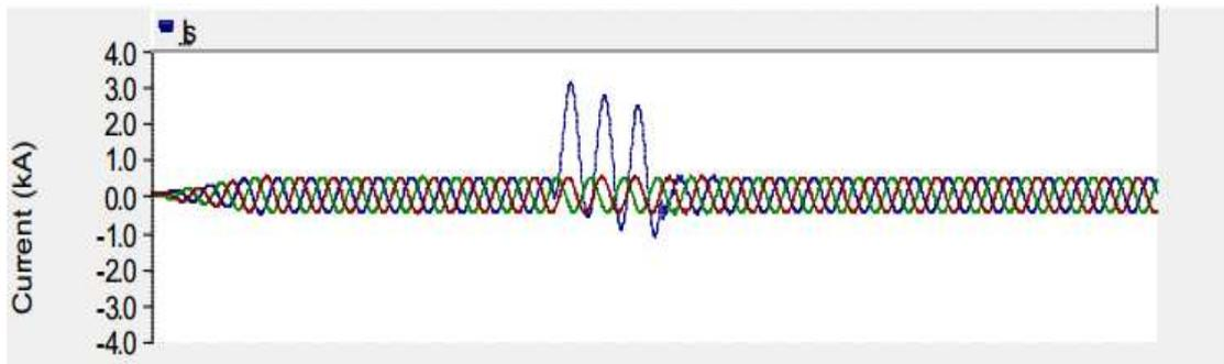
*Fig. 2.27: Variation of current for STATCOM having L-G fault.*
