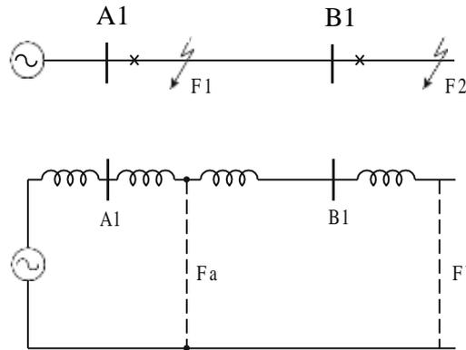
Figure 1.1: Faults occurring on different parts of a power system
