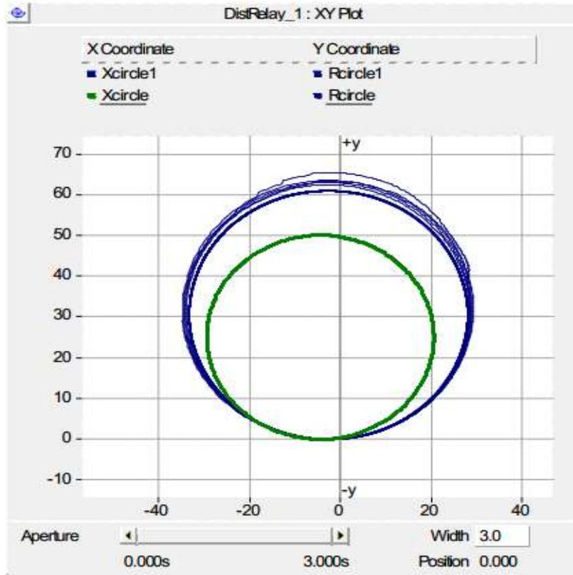
*Fig. 4.4 Adaptive mho relay second zone characteristics with SVC supplying capacitive reactive power of 100 MVAR into the system with forward power flow.*
