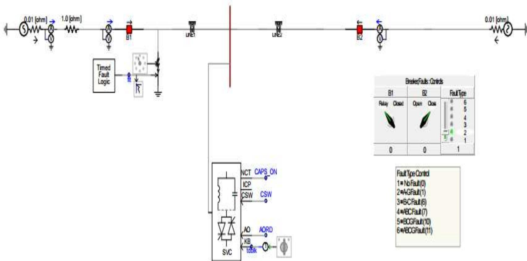
Fig. 2.5: Distance protection setting in presence of mid-point SVC
