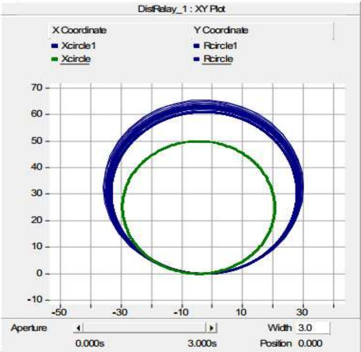
Fig.4.9: Adaptive distance protection mho relay characteristics with STATCOM supplying capacitive reactive power of 100 MVAR into the system with forward power flow from A to B.
