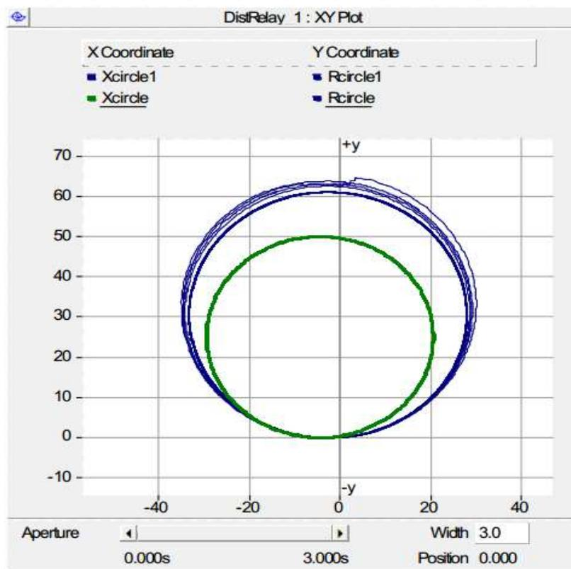
*Fig. 4.3 Adaptive mho relay second zone characteristics with SVC supplying inductive reactive power of 100 MVAR into the system with forward power flow.*
