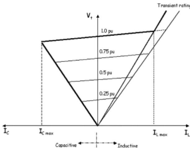
Fig. 2.1: V-I characteristics of a SVC.
