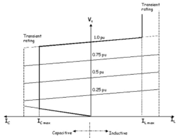
Fig. 2.2: V-I characteristics of a STATCOM.
