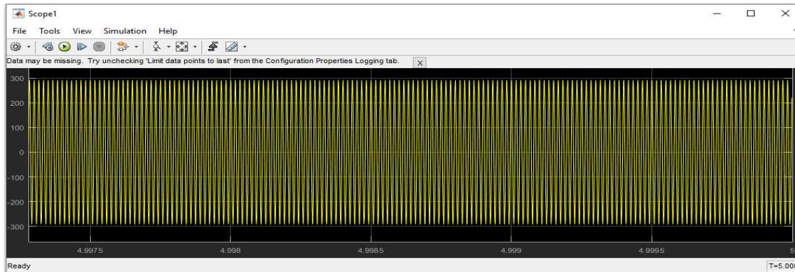
Figure 5.19 Graph of V of RIWPT system with coupling coefficient(k) of 0.8827 and R=35\text{ ohm}
