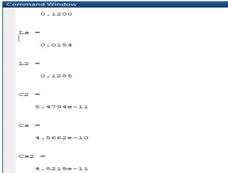
Figure 4.10 Results of parameters of matching network for RIWPT for 2.5 cm coil radius
