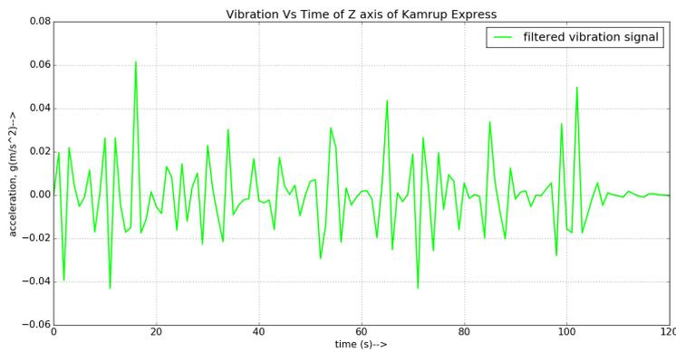
Fig. 2.12 Filtered Vibration signal of Z axis of Kamrup Express
