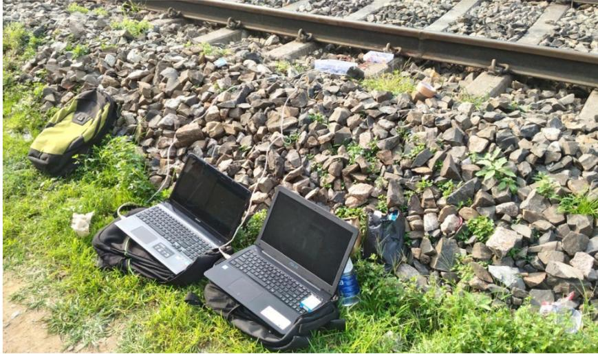
Fig. 3.2 Experimental set-up for capturing 3-D vibration signals from railway track.
