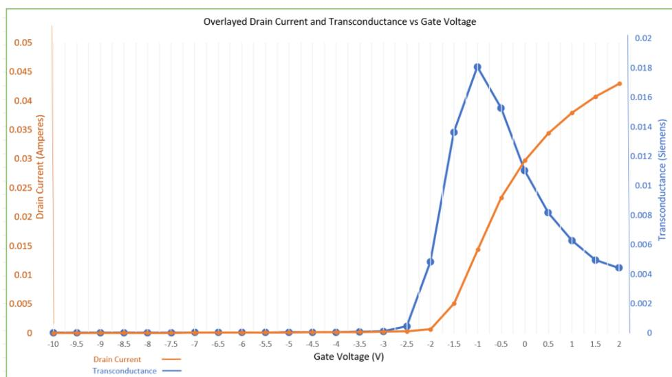
Fig-4.4: Transconductance and Drain current w.r.t. Gate Voltage of AlGaIn/GaN HEMT
