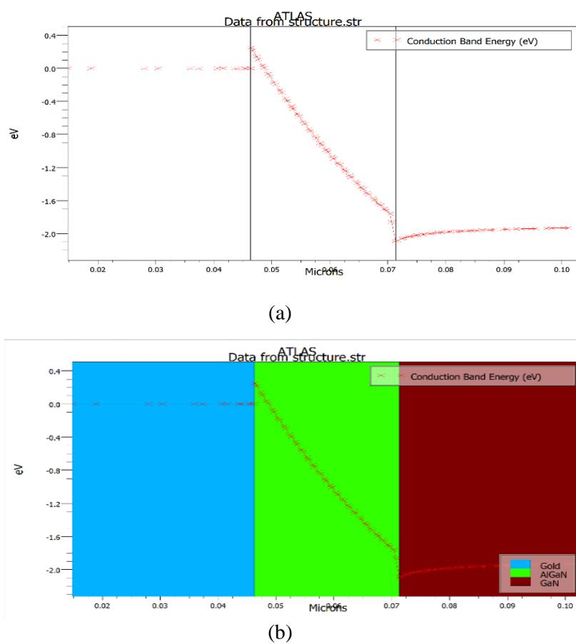
Fig-4.5 (a) and (b): Bending of the conduction band resulting in the formation of 2DEG
