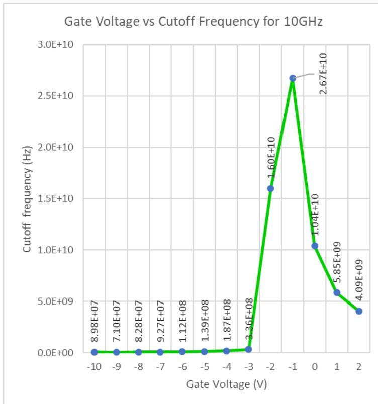
Fig-7.6: Plot depicting cut-off frequency obtained for input signal of 10 GHz
