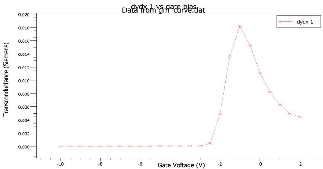
Fig-4.3: Transconductance curve of AlGaIn/GaN HEMT on SiC substrate
