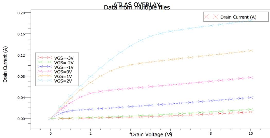
Fig-4.2: Output characteristics AlGaIn/GaN HEMT on SiC substrate
