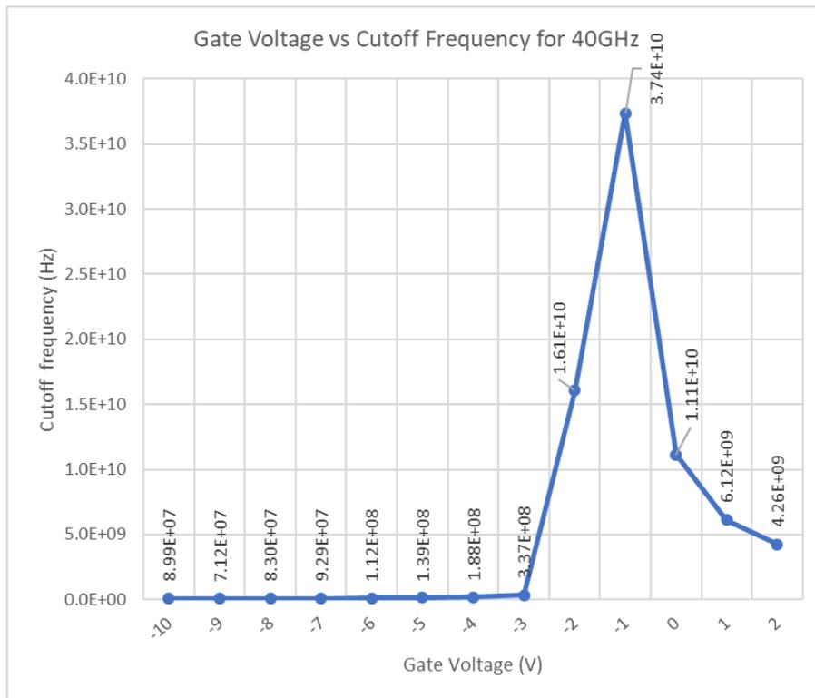
Fig-7.8: Plot depicting cut-off frequency obtained for input signal of 40 GHz
