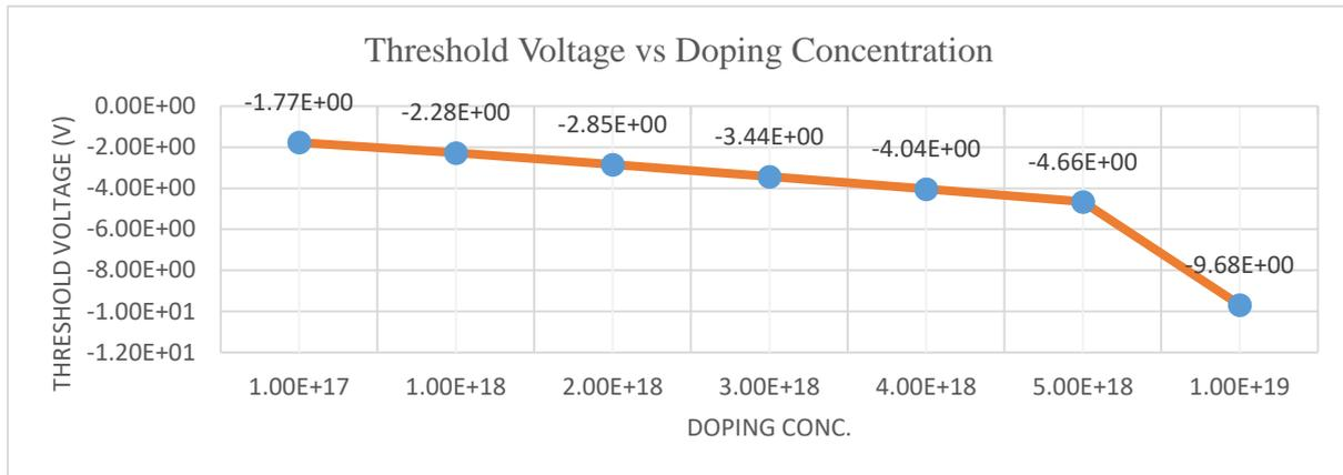
Fig-5.2: Plot showing the variation of threshold voltage ( $V_{th}$ ) w.r.t. doping conc. of AlGaN
