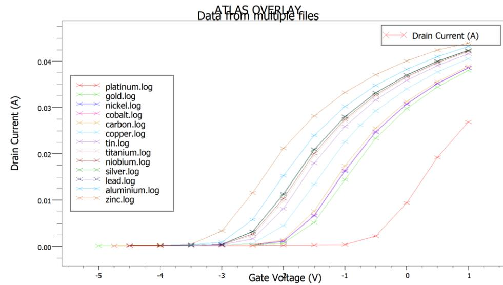
Fig-5.8: Combined transfer characteristics of the device using various gate materials
