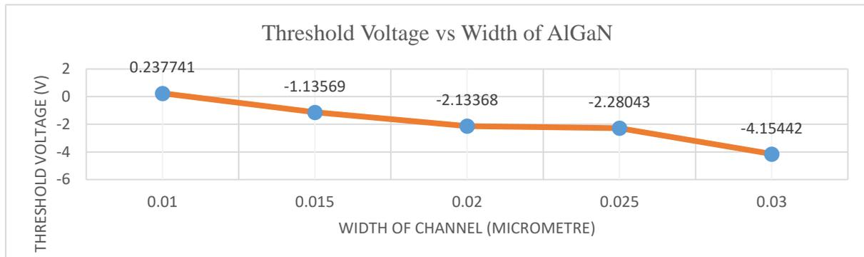
Fig-5.1: Plot showing the variation of threshold voltage ( $V_{th}$ ) w.r.t. width of AlGa<sub>N</sub>
