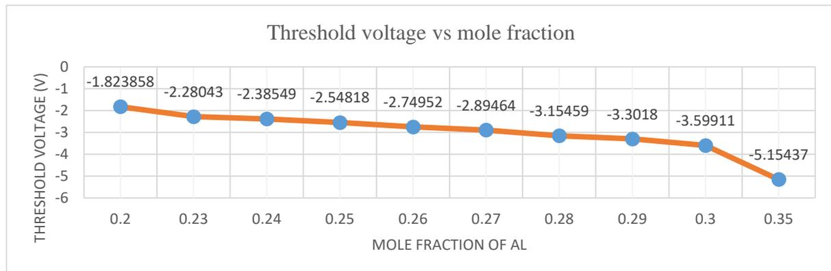
Fig-5.5: Plot showing the variation of threshold voltage ( $V_{th}$ ) w.r.t. mole fraction of Al in AlGaN
