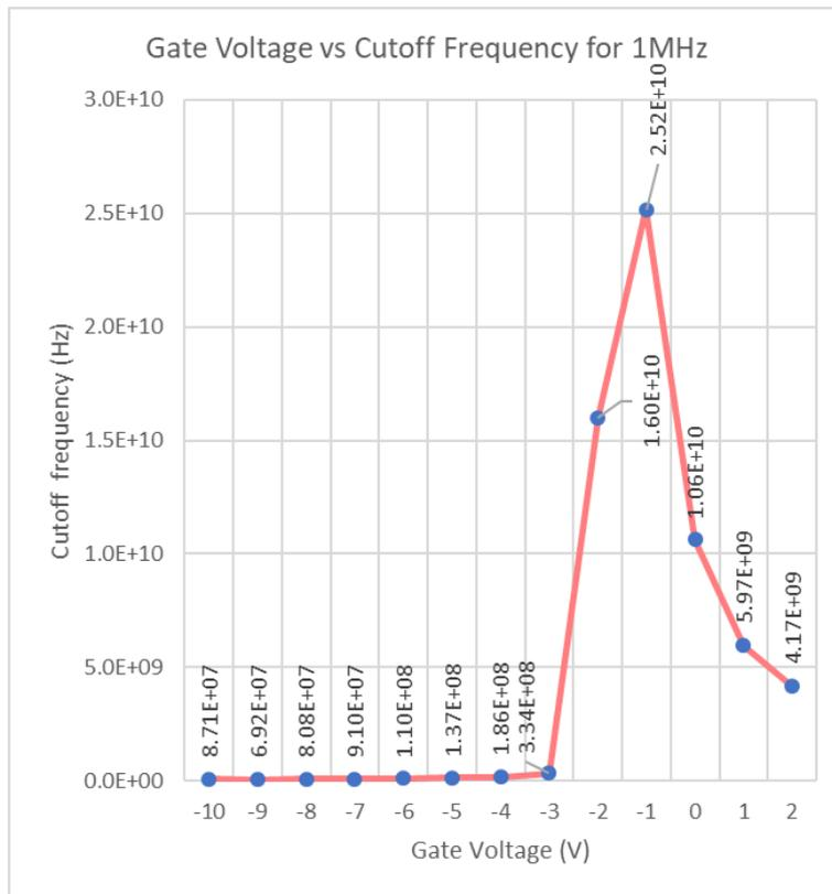
Fig-7.4: Plot depicting cut-off frequency obtained for input signal of 1 MHz
