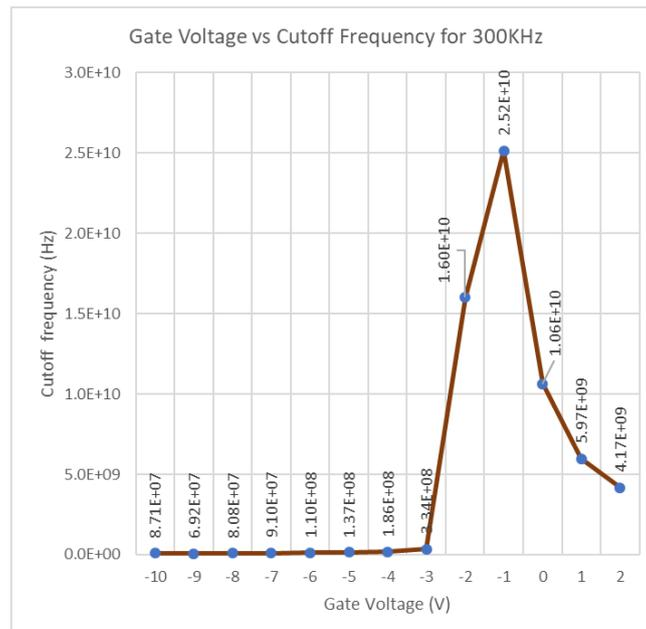
Fig-7.2: Plot depicting cut-off frequency obtained for input signal of 300 KHz
