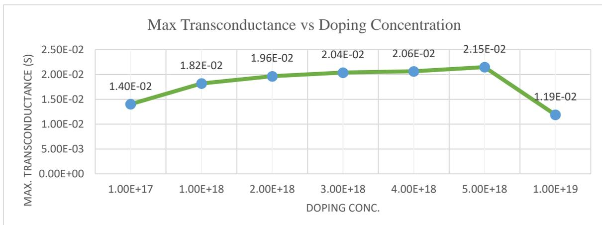
Fig-5.4: Plot showing the variation of peak transconductance ( $g_m$ ) w.r.t. doping conc. of AlGaN
