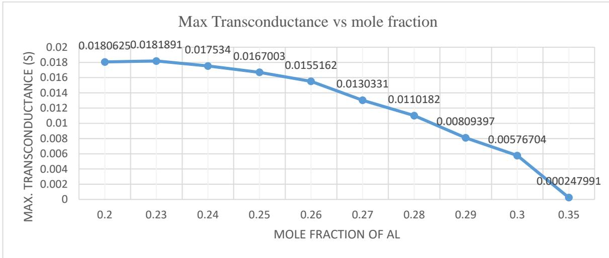
Fig-5.7: Plot showing the variation of max. transconductance w.r.t. mole fraction of Al in AlGa<sub>N</sub>
