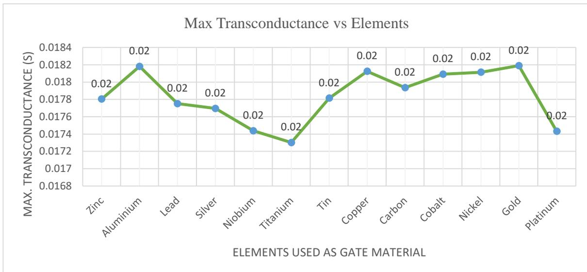
Fig-5.10: Plot showing the variation of max. transconductance w.r.t. different gate materials used
