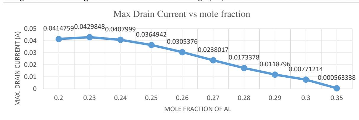
Fig-5.6: Plot showing the variation of maximum. drain current w.r.t. mole fraction of Al in AlGa<sub>N</sub>
