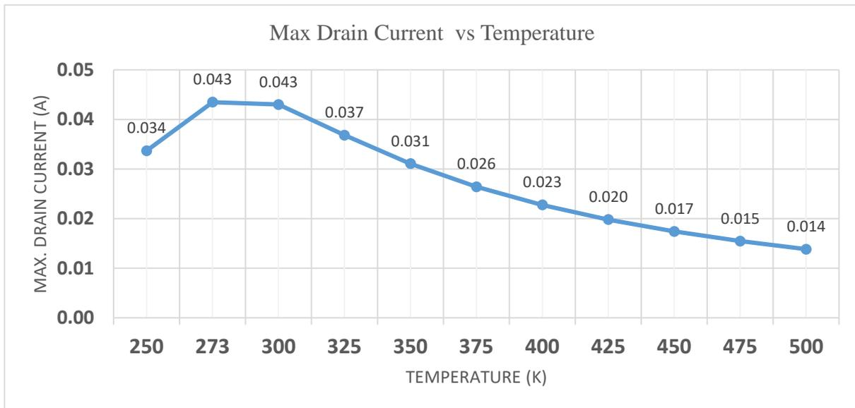
Fig-6.2: Plot showing the max. drain current w.r.t. temperature
