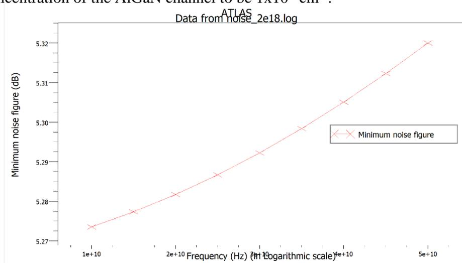
Fig-7.11: Plot for variation of  $NF_{min}$  w.r.t. frequency from 10-50 GHz for doping conc. of AlGaN channel to be  $2 \times 10^{18} \text{cm}^{-3}$
