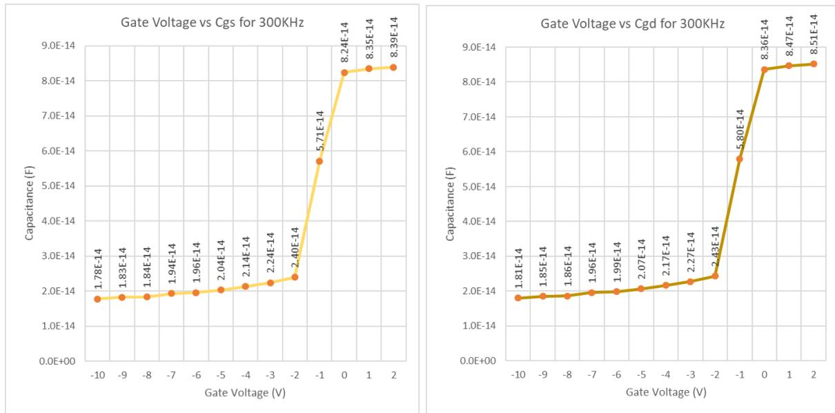
Fig-7.1: Plots depicting the  $C_{GS}$  and  $C_{GD}$  obtained for input signal of 300 KHz
