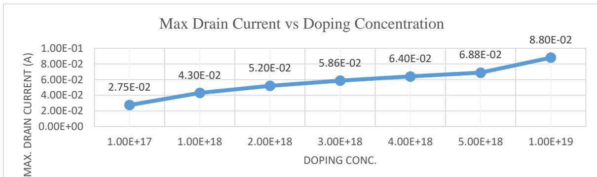
Fig-5.3: Plot showing the variation of maximum drain current (at  $V_{GS}=2\text{V}$ ) w.r.t. doping conc. of AlGaN
