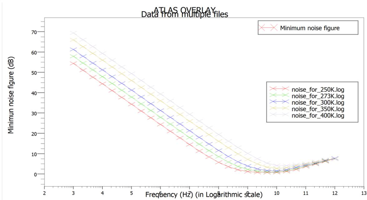
Fig-6.4: Plot showing the noise figure w.r.t. temperature
