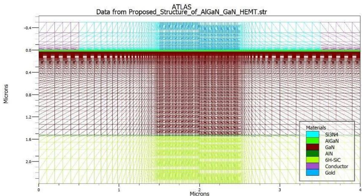
Fig-3.3: Mesh diagram of the proposed structure
