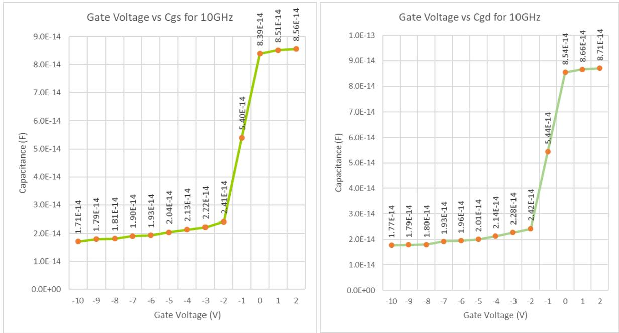
Fig-7.5: Plots depicting the  $C_{GS}$  and  $C_{GD}$  obtained for input signal of 10 GHz
