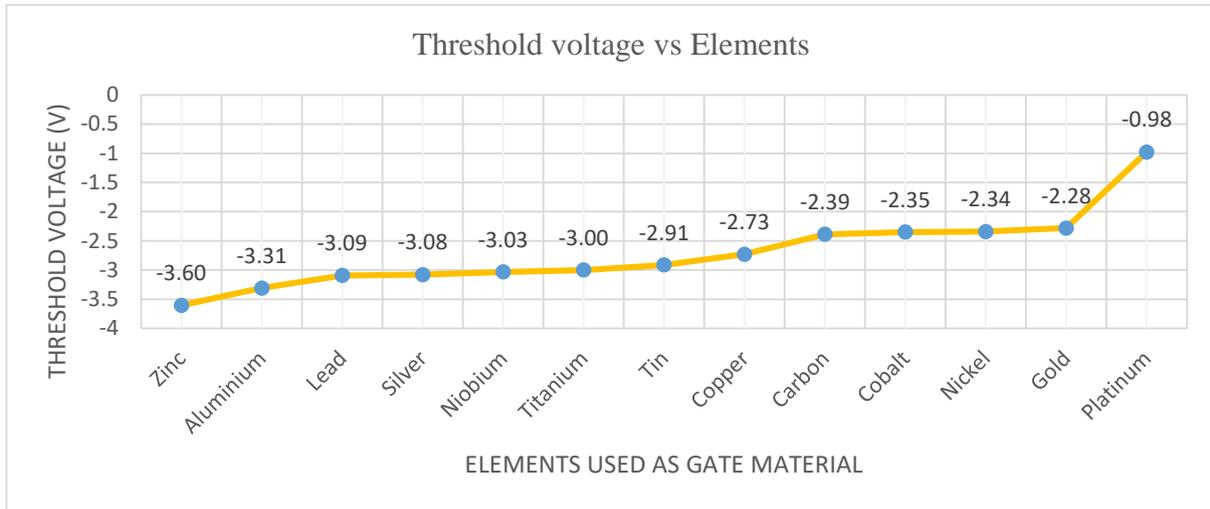
Fig-5.9: Plot showing the variation of threshold voltage w.r.t. different gate materials used
