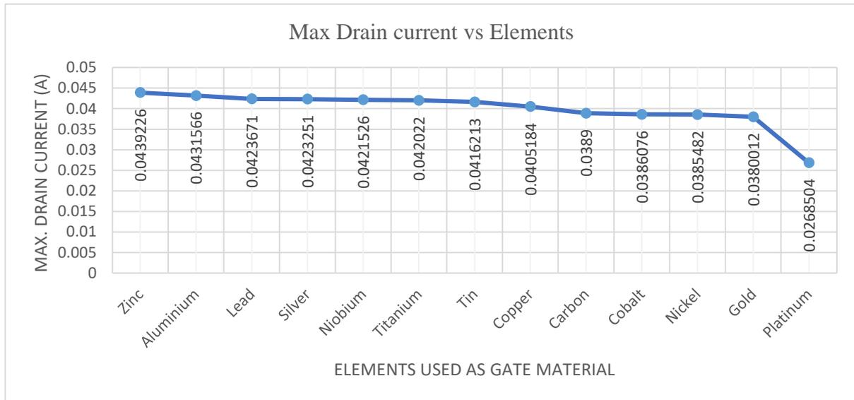
Fig-5.11: Plot showing the variation of max. drain current w.r.t. different gate materials used
