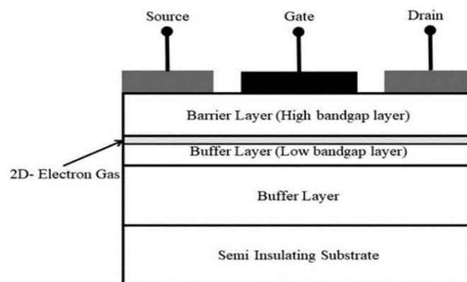
Fig-1.1: Basic cross section of HEMT
