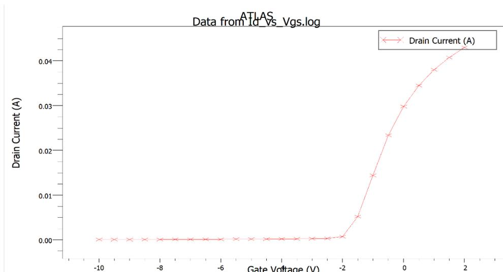
Fig-4.1: Transfer characteristics of AlGa<sub>N</sub>/Ga<sub>N</sub> HEMT on SiC substrate
