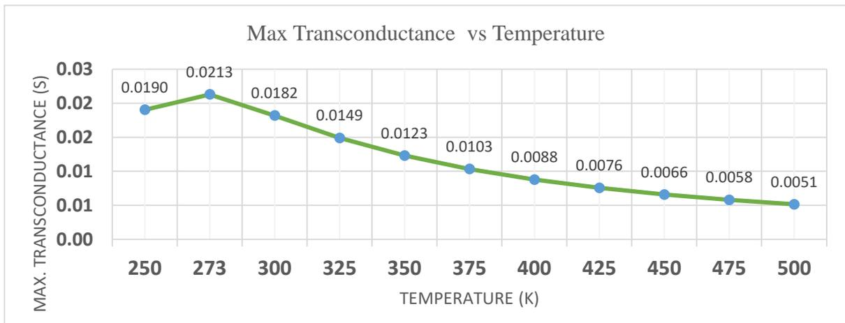
Fig-6.3: Plot showing the peak transconductance w.r.t. temperature
