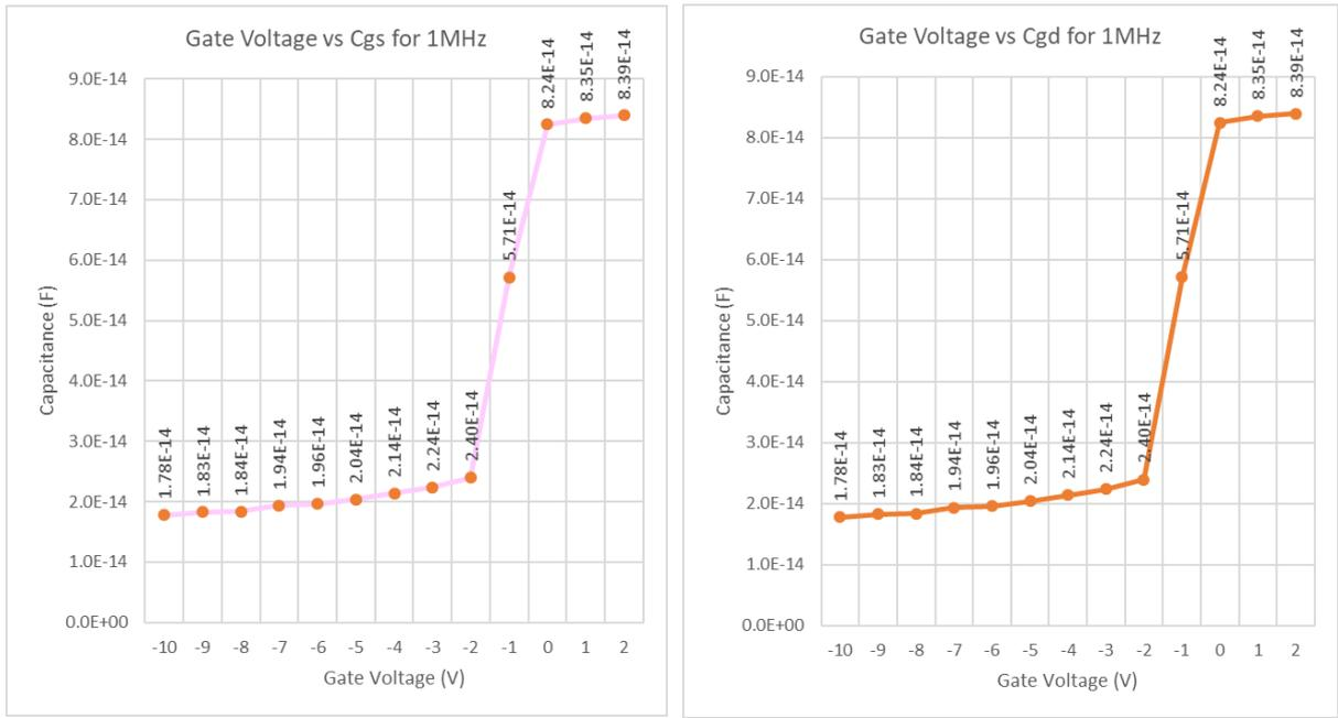
Fig-7.3: Plots depicting the  $C_{GS}$  and  $C_{GD}$  obtained for input signal of 1 MHz
