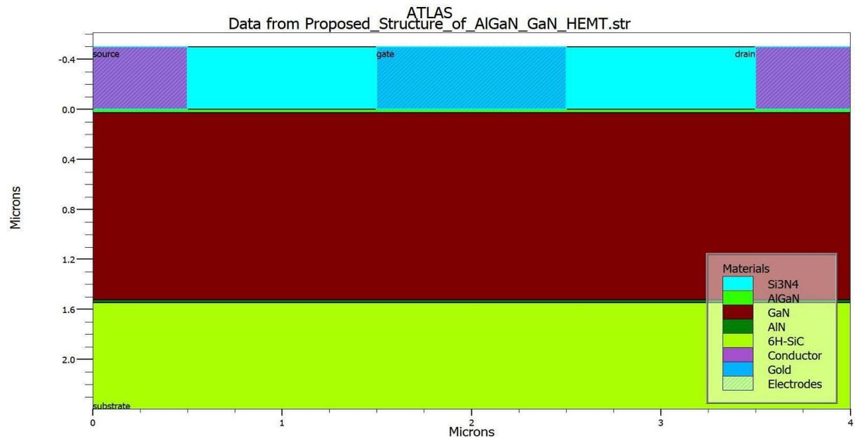
Fig-3.2: Proposed structure of AlGaN/GaN HEMT device
