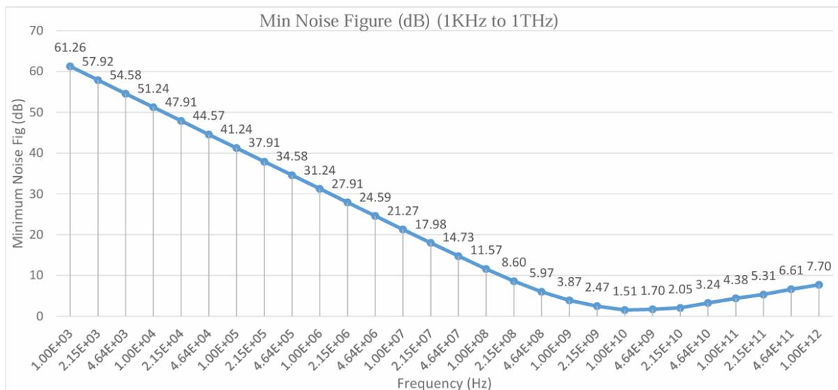
Fig-7.9: Plot for variation of  $NF_{min}$  w.r.t. frequency at the input
