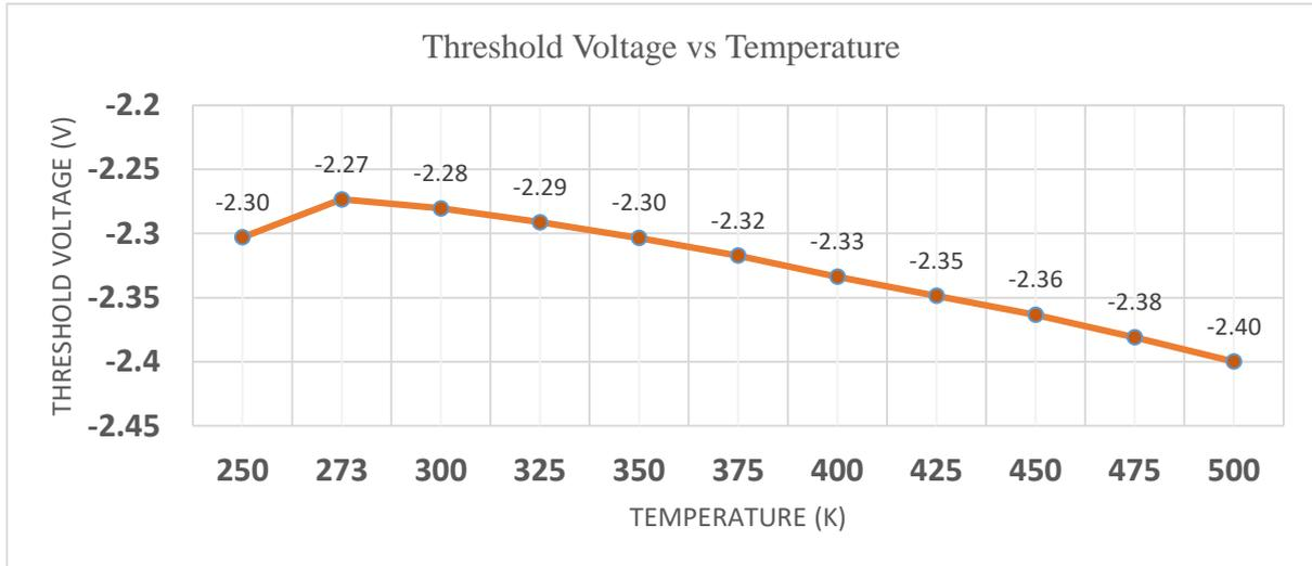
Fig-6.1: Plot showing the variation of threshold voltage w.r.t. temperature
