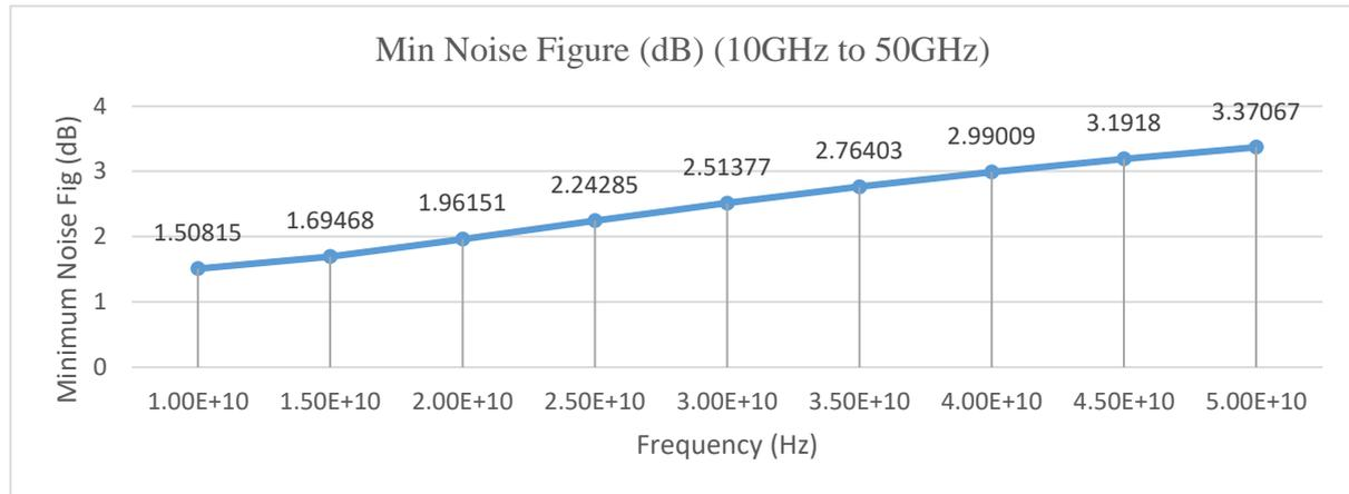
Fig-7.10: Plot for variation of  $NF_{min}$  w.r.t. frequency from 10-50 GHz
