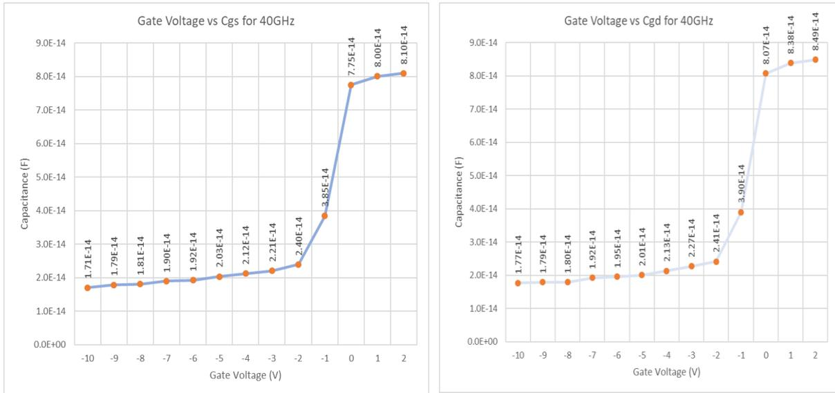
Fig-7.7: Plots depicting the C<sub>GS</sub> and C<sub>GD</sub> obtained for input signal of 40GHz
