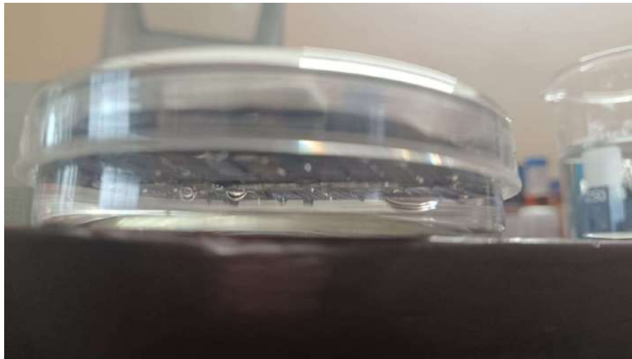
Fig 3.5 Immerring the solar plate in equimolar solution Zinc Nitrate Hexahydrate and Hexamethylenetetramine (HMT).
