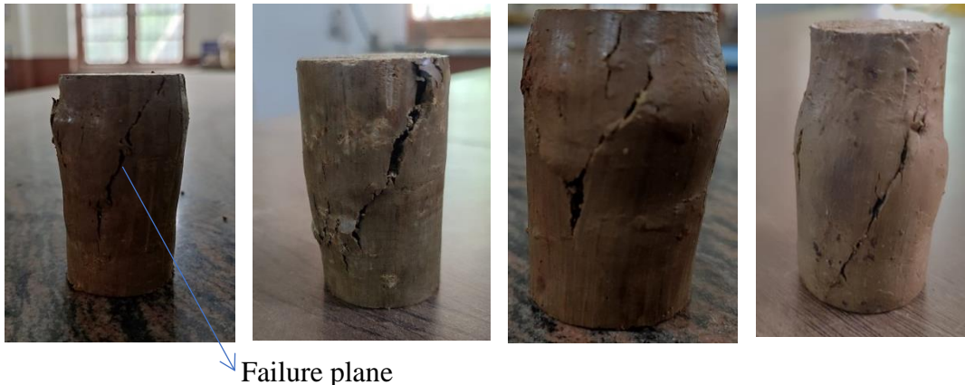
Fig 3.17 The above pictures shows the sample after failure at different waste percentages
