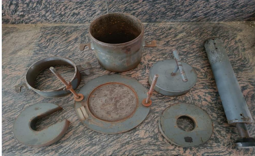
Fig 3.20 CBR mould, base plate, collar, spacer disc, surcharge, rammer
