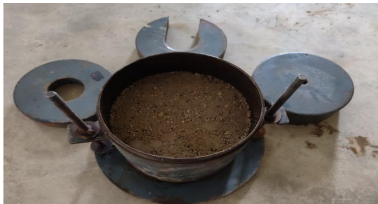
Fig 3.18 Compacted CBR mould with soil, spacer disc, surcharge
