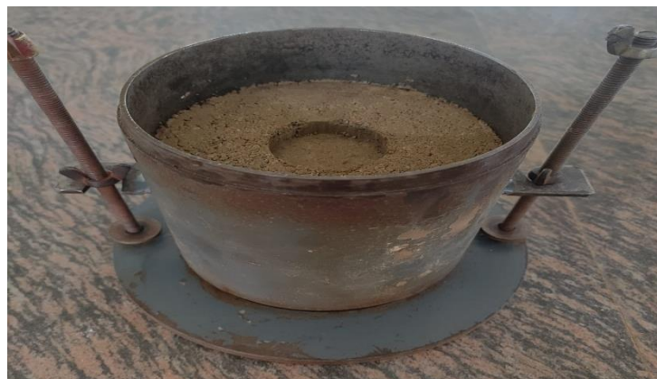
Fig 3.19 Compacted soil with CBR mould after load penetration
