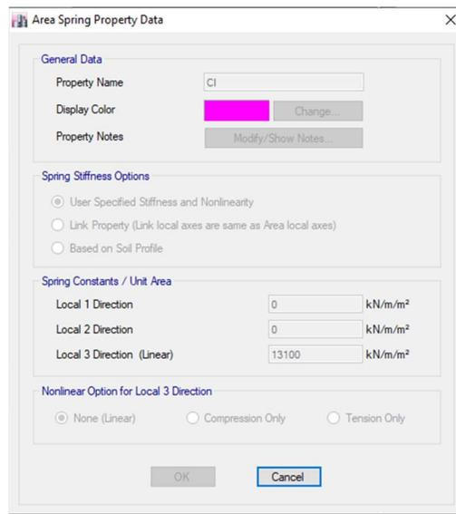
**Figure 6.5.** Application of Modulus of Subgrade with Area Spring
