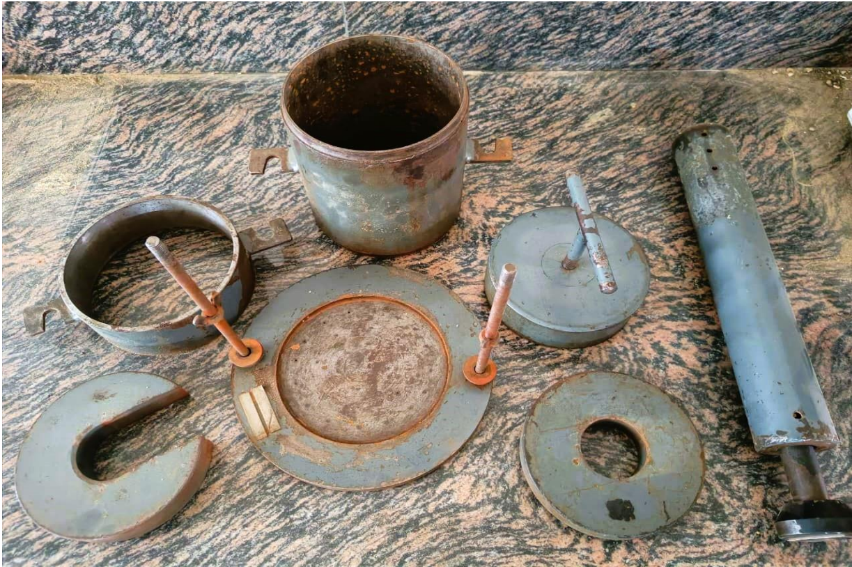
Figure 3.1: Base plate, collar, spacer disc, mould, 2.6 kg rammer, surcharge load 2.5 kg each used in California Bearing Ratio test
