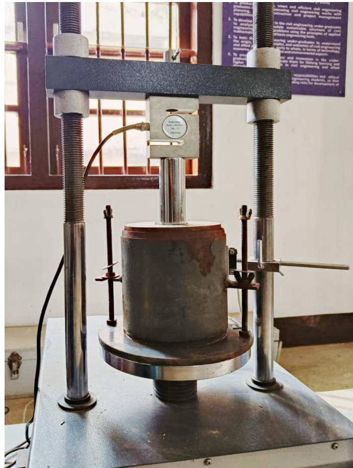
Figure 3.3: Test set up for California Bearing Ratio test
