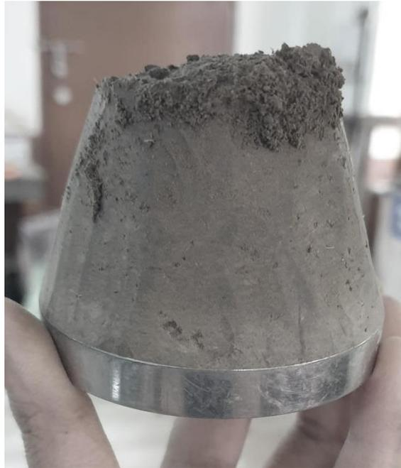
**Figure 3.4:** Recovered soil sample from the Proctor mould
