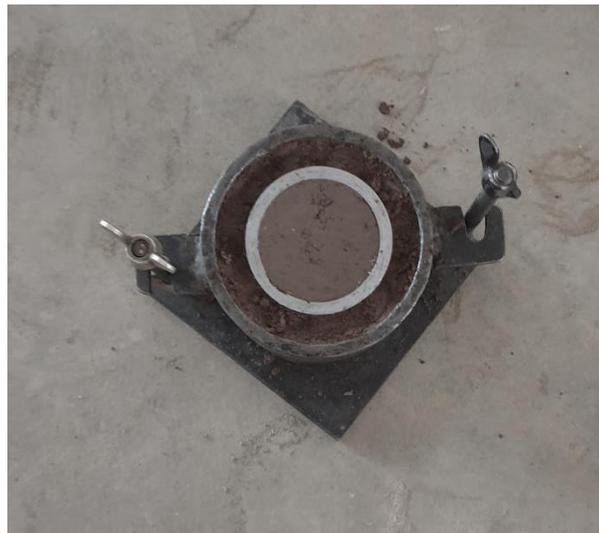
**Figure 3.3:** Insertion of consolidation ring in compacted soil mass
