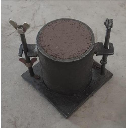
**Figure 3.2:** Dynamically Compacted Soil at Dry of Optimum
