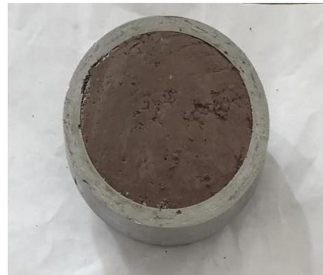
**Figure 3.6:** Lower surface of consolidation sample
