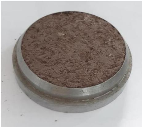
**Figure 3.5:** Upper surface of consolidation sample
