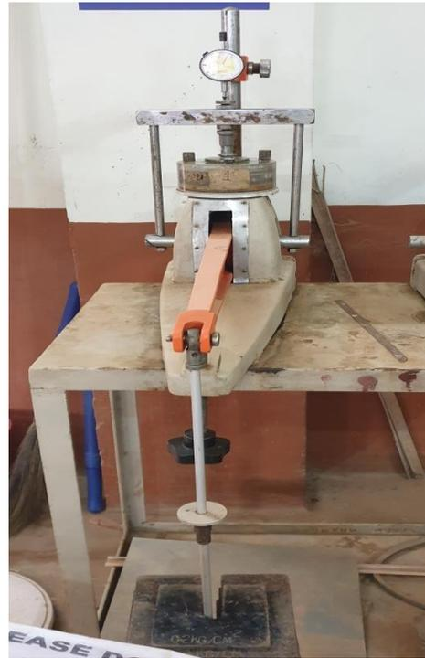
**Figure 3.8:** The whole consolidation setup
