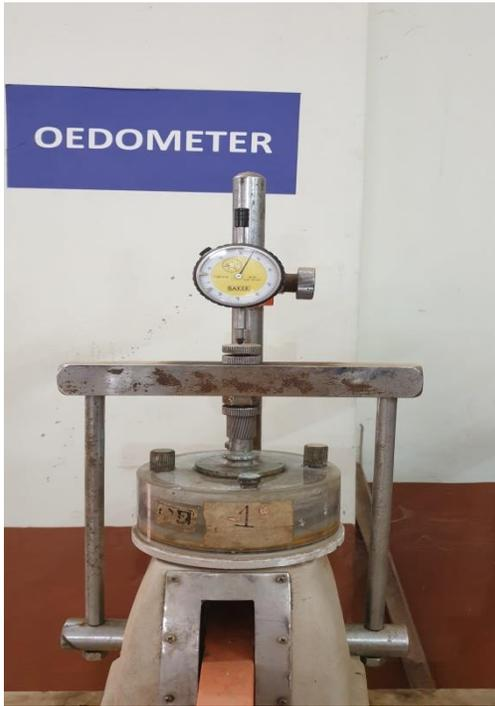
**Figure 3.7:** Consolidation cell under the loading frame
