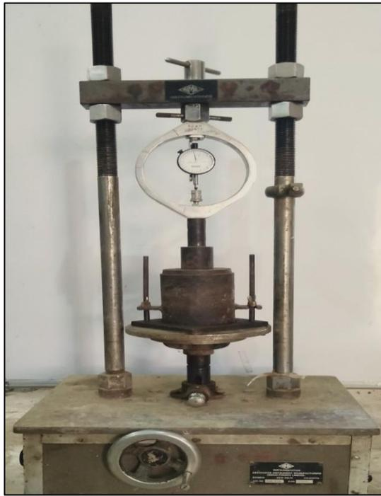
**Figure 3.1** Static Compaction Test Set up
