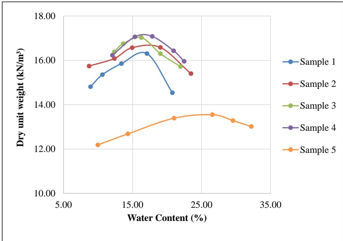
**Figure 4.1 Compaction curve for SLM and native soil**
