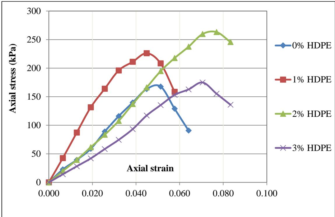
Figure 4.10 super-imposed stress-strain curve of sample 5 at different percentage of HDPE
