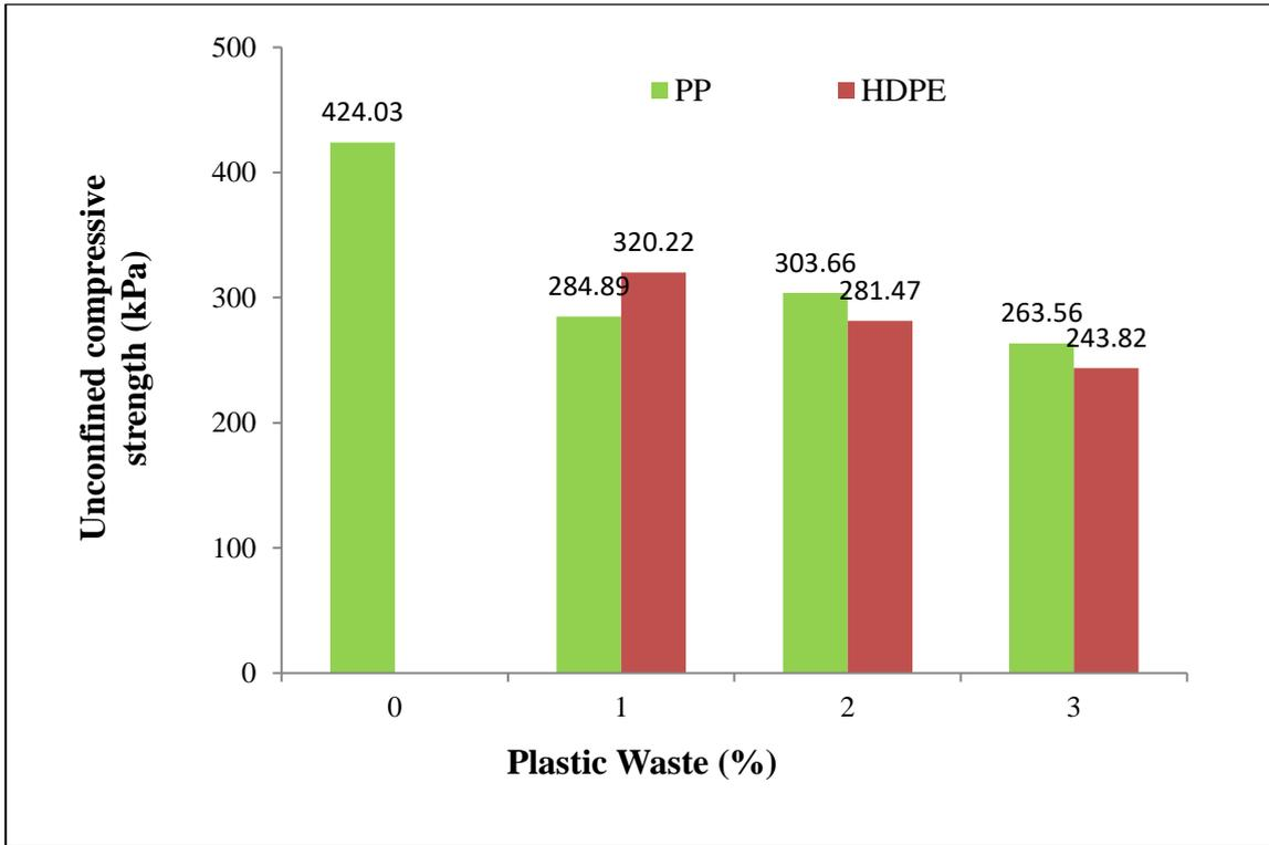
**Figure 4.14 Plastic waste (PP & HDPE) vs UCS of sample 1**
