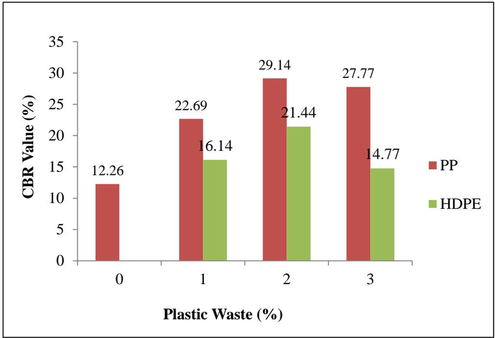
**Figure 4.31: Plastic waste vs CBR of Sample 2 for both PP and HDPE**
