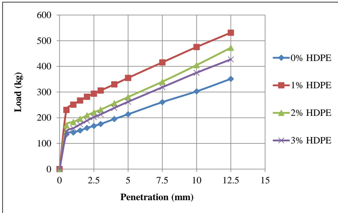
Figure 4.26: Superimposed curves of load vs penetration for Sample 2 with HDPE
