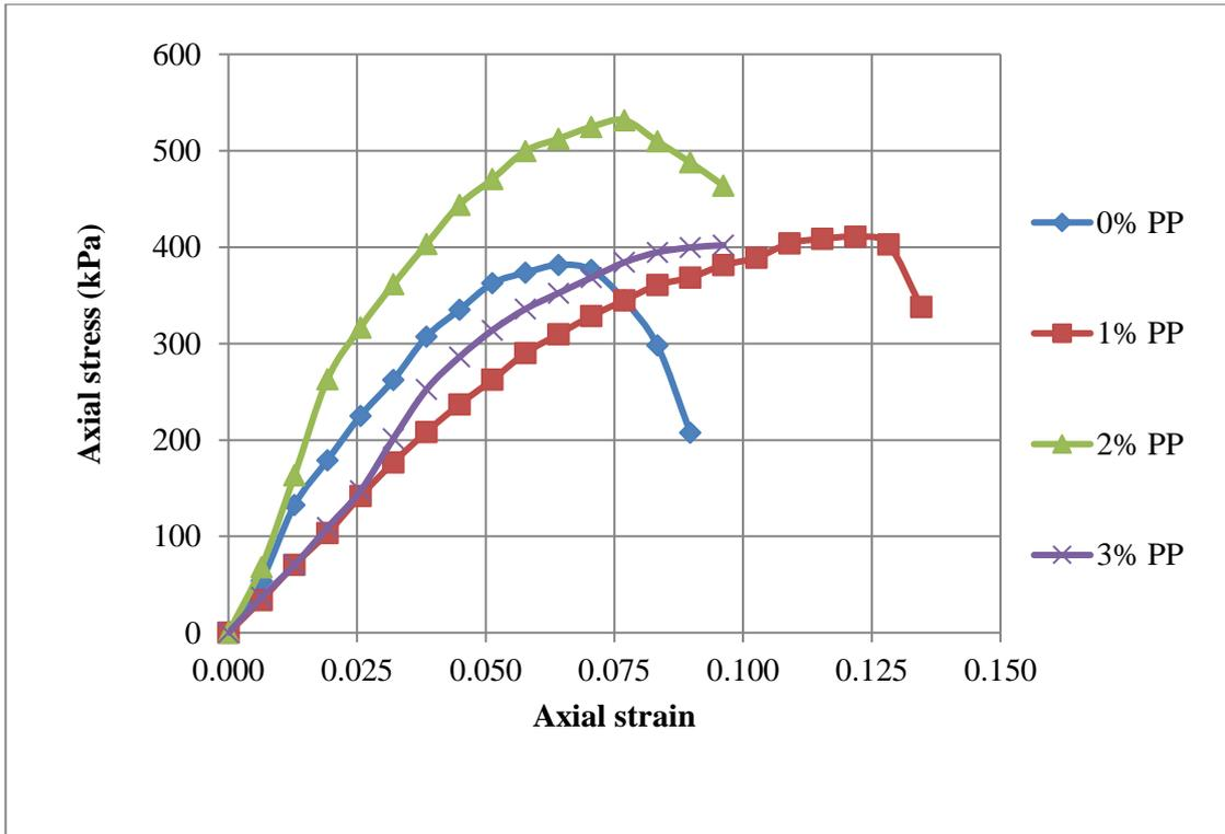
**Figure 4.8 Super-imposed stress-strain curve of sample 4 at different percentage of PP**
