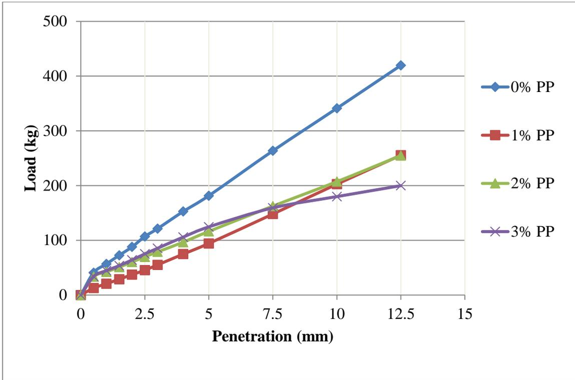
Figure 4.20: Superimposed curves of load vs penetration for Sample 5 with PP
