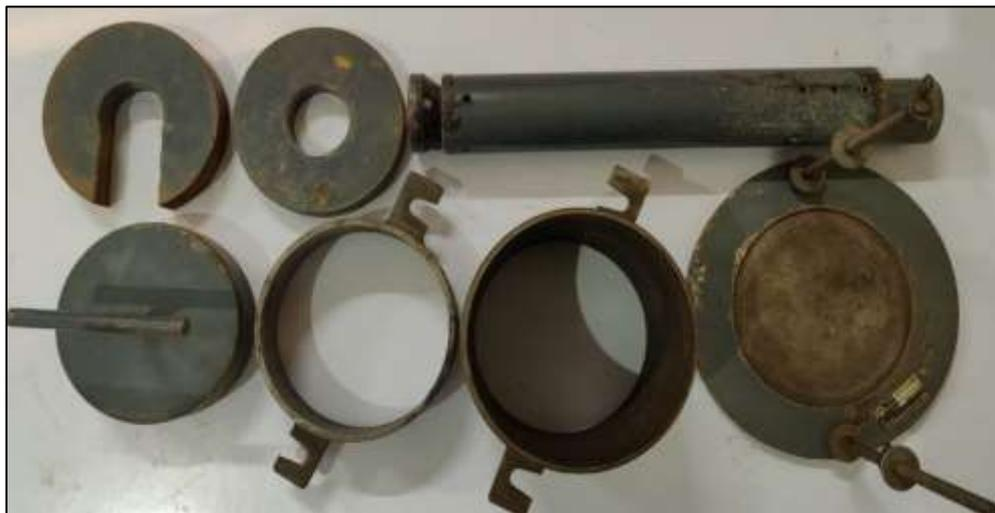
**Fig.3.8: Different component of compaction assembly -base plate, mould, collar. Spacer disc, rammer, surcharge plate (from right hand side)**
