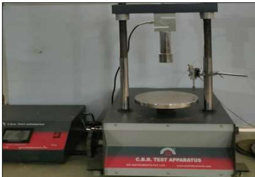
**Fig. 3.9: CBR testing machine (digital)**
