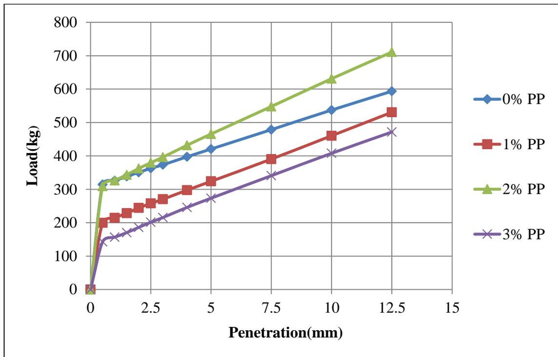
**Figure 4.19: Superimposed curves of load vs penetration for Sample 1 with PP**
