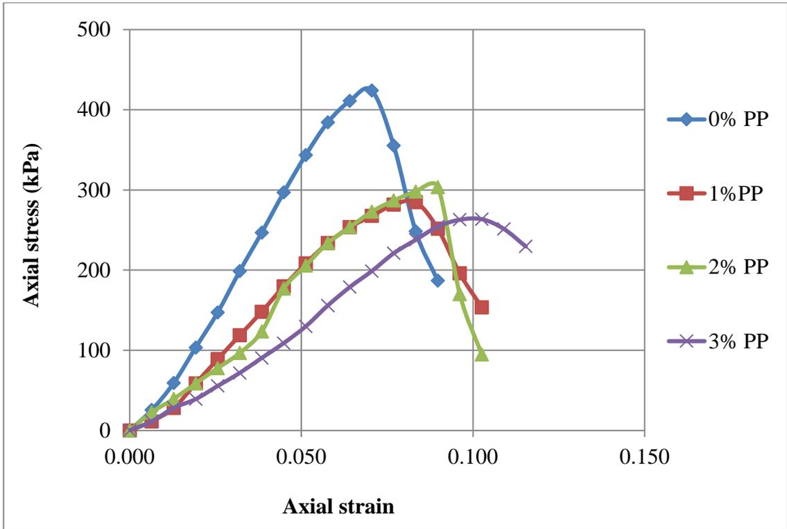
Figure 4.4 super-imposed stress-strain curve of sample 1 at different percentage of PP
