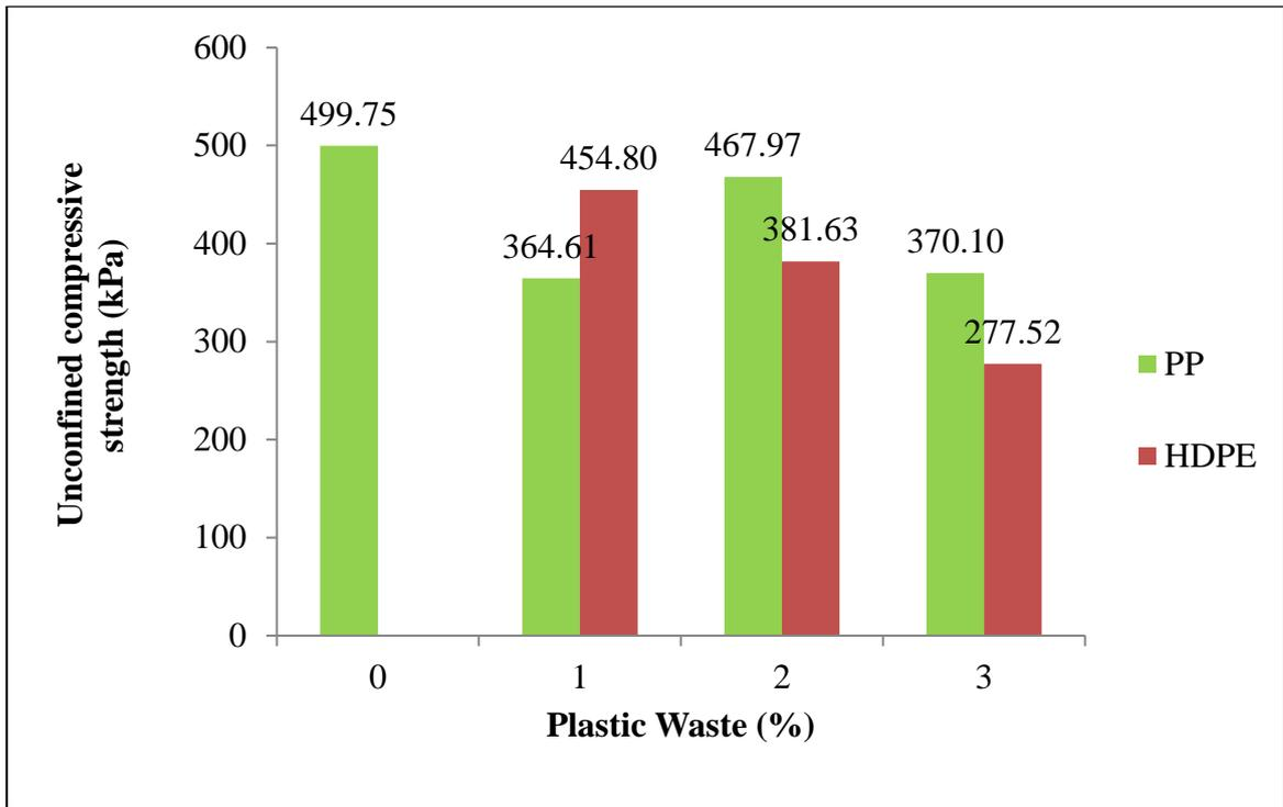
Figure 4.16: Plastic waste vs UCS of Sample 2 for both PP and HDPE
