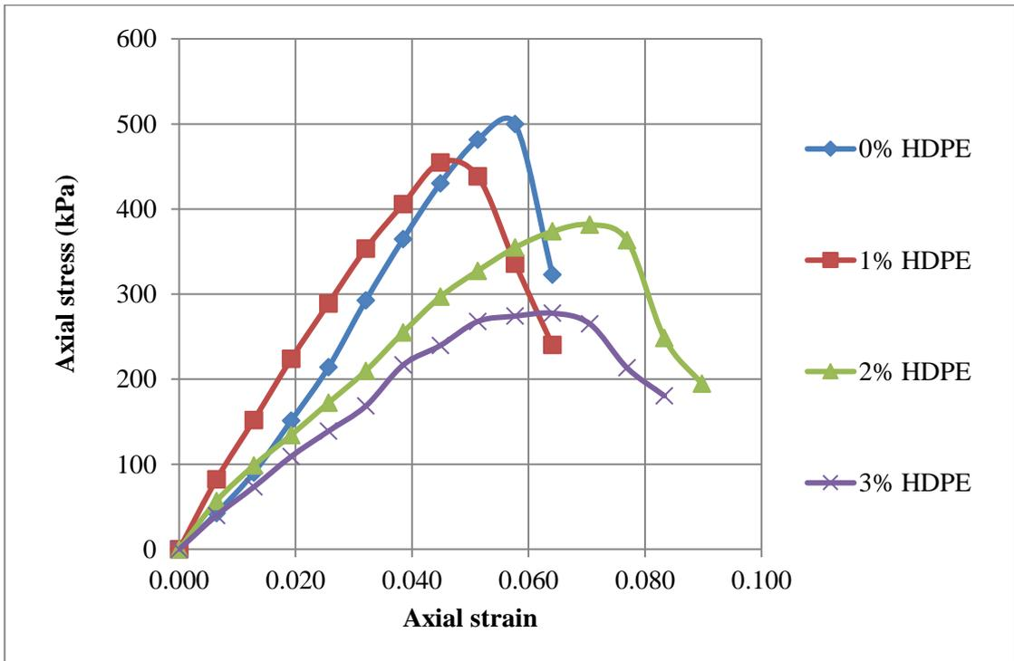
**Figure 4.11 Super-imposed stress-strain curve of sample 2 at different percentage of HDPE**
