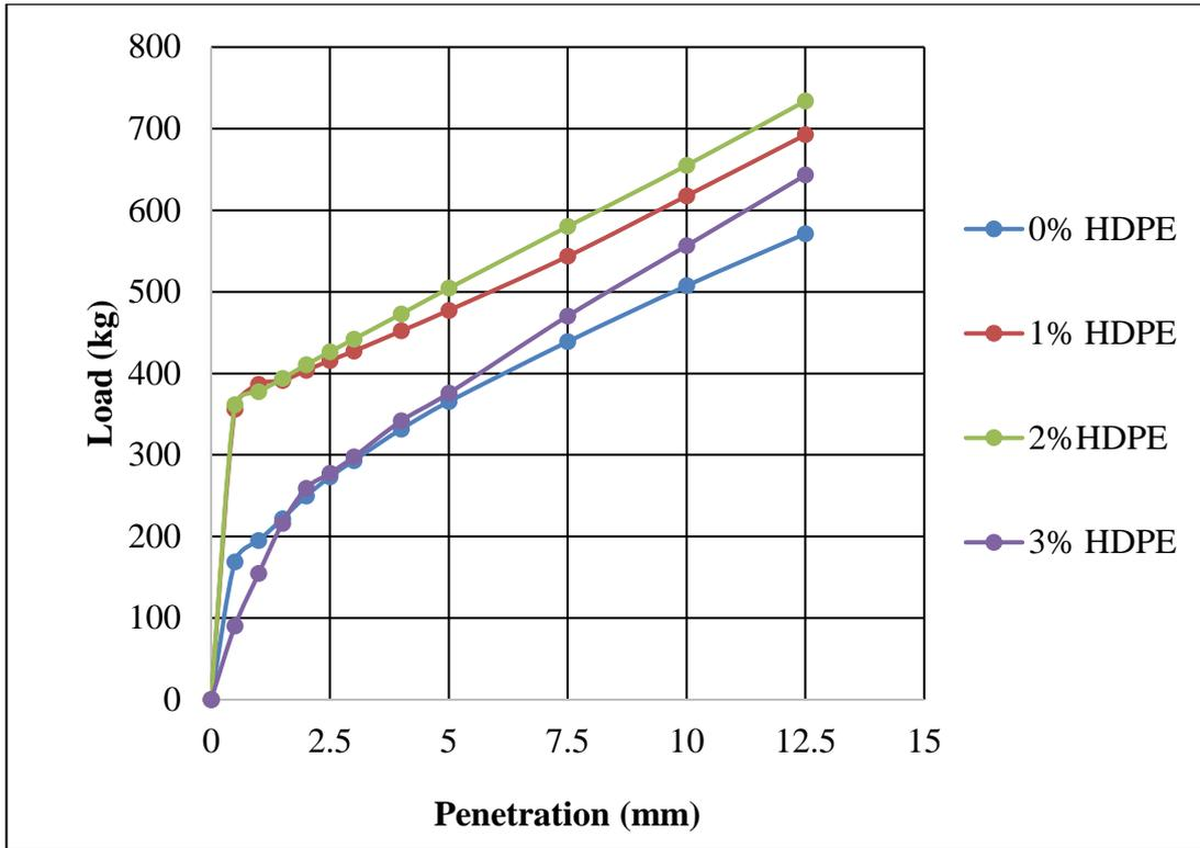
Figure 4.27: Superimposed curves of load vs penetration for Sample 3 with HDPE
