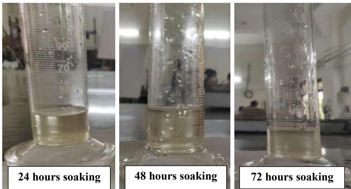
**Figure 4.31: Colour of the leachate extracted from SLM**
