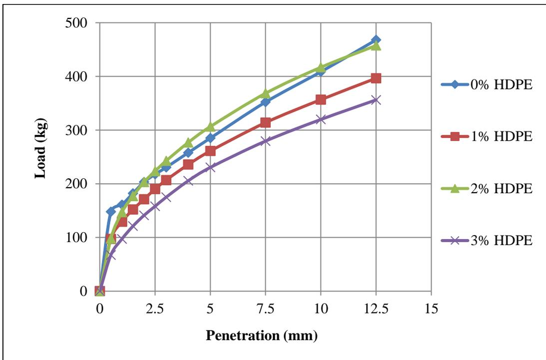
Figure 4.28: Superimposed curves of load vs penetration for Sample 4 with HDPE
