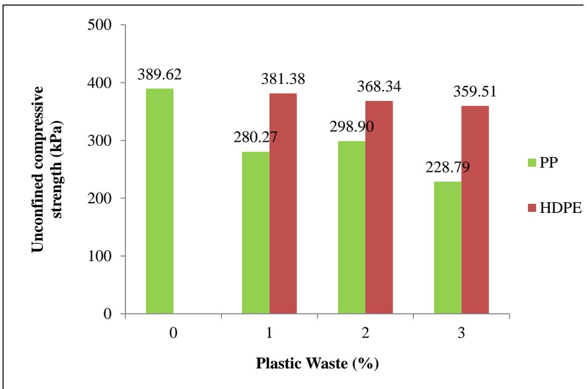
Figure 4.17: Plastic waste vs UCS of Sample 3 for both PP and HDPE
