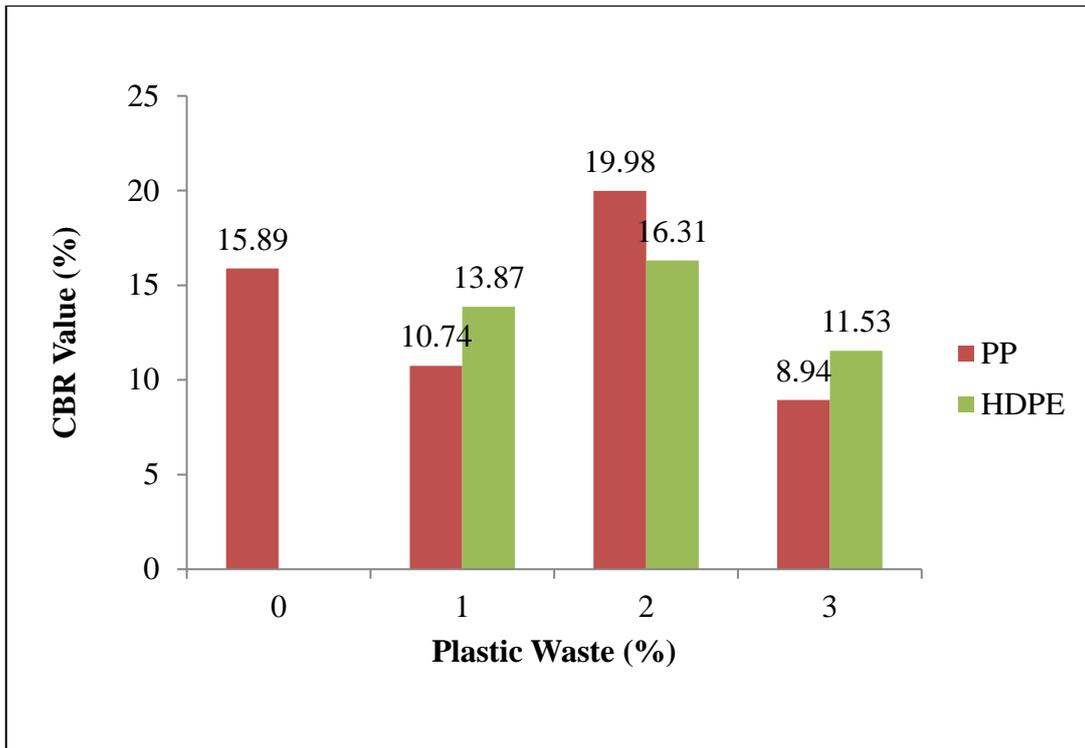
**Figure 4.33: Plastic waste vs CBR of Sample 4 for both PP and HDPE**
