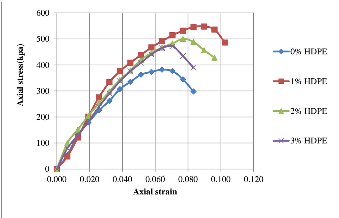
**Figure 4.13 Super-imposed stress-strain curve of sample 4 at different percentage of HDPE**
