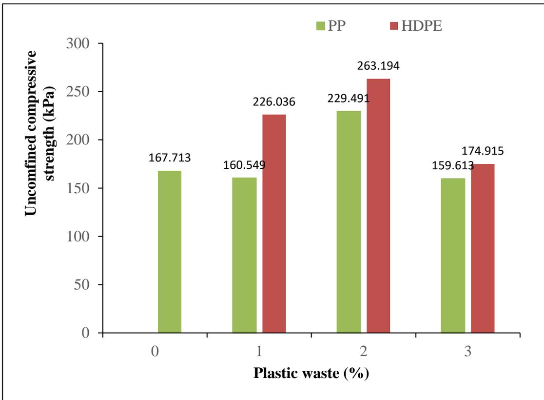
**Figure 4.15 Plastic waste (PP & HDPE) vs UCS of sample 5**
