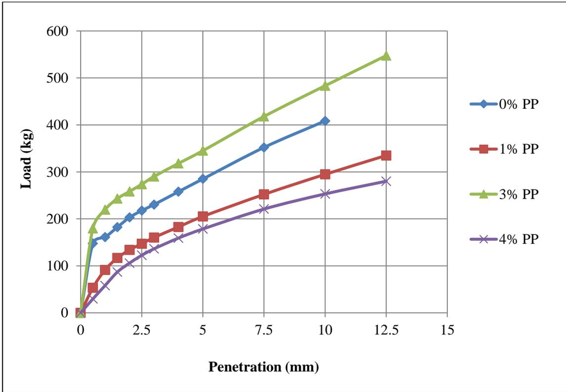
Figure 4.23: Superimposed curves of load vs penetration for Sample 4 with PP
