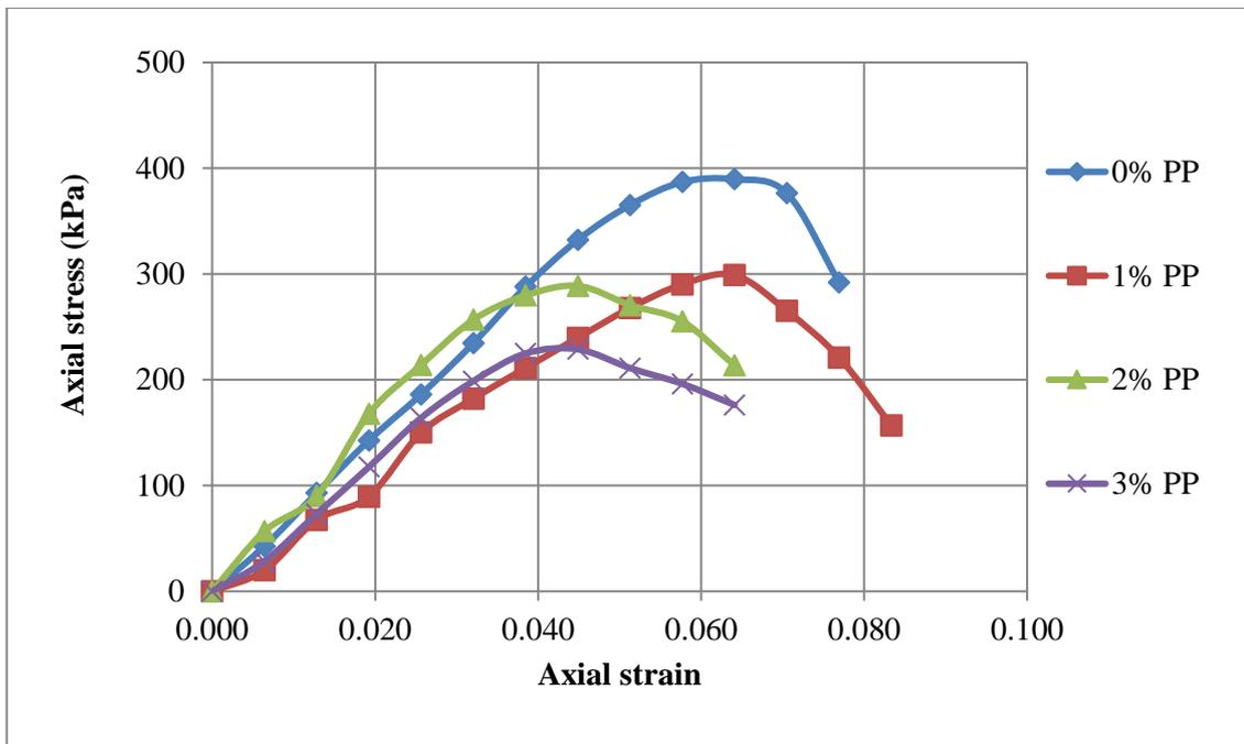
Figure 4.7 Super-imposed stress-strain curve of sample 3 at different percentage of PP
