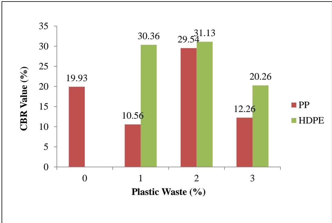
**Figure 4.32: Plastic waste vs CBR of Sample 3 for both PP and HDPE**
