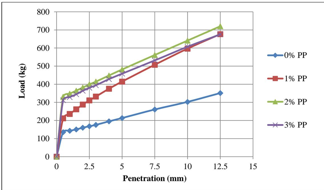
Figure 4.21: Superimposed curves of load vs penetration for Sample 2 with PP
