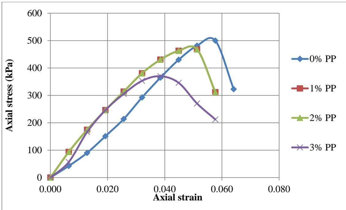
Figure 4.6 Super-imposed stress-strain curve of sample 2 at different percentage of PP
