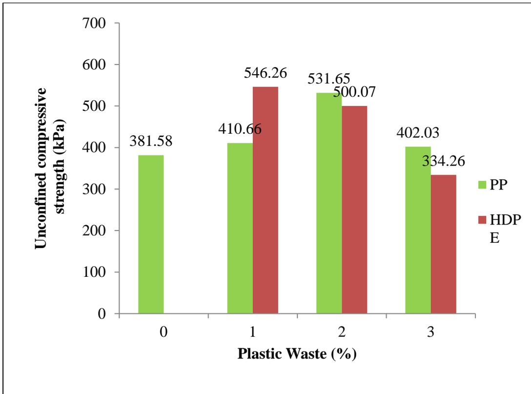
**Figure 4.18: Plastic waste vs UCS of Sample 4 for both PP and HDPE**
