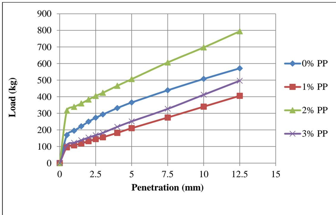
Figure 4.22: superimposed curves of load vs penetration for Sample 3 with PP
