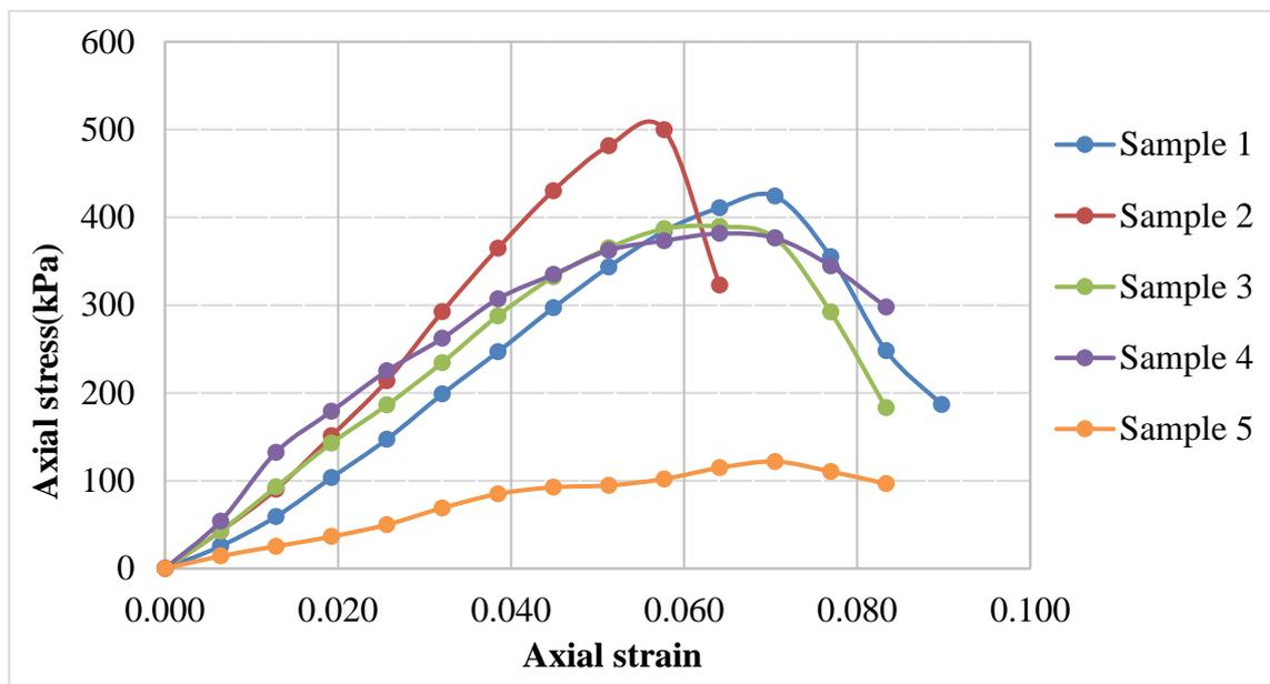
**Figure 4.2 Stress- strain relationship between SLM and native soil**
