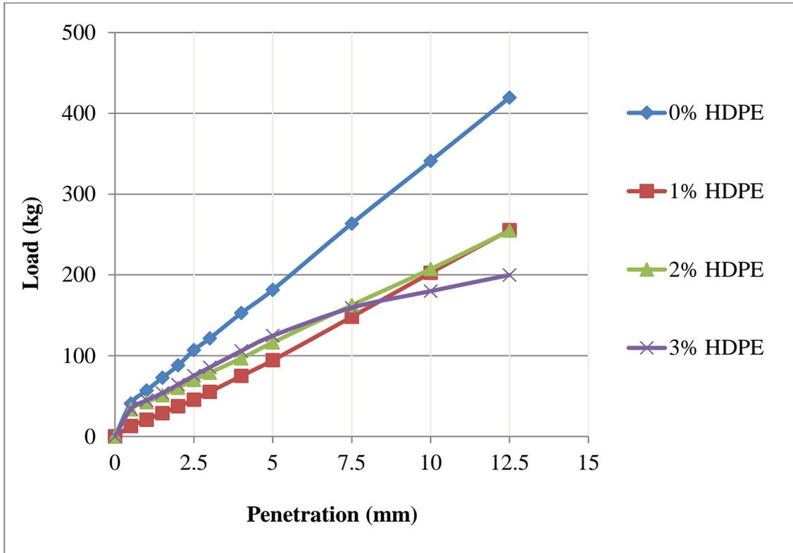
**Figure 4.25: Superimposed curves of load vs penetration for Sample 5 with HDPE**
