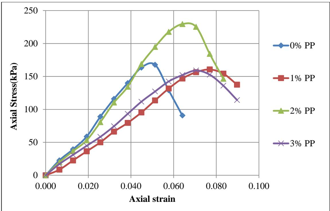
Figure 4.5 super-imposed stress-strain curve of sample 5 at different percentage of PP
