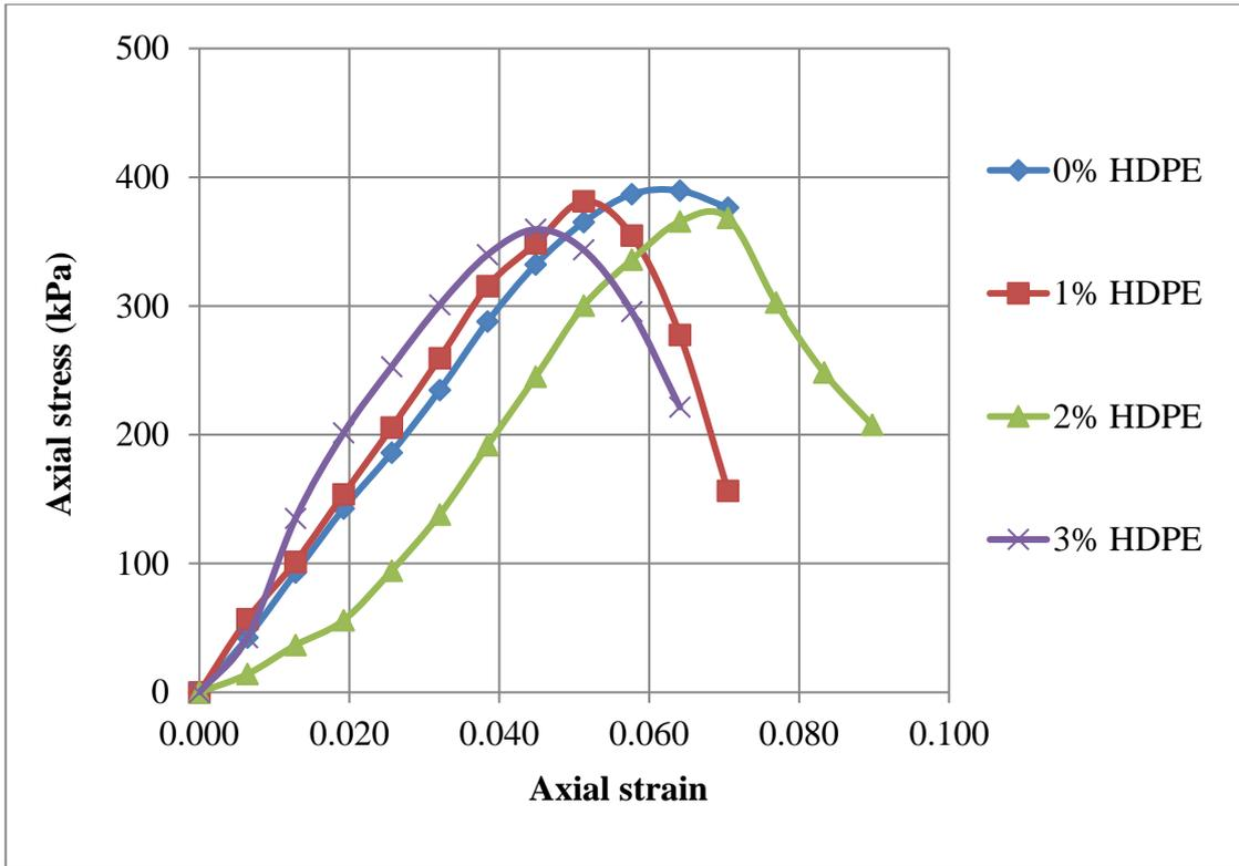
**Figure 4.12 Super-imposed stress-strain curve of sample 3 at different percentage of HDPE**
