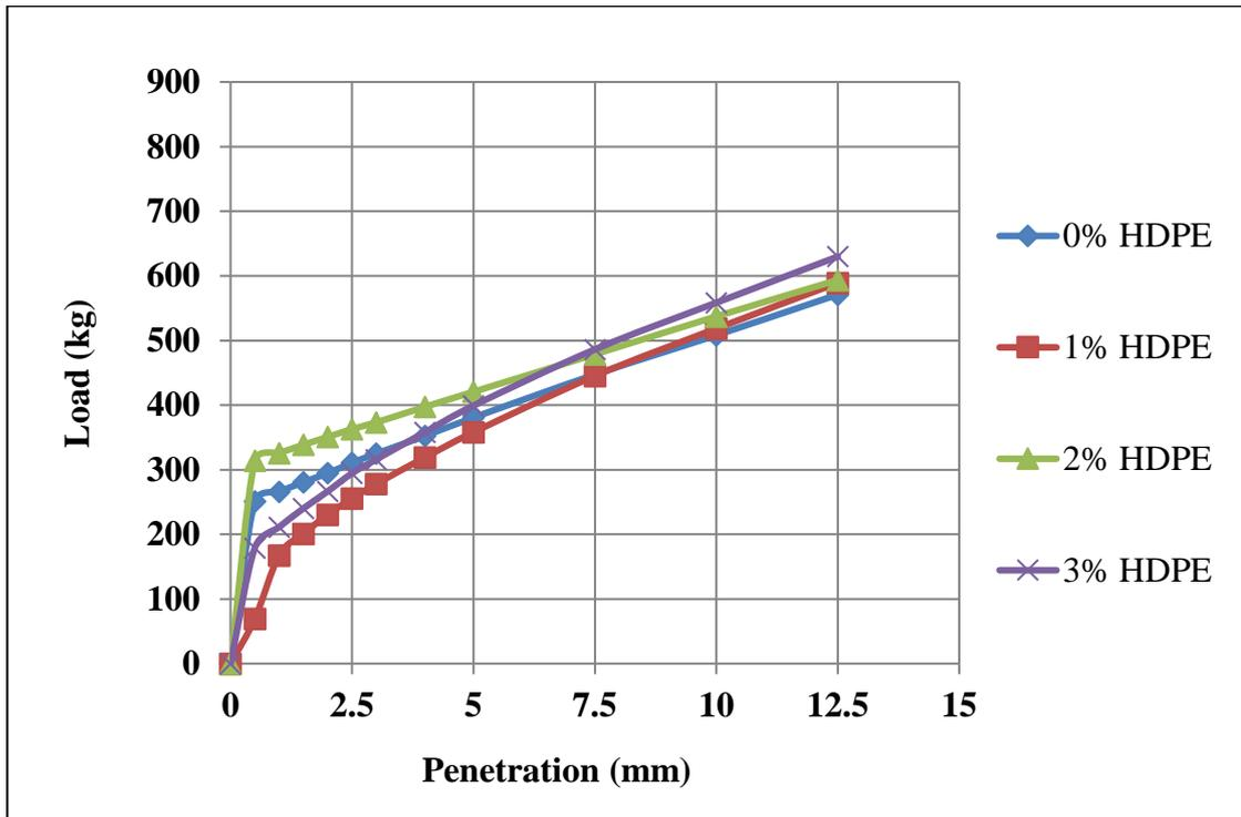
Figure 4.24: Superimposed curves of load vs penetration for Sample 1 with HDPE
