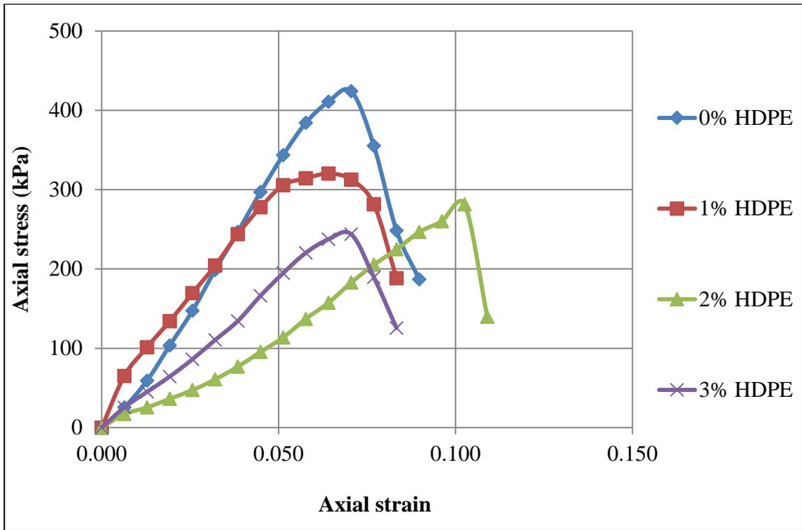
Figure 4.9 super-imposed stress-strain curve of sample 1 at different percentage of HDPE
