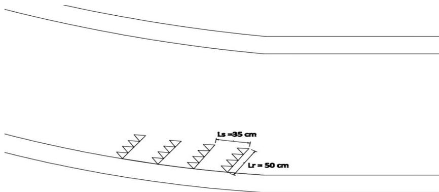
Fig 4.44: Layout of porcupine field for trial 12
