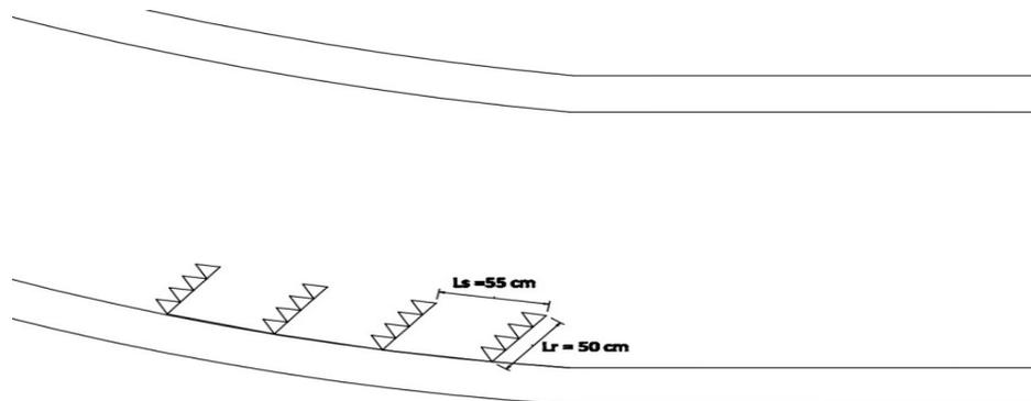
Fig 4.38: Layout of porcupine field for trial 10
