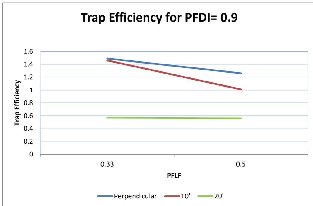
Fig. 5.9 PFLF versus Trap efficiency for PFDI = 0.9, when porcupine is laid at  $10^0$  and  $20^0$  towards upstream and perpendicular to the bank
