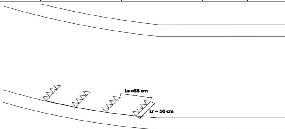
**Fig 4.50:** Layout of porcupine field for trial 14
