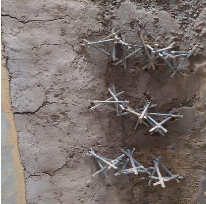
Figure 4.18: Porcupine field for 3<sup>rd</sup> trial
