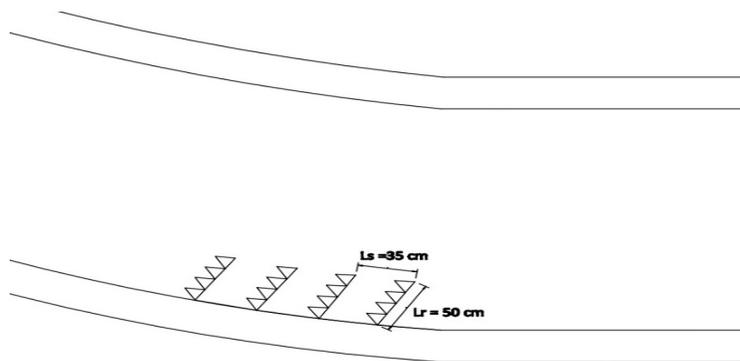
Fig 4.68: Layout of porcupine field for trial 20
