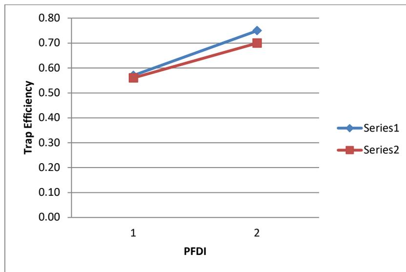
Fig 5.3: PFDI versus Trap efficiency for PFLF = 0.5 and PFLF = 0.33, when 5 kg of sediment was injected
