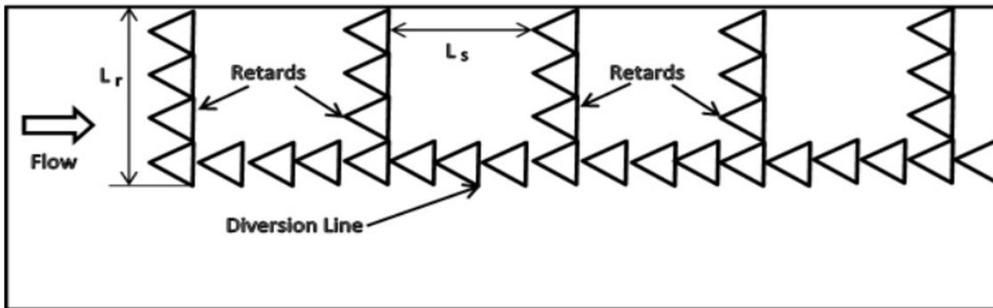
Figure 4.9: Typical layout of porcupine field
