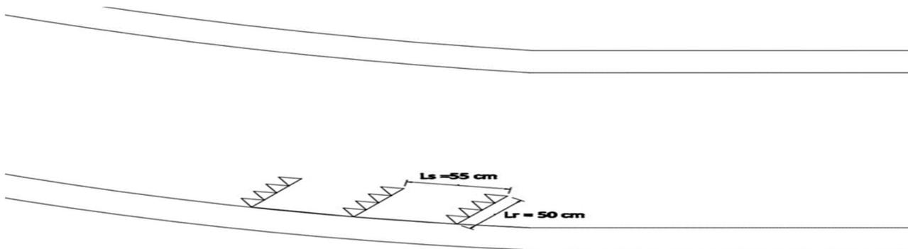
Figure 4.29: Layout of porcupine field for trial 7
