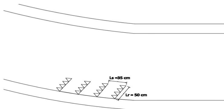
Fig 4.62: Layout of porcupine field for trial 18
