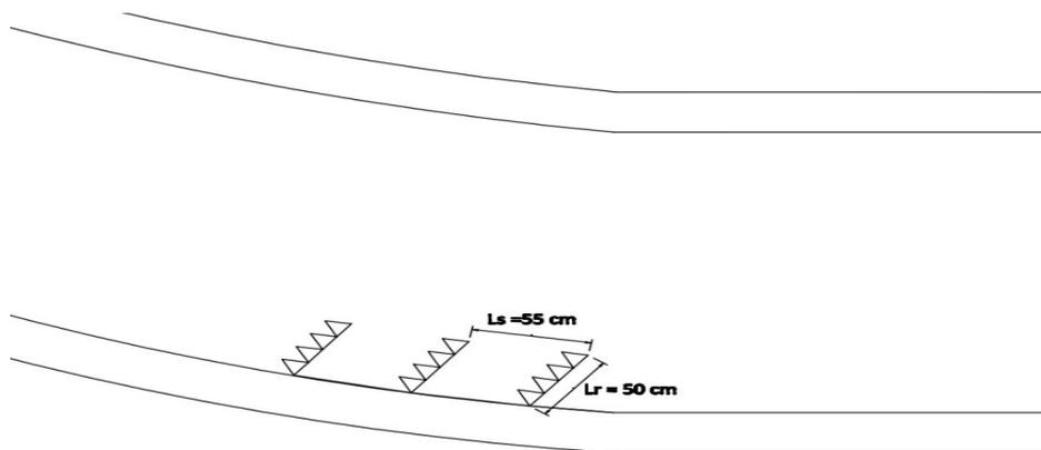
Fig 4.47: Layout of porcupine field for trial 13
