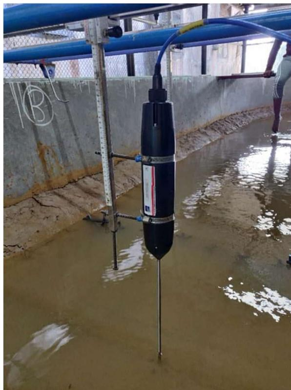
Figure 3.6: Acoustic Doppler Velocimeter (ADV)
