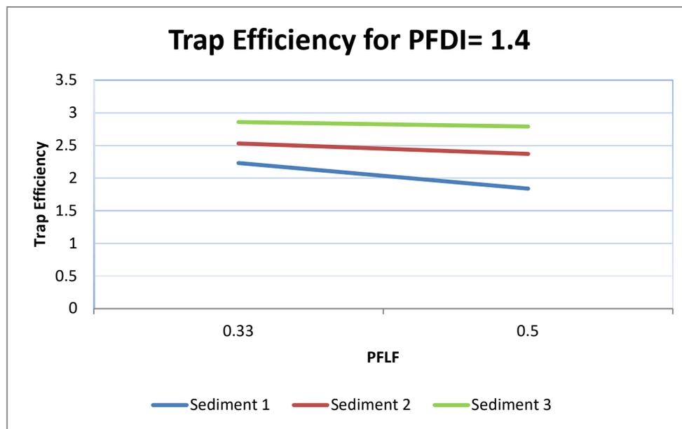
Fig. 5.10 PFLF versus Trap efficiency for PFDI = 1.4 for different Sediment Sample when porcupine is laid perpendicular to the bank
