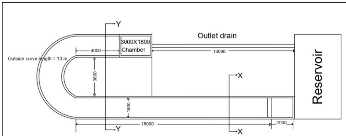
Fig.3.3: Experimental channel
