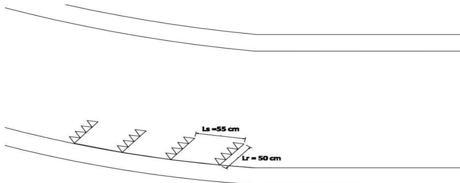
Figure 4.26: Layout of porcupine field for trial 6
