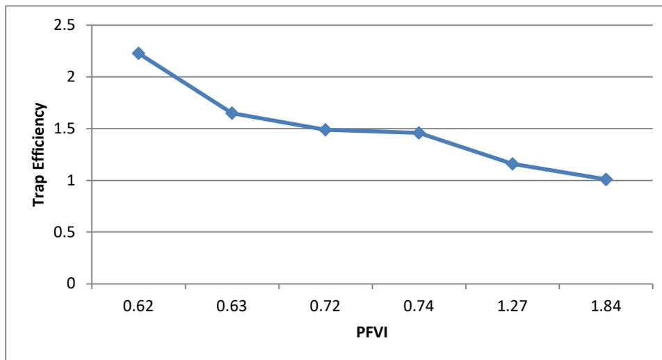
Fig 5.7: PVFI versus Trap efficiency for  $q_s = 600$  ppm
