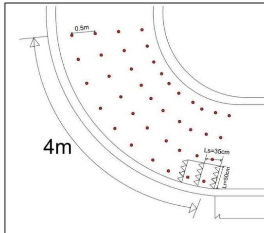
Fig. 3.2: Test points in the experimental channel
