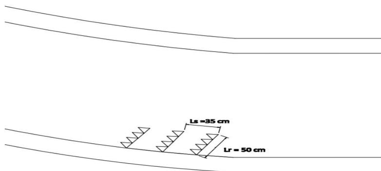
Figure 4.17: Layout of porcupine field for trial 3
