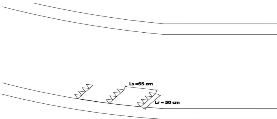
Fig 4.53: Layout of porcupine field for trial 15
