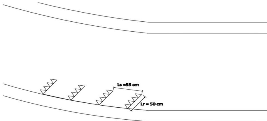
Fig 4.56: Layout of porcupine field for trial 16
