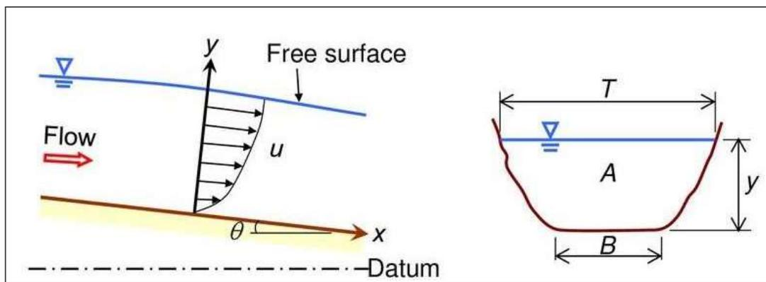
Figure 1.1: Open channel flow.
