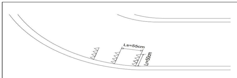
Figure 4.32: Layout of porcupine field for trial 8
