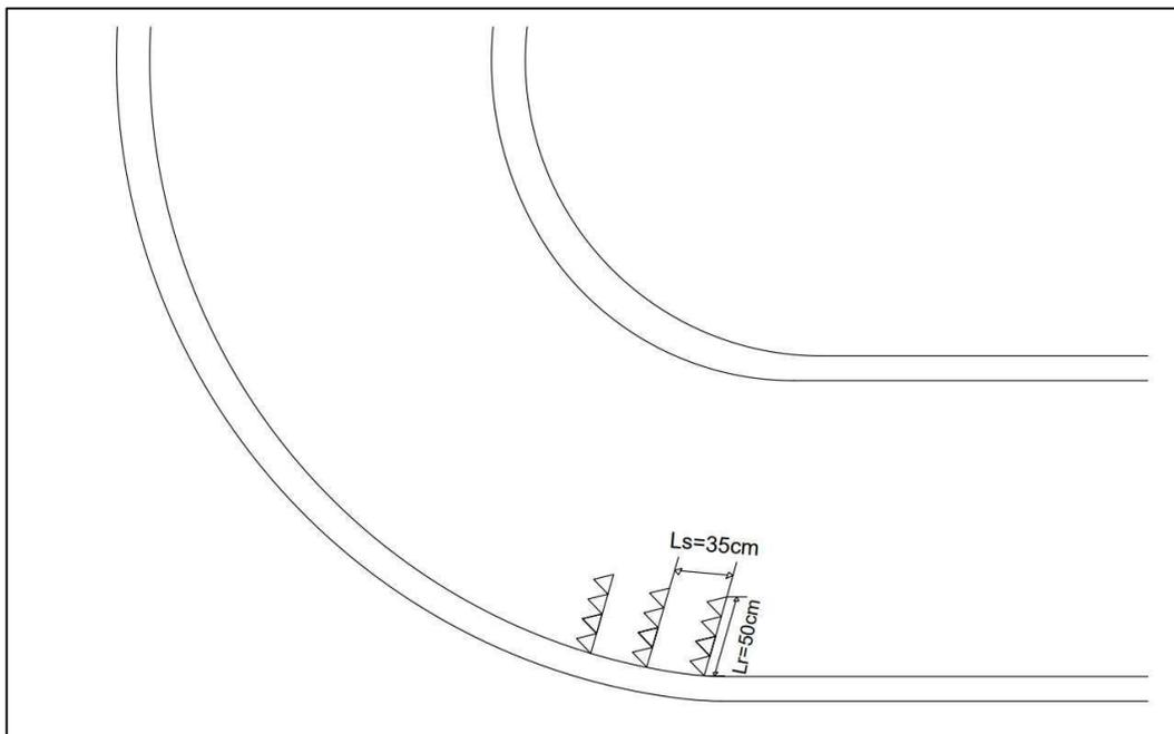
Fig.4.10:Porcupine layout in channel
