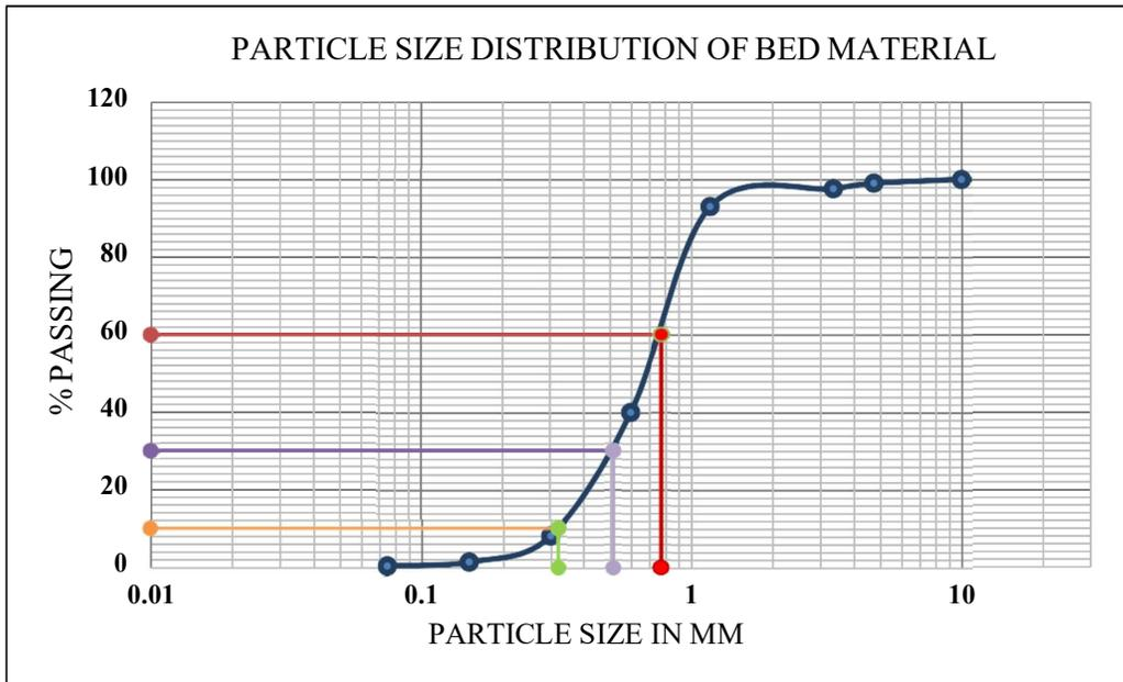
Figure 4.1: Particle size distribution of bed material
