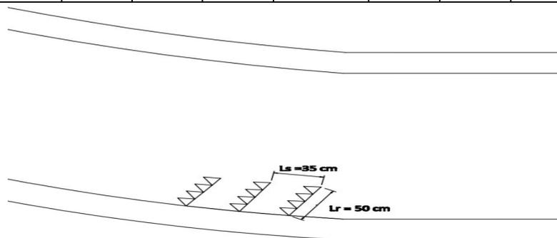
Figure 4.20: Layout of porcupine field for trial 4
