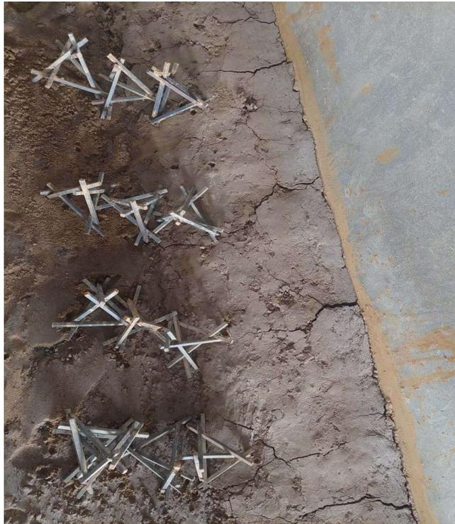
Figure 4.12: Porcupine field for 1<sup>st</sup> trial
