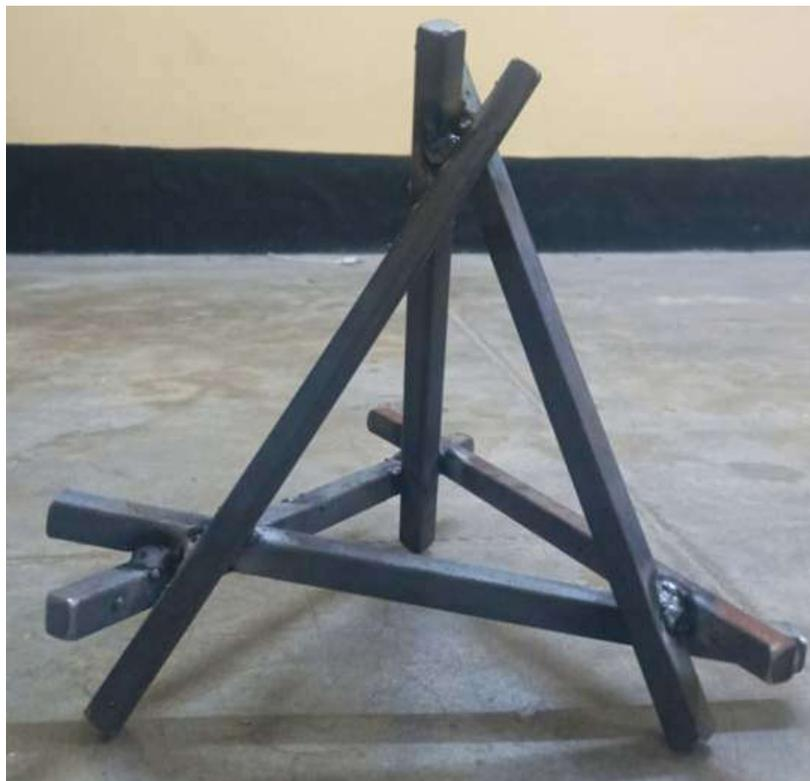
Fig. 3.1: Model of porcupine made of MS Rod
