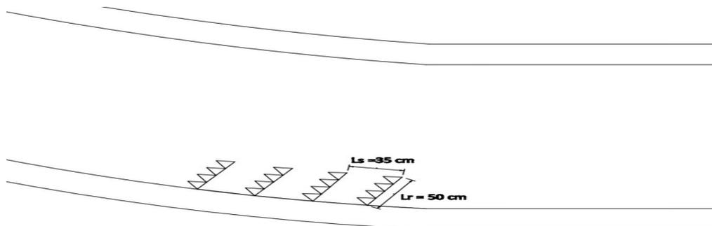
Fig.4.11: Layout of porcupine field for trial 1
