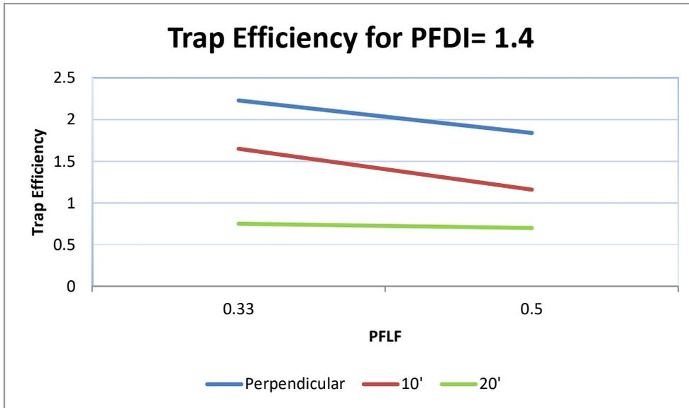
Fig. 5.8 PFLF versus Trap efficiency for **PFDI = 1.4**, when porcupine is laid at  $10^0$  and  $20^0$  towards upstream and perpendicular to the bank
