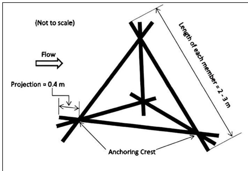
Figure 1.3: Three dimensional sketch of a typical RCC Porcupine unit
