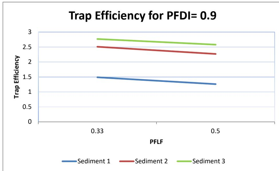
Fig. 5.11 PFLF versus Trap efficiency for PFDI = 0.9 for different Sediment Sample when porcupine is laid perpendicular to the bank
