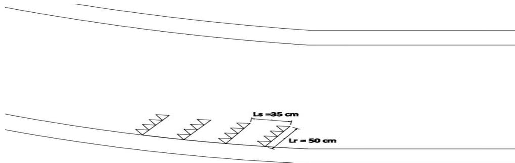
Figure 4.14: Layout of porcupine field for trial 2
