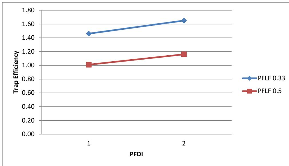
Fig 5.2: PFDI versus Trap efficiency for PFLF = 0.5 and PFLF = 0.33, when 8 kg of sediment
