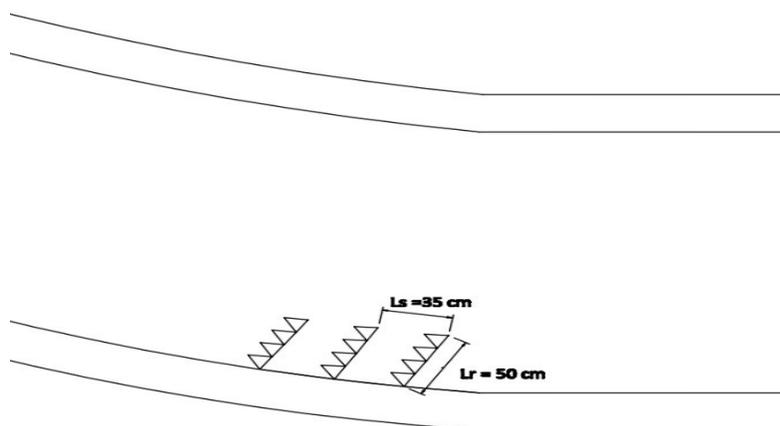
**Fig 4.65:** Layout of porcupine field for trial 19
