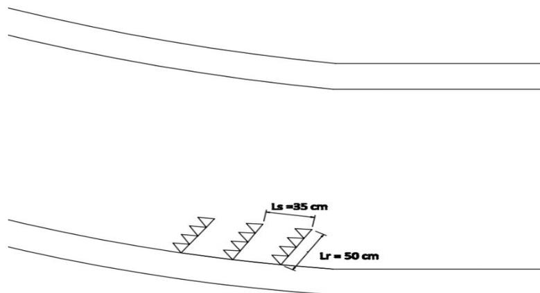
**Fig 4.59:** Layout of porcupine field for trial 17
