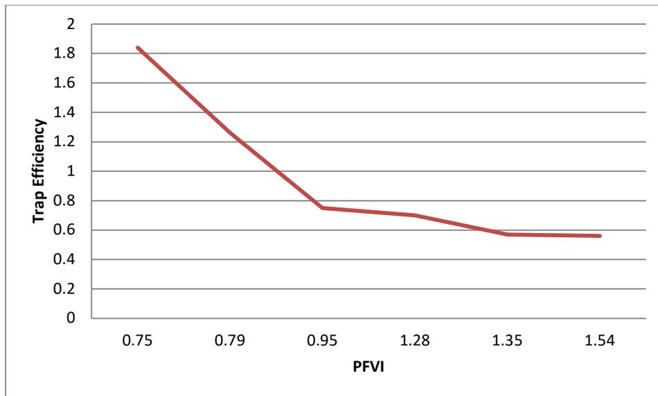
Fig 5.6: PVFI versus Trap efficiency for  $q_s = 300$  ppm
