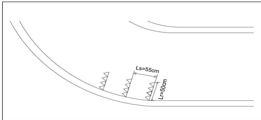
Fig 4.35: Layout of porcupine field for trial 9
