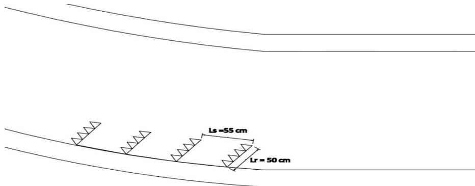
Figure 4.23: Layout of porcupine field for trial 5
