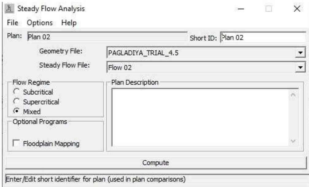
Fig 4.13: Computation of Steady flow analysis
