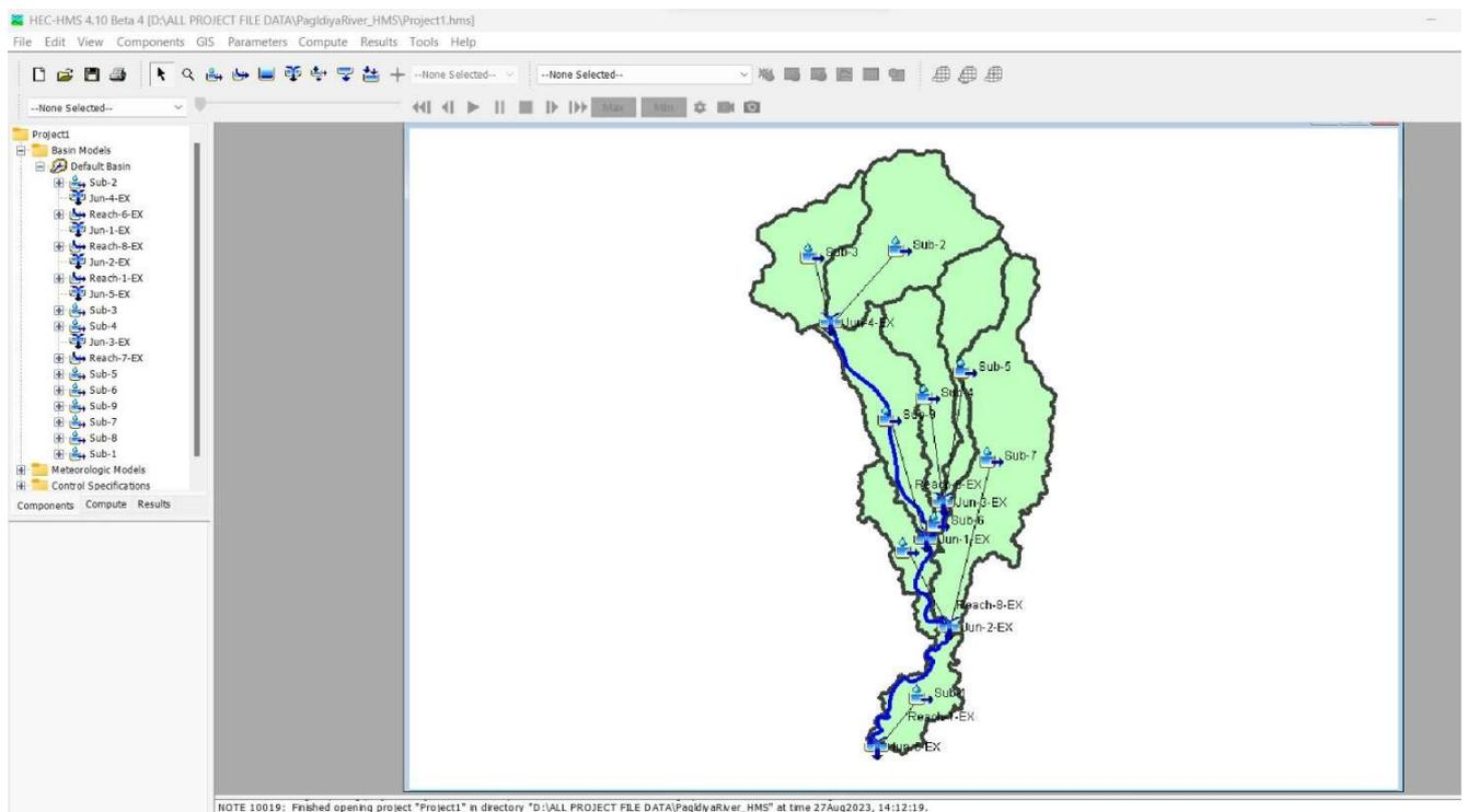
Fig 4.7: HEC-HMS interface showing sub-basins and junctions
