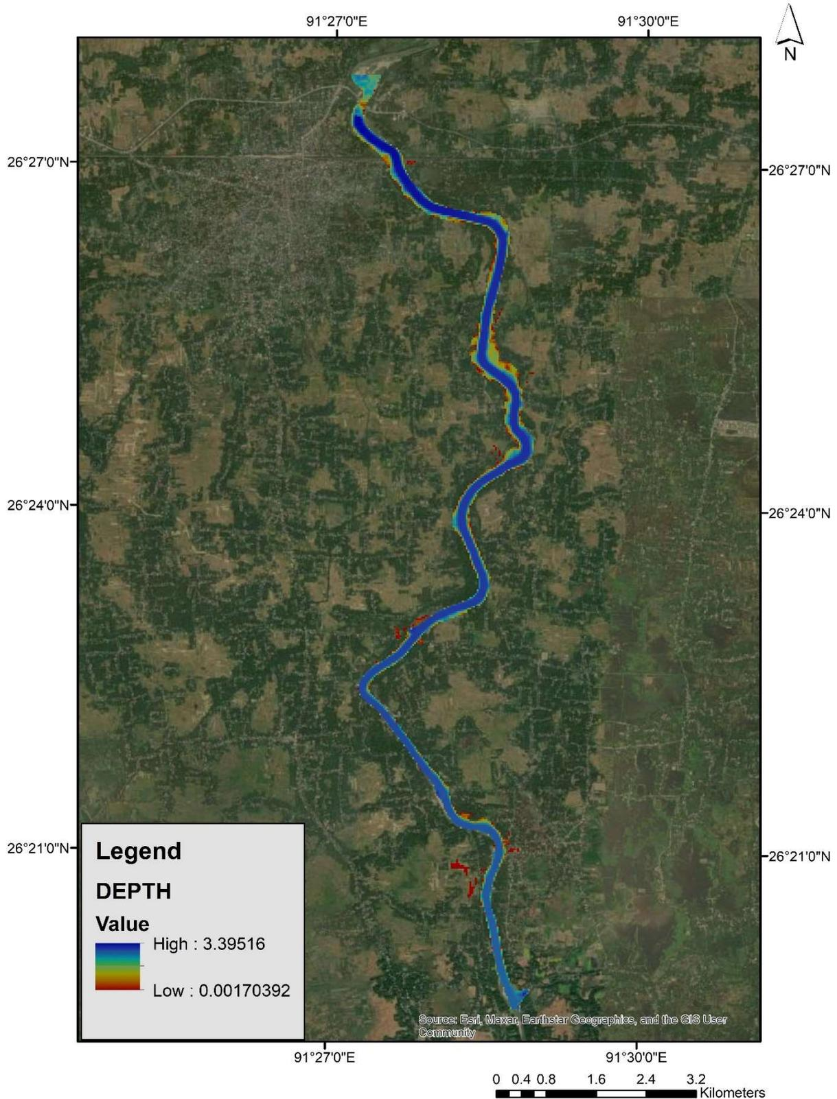
Fig 5.4: Depth Profile with Embankment
