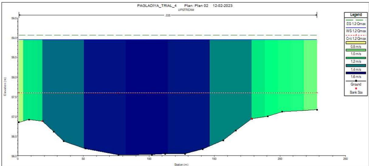
Fig 4.18: Elevation depth graph at upstream section for 1.2 times  $Q_{max}$
