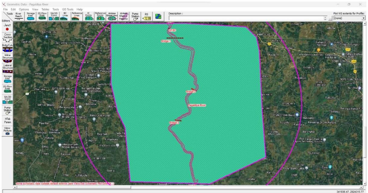
Fig 4.27: Setting up of 2D Flow Area
