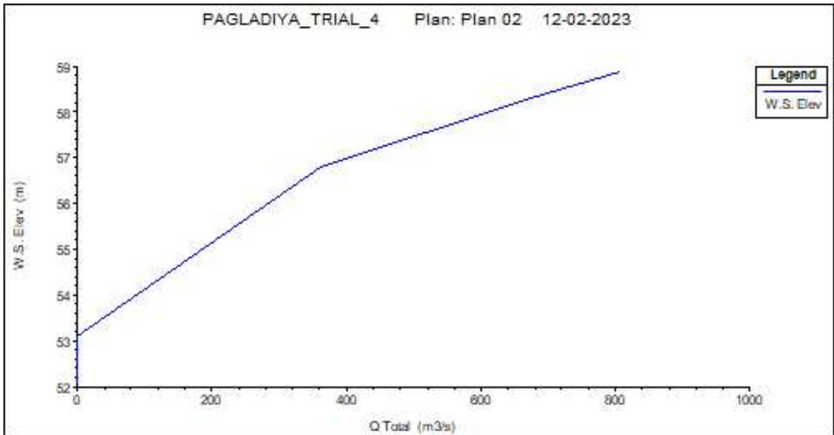
Fig 4.24: Rating curve of Upstream
