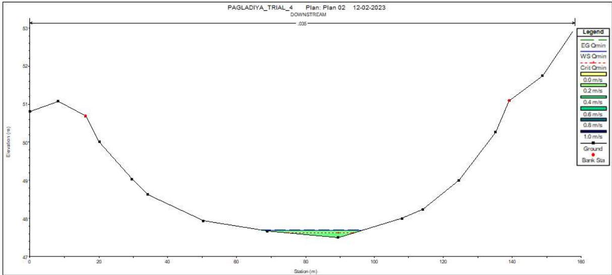
Fig 4.19: Elevation depth graph at downstream section for  $Q_{min}$
