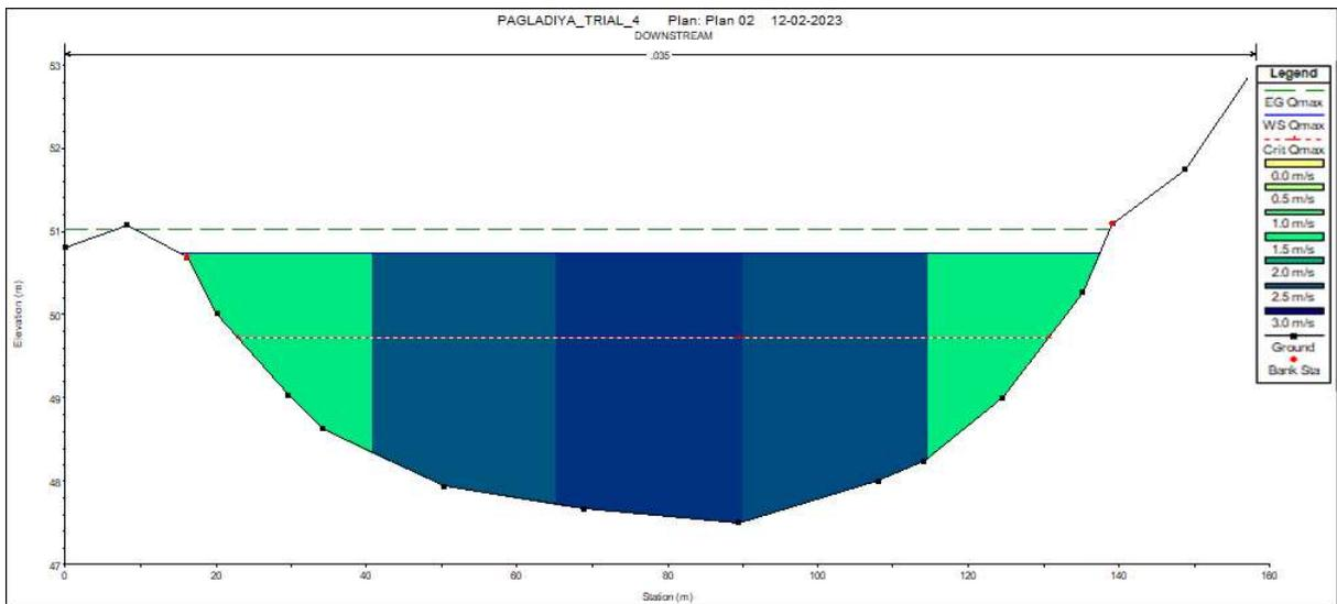
Fig 4.20: Elevation depth graph at downstream section for  $Q_{max}$
