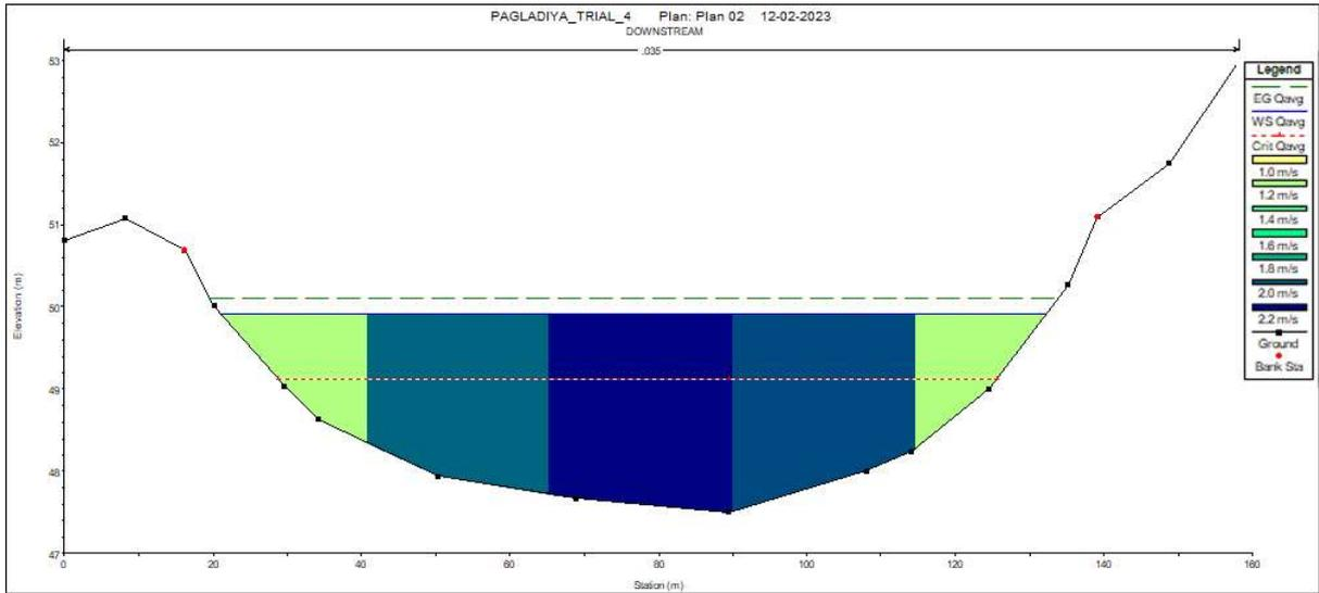
Fig 4.21: Elevation depth graph at downstream section for  $Q_{avg}$
