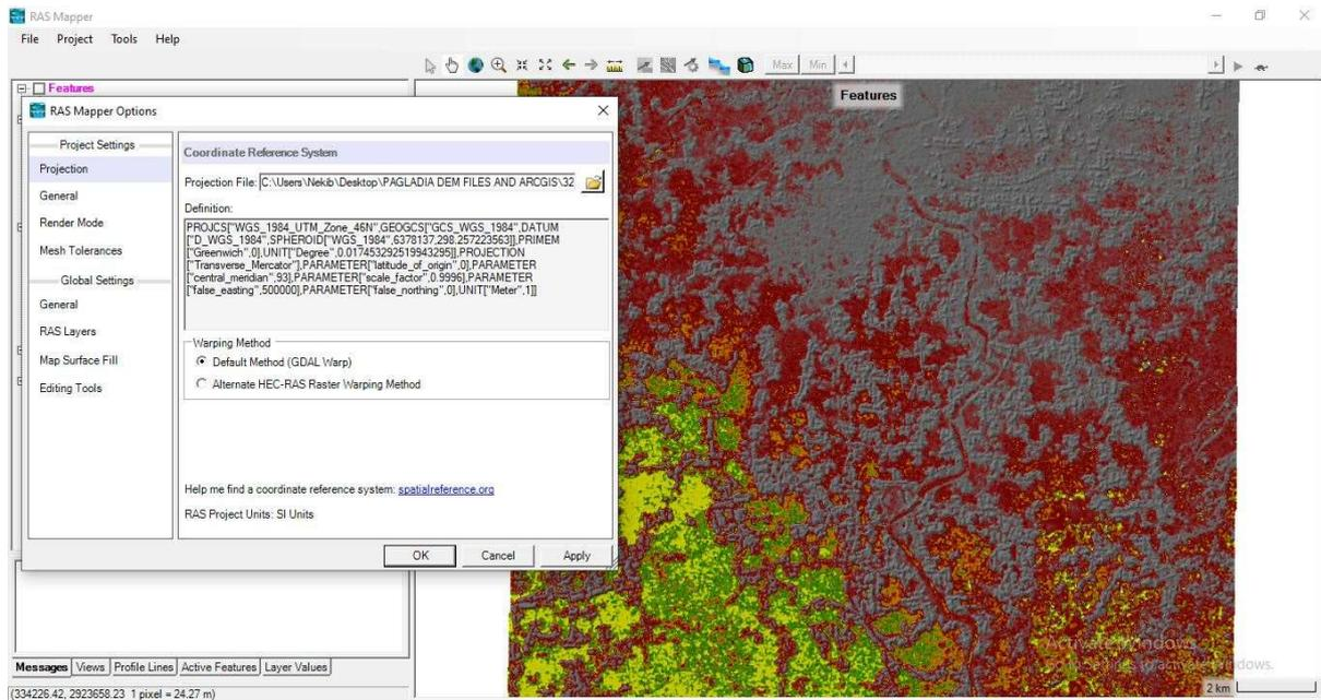
Fig 4.8: Applying projection to the terrain in RAS Mapper
