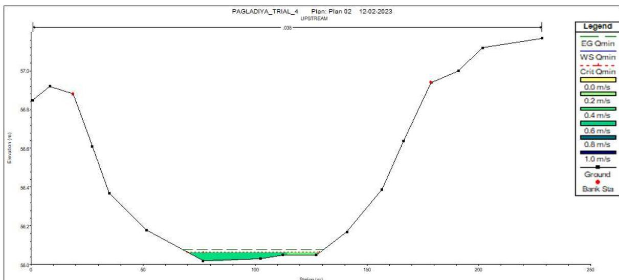
Fig 4.14: Elevation depth graph at upstream section for  $Q_{min}$
