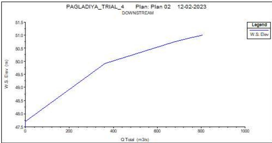
Fig 4.25: Rating curve of Downstream
