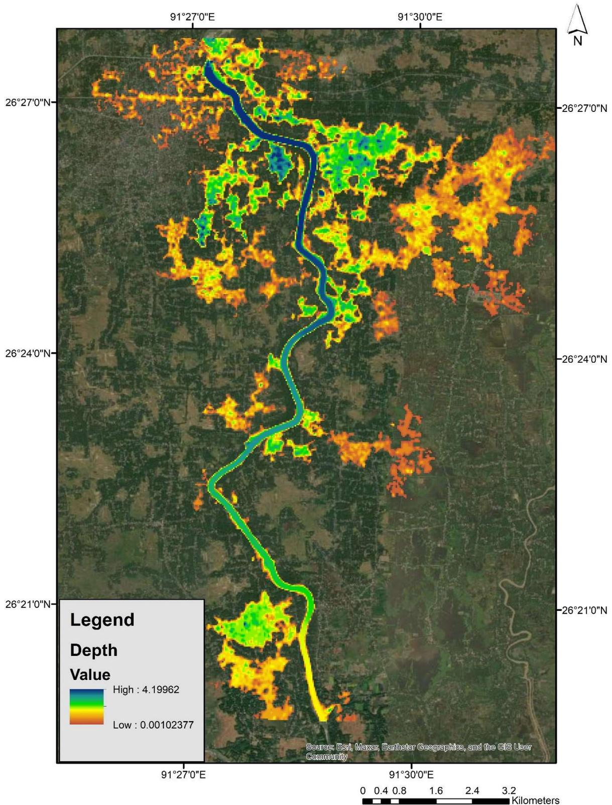
Fig 5.2: Flood inundation depth without Embankment
