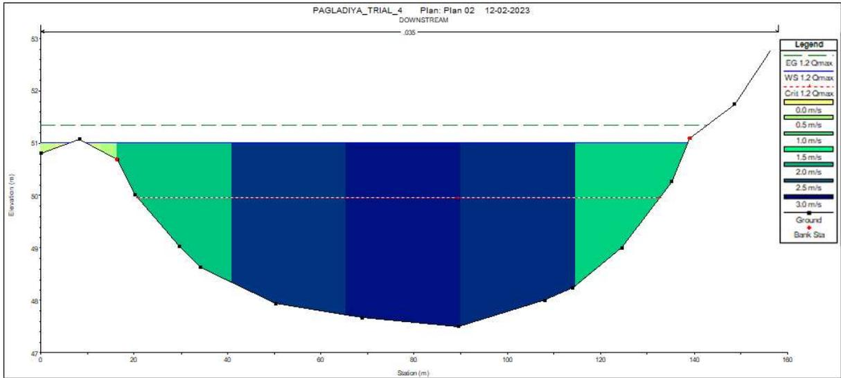
Fig 4.23: Elevation depth graph at downstream section for 1.2 times  $Q_{max}$
