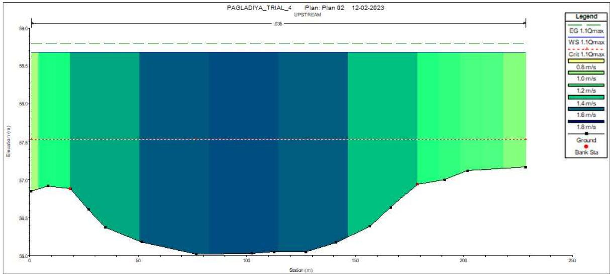
Fig 4.17: Elevation depth graph at upstream section for 1.1 times  $Q_{max}$
