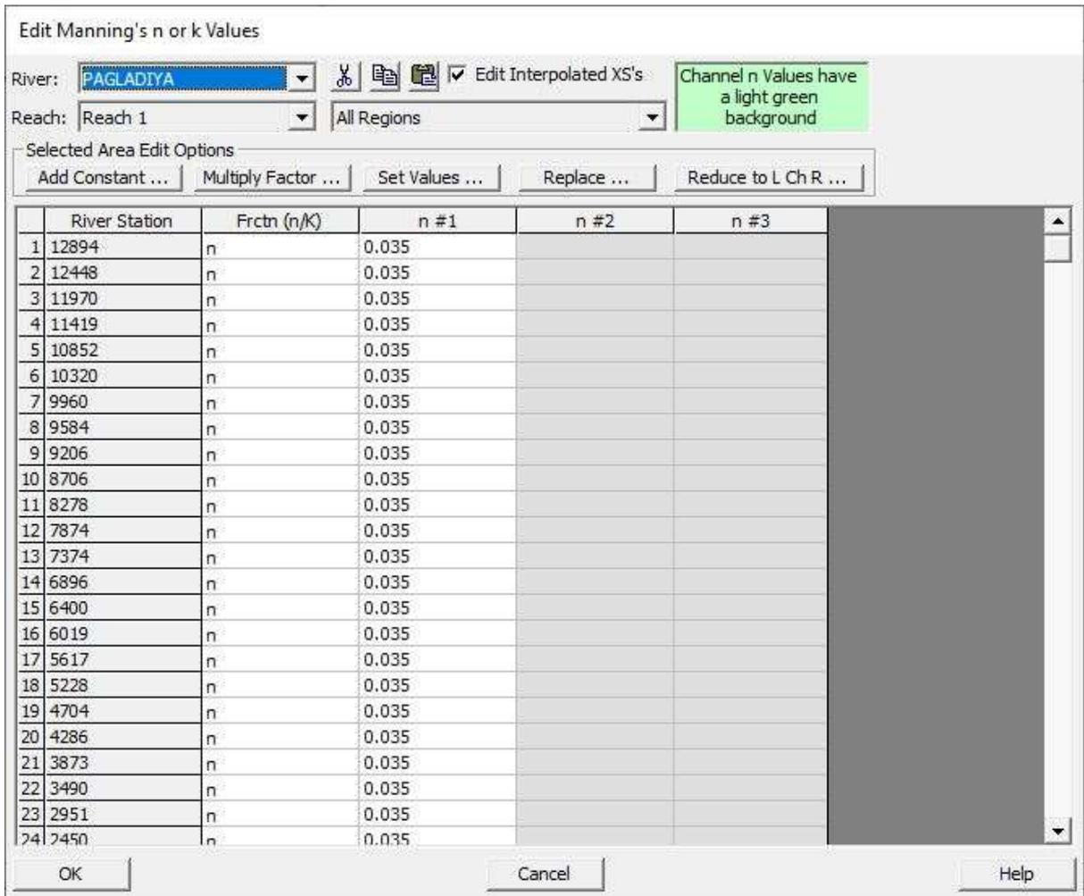
Fig 4.11: Applying Manning's n value for the flow
