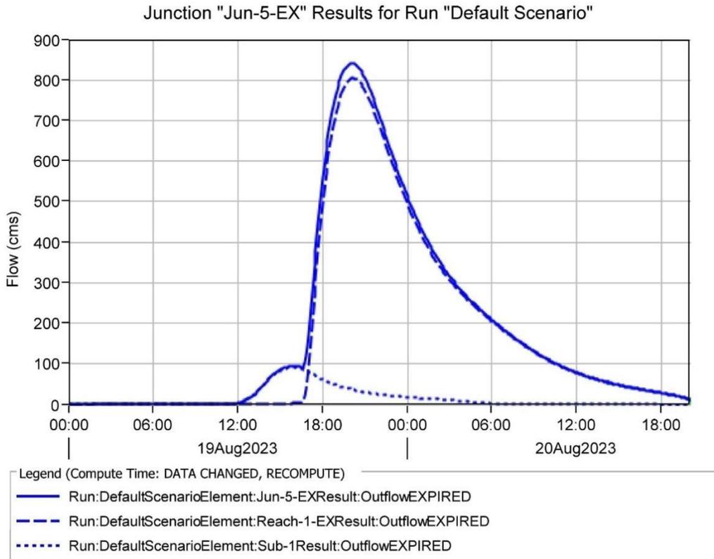
Fig 5.1: Hydrograph of downstream obtained from HEC-HMS
