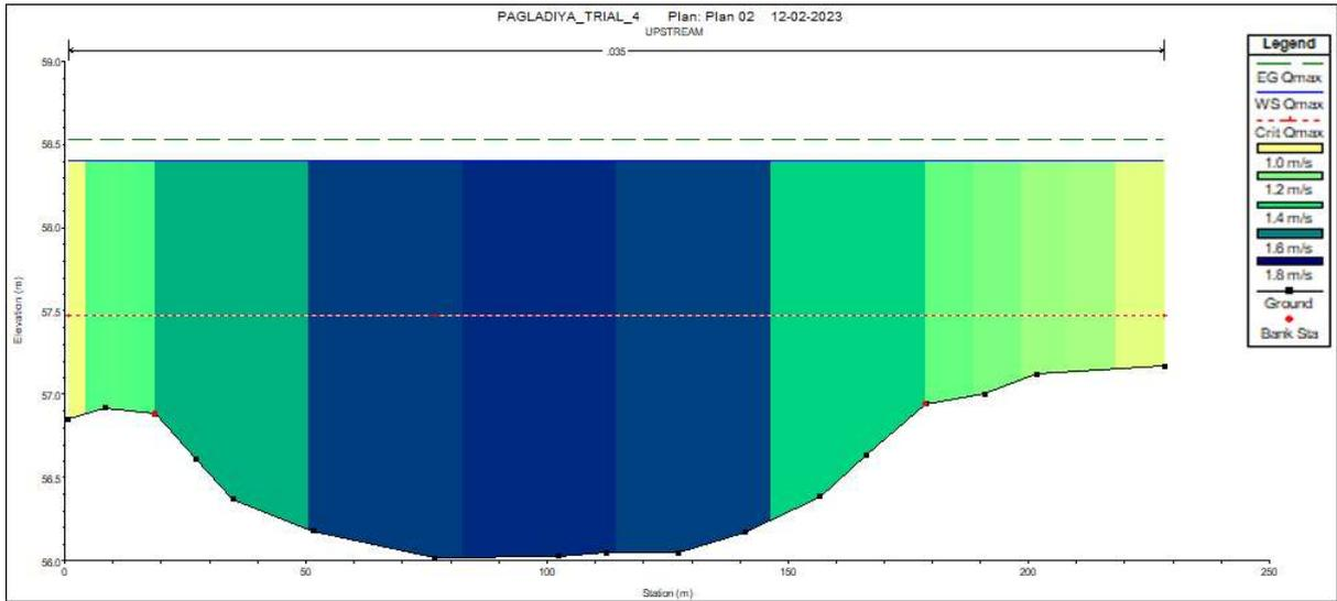
Fig 4.15: Elevation depth graph at upstream section for  $Q_{max}$
