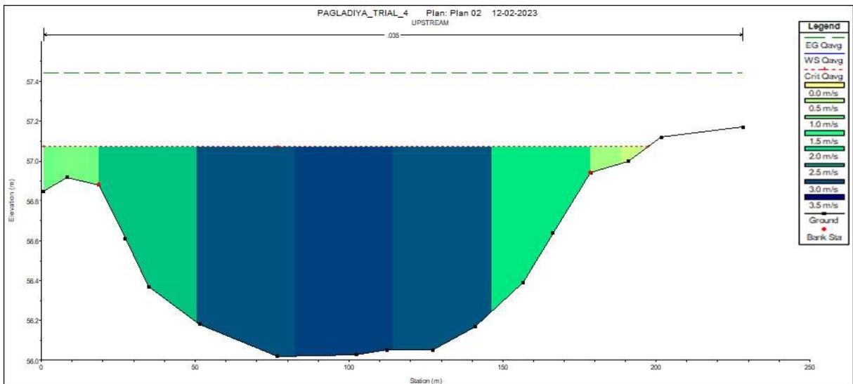
Fig 4.16: Elevation depth graph at upstream section for  $Q_{avg}$
