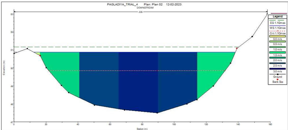
Fig 4.22: Elevation depth graph at downstream section for 1.1 times  $Q_{max}$
