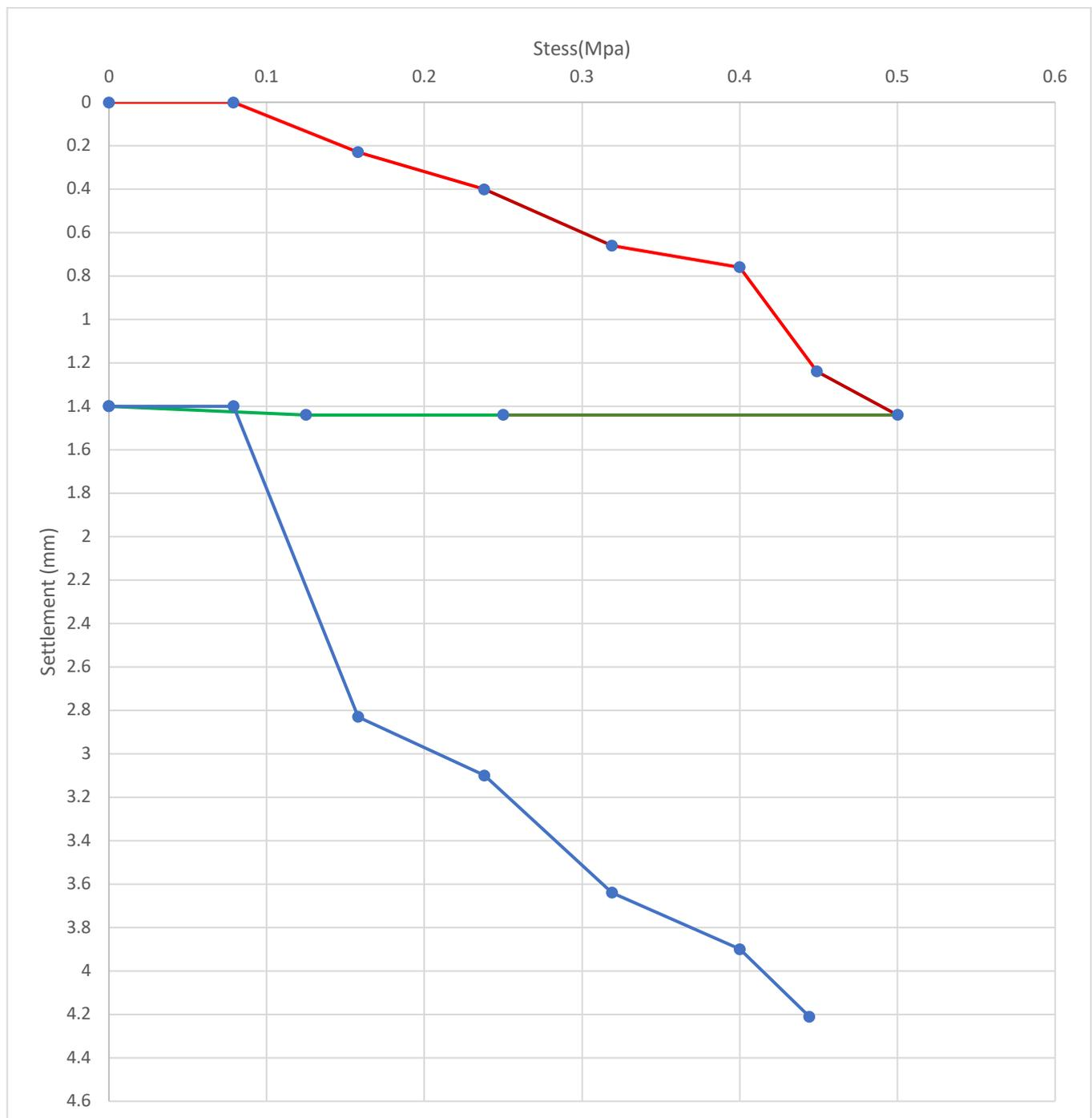
Fig 4.28 Stress vs Settlement curve (pt 10, GL)
