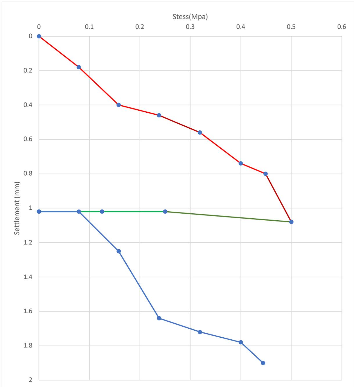
Fig 4.36 Stress vs Settlement curve (pt 12, ballast layer)
