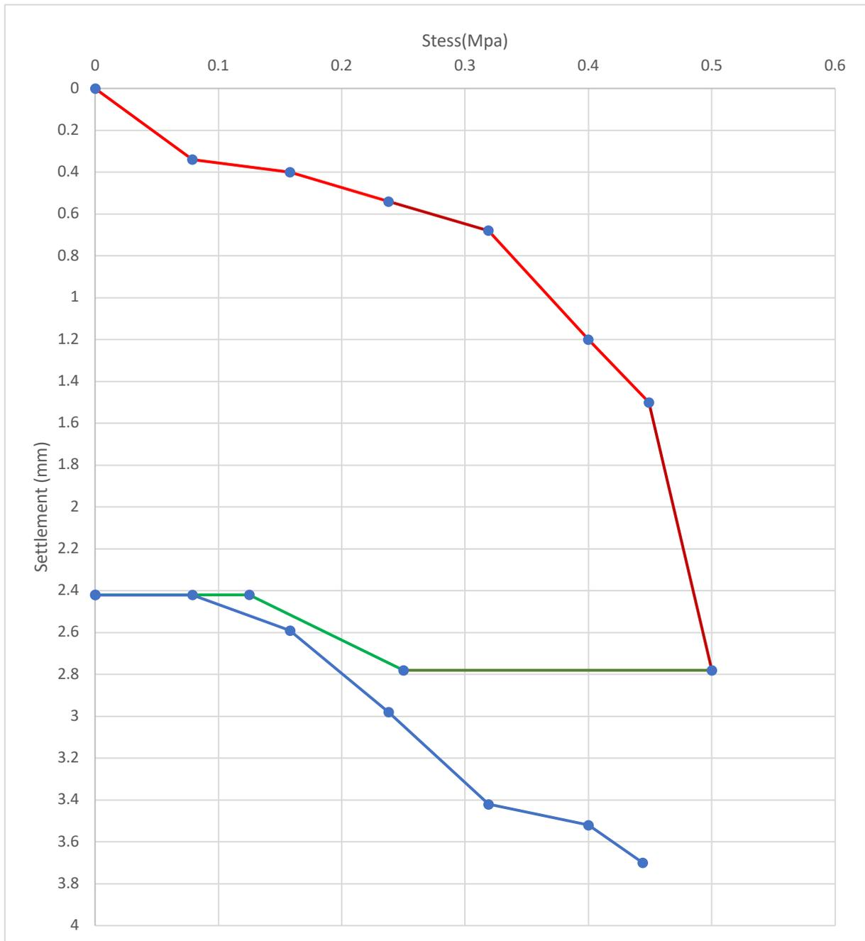
Fig 4.26 Stress vs Settlement curve (pt 9, subgrade)
