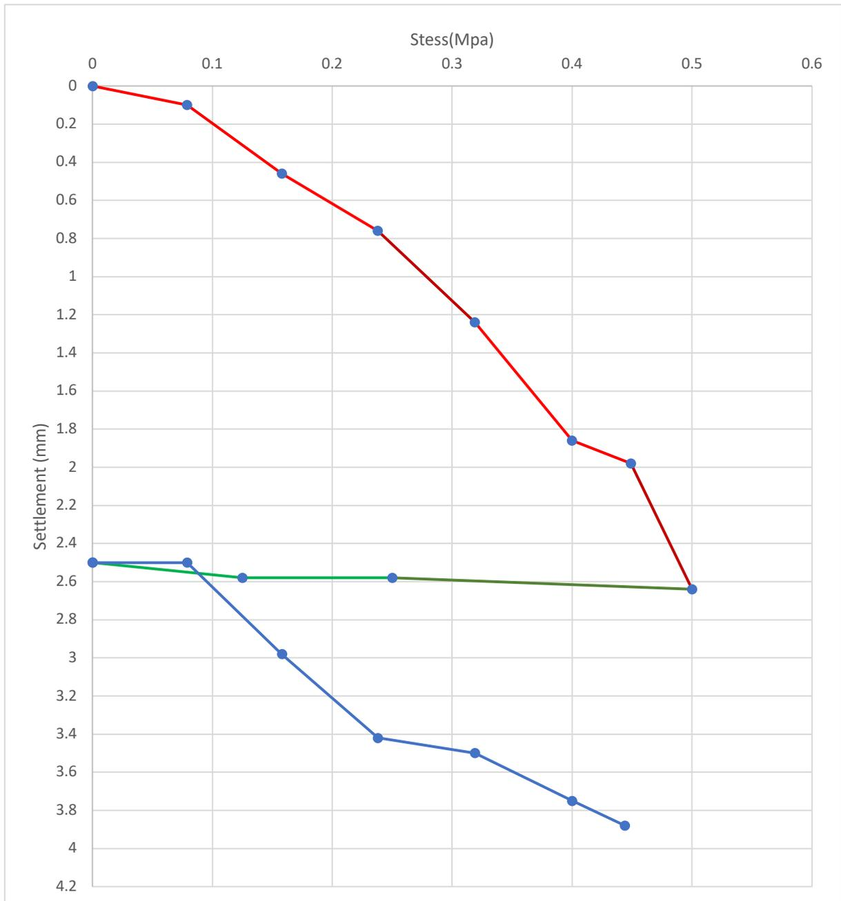
Fig 4.35 Stress vs Settlement curve (pt 12, subgrade)
