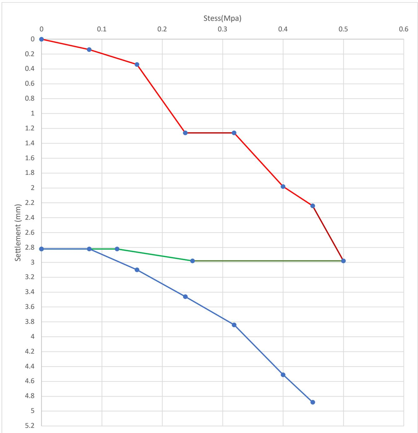
Fig 4.10 Stress vs Settlement curve (pt 4, GL)
