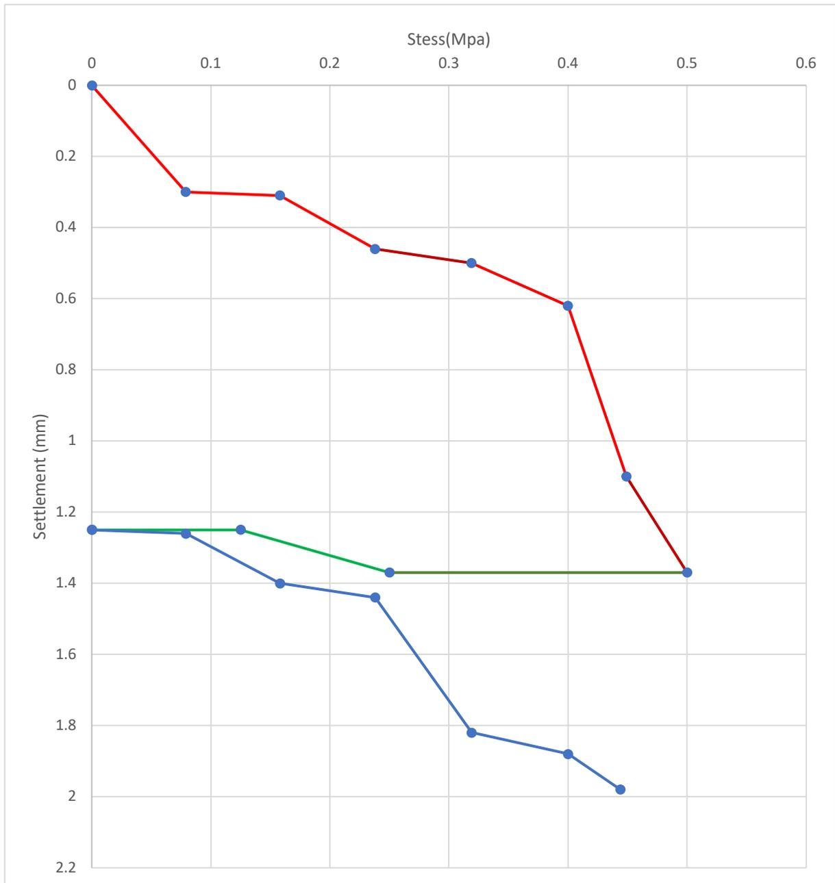
Fig 4.30 Stress vs Settlement curve (pt 10, ballast layer)
