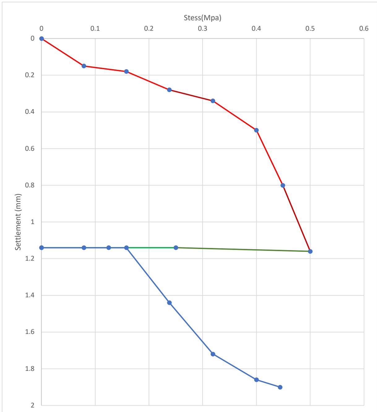
Fig 4.21 Stress vs Settlement curve (pt 7, ballast layer)
