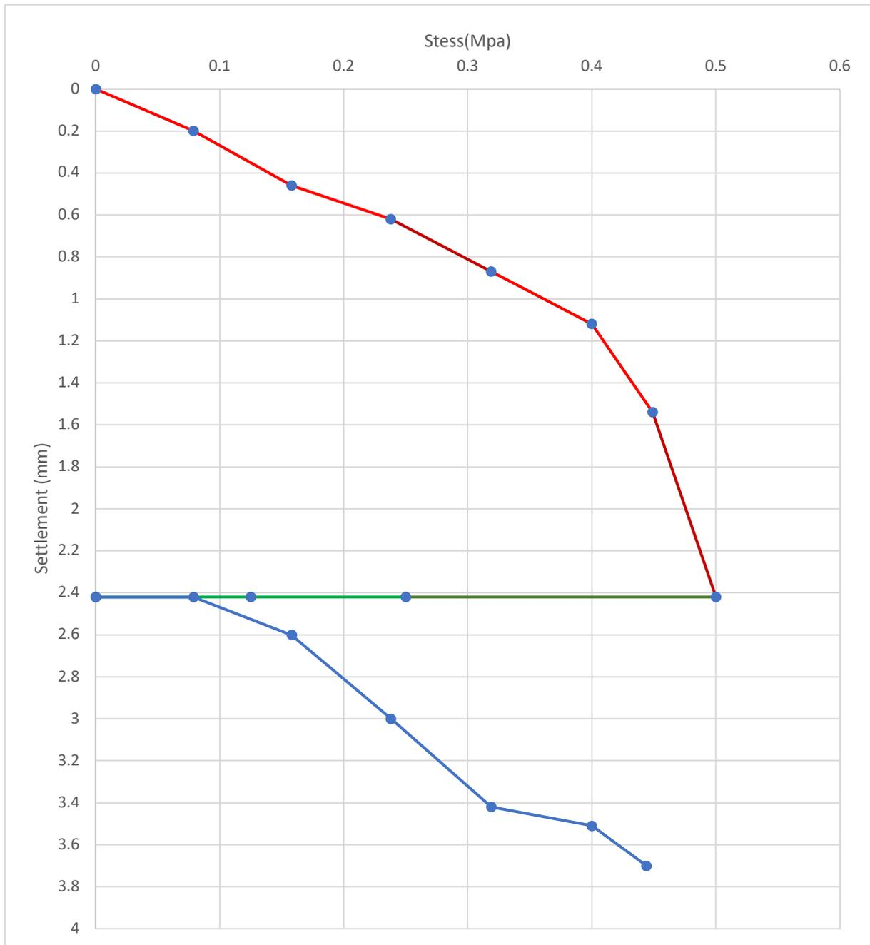
Fig 4.29 Stress vs Settlement curve (pt 10, subgrade)
