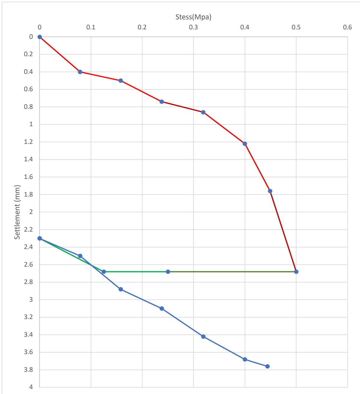
Fig 4.32 Stress vs Settlement curve (pt 11, subgrade)
