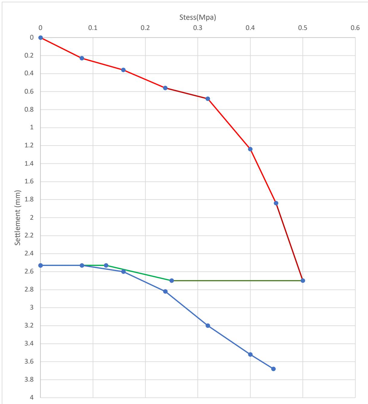
Fig 4.23 Stress vs Settlement curve (pt 8, subgrade)
