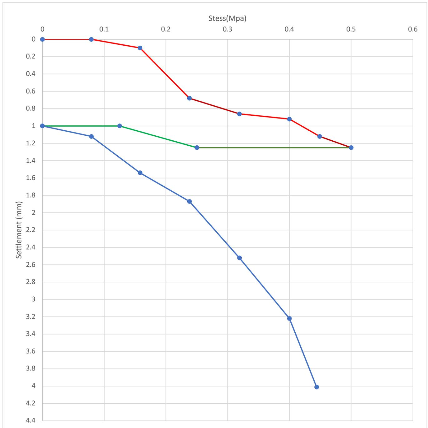
Fig 4.31 Stress vs Settlement curve (pt 11, GL)
