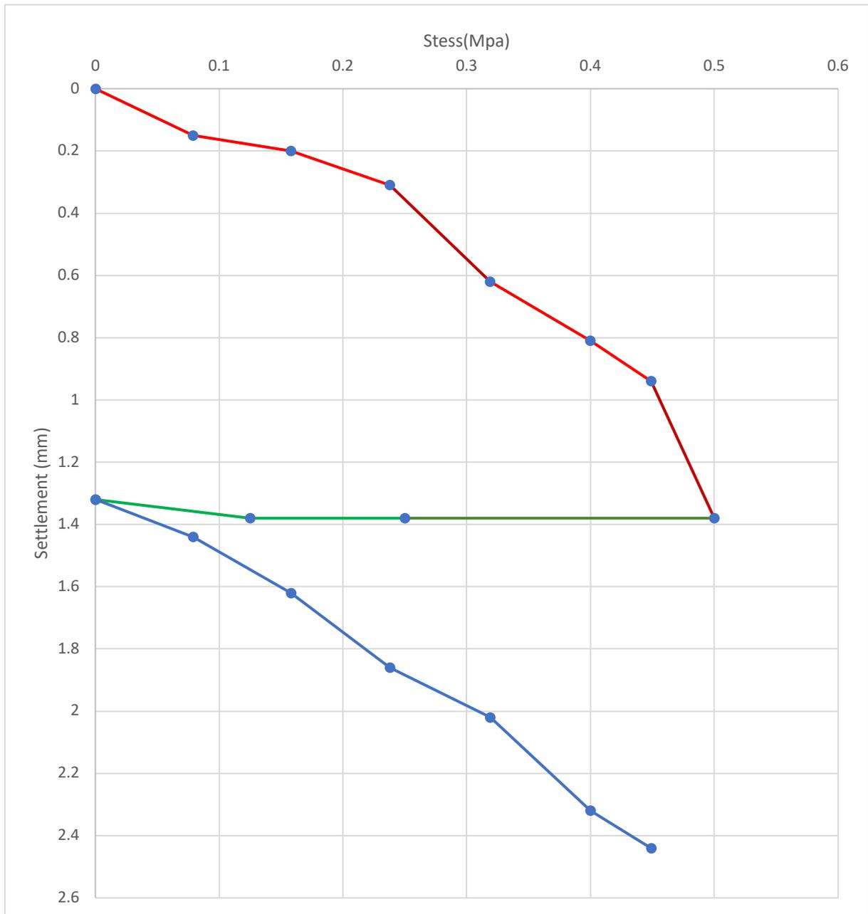
Fig 4.17 Stress vs Settlement curve (pt 6, subgrade)
