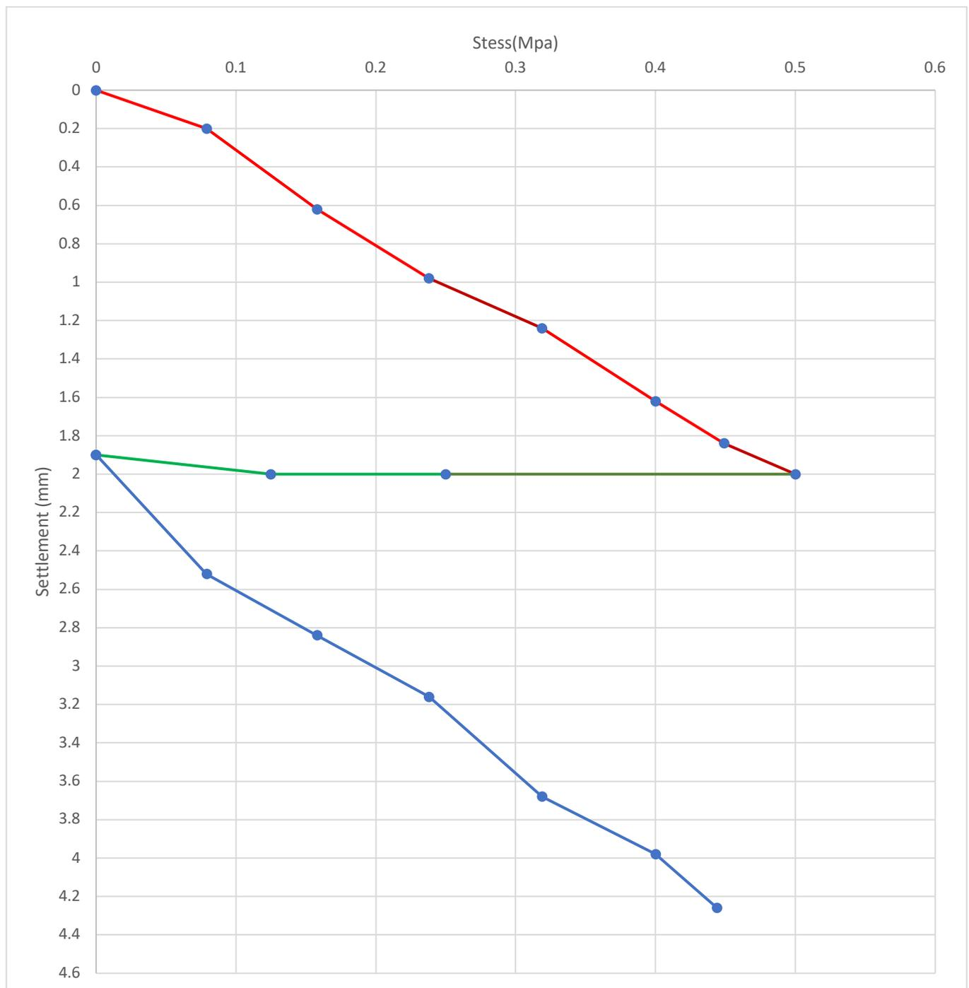
Fig 4.25 Stress vs Settlement curve (pt 9, GL)
