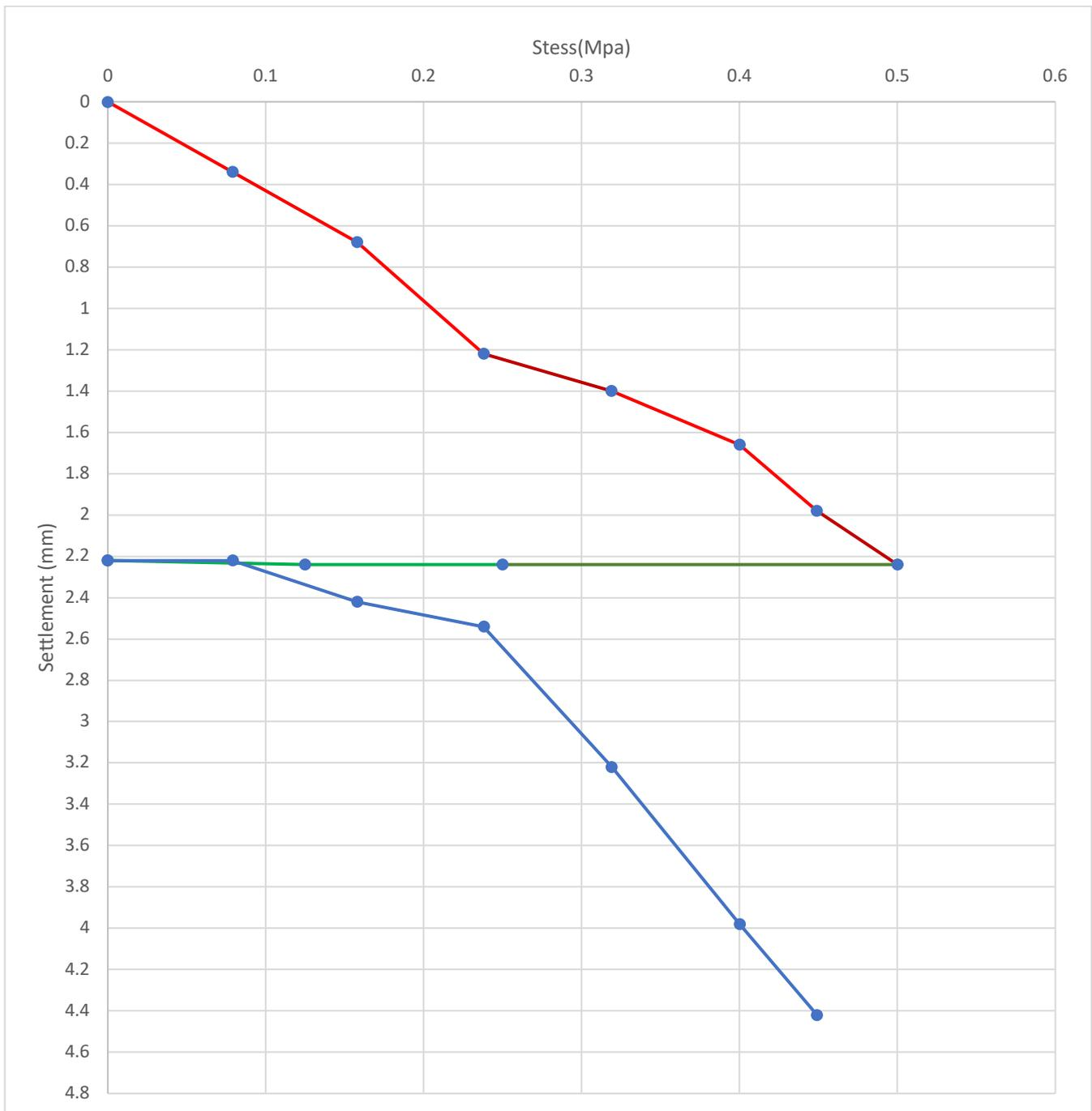
Fig 4.19 Stress vs Settlement curve (pt 7, GL)
