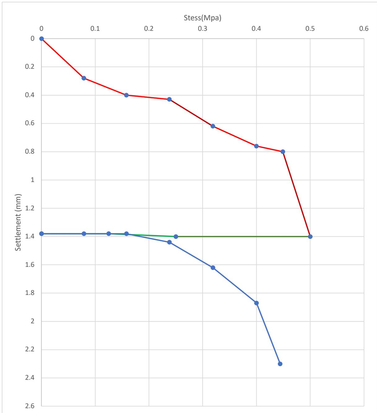
Fig 4.24 Stress vs Settlement curve (pt 8, ballast layer)
