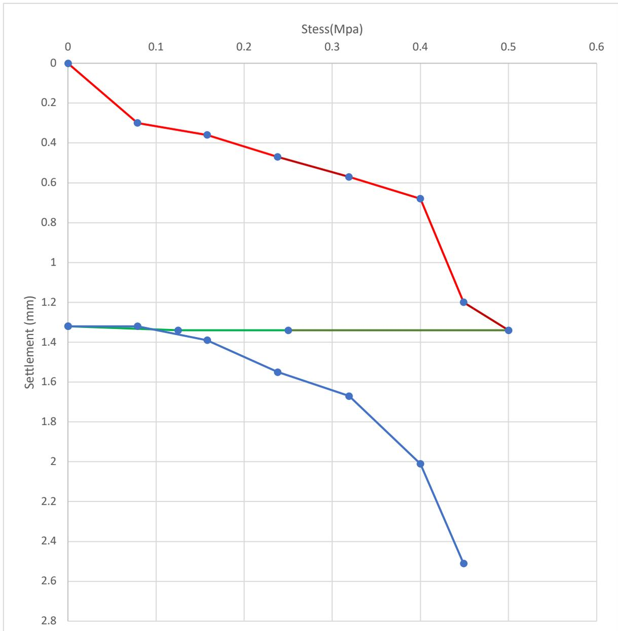
Fig 4.5 Stress vs Settlement curve (pt 2, subgrade)
