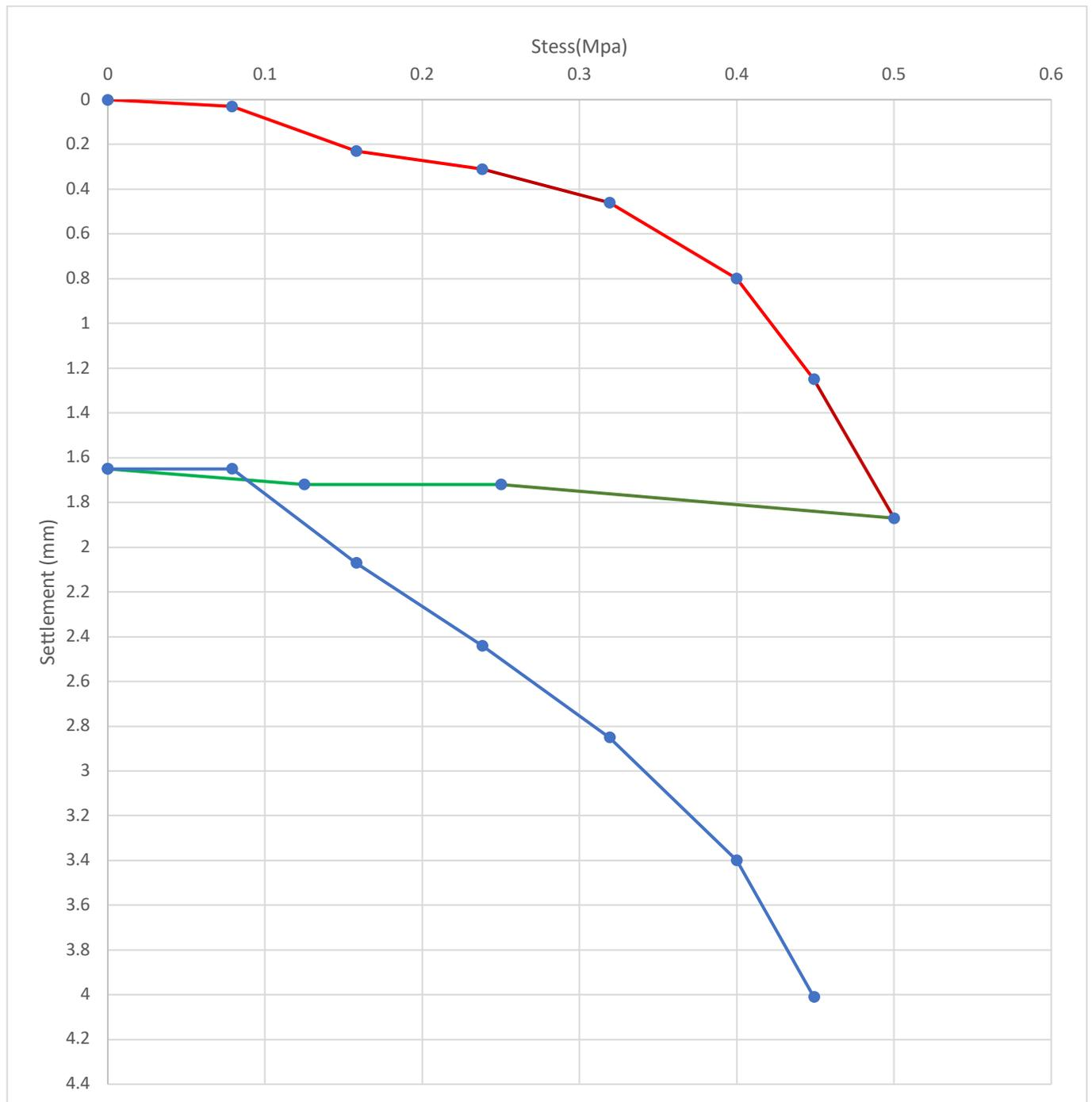
Fig 4.16 Stress vs Settlement curve (pt 6, GL)
