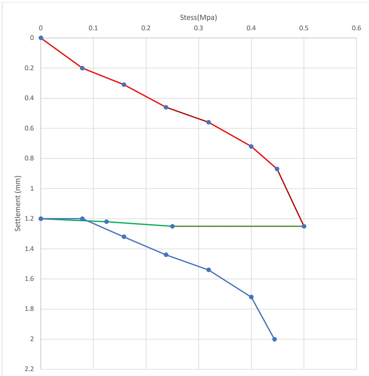
Fig 4.3 Stress vs Settlement curve (pt 1, ballast layer)
