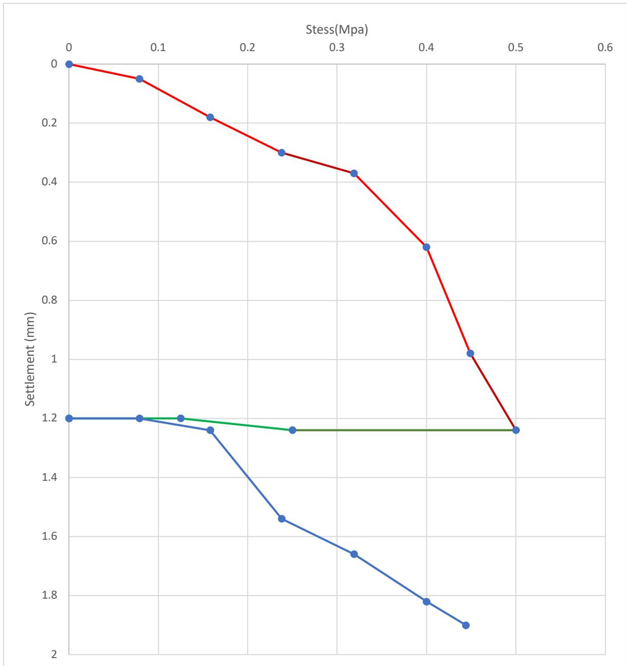
Fig 4.18 Stress vs Settlement curve (pt 6, ballast layer)
