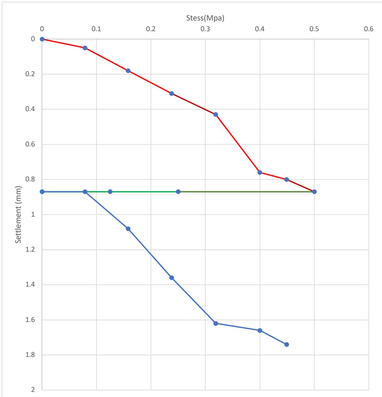
Fig 4.12 Stress vs Settlement curve (pt 4, ballast layer)
