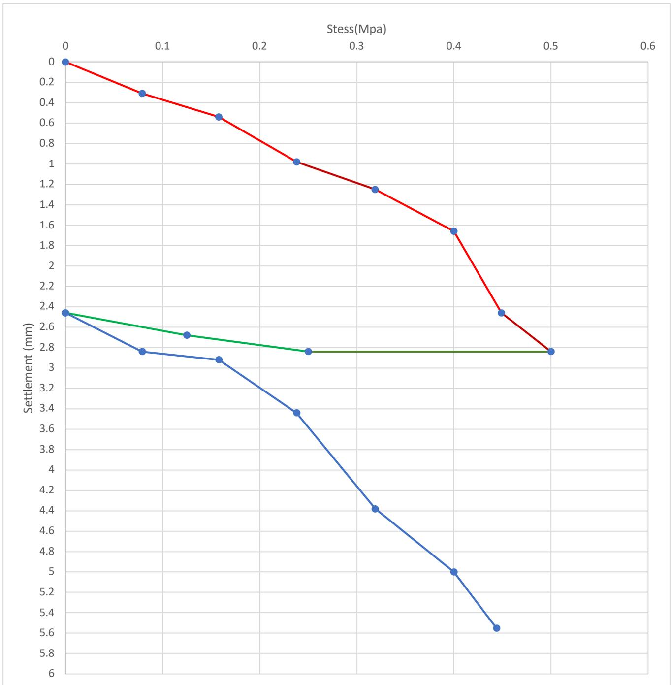
Fig 4.22 Stress vs Settlement curve (pt 8, GL)
