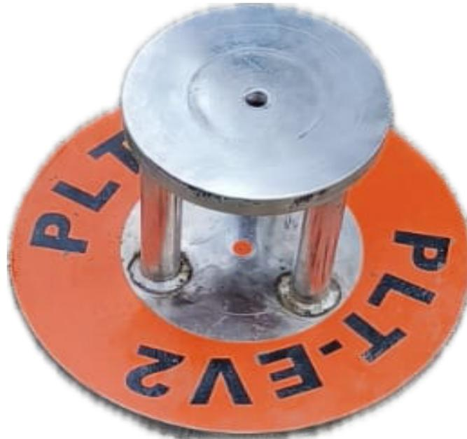
Fig 3.2 300 mm loading plate with measuring tunnel
