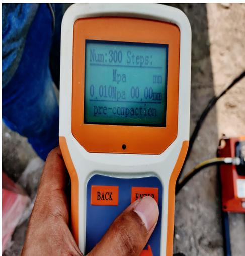
Fig: 3.8 Pre loading of 10 kN/m<sup>2</sup>
