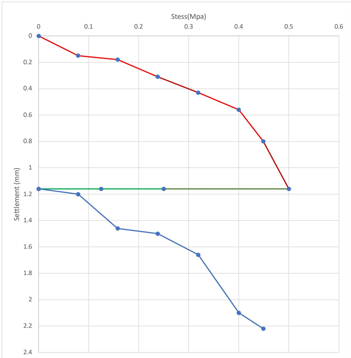
Fig 4.11 Stress vs Settlement curve (pt 4, subgrade)
