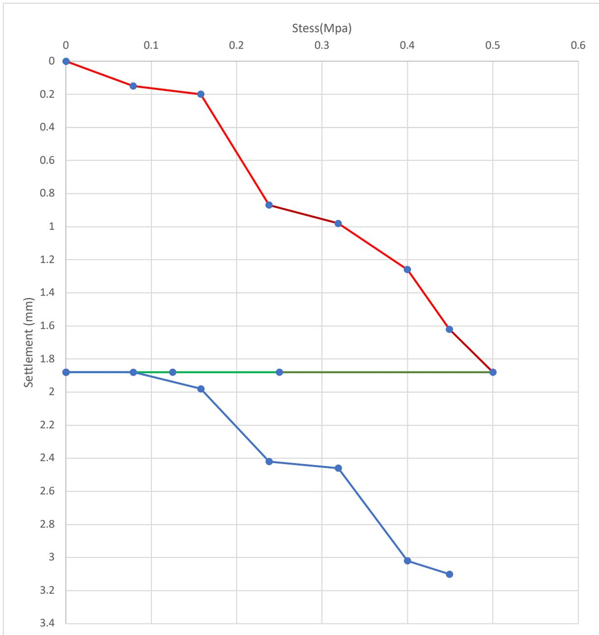
Fig 4.14 Stress vs Settlement curve (pt 5, subgrade)
