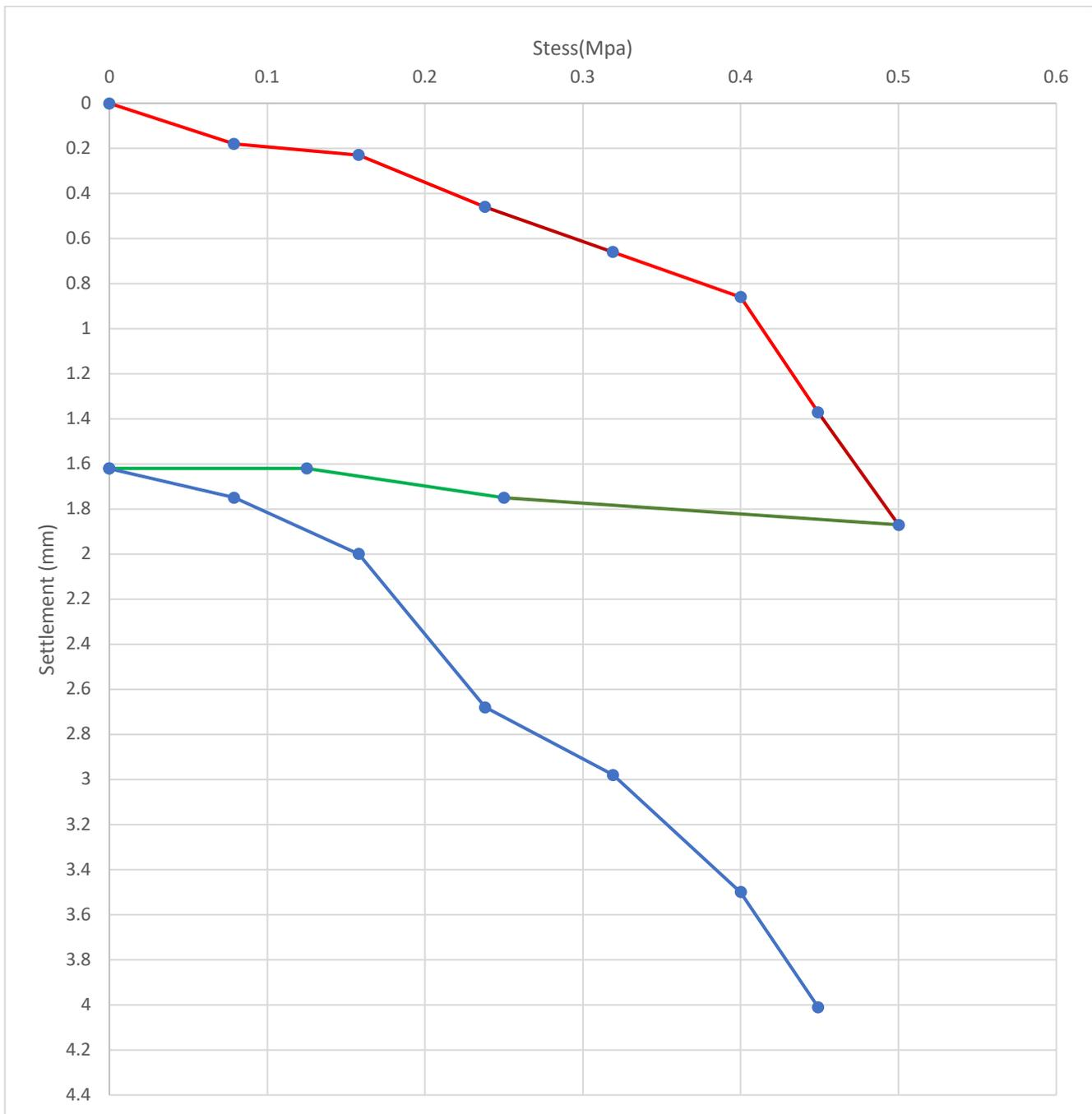
Fig 4.13 Stress vs Settlement curve (pt 5, GL)
