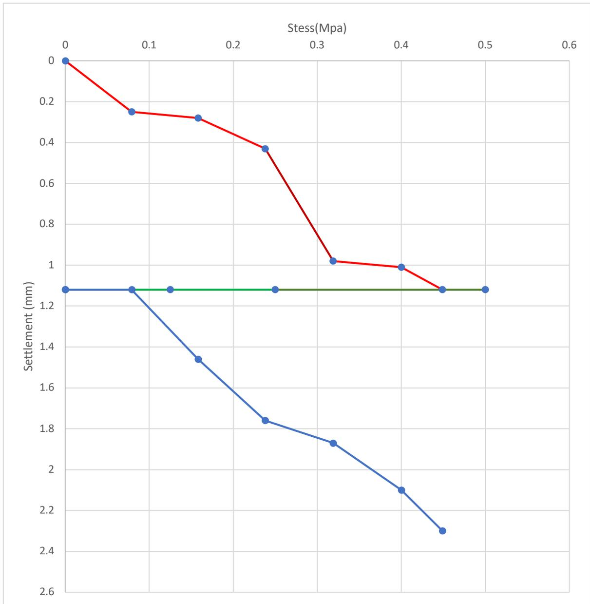
Fig 4.8 Stress vs Settlement curve (pt 3, subgrade)
