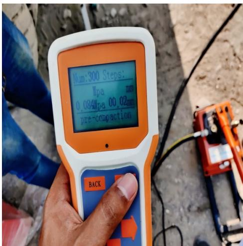
Fig 3.9 First loading of 80 kN/m<sup>2</sup>.
