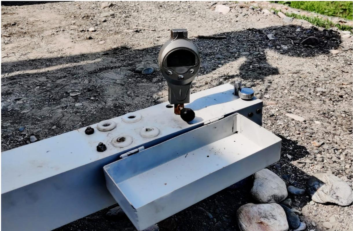
Fig 3.5 A digital displacement transducer or dial gauge
