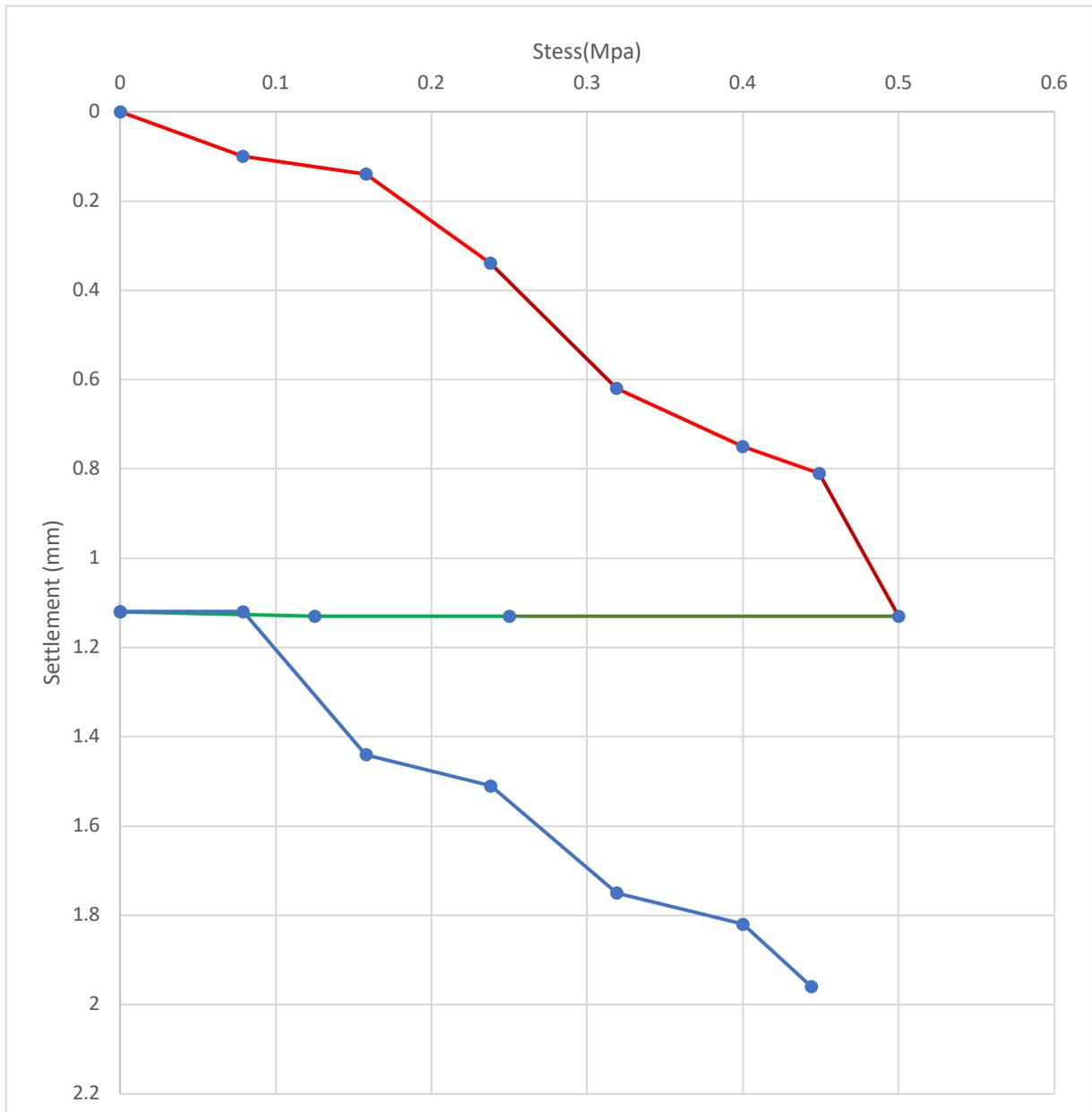
Fig 4.6 Stress vs Settlement curve (pt 2, ballast layer)
