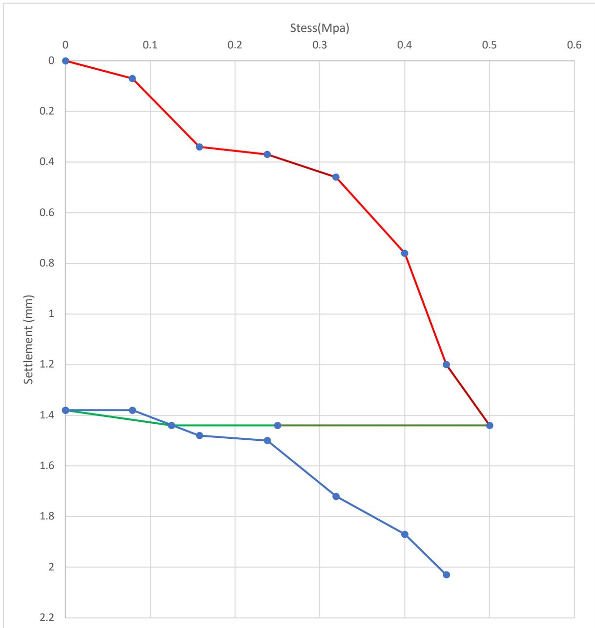
Fig 4.15 Stress vs Settlement curve (pt 5, ballast layer)
