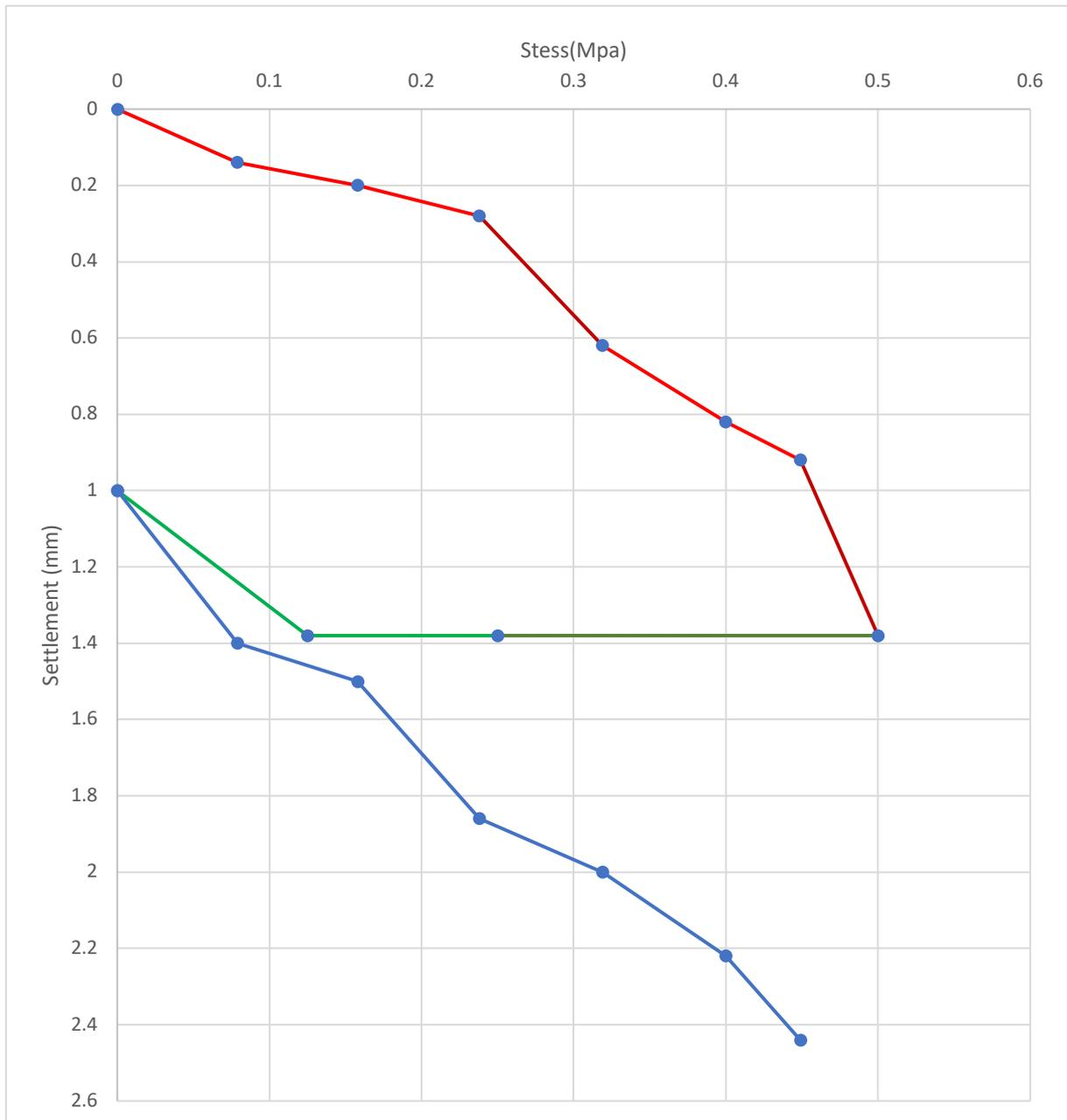
Fig 4.20 Stress vs Settlement curve (pt 7, subgrade)
