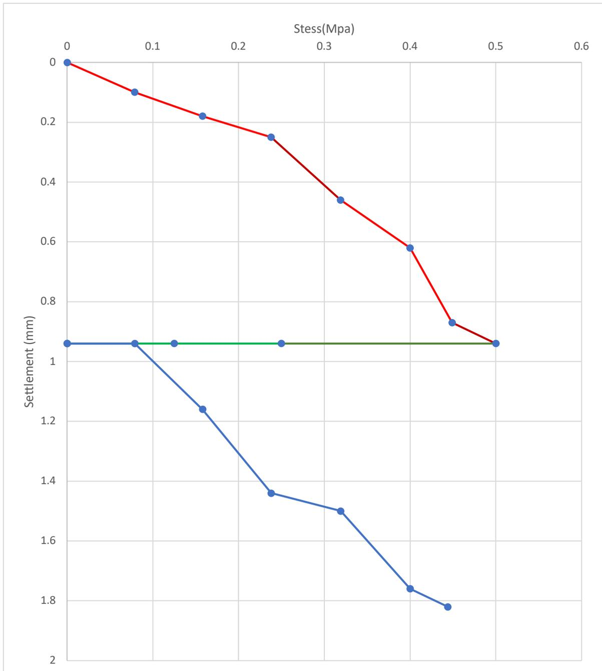
Fig 4.33 Stress vs Settlement curve (pt 11, ballast layer)
