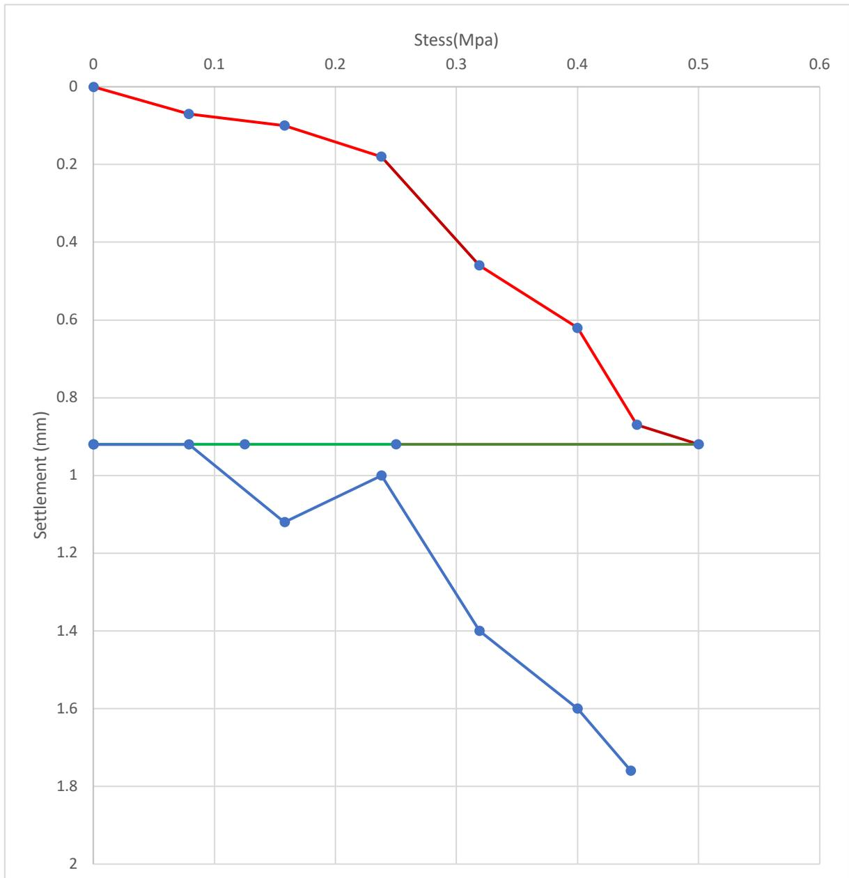
Fig 4.9 Stress vs Settlement curve (pt 3, ballast layer)
