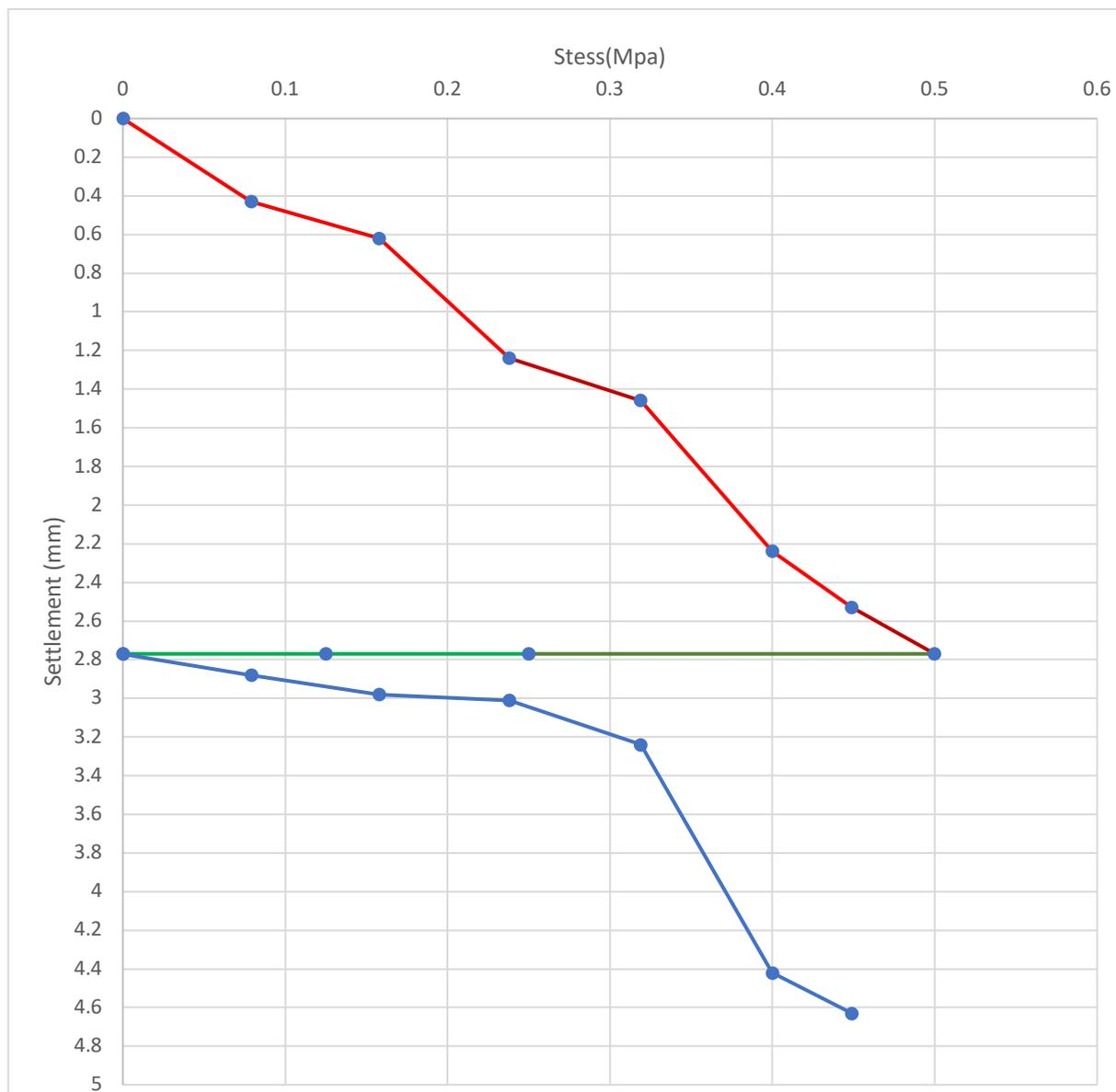
Fig 4.4 Stress vs Settlement curve (pt 2, GL)
