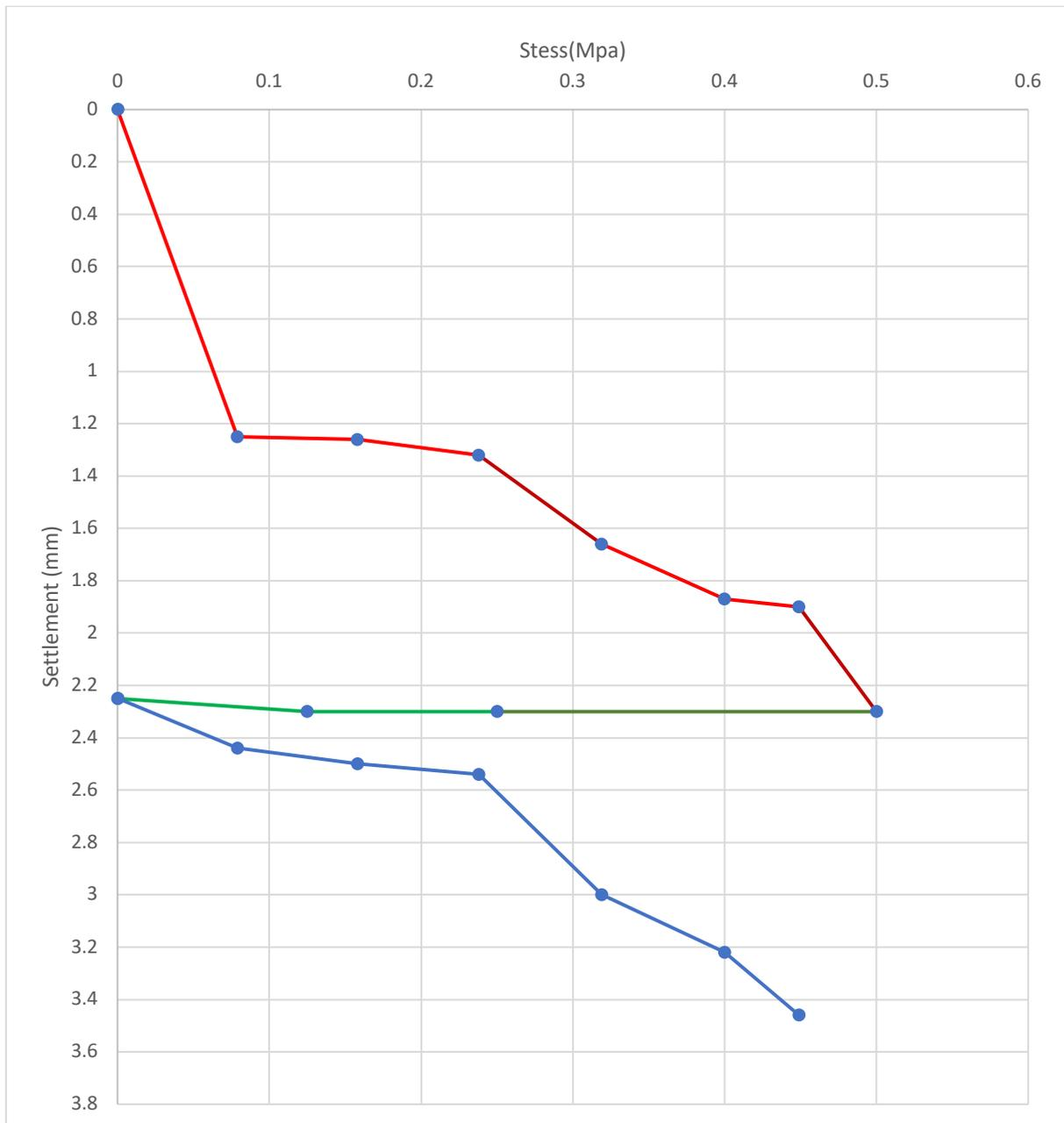
Fig 4.2 Stress vs Settlement curve (pt 1, subgrade)
