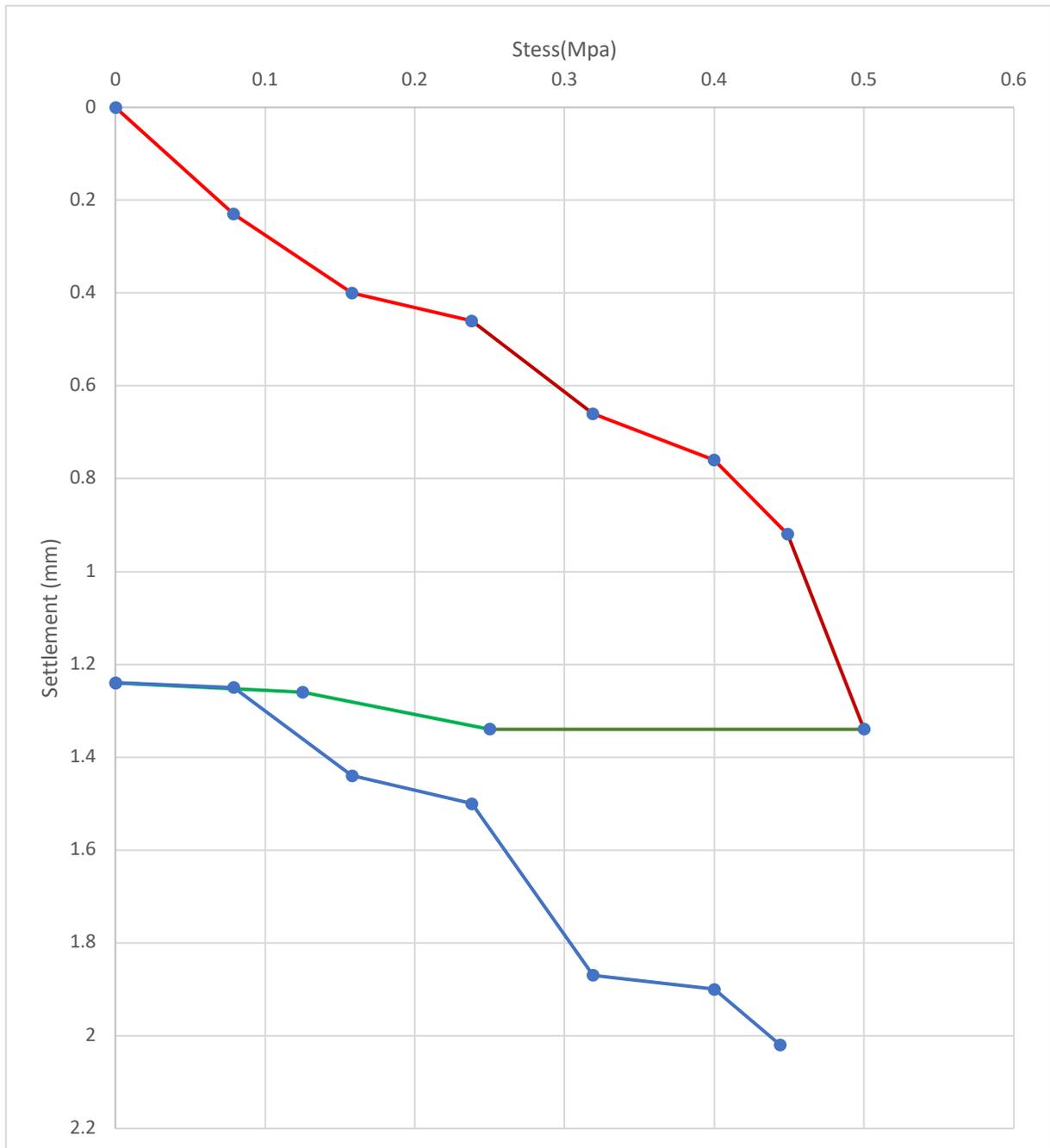
Fig 4.27 Stress vs Settlement curve (pt 9, ballast layer)
