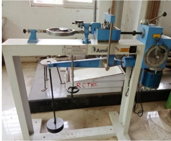
Figure 4.9 Test setup-DST machine.(AIMIL-Manually operated)
