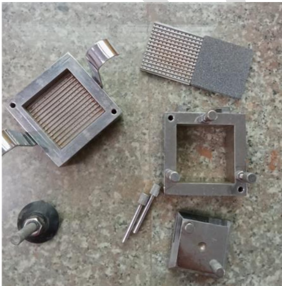
Figure 4.7 Direct Shear Box Parts
