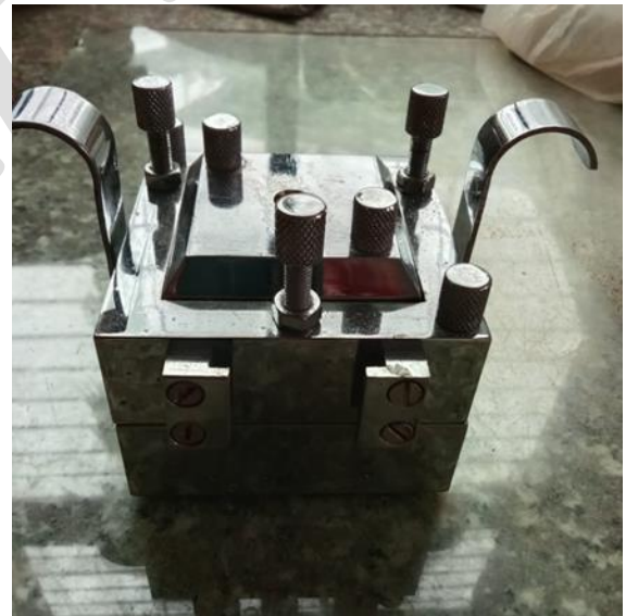
Figure 4.8 Direct Shear box with soil
