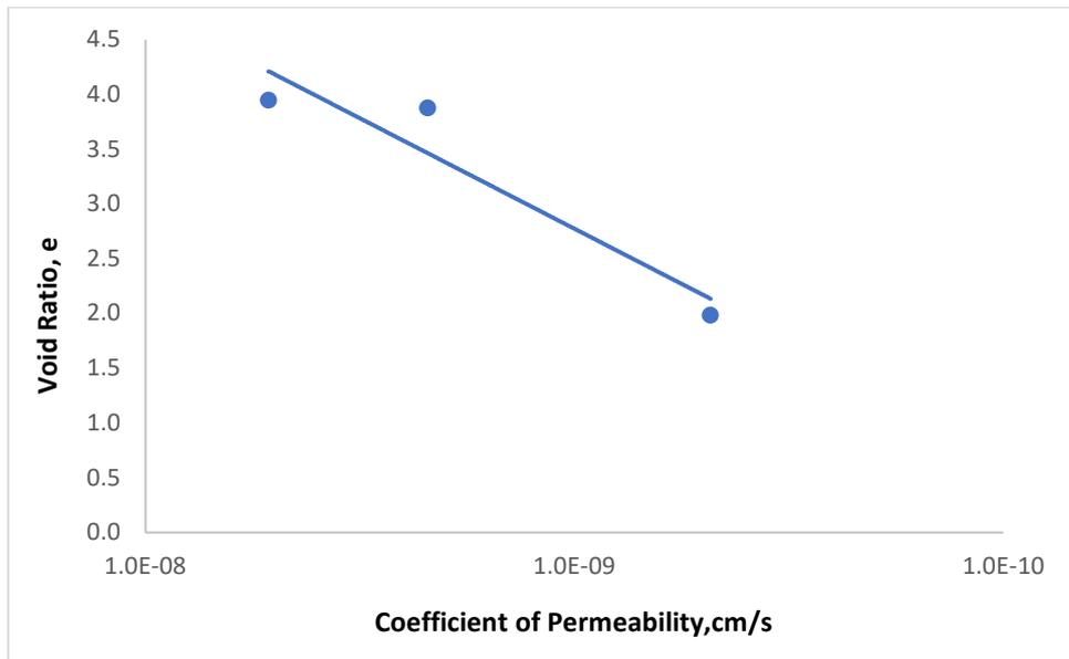
**Fig.6.1: Coefficient of permeability vs. void ratio relationship for 100% Distilled water**
