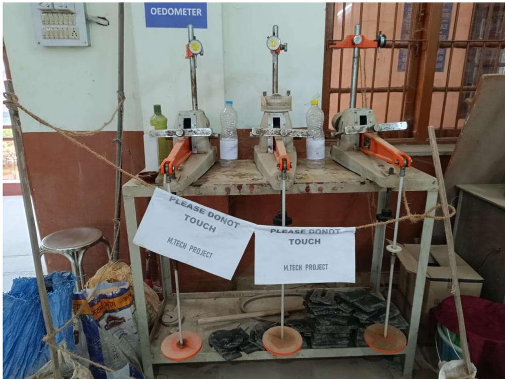
**Fig3.1: Consolidation setup**
