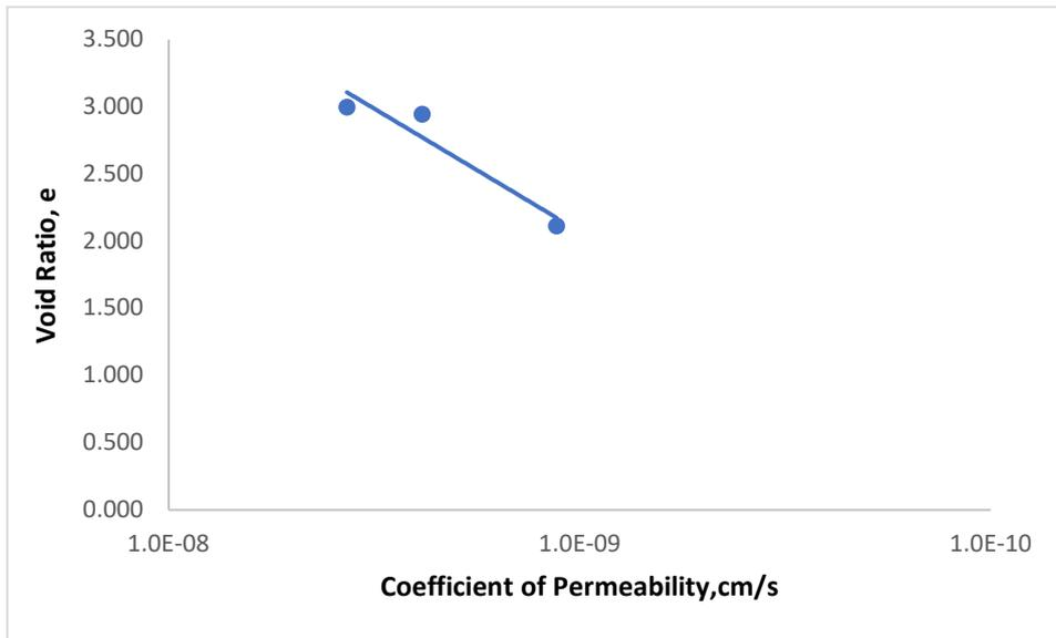
**Fig6.5: Coefficient of permeability vs. void ratio relationship for 80%Ethanol+ 20% Distilled water**
