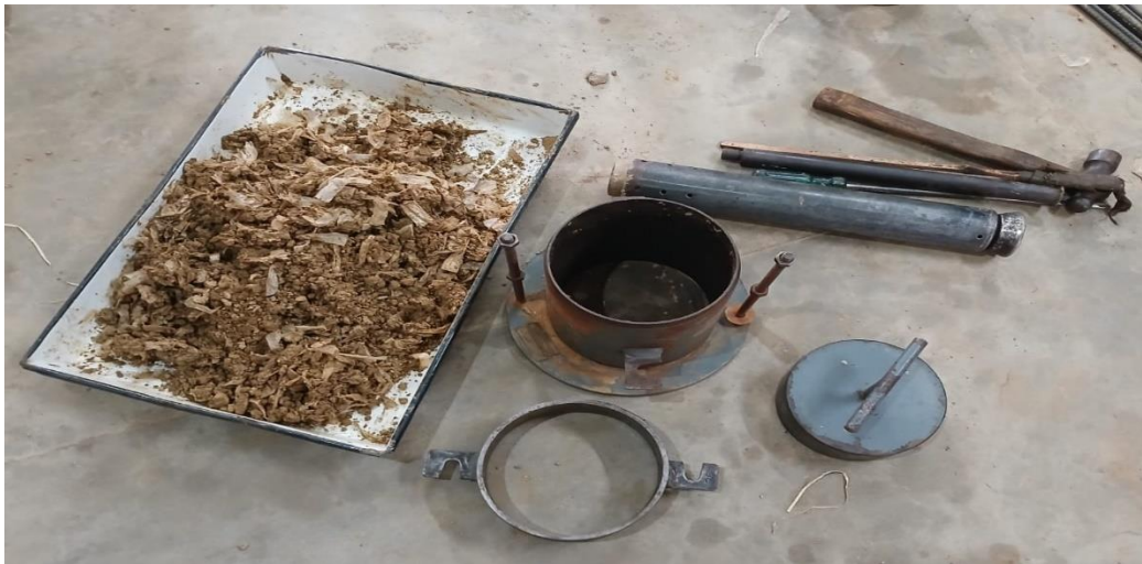
Fig 3.10 CBR mould, base plate collar,spacer disc, rammer
