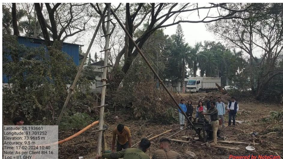
Fig.4.2 Photograph of Standard Penetration Test conducted at site
