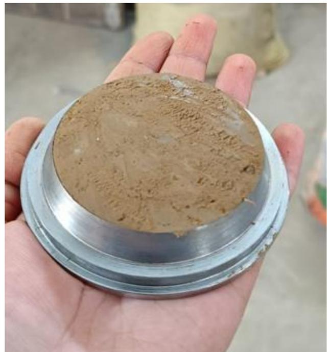
**Figure 4.3: Lower surface of consolidation sample**
