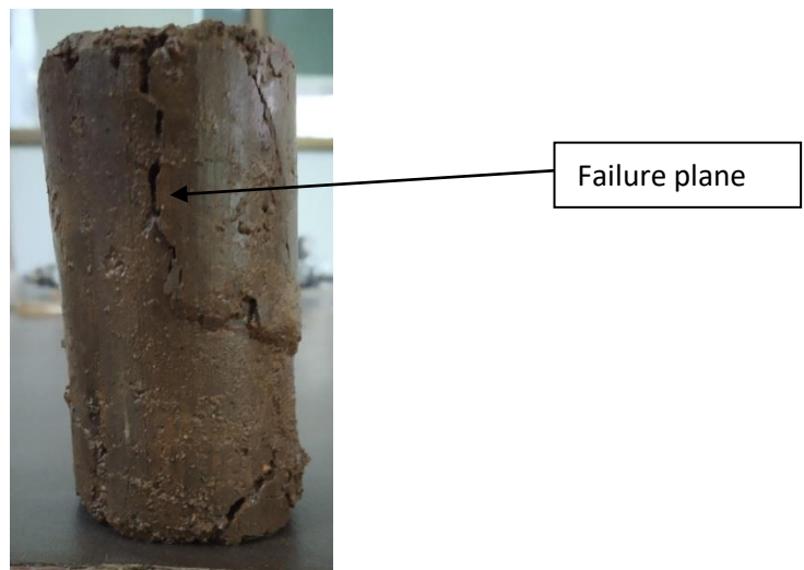
Figure 5.56: Failed sample at 150kPa cell pressure for lime 2% and cement 4% stabilized soil (7 th day curing)
