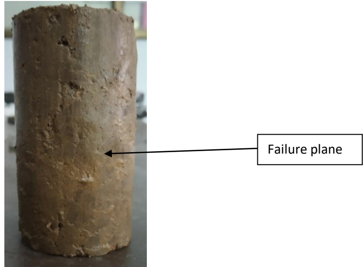
Figure 5.39: Failed sample at 50kPa cell pressure for cement 2% and lime 8% stabilized soil (0 th day curing)
