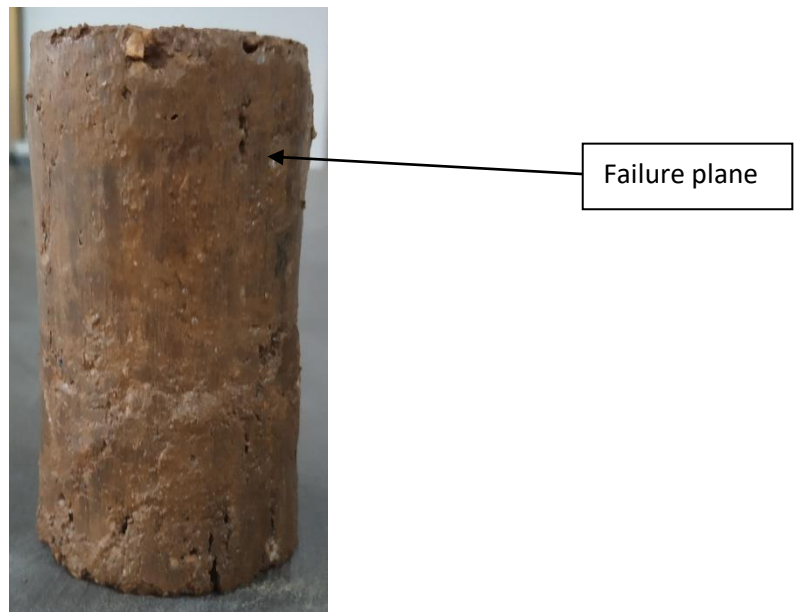
Figure 5.40: Failed sample at 100kPa cell pressure for cement 2% and lime 8% stabilized soil (0 th day curing)
