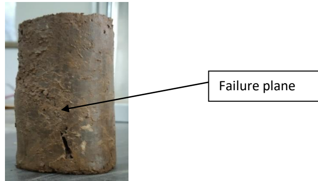
Figure 5.51: Failed sample at 150kPa cell pressure for lime 2% and cement 4% stabilized soil (0 th day curing)
