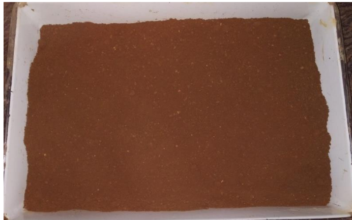
Figure 4.8: Cement lime stabilized soil (lime 2% + cement 4%)
