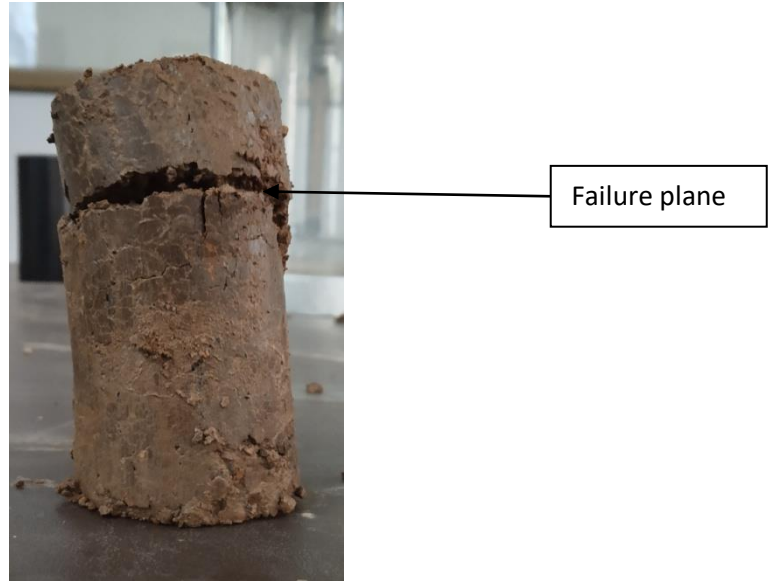
Figure 5.19: Failed sample at 50kPa cell pressure for cement 2% and lime 4% stabilized soil (0 th day curing)
