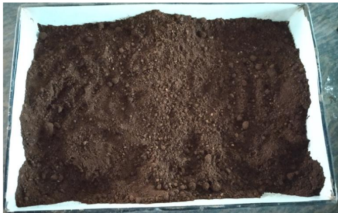
Figure 4.6: Cement lime stabilized soil (cement 2% + lime 6%)
