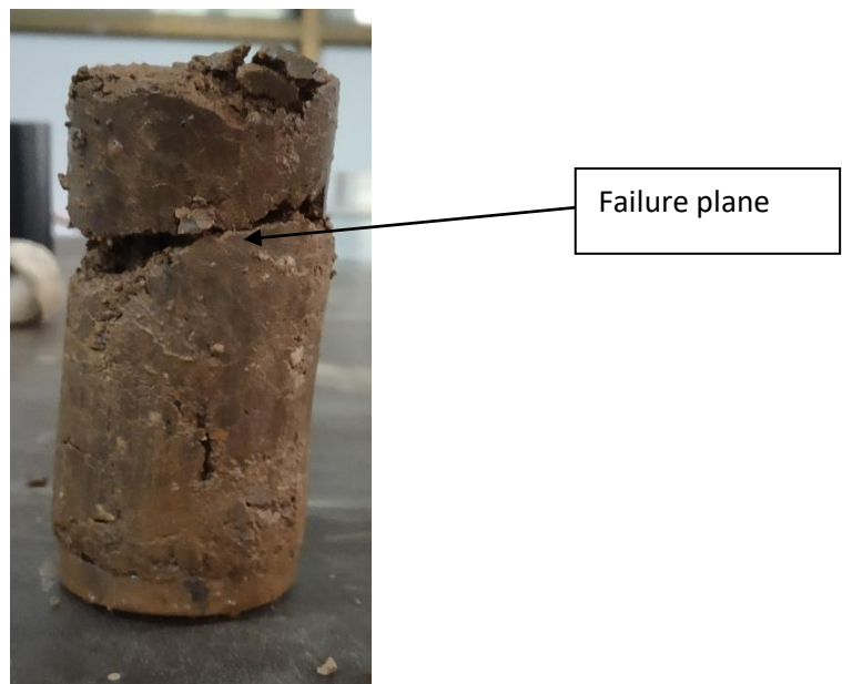
Figure 5.20: Failed sample at 100kPa cell pressure for cement 2% and lime 4% stabilized soil (0 th day curing)
