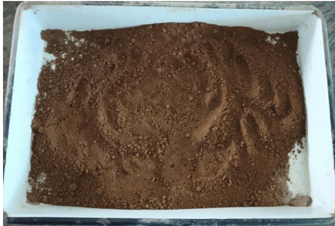
Figure 4.4: Cement lime stabilized soil (cement 2% + lime 2%)
