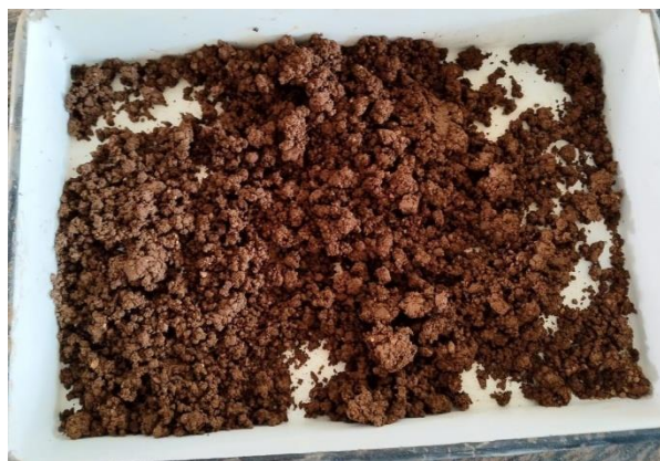
Figure 4.3: Uniform mixture of soil and water (cement 0% + lime 0%)
