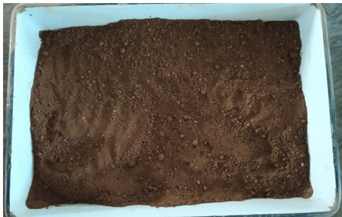
Figure 4.5: Cement lime stabilized soil (cement 2% + lime 4%)
