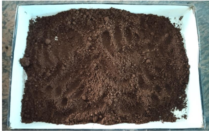
Figure 4.7: Cement lime stabilized soil (cement 2% + lime 8%)
