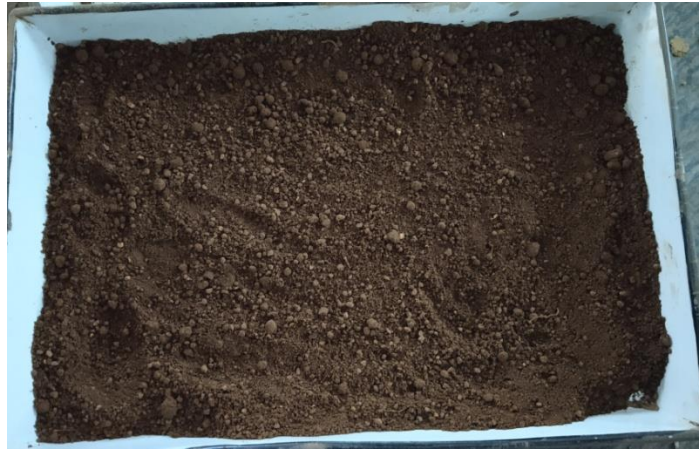
Figure 4.10: Cement lime stabilized soil (lime 2% + cement 8%)
