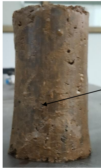
Figure 5.49: Failed sample at 50kPa cell pressure for lime 2% and cement 4% stabilized soil (0 th day curing)
