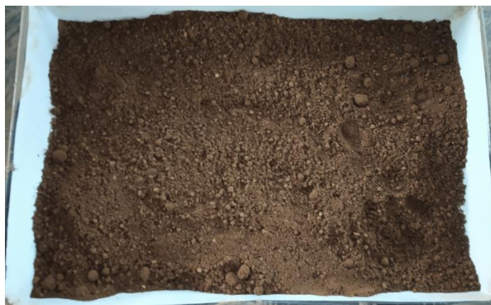
Figure 4.9: Cement lime stabilized soil (lime 2% + cement 6%)
