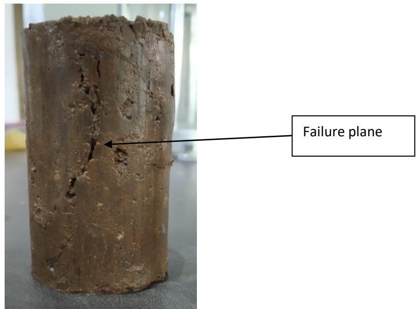
Figure 5.70: Failed sample at 100kPa cell pressure for lime 2% and cement 8% stabilized soil (0 th day curing)
