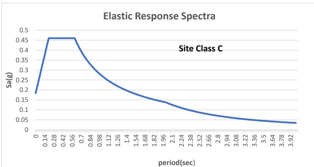
**Figure 7.8 - Representing Design Spectrum for Goalpara Station**
