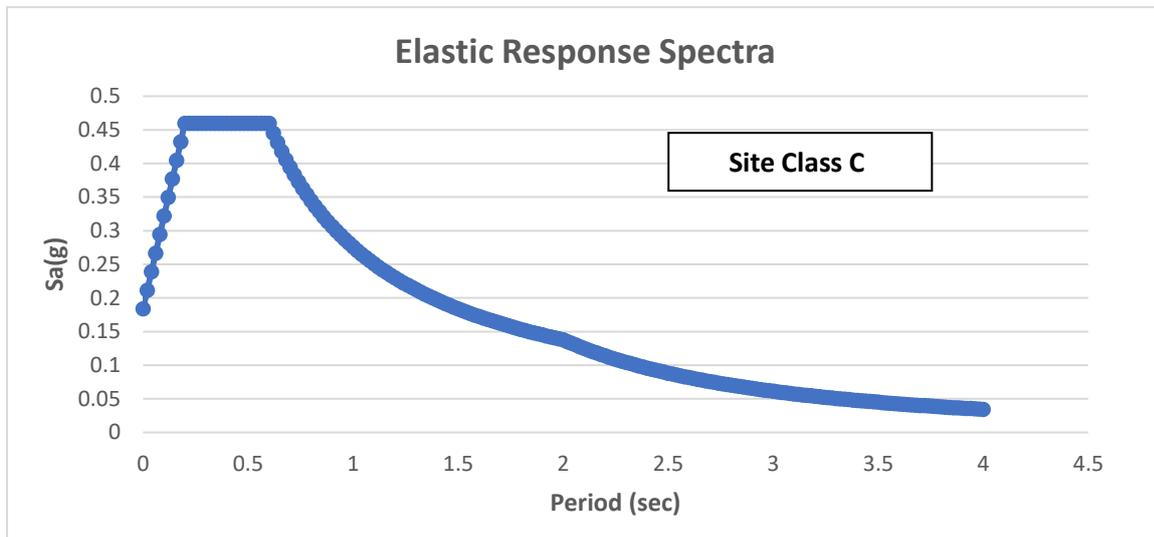
**Figure 7.6 Representing elastic Response Spectra of Boko Station**
