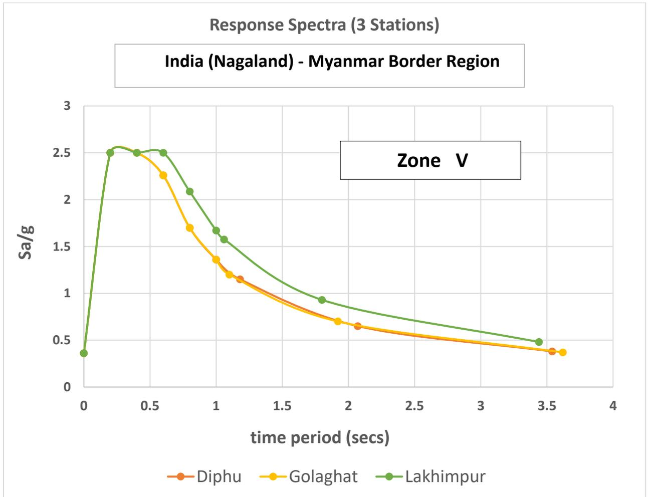
**Figure 7.4** Plot of time period vs Sa/g of 24 Feb 2009 Earthquake
