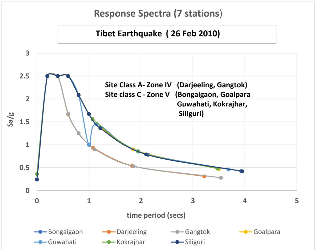
**Figure 7.3 Plot between time period vs Sa/g of 26 Feb 2010 Earthquake**
