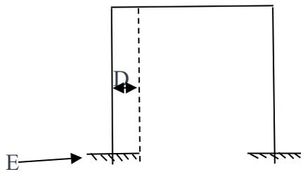
**Figure 2.1 - Building with no mass (moves back and forth with no force generated)**
