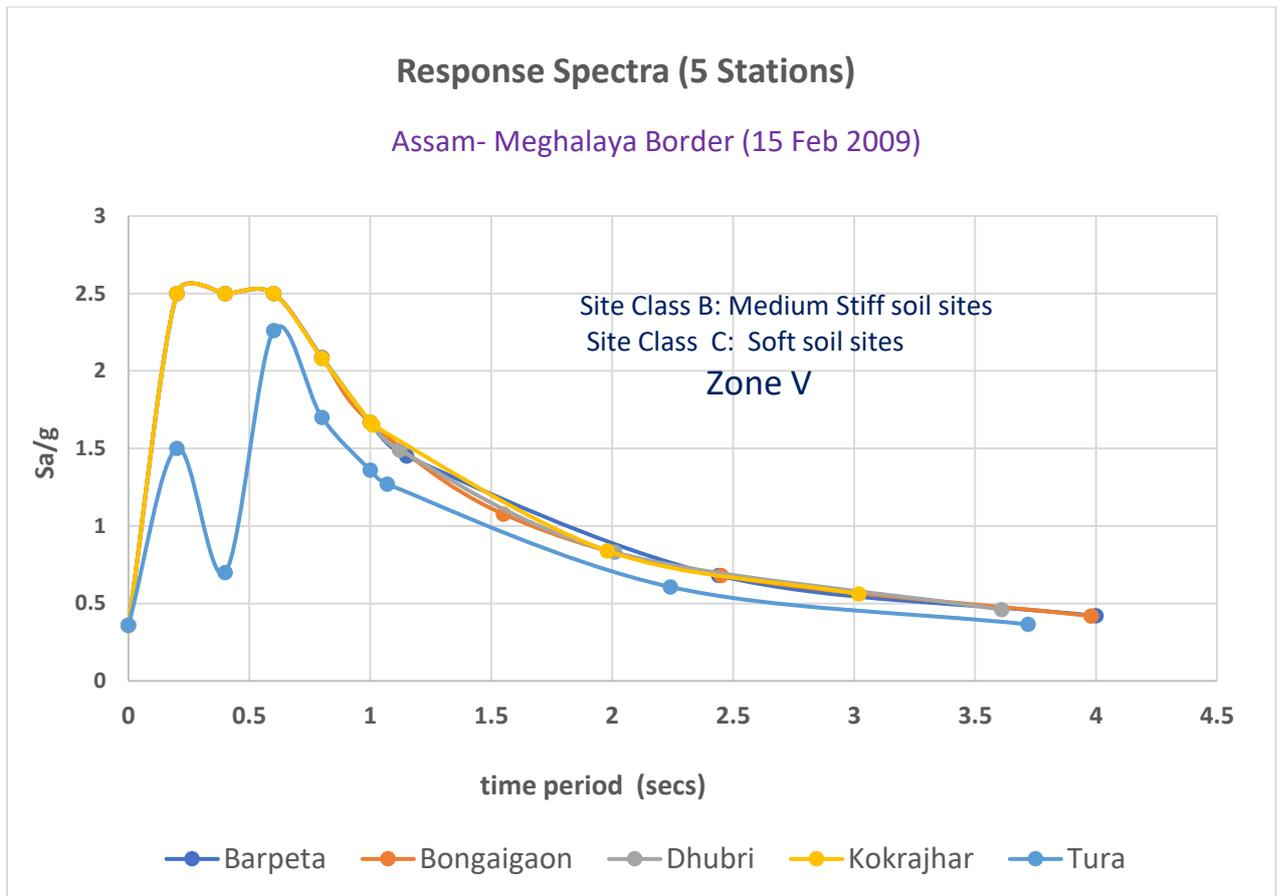
**Figure 7.2 : Plot of time period vs Sa/g of 15 Feb 2009 Earthquake**
