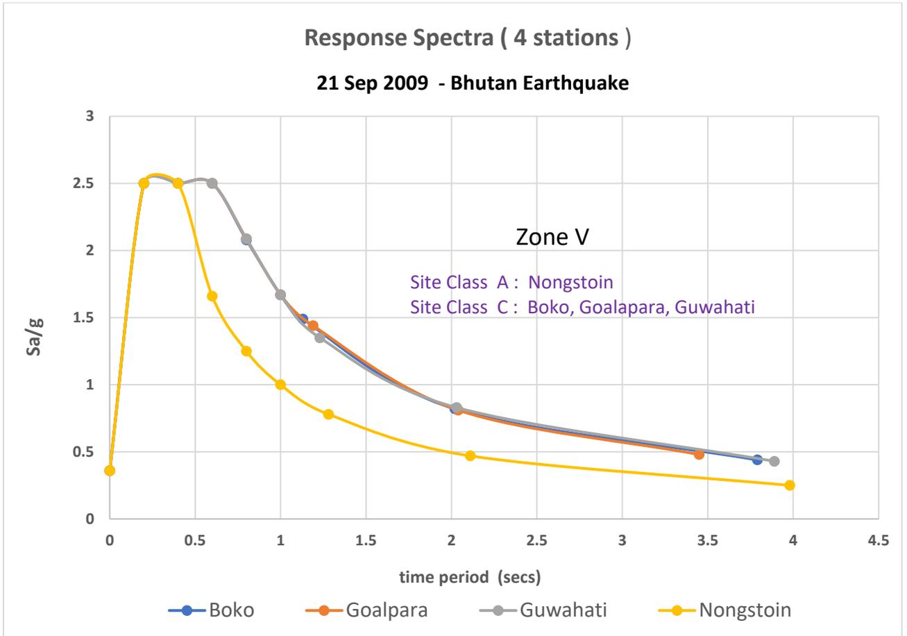
**Figure 7.1 : Plot between time period vs Sa/g of 21 Sep 2009 Bhutan Earthquake**
