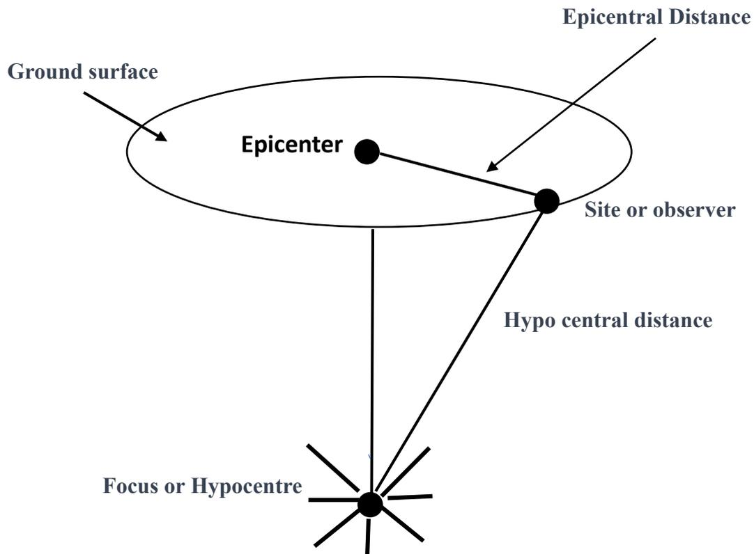
**Figure 1 : Notation for description of earthquake (Kramer 1996)**
