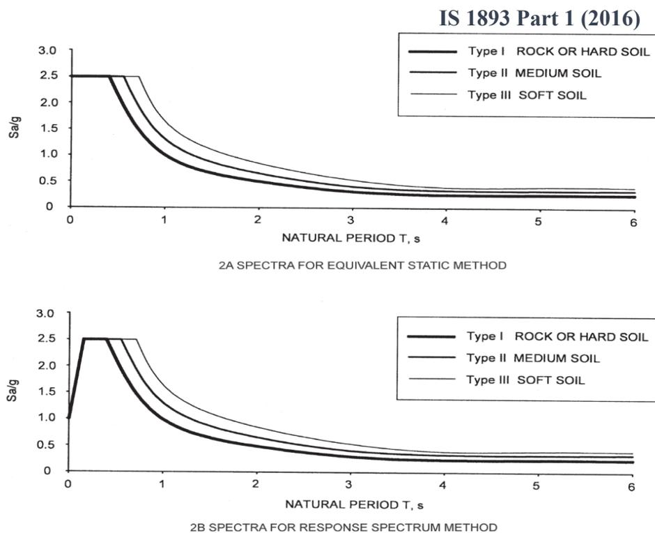
**Figure 2.3: Design Acceleration Coefficients ( $S_a/g$ ) (Corresponding to 5% Damping)**
