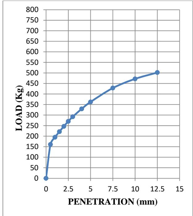
**Fig.3.18: Load-penetration curve at OMC-3% of sample1 (statically compacted soil)**
