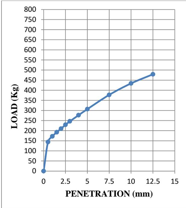
**Fig 3.17: Load-penetration curve at OMC-3% of sample 1 (dynamically compacted soil)**
