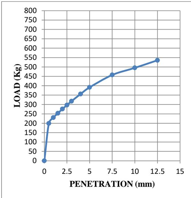
**Fig. 3.35: Load-penetration curve at OMC-3% of sample 4 (Dynamically compacted soil)**
