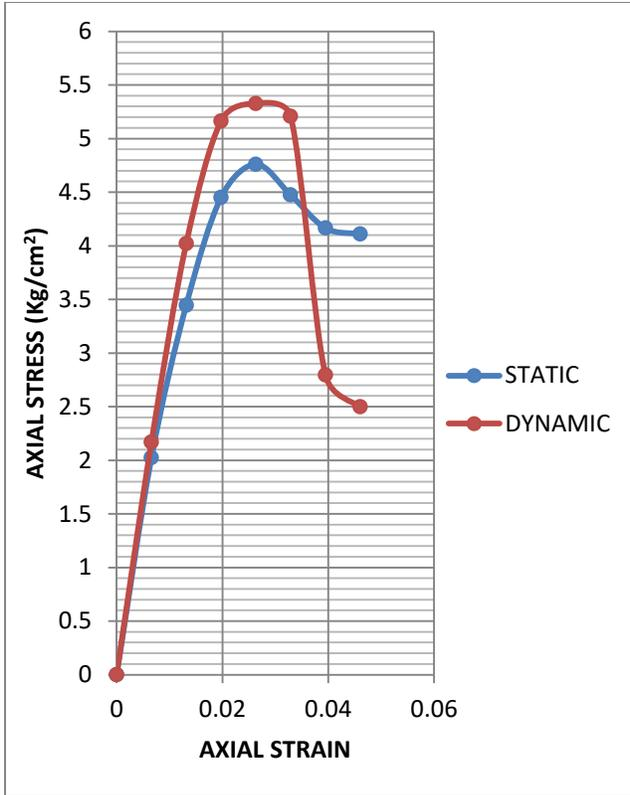
**Fig. 4.31: Superimposed curves of UCS test on statically and dynamically compacted soil- sample 5 at OMC-3%**
