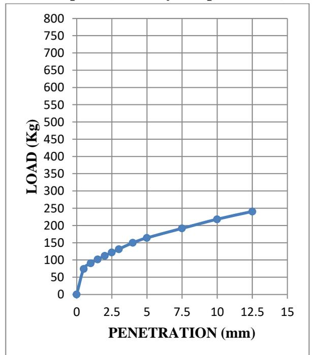
**Fig. 3.28: Load-penetration curve at OMC+5% of sample 2 (statically compacted soil)**
