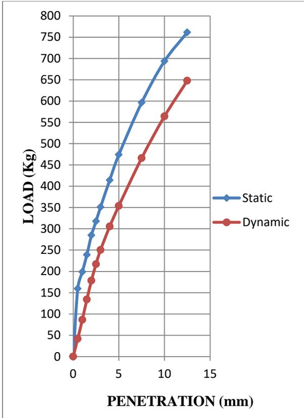
**Fig. 4.4: Superimposed curves of CBR test on statically and dynamically compacted soil- sample 2 at OMC-5%**
