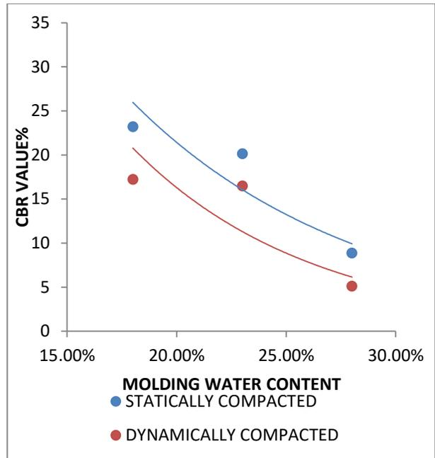
**Fig. 4.38: Superimposed curves of CBR values vs. molding water contents of statically and dynamically compacted soil for sample 2**
