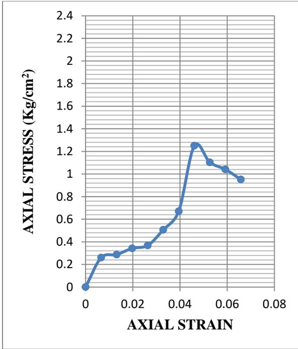
**Fig.3.61: Stress-strain graph of UCS test for sample 2 at OMC (Statically Compacted)**
