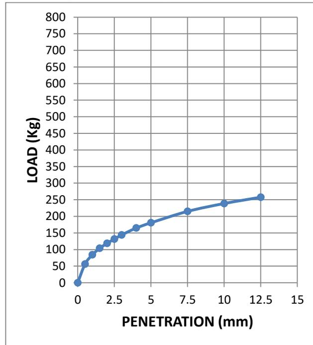
**Fig. 3.40: Load-penetration curve at OMC+3% of sample 4 (statically compacted soil)**
