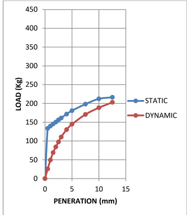
**Fig. 4.17: Superimposed curves of CBR test on statically and dynamically compacted soil- sample 6 at OMC**
