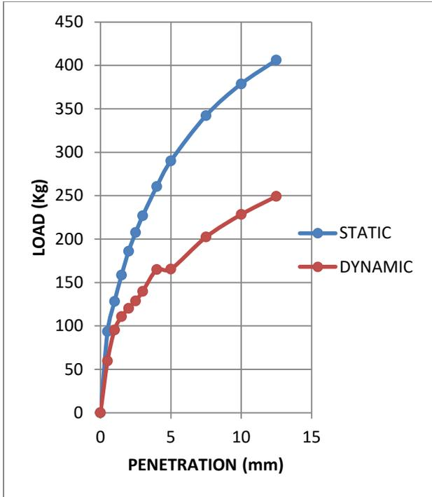
**Fig. 4.16: Superimposed curves of CBR test on statically and dynamically compacted soil-sample 6 at OMC-3%**
