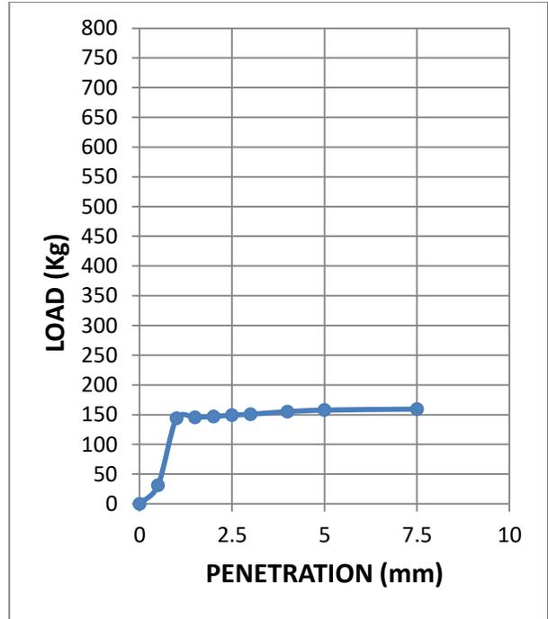
**Fig. 3.34: Load-penetration curve at OMC+3% of sample 3 (statically compacted soil)**
