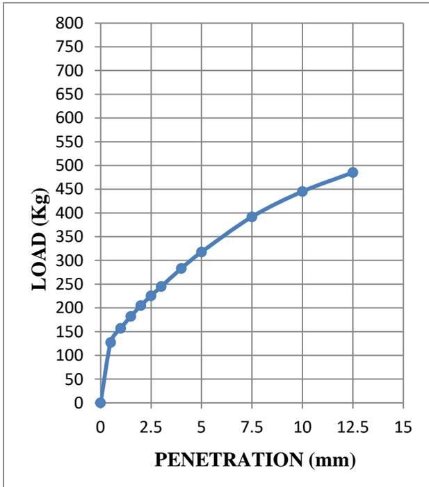
**Fig. 3.25: Load-penetration curve soil at OMC of sample 2 (dynamically compacted)**
