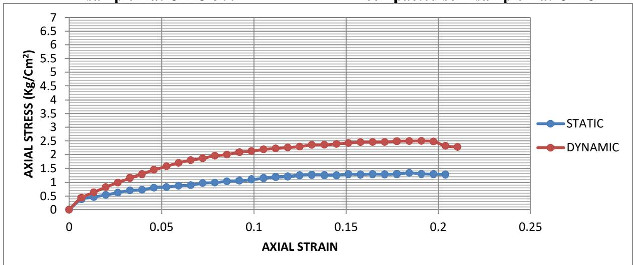
**Fig. 4.21: Superimposed curves of UCS test on statically and dynamically compacted soil-sample 1 at OMC+3%**
