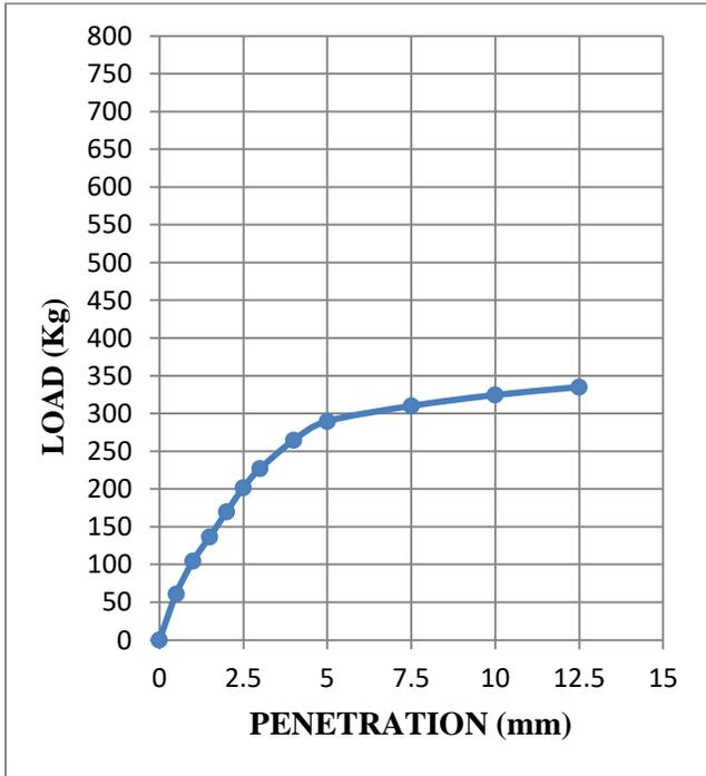
**Fig. 3.31: Load-penetration curve at OMC of sample 3 (dynamically compacted soil)**
