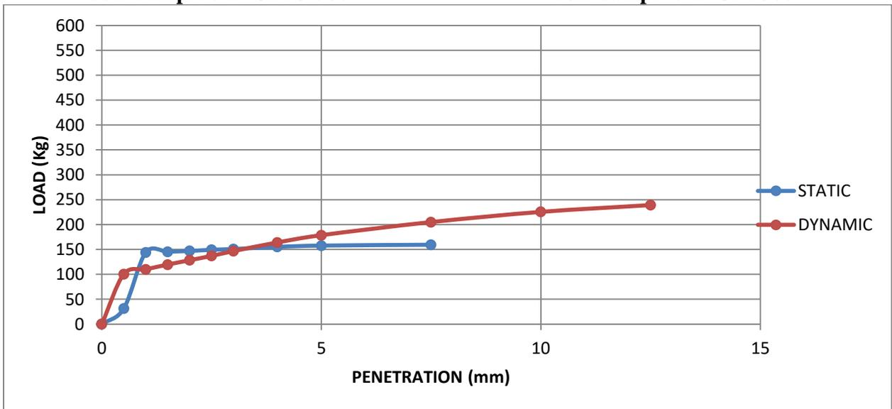
**Fig. 4.9: Superimposed curves of CBR test on statically and dynamically compacted soil- sample 3 at OMC+3%**
