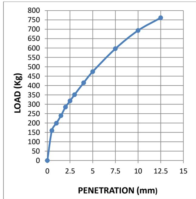
**Fig. 3.24: Load-penetration curve at OMC-5% of sample2 (statically compacted soil)**
