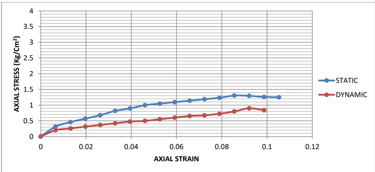
**Fig. 4.27: Superimposed curves of UCS test on statically and dynamically compacted soil- sample 3 at OMC+3%**
