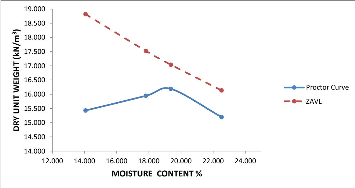
**Fig.3.15. Dynamic compaction curve for sample 5**
