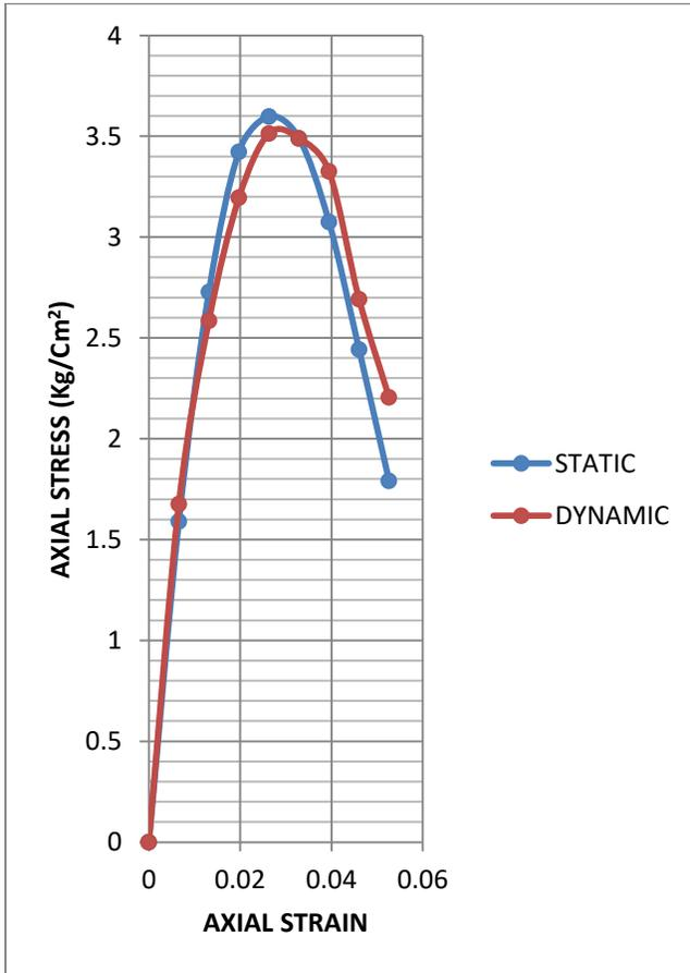
**Fig. 4.25: Superimposed curves of UCS test on statically and dynamically compacted soil- sample 3 at OMC-3%**
