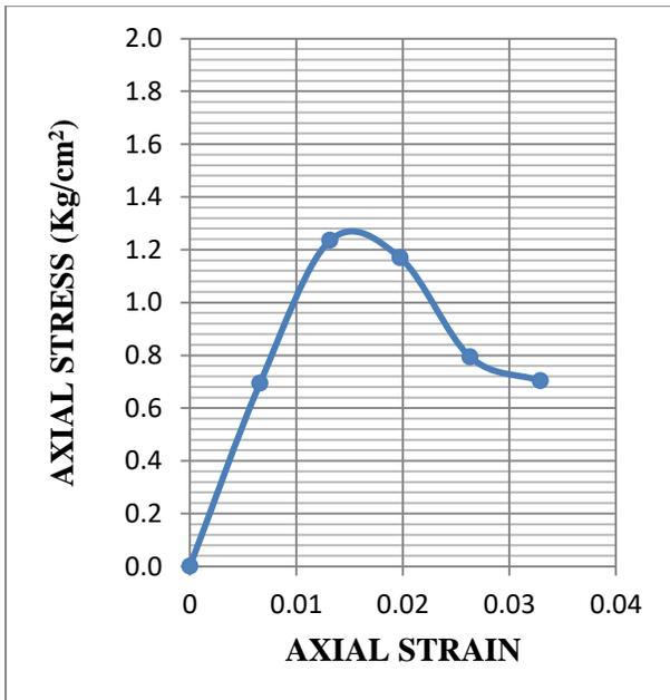
**Fig.3.59: Stress-strain graph of UCS test for sample 2 at OMC-5% (Statically Compacted)**
