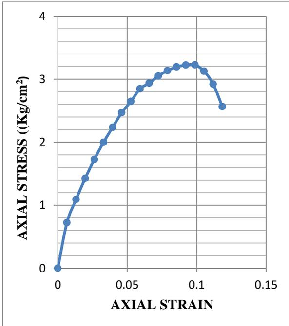
**Fig.3.75: Stress-strain graph of UCS test for sample 4 at OMC+3% (Statically Compacted)**
