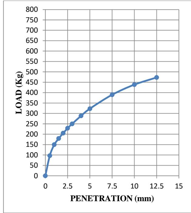
**Fig. 3.38: Load-penetration curve at OMC of sample 4 (Statically compacted soil)**
