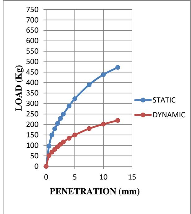
**Fig. 4.11: Superimposed curves of CBR test on statically and dynamically compacted soil- sample 4 at OMC**
