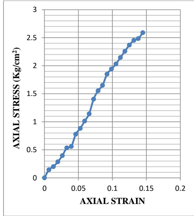
**Fig.3.82: Stress-strain graph of UCS test for sample 5 at OMC+3% (Dynamically Compacted)**
