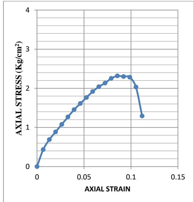
**Fig.3.76: Stress-strain graph of UCS test for sample 4 at OMC+3% (Dynamically Compacted)**
