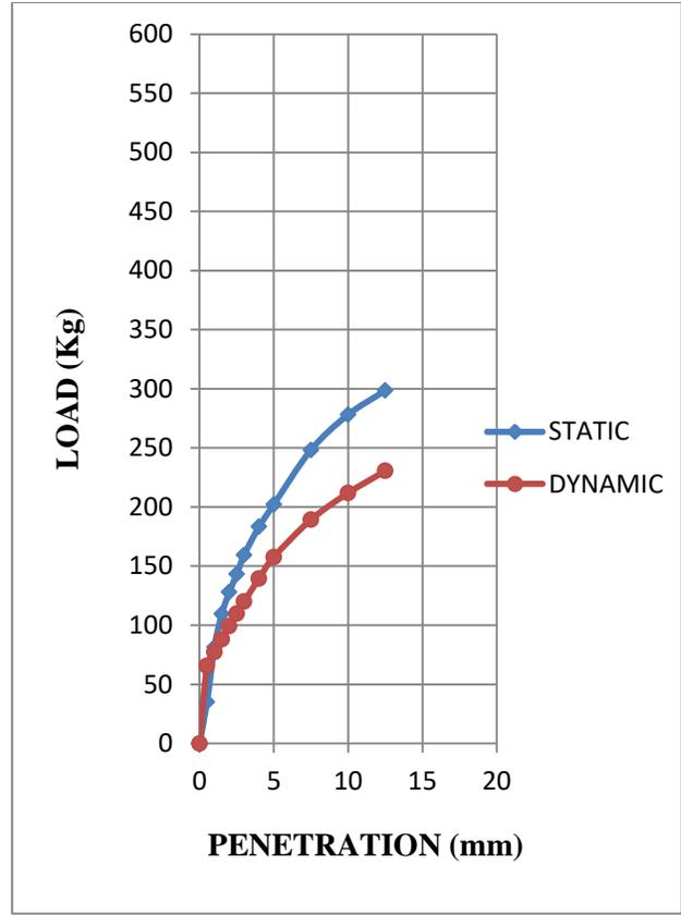
**Fig. 4.2: Superimposed curves of CBR test on statically and dynamically compacted soil- sample 1 at OMC**
