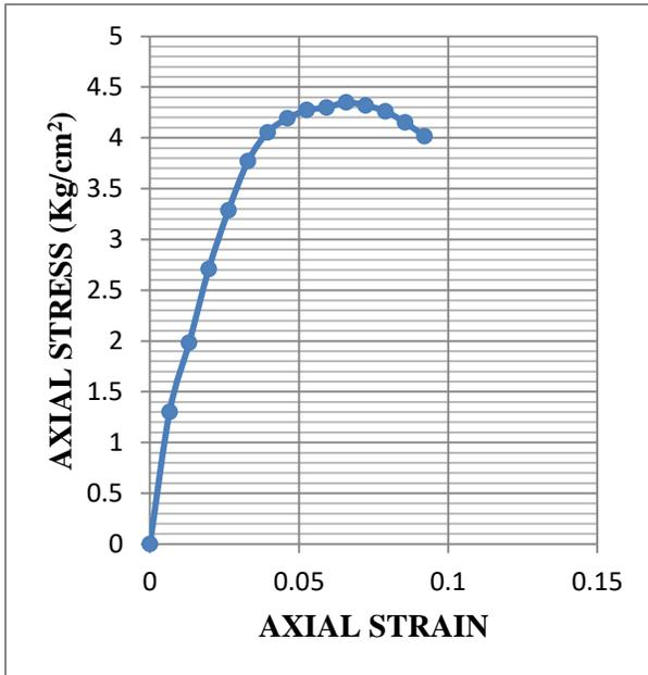
**Fig.3.83: Stress-strain graph of UCS test for sample 6 at OMC-3% (Statically Compacted)**
