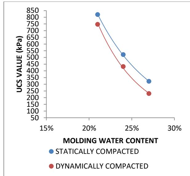
**Fig. 4.46: Superimposed curves of UCS values vs. molding water contents of statically and dynamically compacted soil for sample 4**
