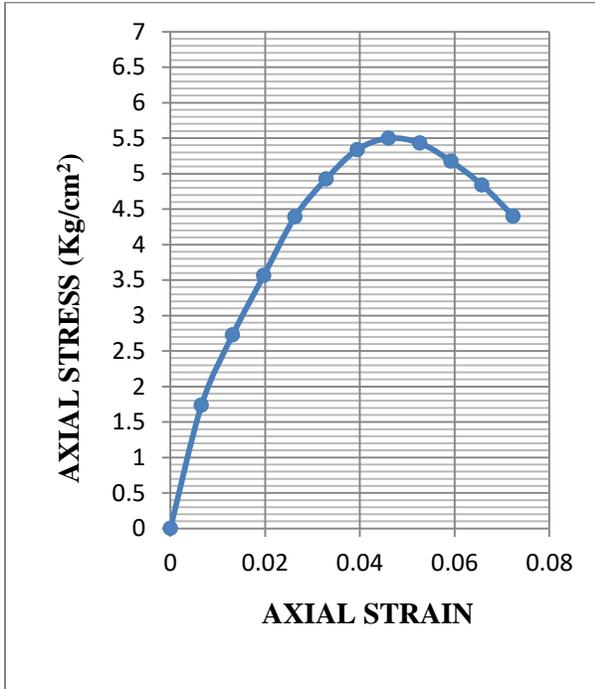
**Fig.3.53: Stress-strain graph of UCS test for sample 1 at OMC-3% (Statically Compacted)**
