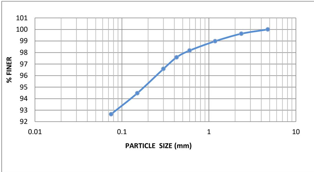
**Fig. 3.5: Gradation curve for sample 1**
