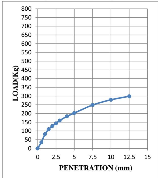
**Fig.3.20: Load-penetration curve at OMC of sample1 (statically compacted soil)**
