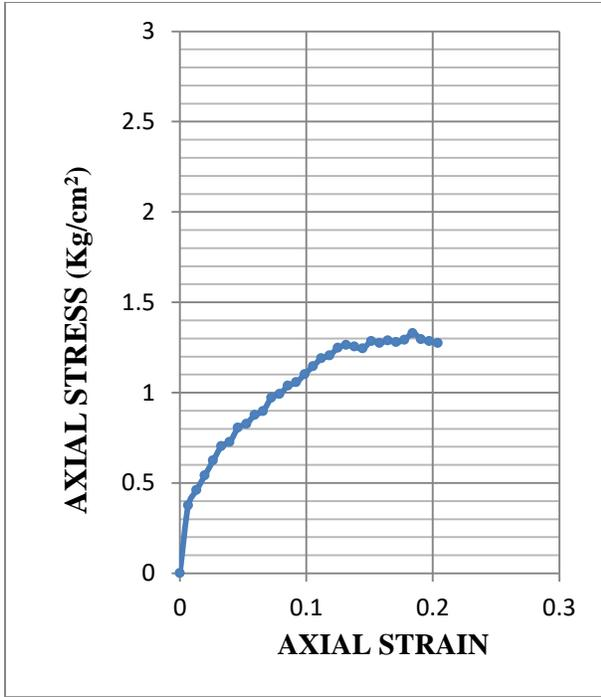
**Fig.3.57: Stress-strain graph of UCS test for sample 1 at OMC+3% (Statically Compacted)**
