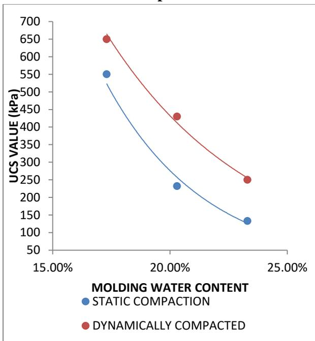
**Fig. 4.43: Superimposed curves of UCS values vs. molding water contents of statically and dynamically compacted soil for sample 1**
