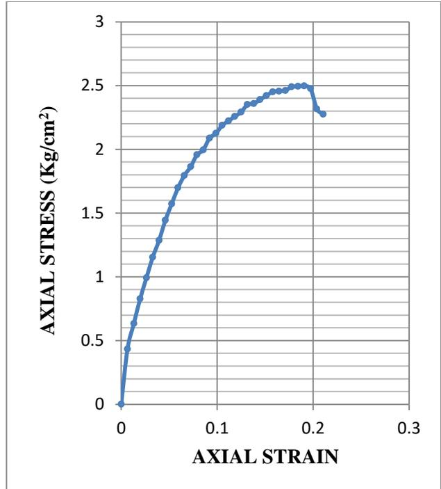
**Fig.3.58: Stress-strain graph of UCS test for sample 1 at OMC+3% (Dynamically Compacted)**
