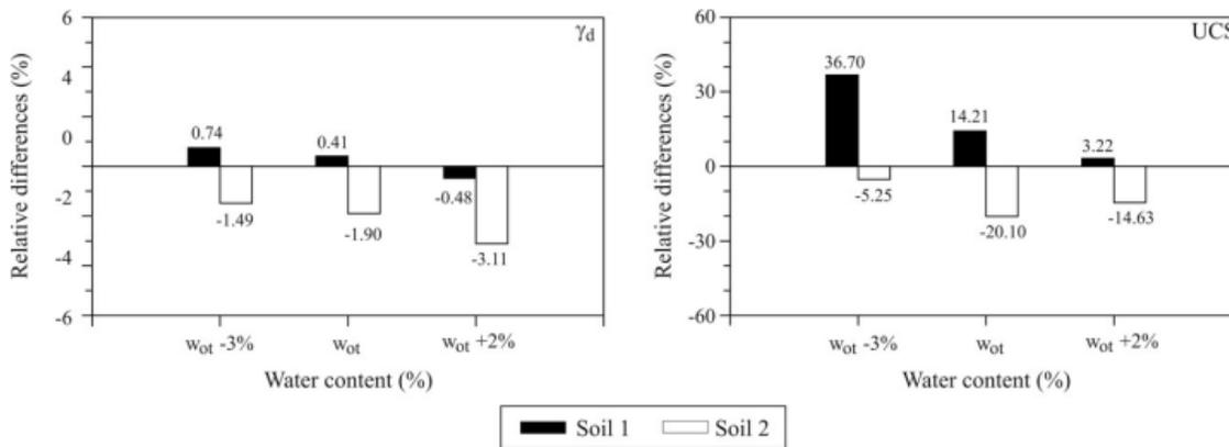
**Fig. 2.4: Relative differences between mean values of the parameters  $\gamma_d$  and UCS of soils 1 and 2, adopting the dynamic compaction data as reference (Dario et al. 2010)**
