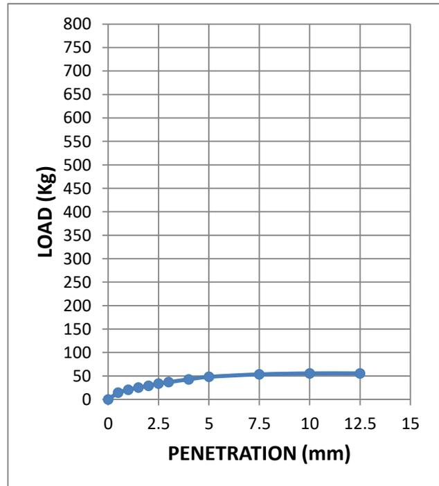
**Fig. 3.52: Load-penetration curve at OMC+3% of sample 6 (statically compacted soil)**
