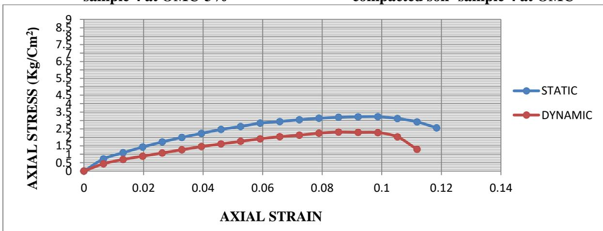
**Fig. 4.30: Superimposed curves of UCS test on statically and dynamically compacted soil- sample 4 at OMC+3%**
