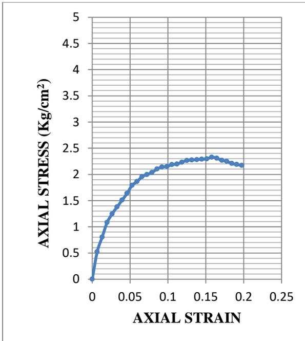
**Fig.3.55: Stress-strain graph of UCS test for sample 1 at OMC (Statically Compacted)**
