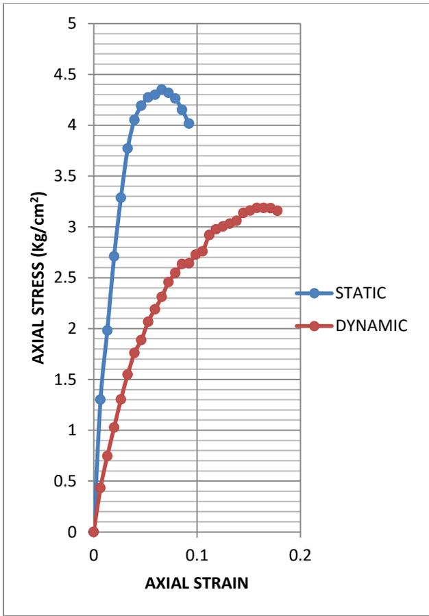
**Fig. 4.34: Superimposed curves of UCS test on statically and dynamically compacted soil- sample 6 at OMC-3%**
