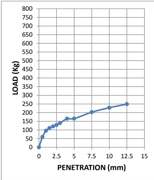
**Fig. 3.47: Load-penetration curve at OMC-3% of sample 6 (dynamically compacted soil)**
