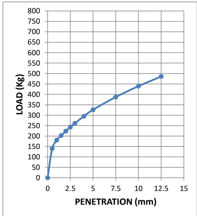
**Fig. 3.44: Load-penetration curve at OMC of sample 5 (statically compacted soil)**
