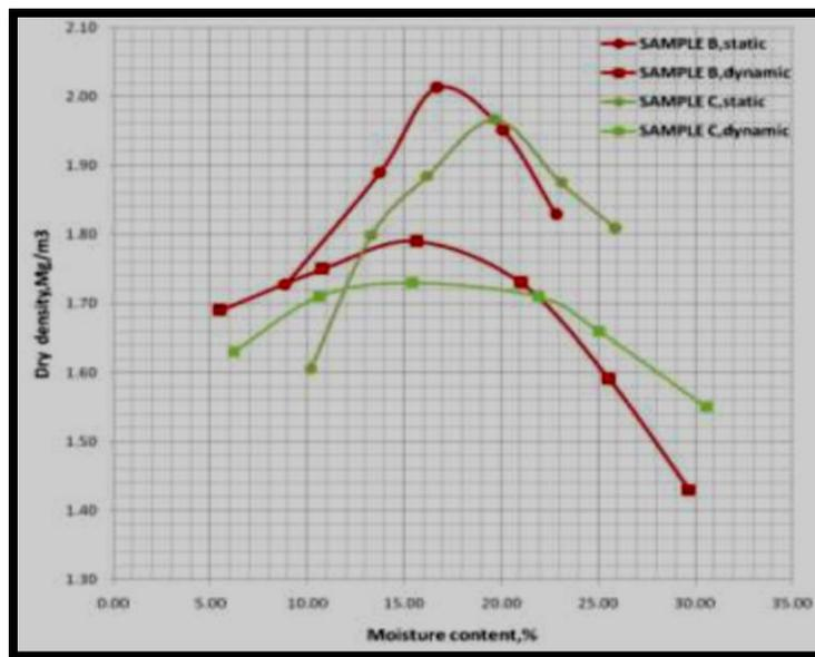
**Fig. 2.2: Comparison between static compaction method and the dynamic compaction method by Hafez et.al (2010)**
