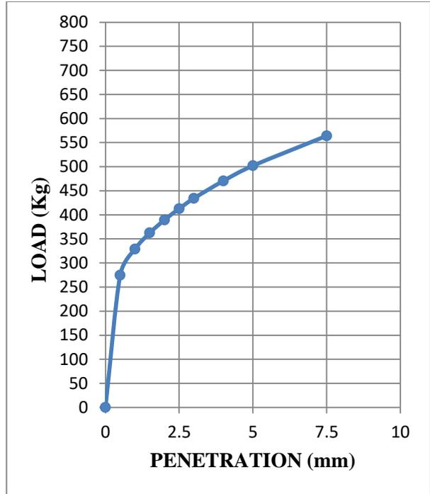
**Fig. 3.30: Load-penetration curve at OMC-3% of sample 3 (statically compacted soil)**
