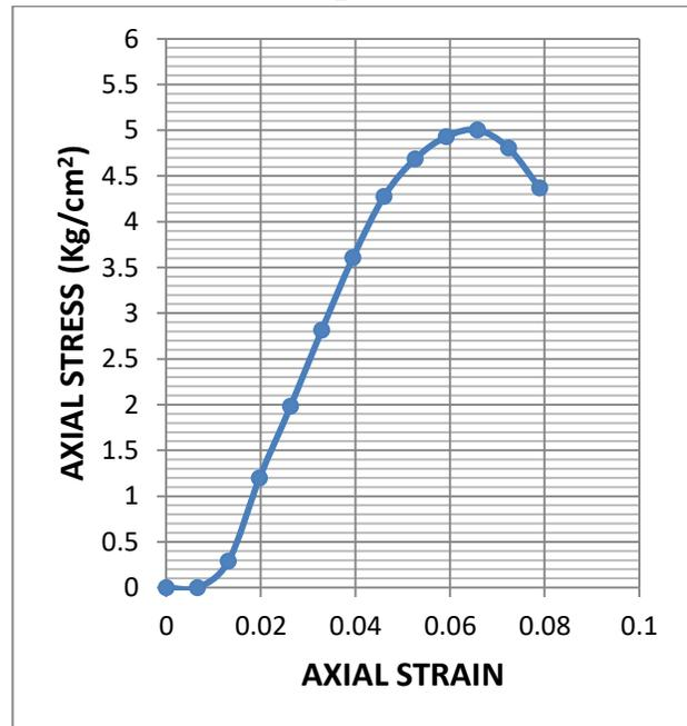
**Fig.3.80: Stress-strain graph of UCS test for sample 5 at OMC (Dynamically Compacted)**
