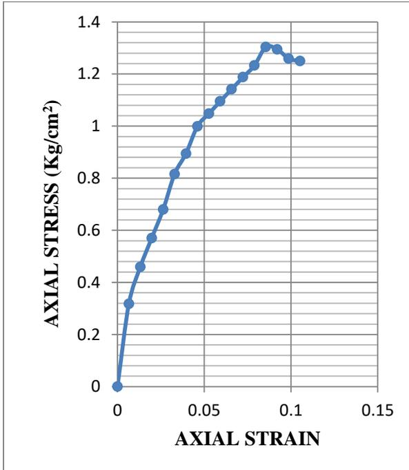
**Fig.3.69: Stress-strain graph of UCS test for sample 3 at OMC+3% (Statically Compacted)**
