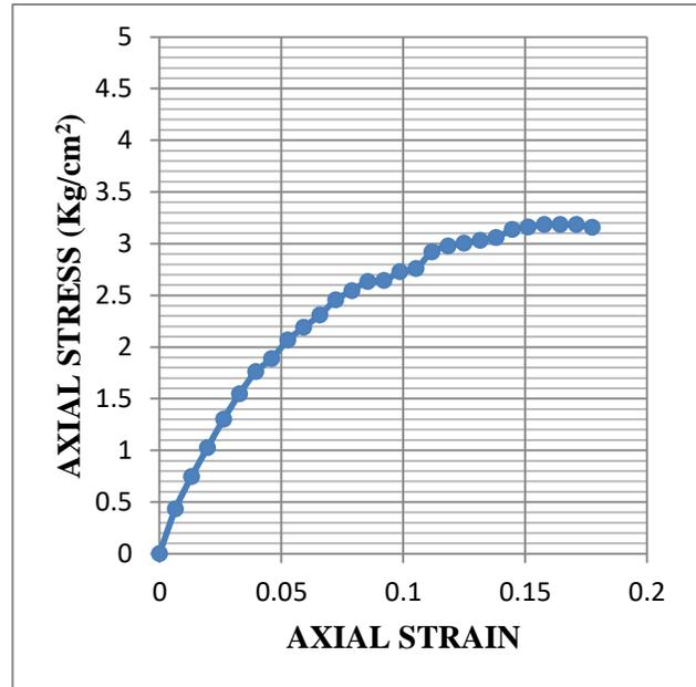
**Fig.3.84: Stress-strain graph of UCS test for sample 6 at OMC-3% (Dynamically Compacted)**
