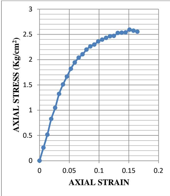
**Fig.3.85: Stress-strain graph of UCS test for sample 6 at OMC (Statically Compacted)**
