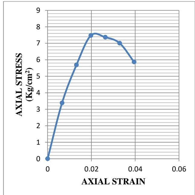
**Fig.3.72: Stress-strain graph of UCS test for sample 4 at OMC-3% (Dynamically Compacted)**
