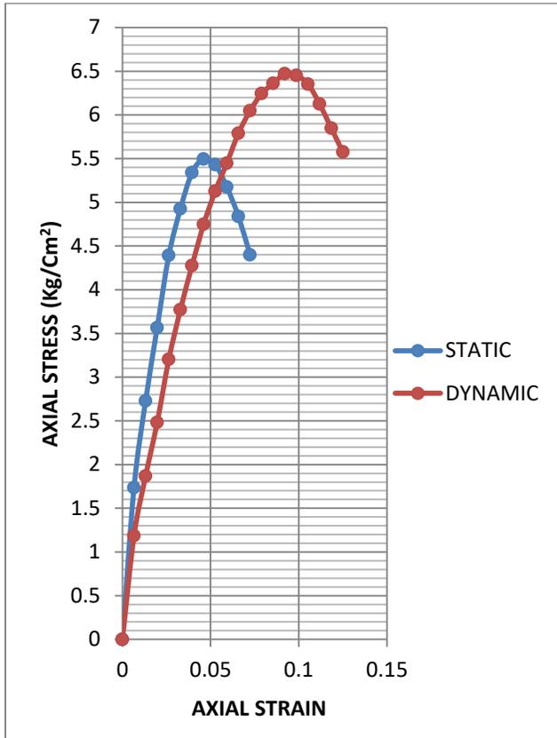
**Fig. 4.19: Superimposed curves of UCS test on statically and dynamically compacted soil-sample 1 at OMC-3%**
