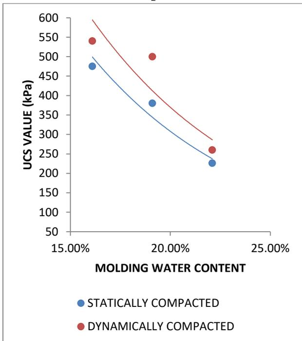
**Fig. 4.47: Superimposed curves of UCS values vs. molding water contents of statically and dynamically compacted soil for sample 5**
