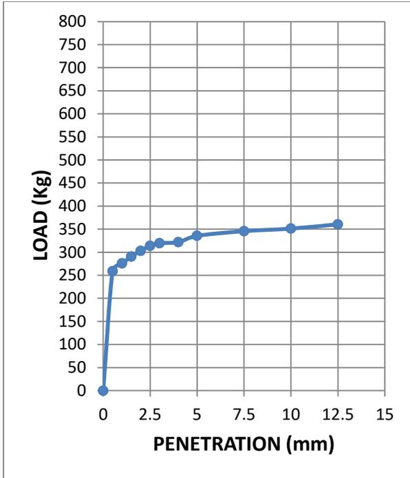
**Fig. 3.41: Load-penetration curve at OMC-3% of sample 5 (dynamically compacted soil)**
