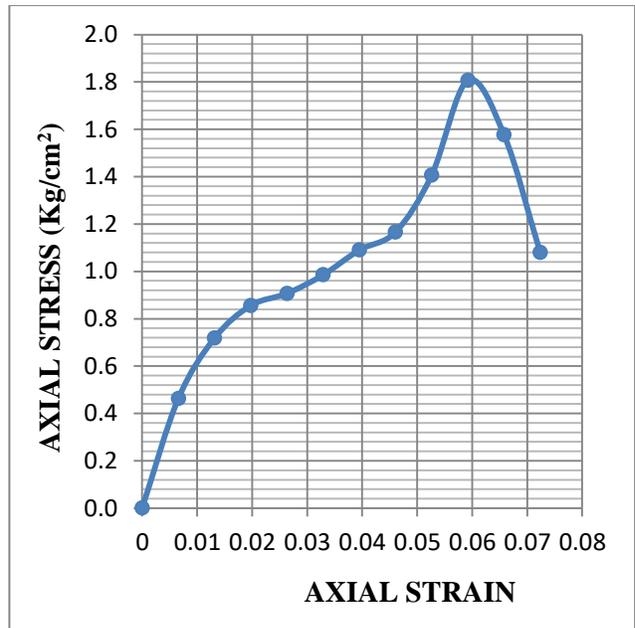
**Fig.3.60: Stress-strain graph of UCS test for sample 2 at OMC-5% (Dynamically Compacted)**
