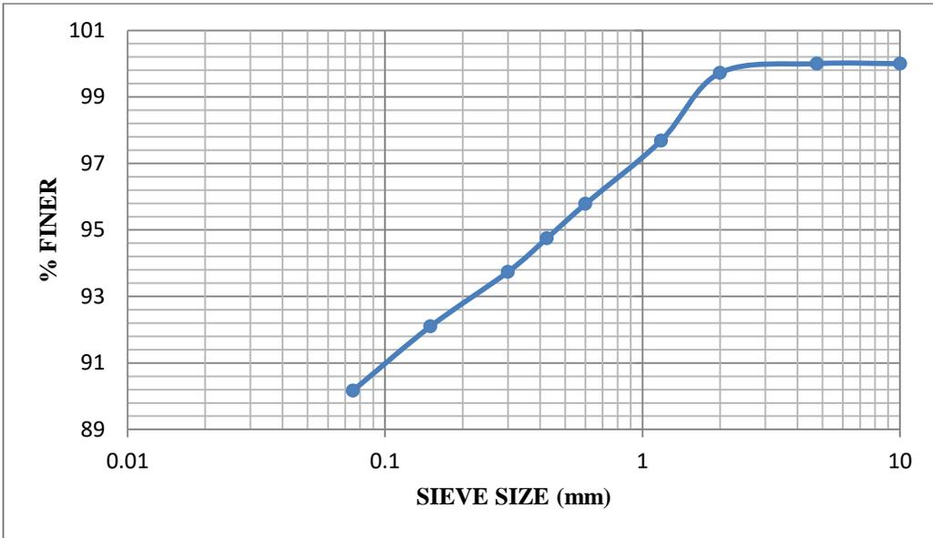
**Fig. 3.8: Gradation curve for sample 4**
