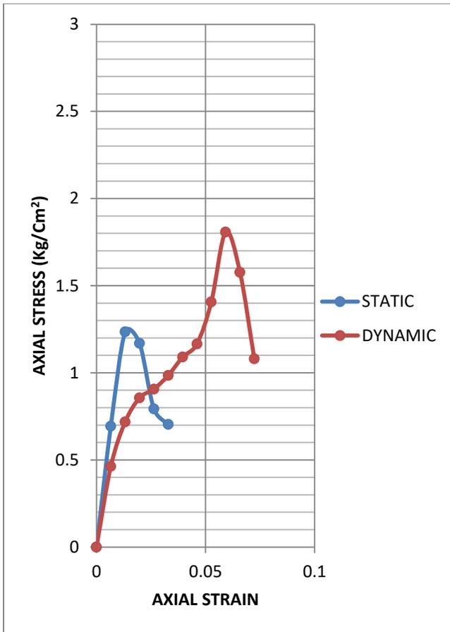
**Fig. 4.22: Superimposed curves of UCS test on statically and dynamically compacted soil- sample 2 at OMC-5%**
