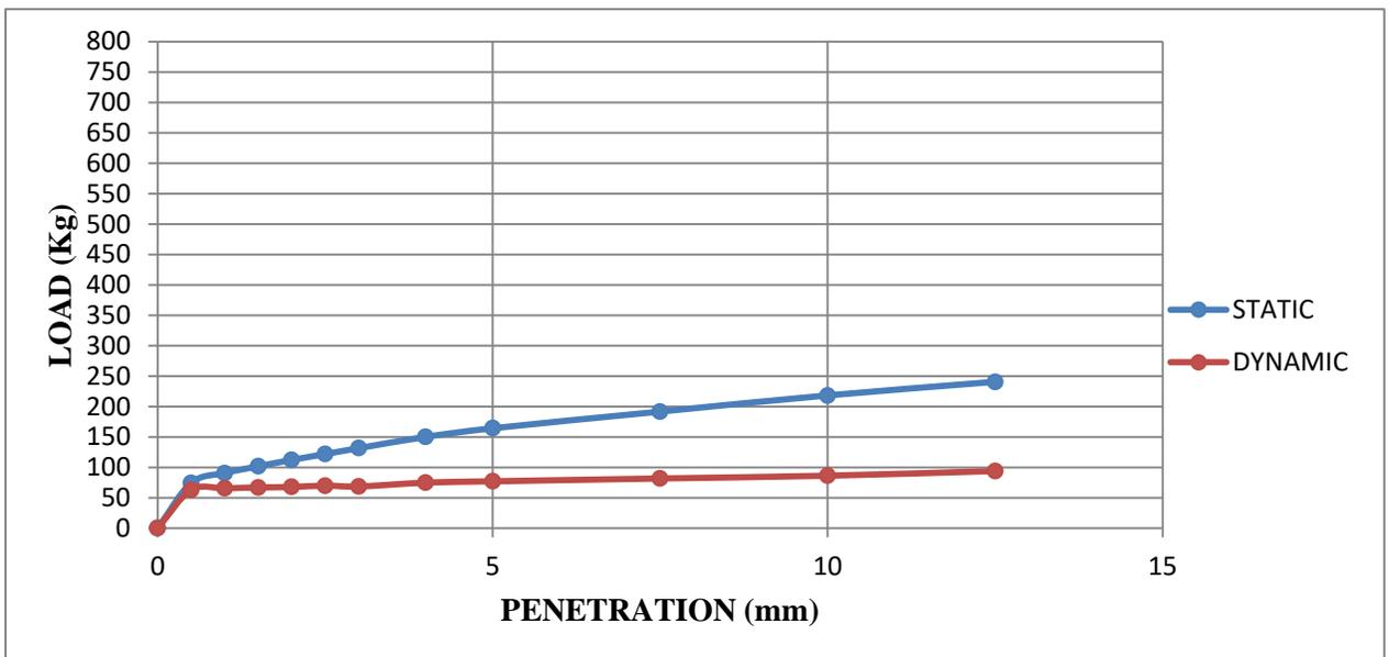
**Fig. 4.6: Superimposed curves of CBR test on statically and dynamically compacted soil- sample 2 at OMC+5%**
