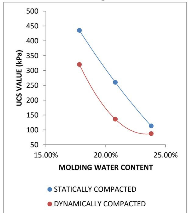
**Fig. 4.48: Superimposed curves of UCS values vs. molding water contents of statically and dynamically compacted soil for sample 6**
