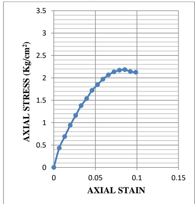
**Fig.3.68: Stress-strain graph of UCS test for sample 3 at OMC (Dynamically Compacted)**
