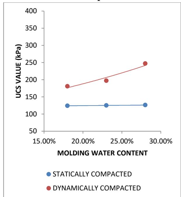
**Fig. 4.44: Superimposed curves of UCS values vs. molding water contents of statically and dynamically compacted soil for sample 2**
