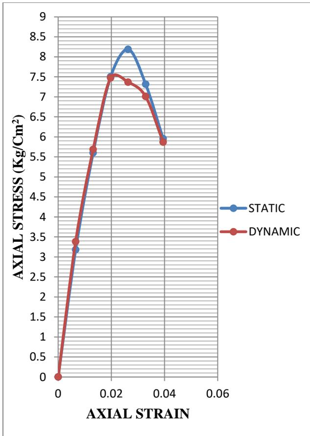
**Fig. 4.28: Superimposed curves of UCS test on statically and dynamically compacted soil-sample 4 at OMC-3%**
