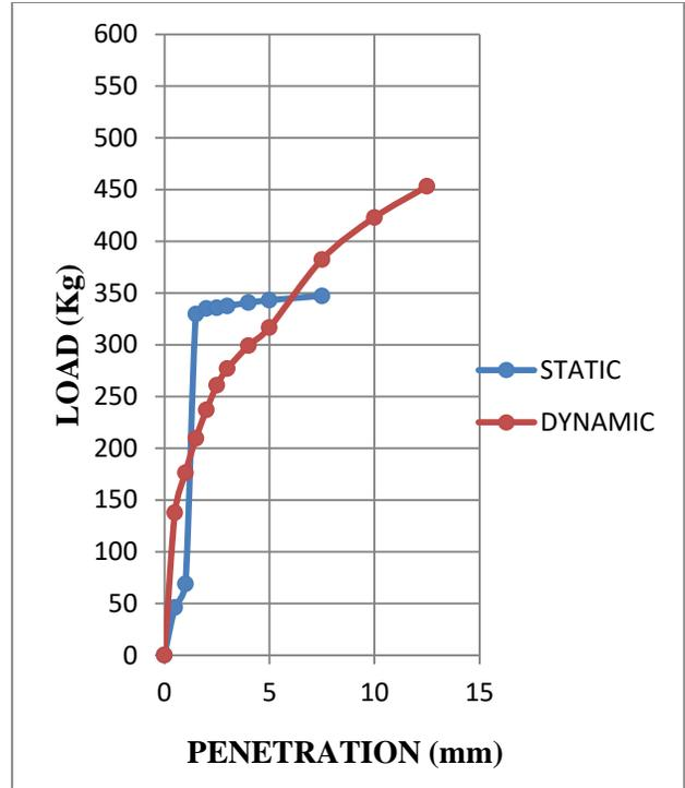
**Fig. 4.8: Superimposed curves of CBR test on statically and dynamically compacted soil- sample 3 at OMC%**
