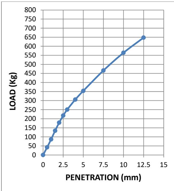
**Fig. 3.23: Load-penetration curve at OMC-5% of sample 2 (dynamically compacted soil)**
