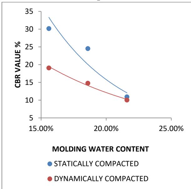
**Fig. 4.39: Superimposed curves of CBR values vs. molding water contents of statically and dynamically compacted soil for sample 3**
