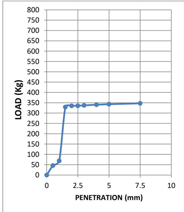
**Fig. 3.32: Load-penetration curve at OMC of sample 3 (statically compacted soil)**
