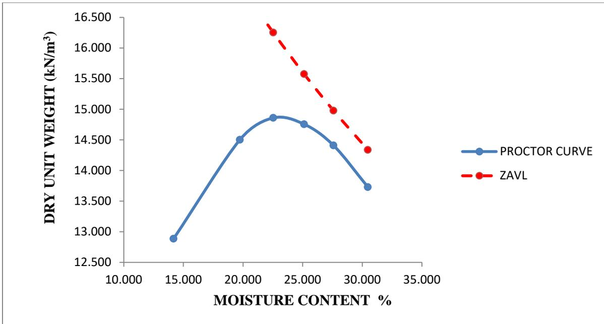
**Fig.3.12. Dynamic compaction curve for sample 2**
