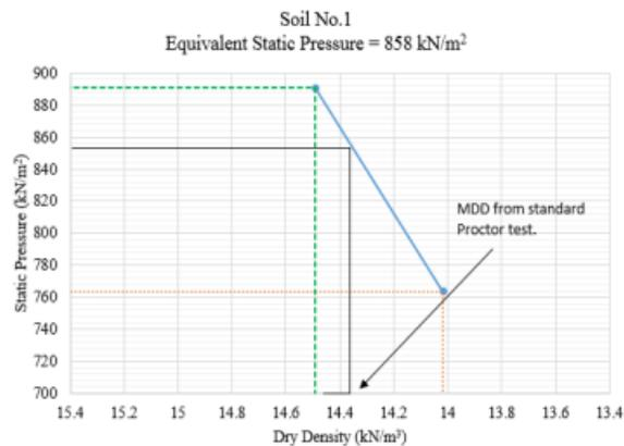
**Fig. 2.11: Determination of equivalent static pressure for soil no.1 (B.Sharma et.al,2014)**
