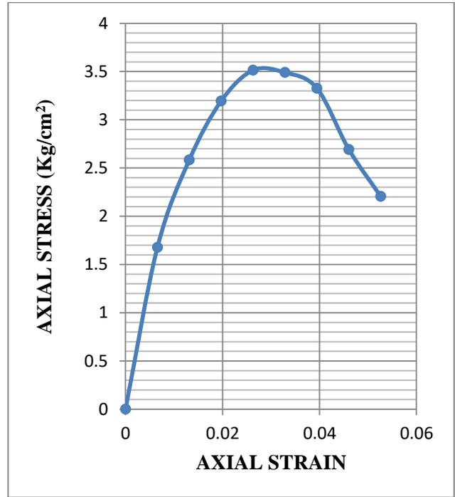
**Fig.3.66: Stress-strain graph of UCS test for sample 3 at OMC-3% (Dynamically Compacted)**
