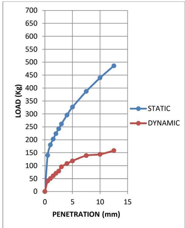
**Fig. 4.14: Superimposed curves of CBR test on statically and dynamically compacted soil- sample 5 at OMC**
