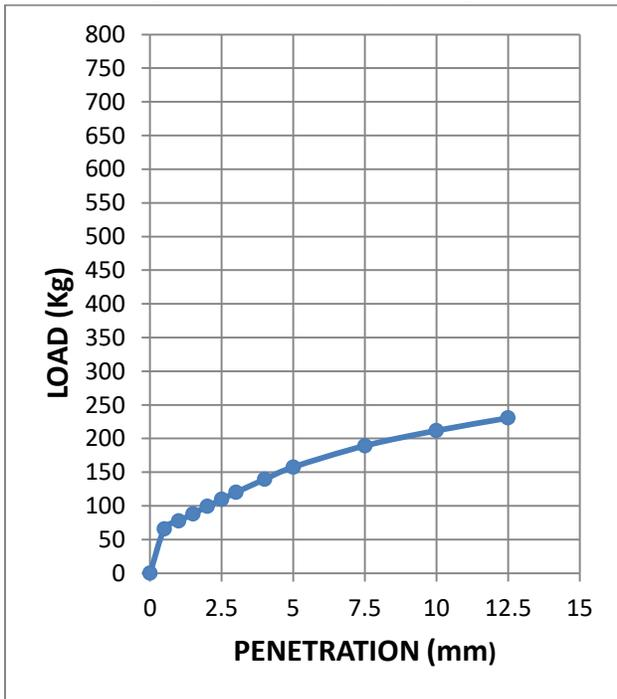
**Fig.3.19: Load-penetration curve at OMC of sample 1 (dynamically compacted soil)**
