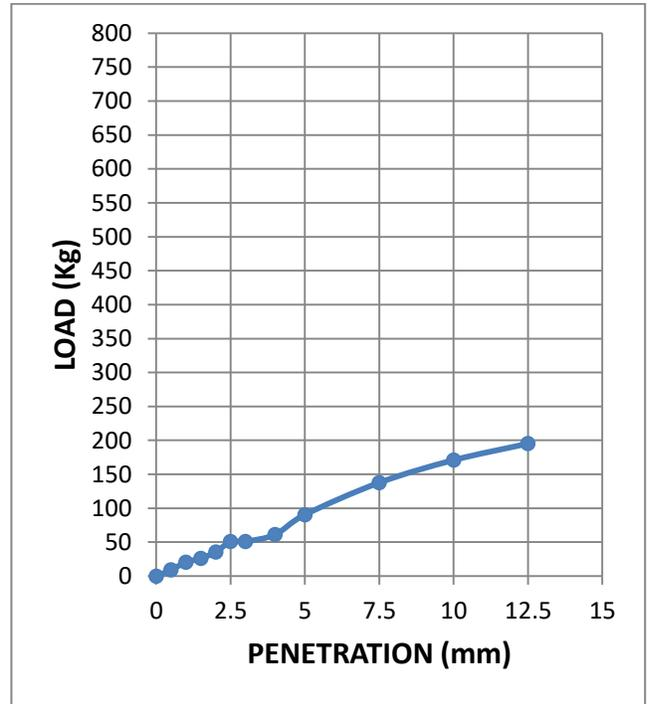
**Fig. 3.46: Load-penetration curve at OMC+3% of sample 5 (statically compacted soil)**
