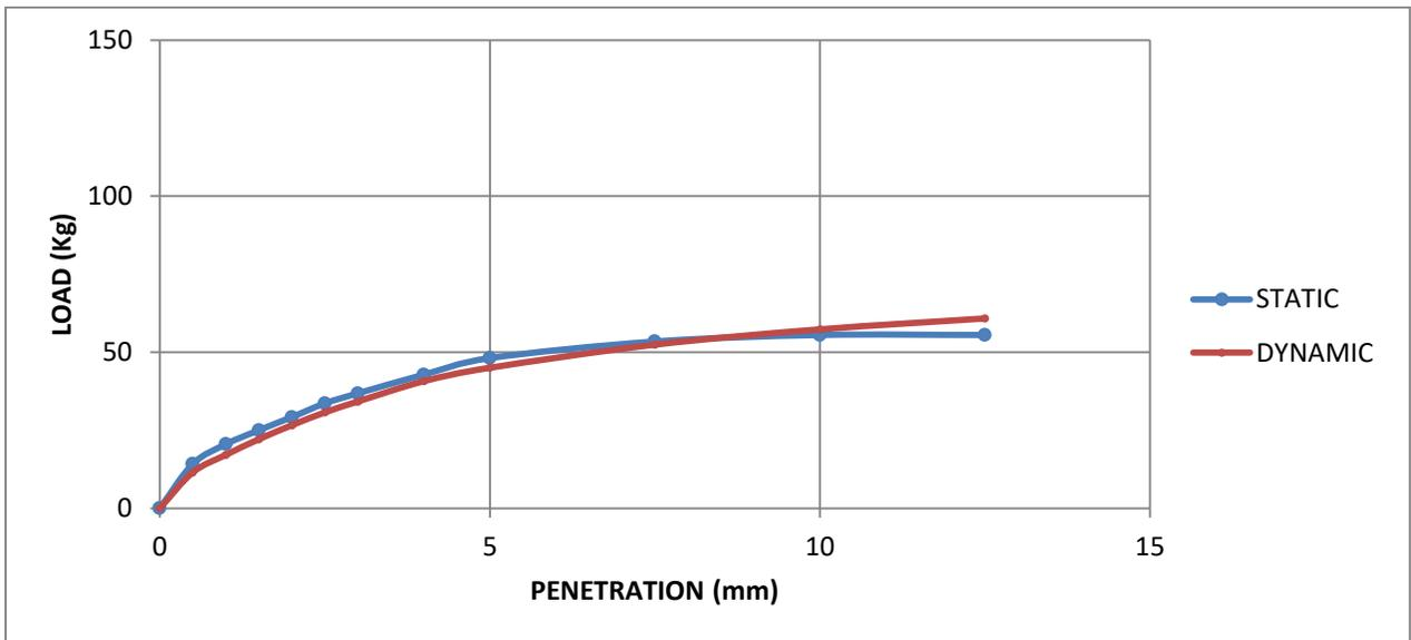
**Fig. 4.18: Superimposed curves of CBR test on statically and dynamically compacted soil-sample 6 at OMC+3%**
