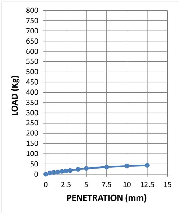
**Fig 3.21: Load-penetration curve at OMC+3% of sample1 (dynamically compacted soil)**
