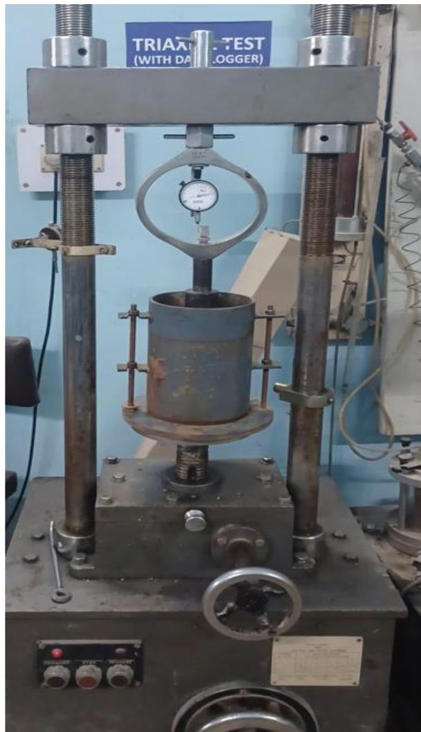
**Fig.3.2: Static Compaction Set Up**
