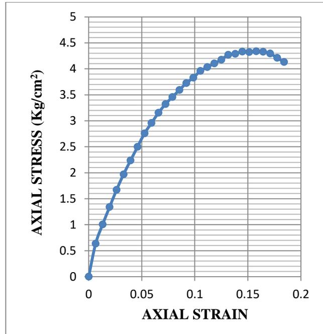
**Fig.3.56: Stress-strain graph of UCS test for sample 1 at OMC (Dynamically Compacted)**
