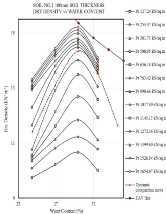
**Fig. 2.10: Dry density vs moisture content curve for soil no.1 (B.Sharma et.al,2014)**
