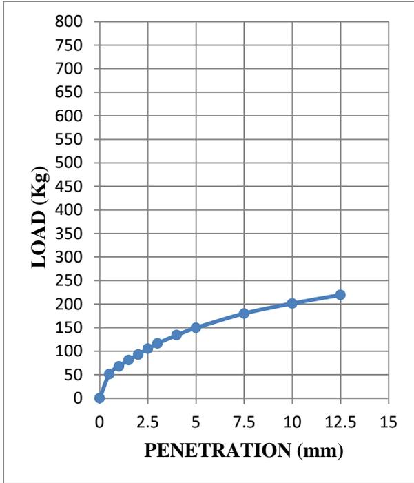
**Fig. 3.37: Load-penetration curve at OMC of sample 4 (Dynamically compacted soil)**
