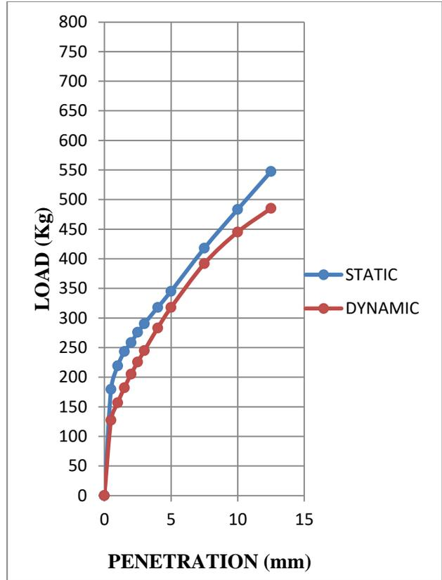
**Fig. 4.5: Superimposed curves of CBR test on statically and dynamically compacted soil- sample 2 at OMC**
