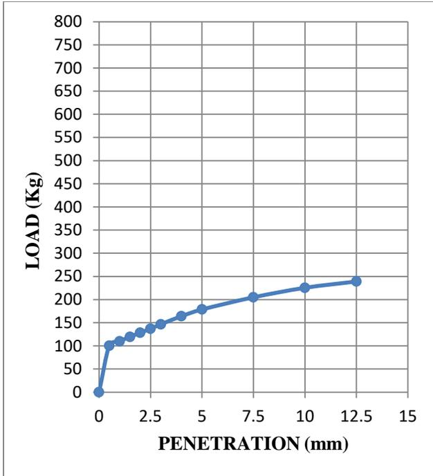
**Fig. 3.33: Load-penetration curve at OMC+3% of sample 3 (dynamically compacted soil)**
