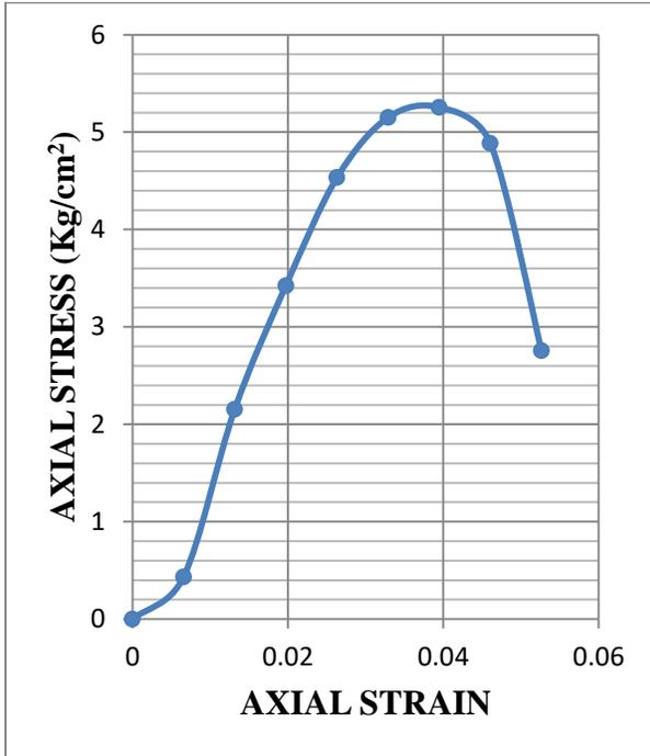
**Fig.3.73: Stress-strain graph of UCS test for sample 4 at OMC (Statically Compacted)**
