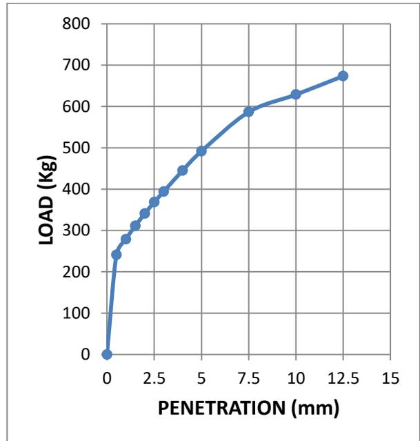
**Fig. 3.36: Load-penetration curve at OMC-3% of sample 4 (Statically compacted soil)**
