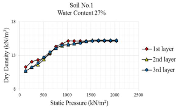
**Fig. 2.7: Dry density vs static pressure for soil no.1 at 27% water content (B.Sharma et.al,2014)**
