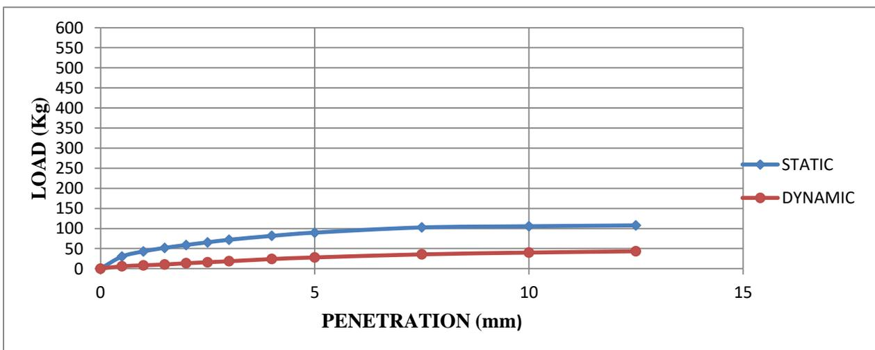
**Fig. 4.3: Superimposed curves of CBR test on statically and dynamically compacted soil- sample 1 at OMC+3%**
