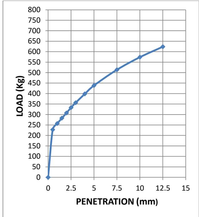
**Fig. 3.42: Load-penetration curve at OMC-3% of sample 5 (statically compacted soil)**
