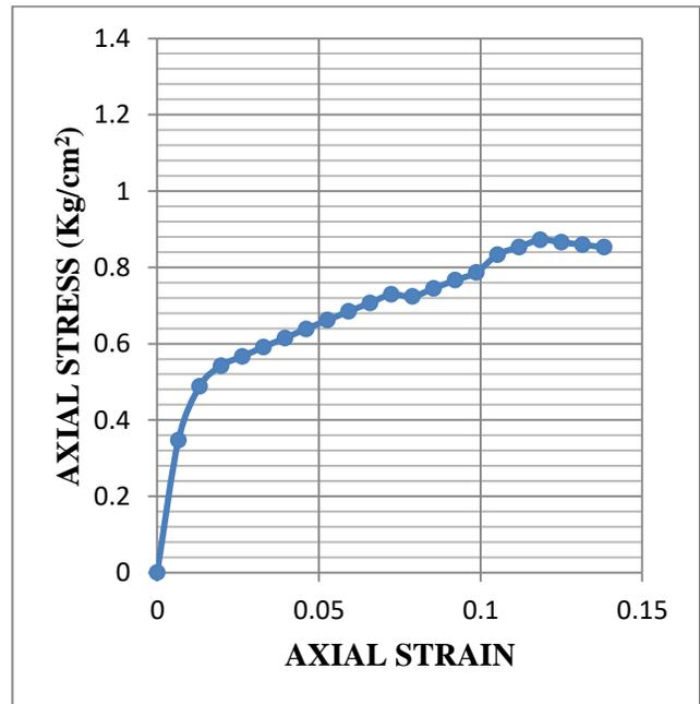
**Fig.3.88: Stress-strain graph of UCS test for sample 6 at OMC+3% (Dynamically Compacted)**
