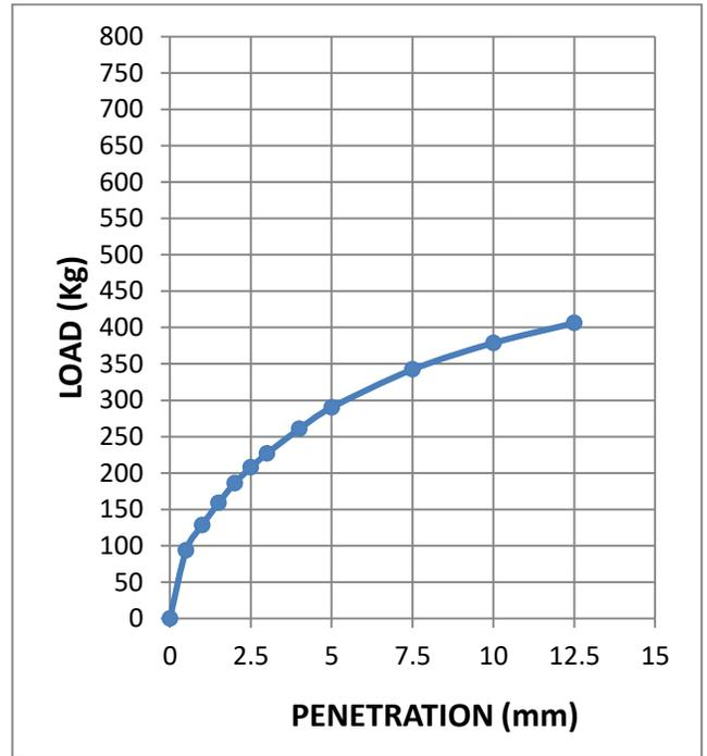
**Fig. 3.48: Load-penetration curve at OMC-3% of sample 6 (statically compacted soil)**
