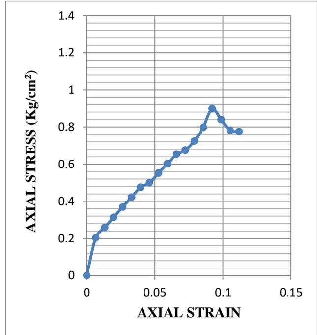
**Fig.3.70: Stress-strain graph of UCS test for sample 3 at OMC+3% (Dynamically Compacted)**
