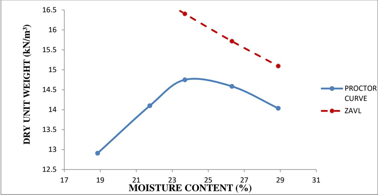
**Fig.3.14. Dynamic compaction curve for sample 4**
