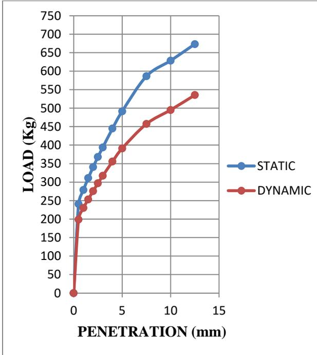
**Fig. 4.10: Superimposed curves of CBR test on statically and dynamically compacted soil- sample 4 at OMC-3%**
