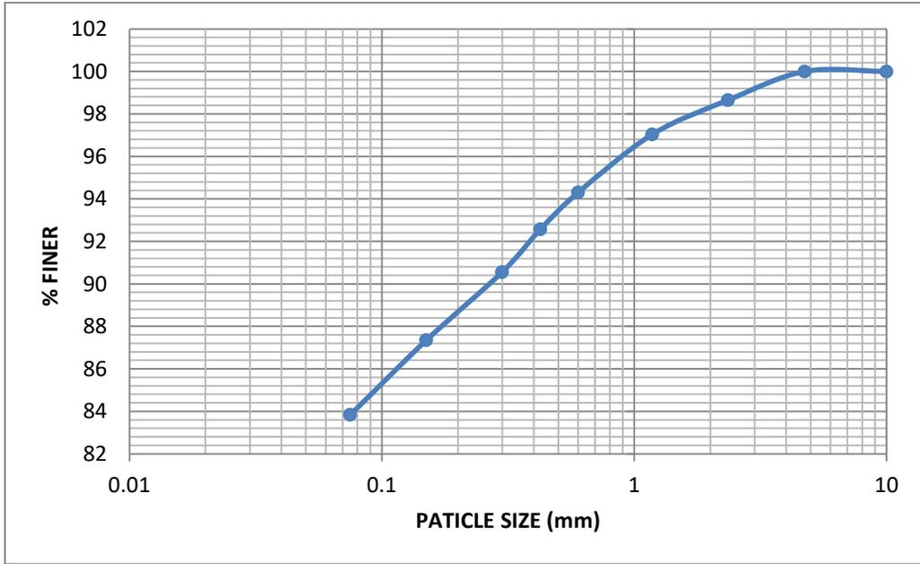
**Fig. 3.7: Gradation curve for sample 3**
