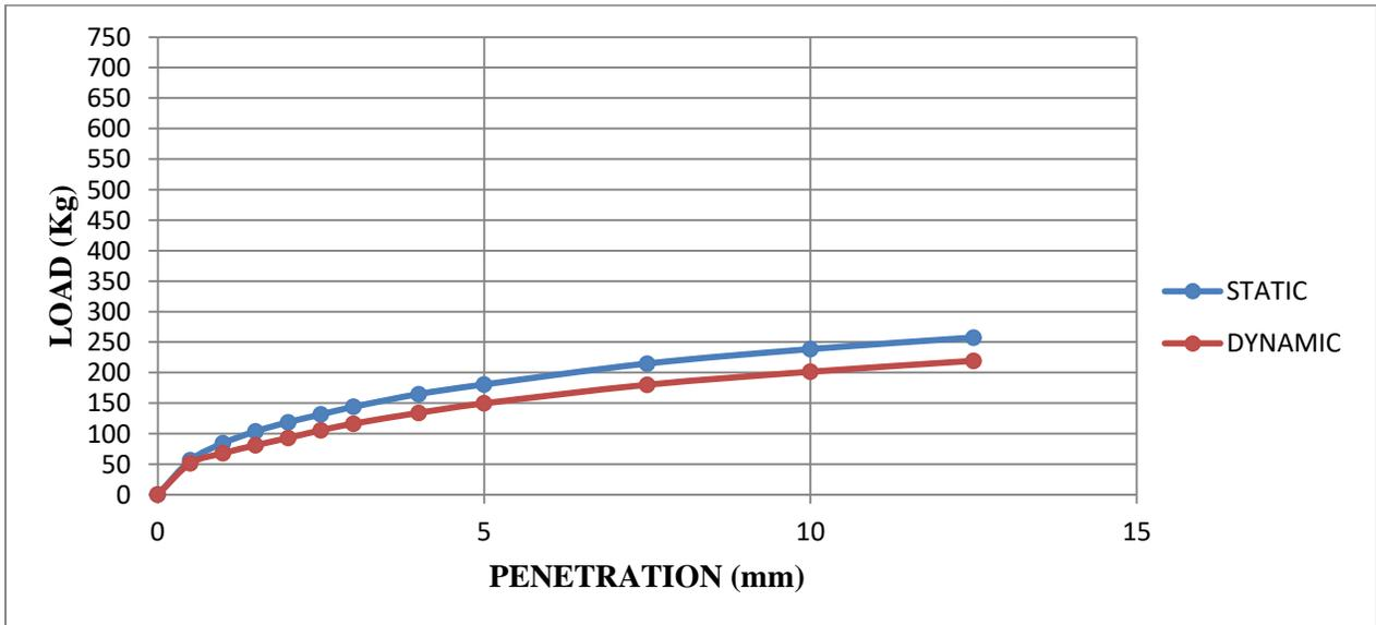
**Fig. 4.12: Superimposed curves of CBR test on statically and dynamically compacted soil- sample 4 at OMC+3%**
