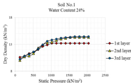
**Fig. 2.6: Dry density vs static pressure for soil no.1 at 24% water content (B.Sharma et.al,2014)**
