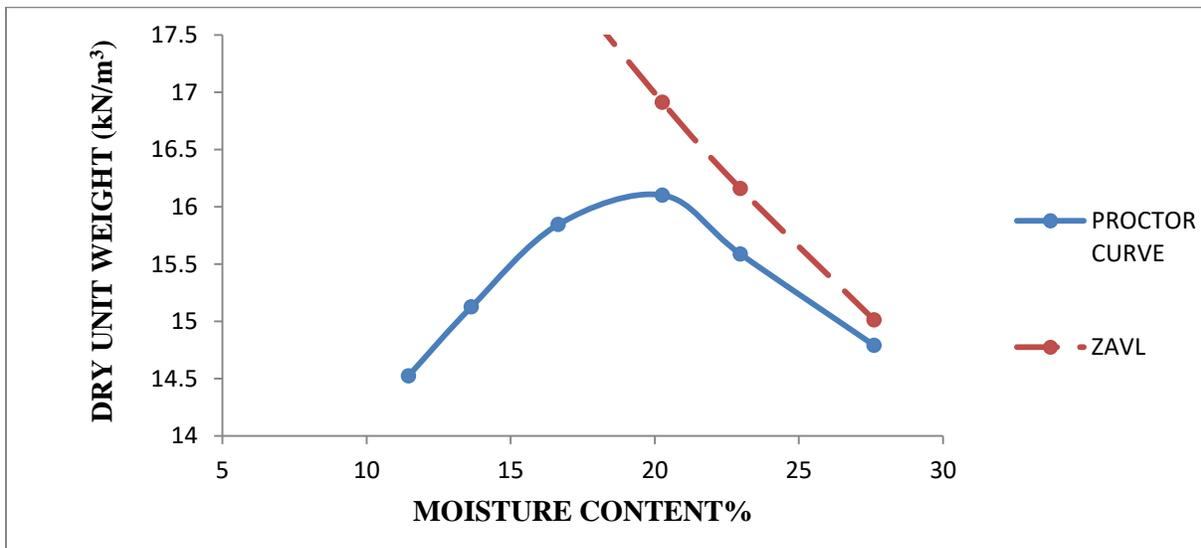
**Fig.3.11. Dynamic compaction curve for sample 1**
