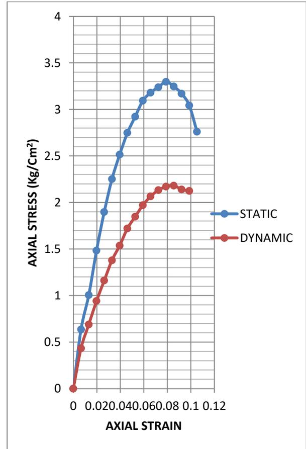
**Fig. 4.26: Superimposed curves of UCS test on statically and dynamically compacted soil- sample 3 at OMC**
