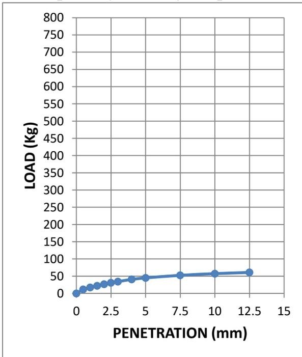
**Fig. 3.51: Load-penetration curve at OMC+3% of sample 6 (dynamically compacted soil)**
