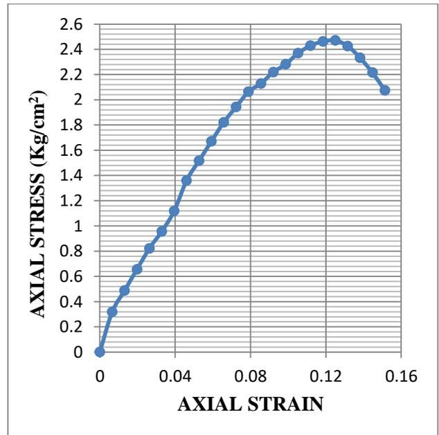
**Fig.3.64: Stress-strain graph of UCS test for sample 2 at OMC+5% (Dynamically Compacted)**
