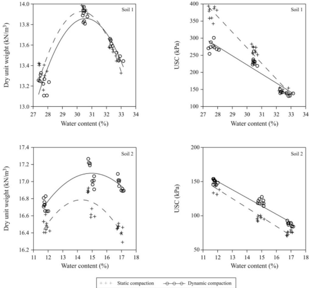
**Fig. 2.3: Compaction curves and Unconfined Compressive Strength (UCS) of soil 1 and soil 2 (Dario et al. (2010))**
