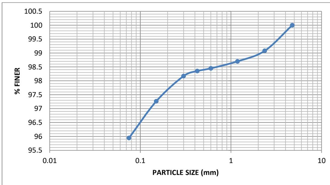
**Fig. 3.10: Gradation curve for sample 6**
