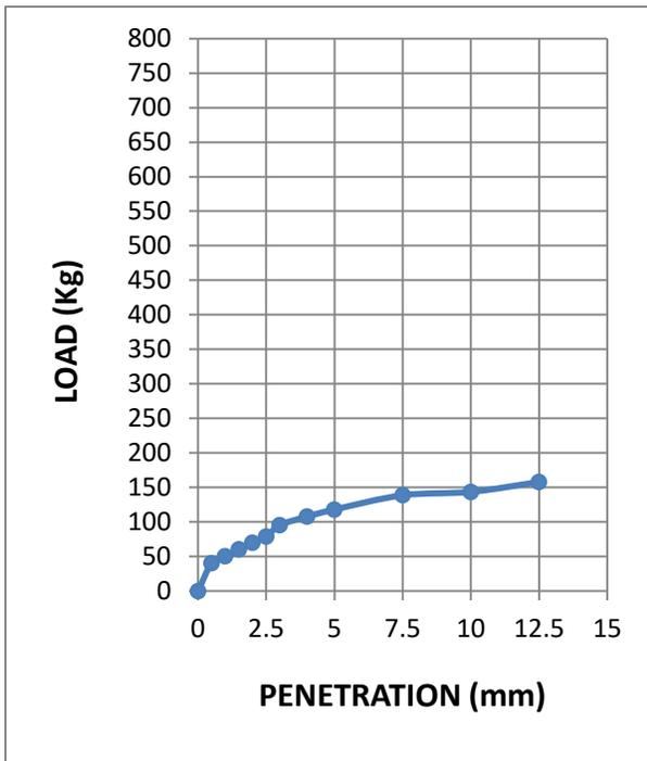
**Fig. 3.43: Load-penetration curve at OMC of sample 5 (dynamically compacted soil)**
