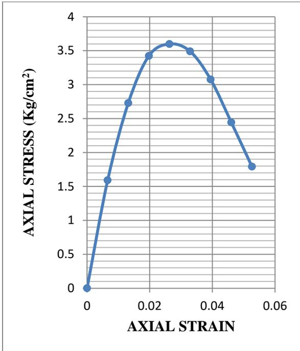
**Fig.3.65: Stress-strain graph of UCS test for sample 3 at OMC-3% (Statically Compacted)**
