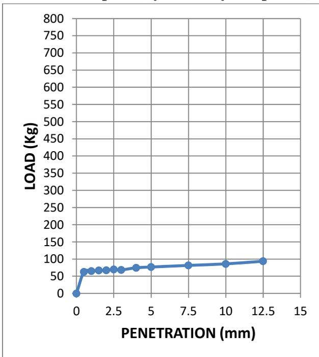
**Fig. 3.27: Load-penetration curve at OMC+5% of sample 2 (dynamically compacted soil)**
