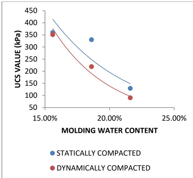
**Fig. 4.45: Superimposed curves of UCS values vs. molding water contents of statically and dynamically compacted soil for sample 3**
