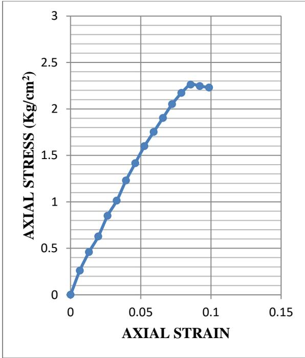
**Fig.3.81: Stress-strain graph of UCS test for sample 5 at OMC+3% (Statically Compacted)**
