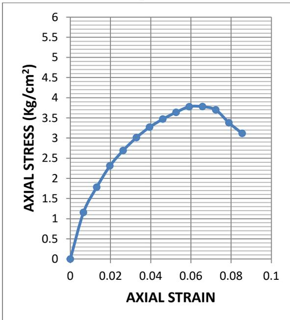
**Fig.3.79: Stress-strain graph of UCS test for sample 5 at OMC (Statically Compacted)**
