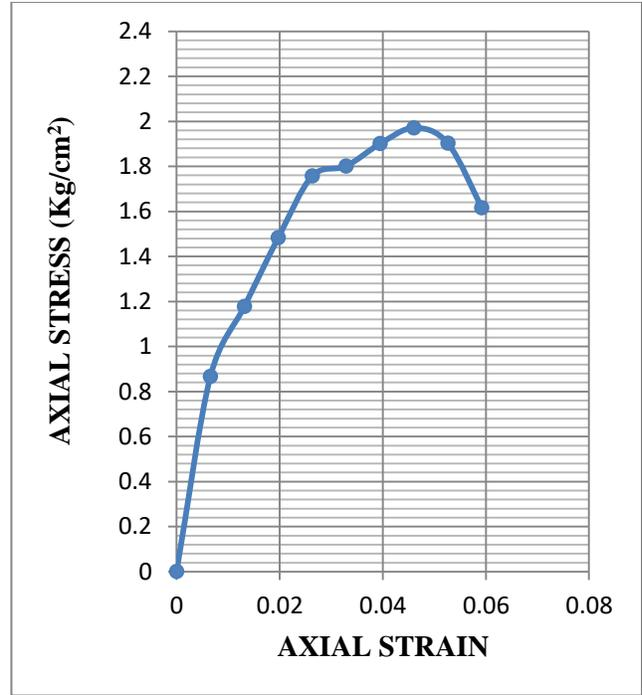
**Fig.3.62: Stress-strain graph of UCS test for sample 2 at OMC (Dynamically Compacted)**
