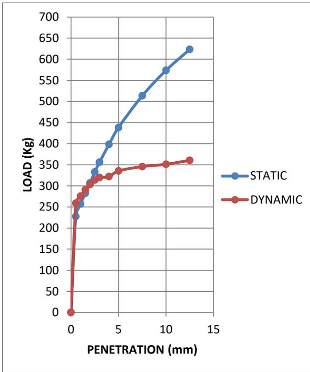
**Fig. 4.13: Superimposed curves of CBR test on statically and dynamically compacted soil-sample 5 at OMC-3%**
