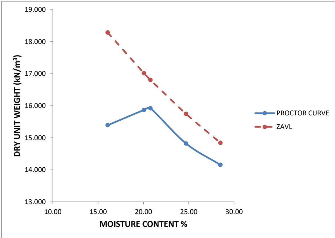
**Fig.3.16. Dynamic compaction curve for sample 6**
