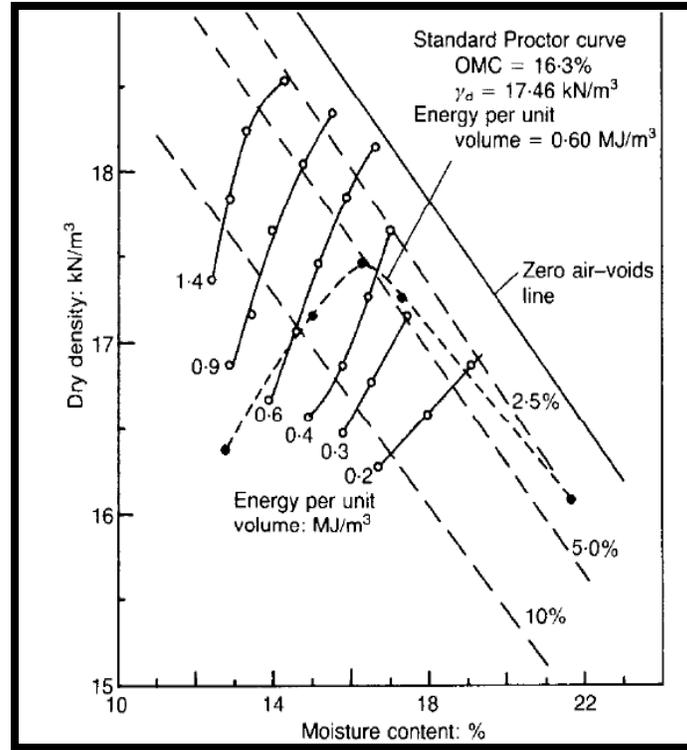
**Fig. 2.1: Comparison between static compaction method and the standard Proctor compaction method by Reddy and Jagadish (1993).**
