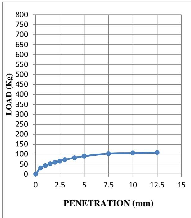
**Fig.3.22: Load-penetration curve at OMC+3% of sample1 (statically compacted soil)**
