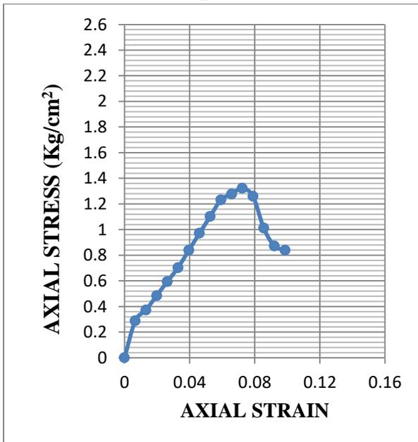
**Fig.3.63: Stress-strain graph of UCS test for sample 2 at OMC+5% (Statically Compacted)**
