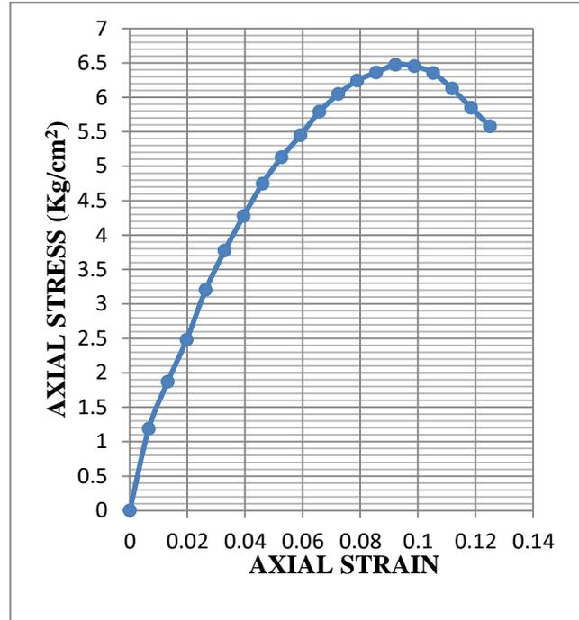
**Fig.3.54: Stress-strain graph of UCS test for sample 1 at OMC-3% (Dynamically Compacted)**
