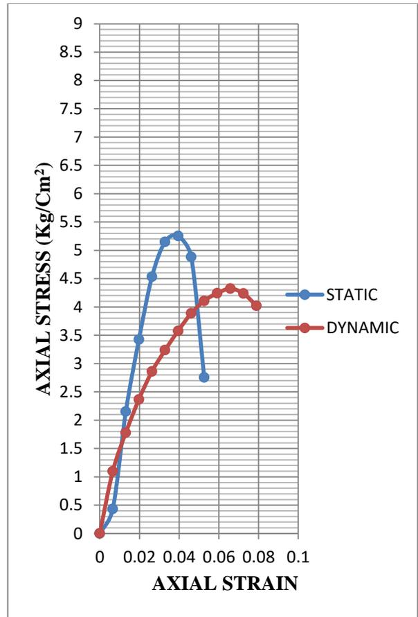
**Fig. 4.29: Superimposed curves of UCS test on statically and dynamically compacted soil- sample 4 at OMC**
