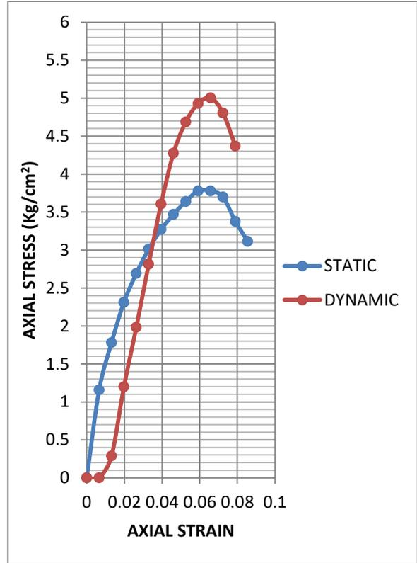
**Fig. 4.32: Superimposed curves of UCS test on statically and dynamically compacted soil- sample 5 at OMC**
