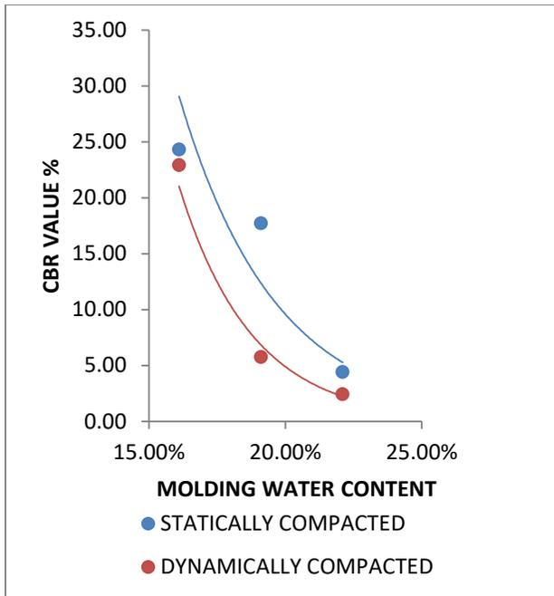
**Fig. 4.41: Superimposed curves of CBR values vs. molding water contents of statically and dynamically compacted soil for sample 5**
