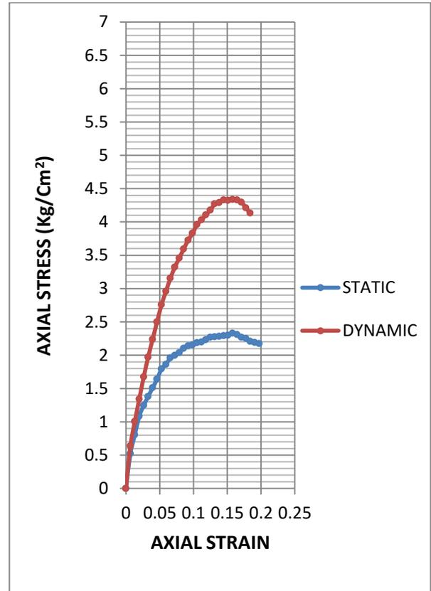
**Fig. 4.20: Superimposed curves of UCS test on statically and dynamically compacted soil- sample 1 at OMC**
