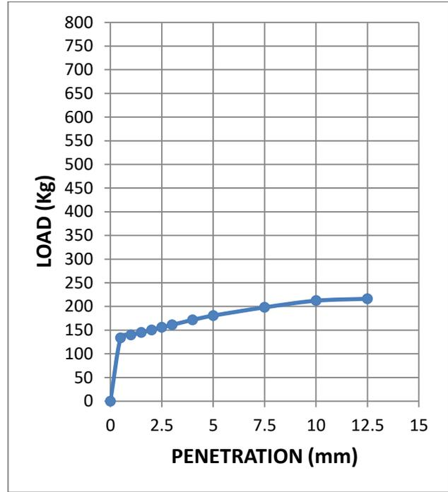
**Fig. 3.50: Load-penetration curve at OMC of sample 6 (statically compacted soil)**
