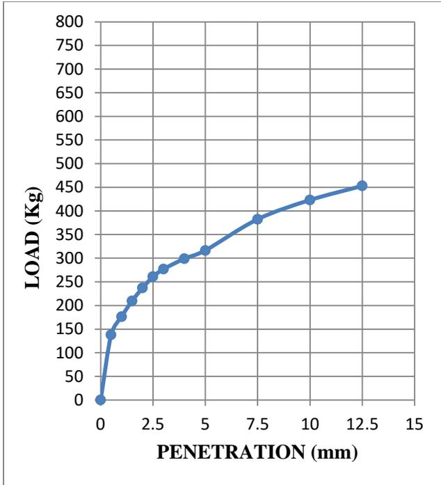
**Fig. 3.29: Load-penetration curve at OMC-3% of sample 3 (dynamically compacted soil)**
