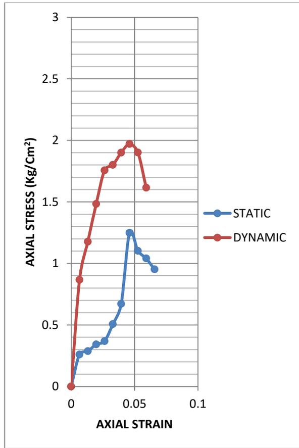
**Fig. 4.23: Superimposed curves of UCS test on statically and dynamically compacted soil- sample 2 at OMC**
