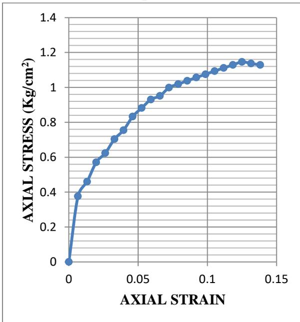
**Fig.3.87: Stress-strain graph of UCS test for sample 6 at OMC+3% (Statically Compacted)**
