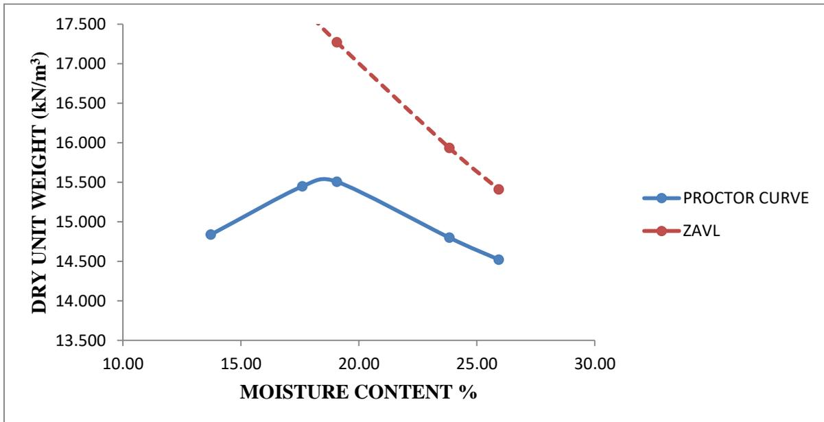
**Fig.3.13. Dynamic compaction curve for sample 3**
