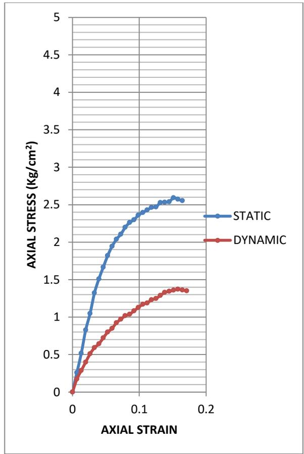
**Fig. 4.35: Superimposed curves of UCS test on statically and dynamically compacted soil- sample 6 at OMC**
