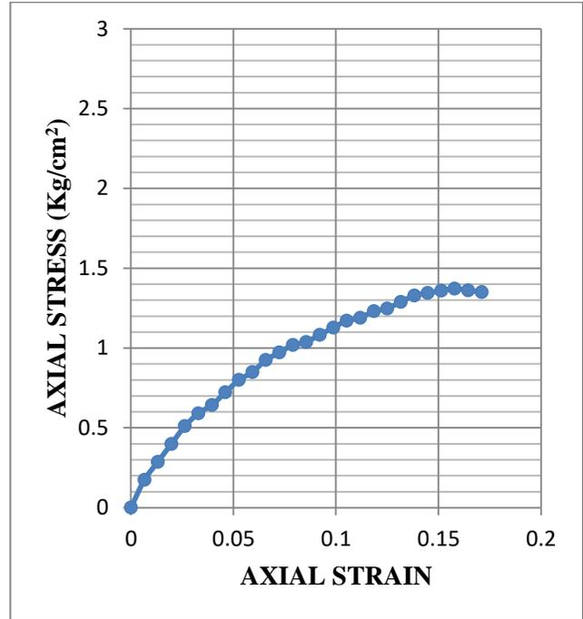
**Fig.3.86: Stress-strain graph of UCS test for sample 6 at OMC (Dynamically Compacted)**
