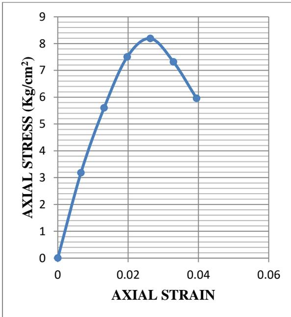
**Fig.3.71: Stress-strain graph of UCS test for sample 4 at OMC-3% (Statically Compacted)**
