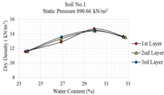
**Fig. 2.9: Dry density vs water content curve for soil no.1 at 890.66 kN/m<sup>2</sup>(B.Sharma et.al,2014)**
