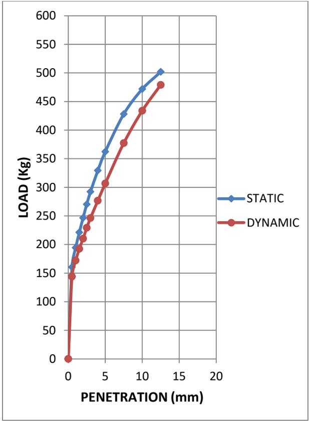
**Fig. 4.1: Superimposed curves of CBR test on statically and dynamically compacted soil- sample 1 at OMC-3%**
