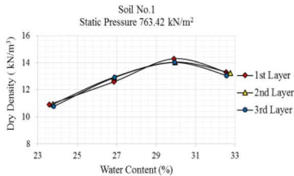
**Fig. 2.8: Dry density vs water content curve for soil no.1 at 763.42 kN/m² (B.Sharma et.al,2014)**
