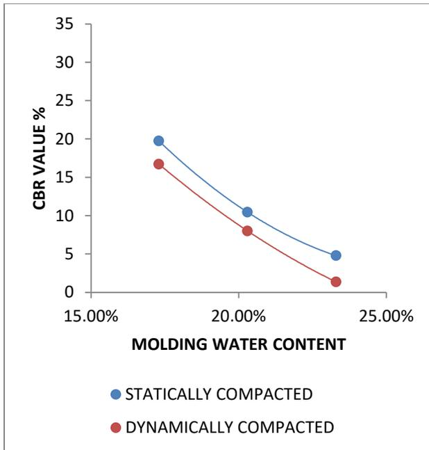
**Fig. 4.37: Superimposed curves of CBR values vs. molding water contents of statically and dynamically compacted soil for sample 1**
