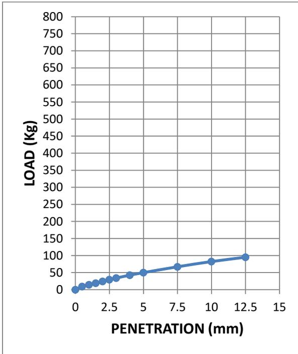
**Fig. 3.45: Load-penetration curve at OMC+3% of sample 5 (dynamically compacted soil)**
