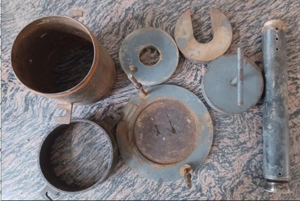
**Fig 3.1: Different Apparatus Required to Conduct CBR Test**
