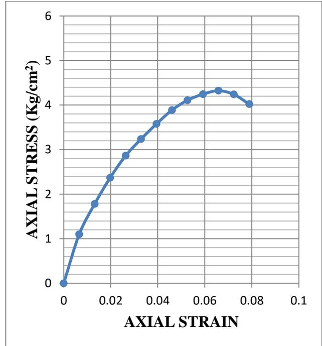
**Fig.3.74: Stress-strain graph of UCS test for sample 4 at OMC (Dynamically Compacted)**
