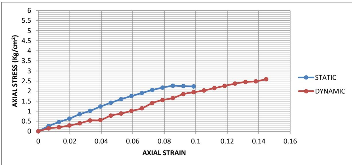
**Fig. 4.33: Superimposed curves of UCS test on statically and dynamically compacted soil- sample 5 at OMC+3%**
