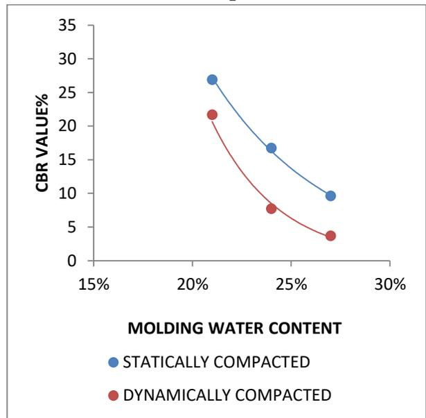
**Fig. 4.40: Superimposed curves of CBR values vs. molding water contents of statically and dynamically compacted soil for sample 4**
