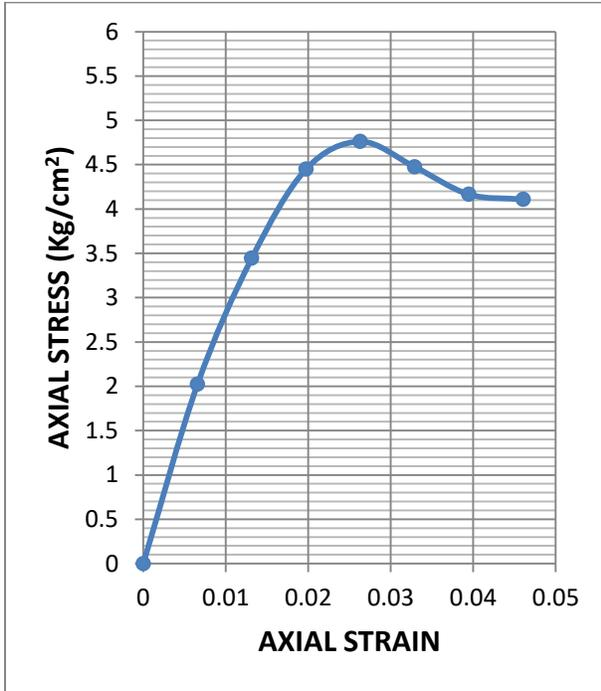
**Fig.3.77: Stress-strain graph of UCS test for sample 5 at OMC-3% (Statically Compacted)**
