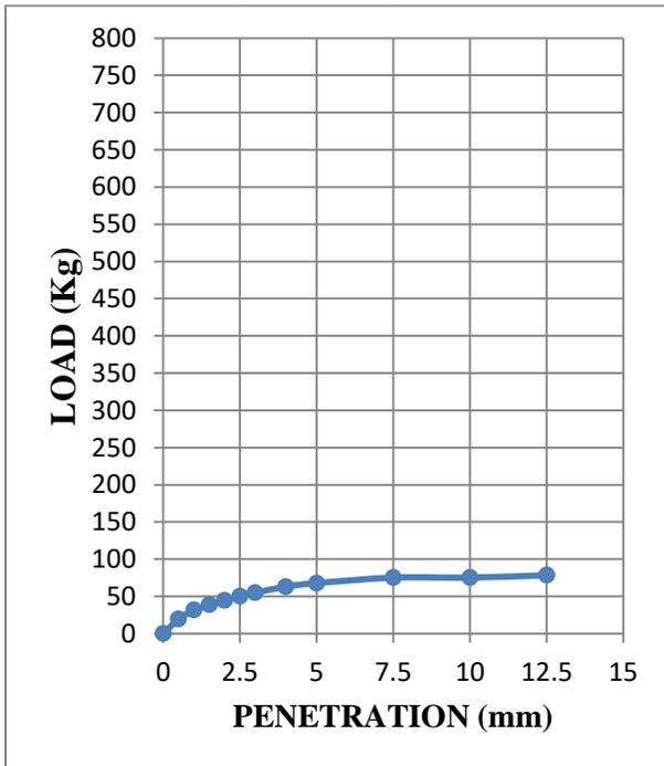
**Fig. 3.39: Load-penetration curve at OMC+3% of sample 4 (Dynamically compacted soil)**
