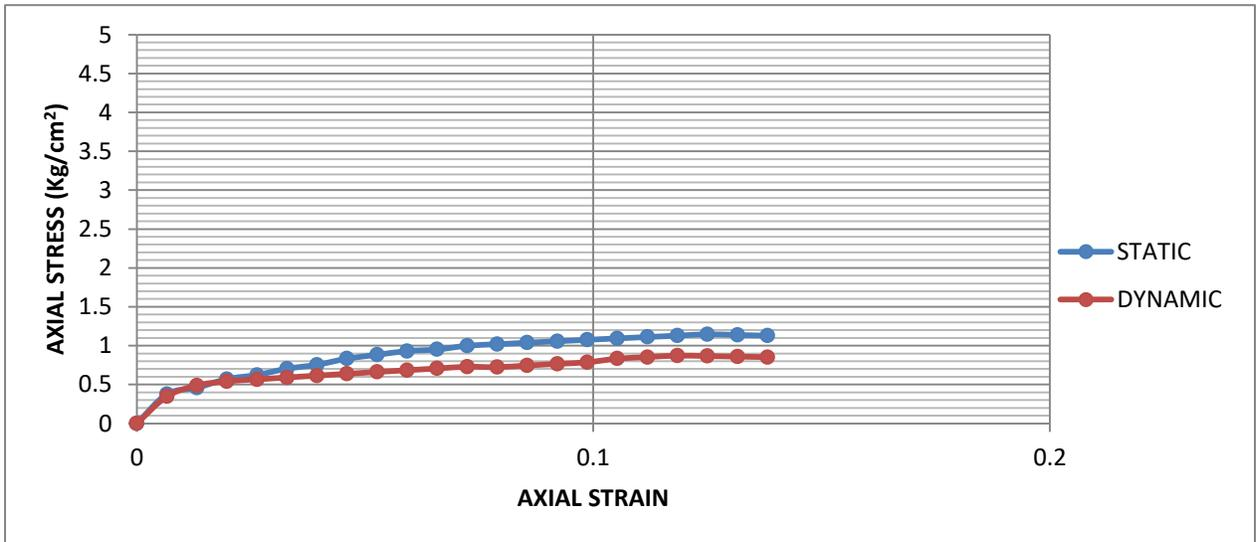
**Fig. 4.36: Superimposed curves of UCS test on statically and dynamically compacted soil- sample 6 at OMC+3%**
