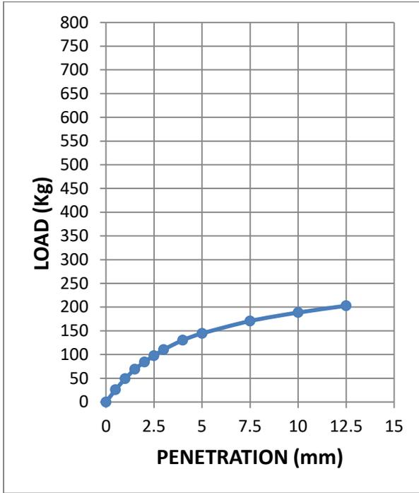
**Fig. 3.49: Load-penetration curve at OMC of sample 6 (dynamically compacted soil)**
