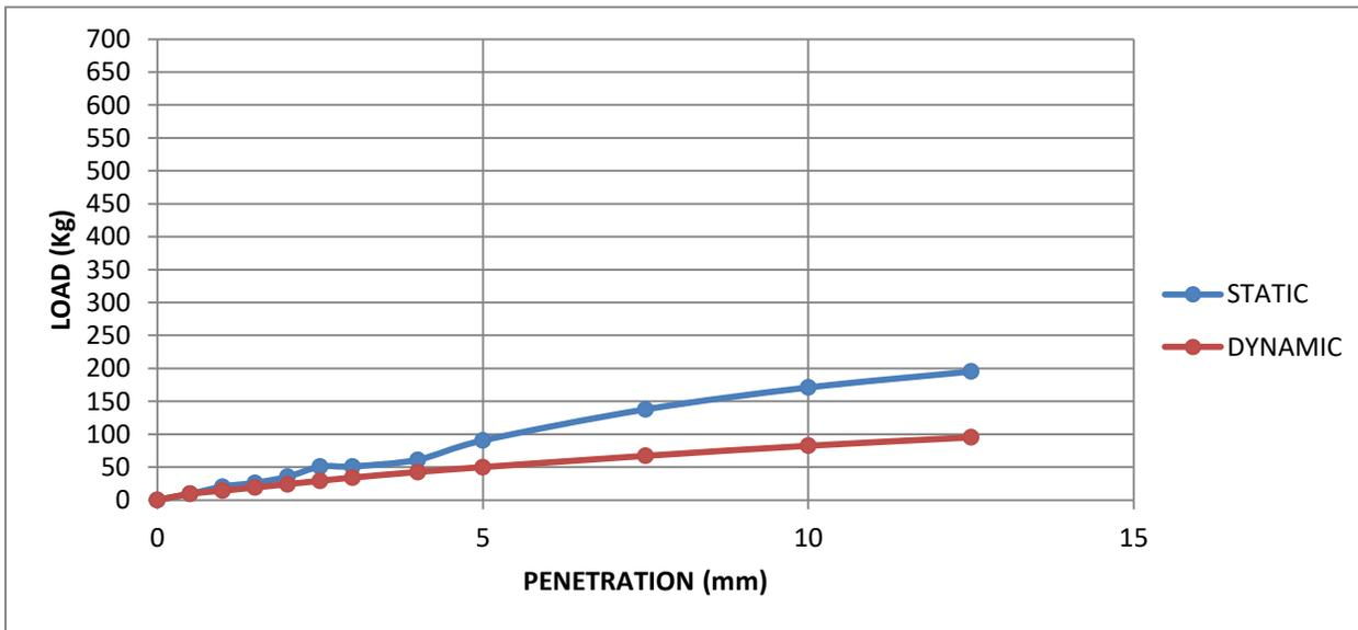
**Fig. 4.15: Superimposed curves of CBR test on statically and dynamically compacted soil-sample 5 at OMC+3%**
