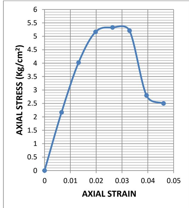
**Fig.3.78: Stress-strain graph of UCS test for sample 5 at OMC-3% (Dynamically Compacted)**
