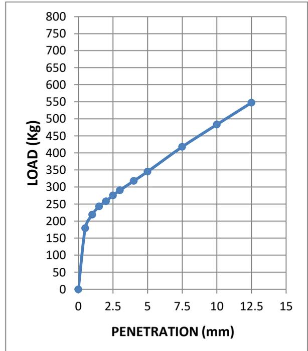
**Fig. 3.26: Load-penetration curve at OMC of sample 2 (statically compacted soil)**
