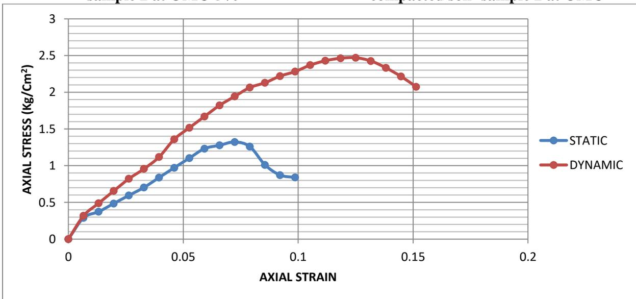
**Fig. 4.24: Superimposed curves of UCS test on statically and dynamically compacted soil- sample 2 at OMC+5%**
