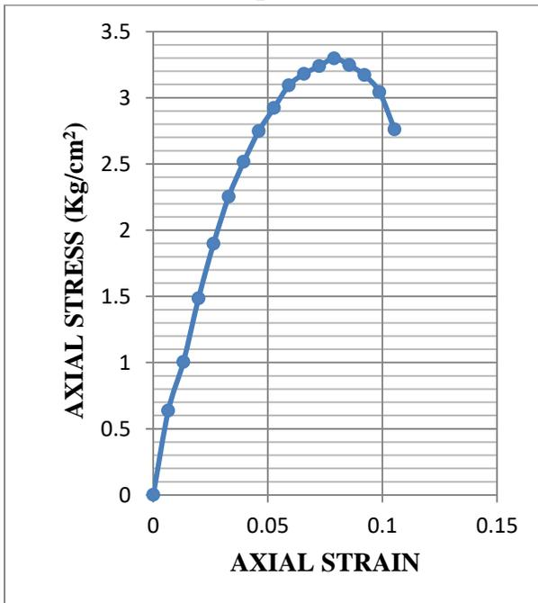
**Fig.3.67: Stress-strain graph of UCS test for sample 3 at OMC (Statically Compacted)**
