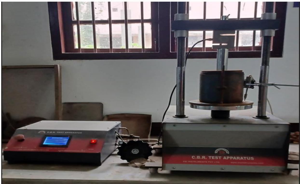
**Fig.3.3: Digital CBR Testing Machine**
