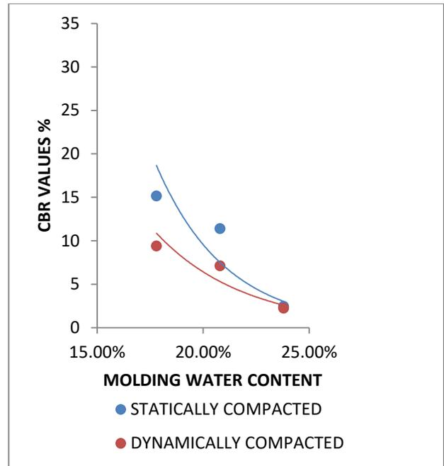
**Fig. 4.42: Superimposed curves of CBR values vs. molding water contents of statically and dynamically compacted soil for sample 6**
