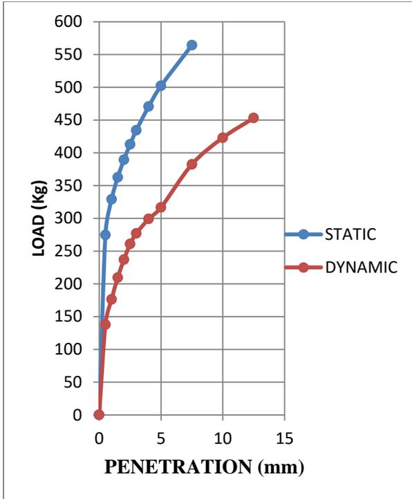
**Fig. 4.7: Superimposed curves of CBR test on statically and dynamically compacted soil- sample 3 at OMC-3%**
