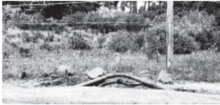
**Figure 3.6.** Beam buckling of water pipeline made of iron.
