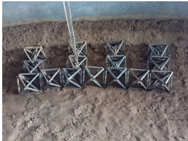
Figure 4.27: Channel bed after experimental run for low depth of flow in Arrangement 2, set
