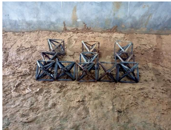
Figure 4.10: octahedron field for arrangement 1, set 1 before experiment, (medium depth)
