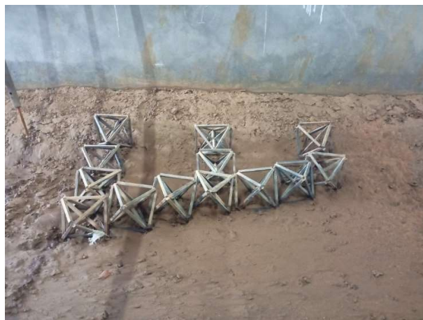
Figure 4.23: Channel bed after experimental run for medium depth of flow in Arrangement 1, set 2
