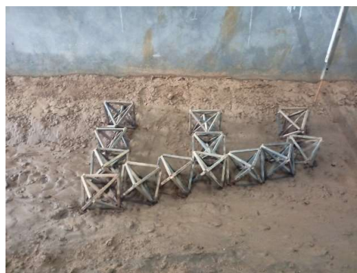
Fig 4.21: Channel bed after experimental run for low depth of flow in Arrangement 1, set 2
