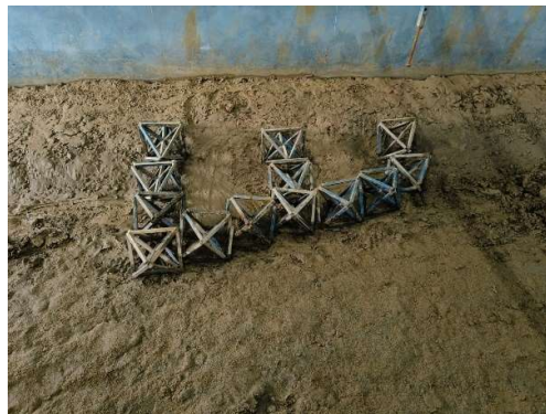
Figure 4.20: octahedron field for arrangement 1, set2, before experiment, (low depth)
