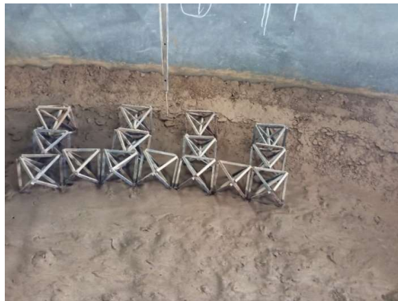
Figure 4.31: Channel bed after experimental run for high depth of flow in Arrangement 2, set
