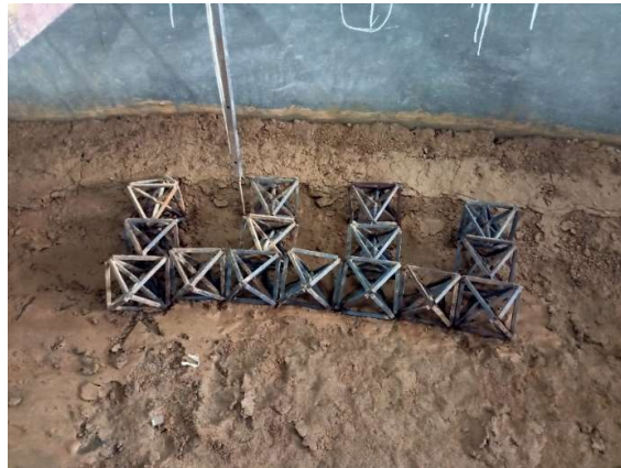
Figure 4.26: octahedron field for arrangement 2, set2, before experiment, (low depth)
