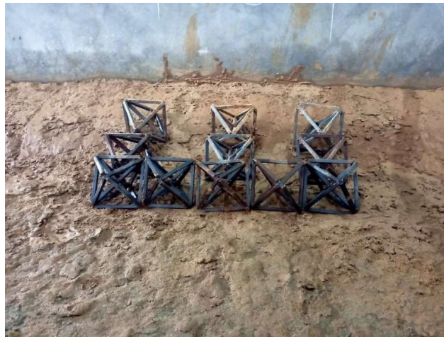
Figure 4.8: octahedron field for arrangement 1, set1, before experiment, (low depth)
