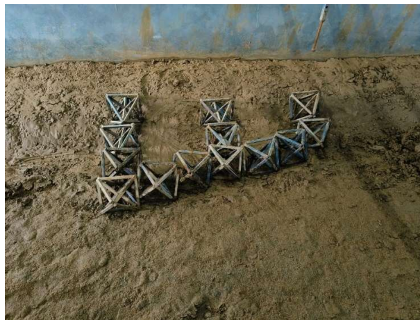
Figure 4.22: octahedron field for arrangement 1, set2, before experiment, (medium depth)
