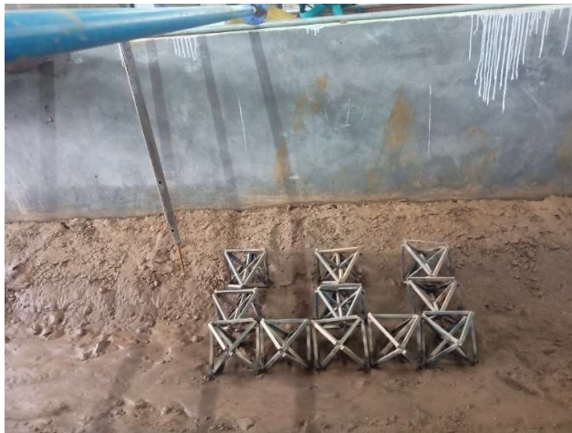
Figure 4.13: Channel bed after experimental run for high depth of flow in Arrangement 1, set
