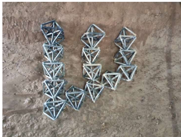
Figure 4.37: Channel bed after experimental run for high depth of flow in Arrangement 1, set
