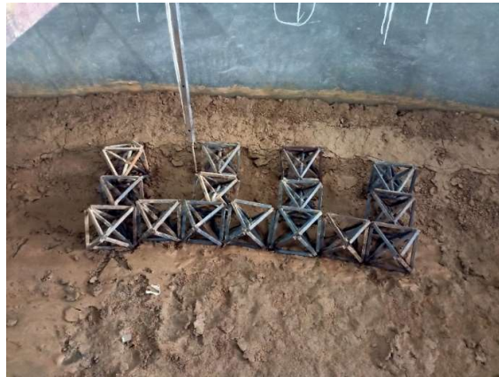
Figure 4.18: octahedron field for arrangement 2, set 1 before experiment, (High depth)
