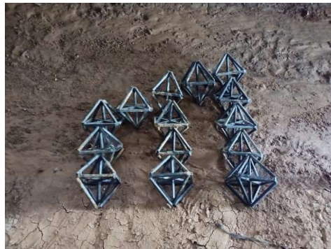
Figure 4.32: octahedron field for arrangement 1, set3, before experiment, (low depth)
