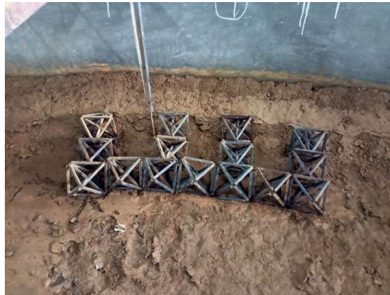
Figure 4.14: octahedron field for arrangement 2, set 1 before experiment, (low depth)
