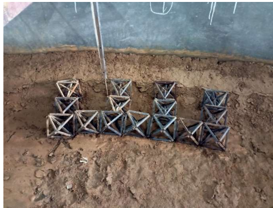
Figure 4.38: octahedron field for arrangement 2, set3, before experiment, (low depth)
