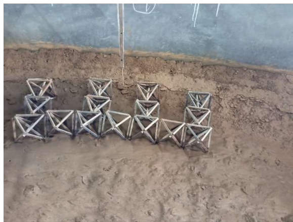
Figure 4.19: Channel bed after experimental run for high depth of flow in Arrangement 2, set
