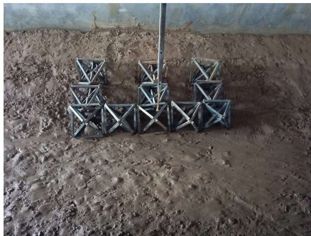
Figure 4.9: Channel bed after experimental run for low depth of flow in Arrangement 1, set 1
