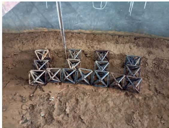
Figure 4.16: octahedron field for arrangement 2, set 1 before experiment, (medium depth)
