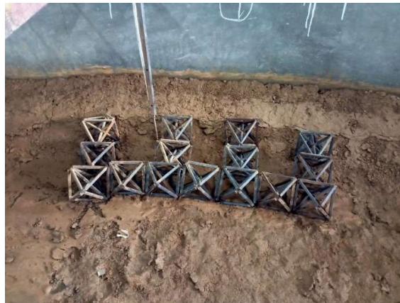
Figure 4.42: octahedron field for arrangement 2, set3, before experiment, (high depth)
