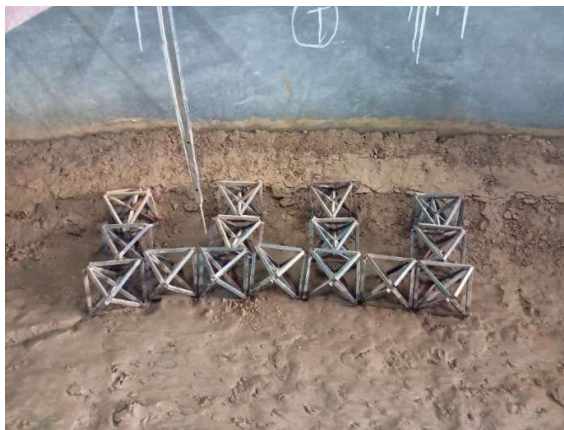
Figure 4.29: Channel bed after experimental run for medium depth of flow in Arrangement 2, set 2
