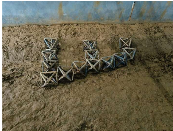
Figure 4.24: octahedron field for arrangement 1, set2, before experiment, (high depth)
