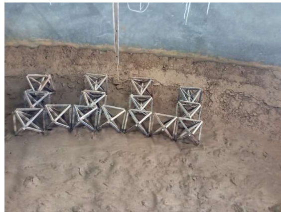
Figure 4.43: Channel bed after experimental run for high depth of flow in Arrangement 2, set 3
