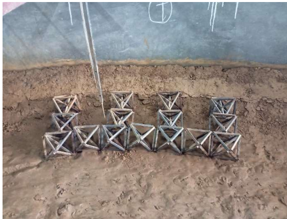
Figure 4.17: Channel bed after experimental run for medium depth of flow in Arrangement 2, set 1
