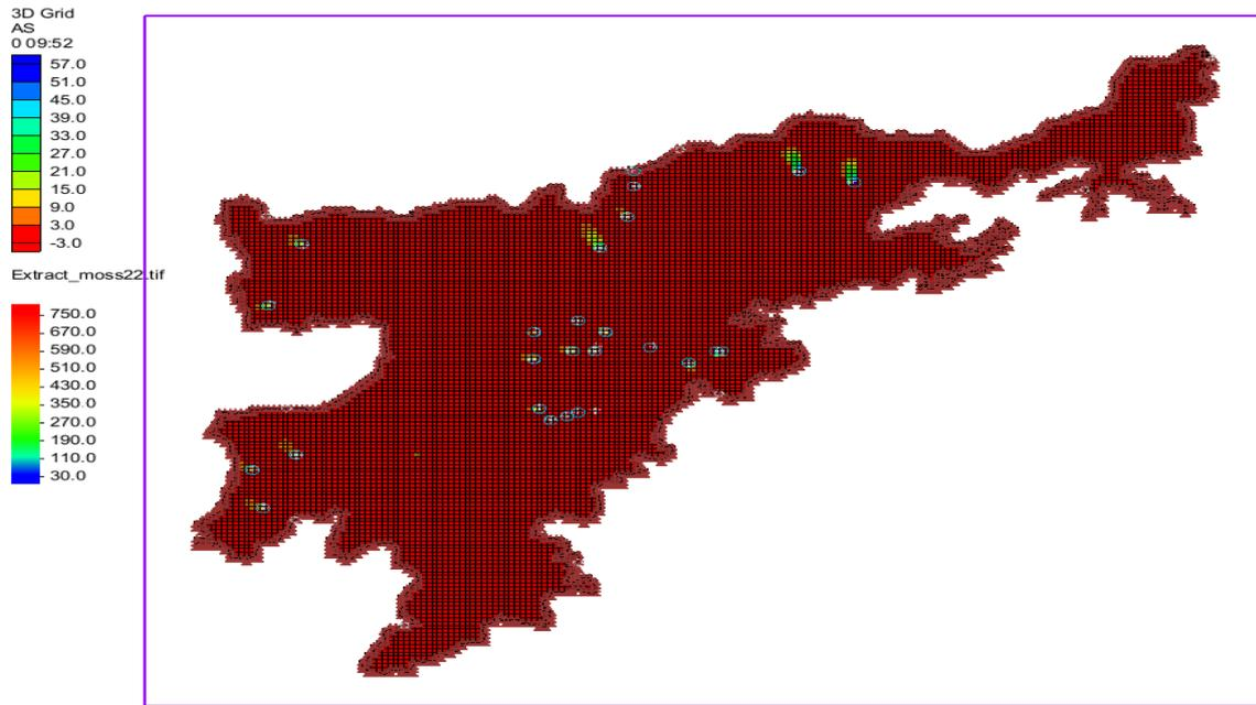
Figure 8.15: Transport of arsenic over a 90-day period simulated using MT3DMS in Nagaon
