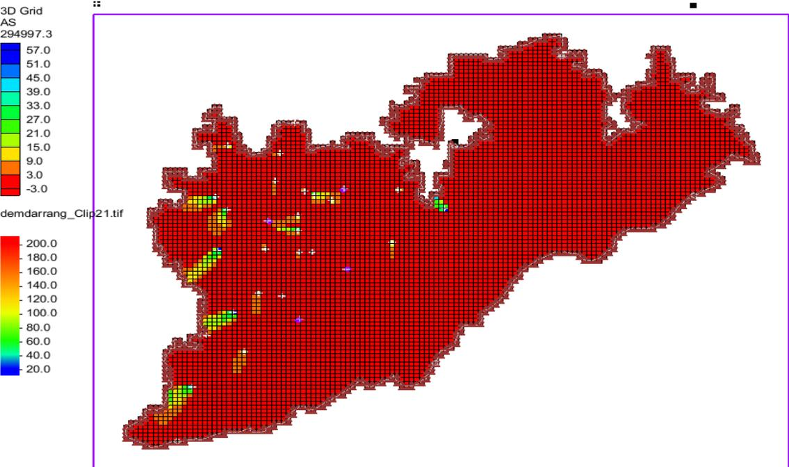
Figure 8.11: Transport of arsenic over a 630-day period simulated using MT3DMS in Darrang
