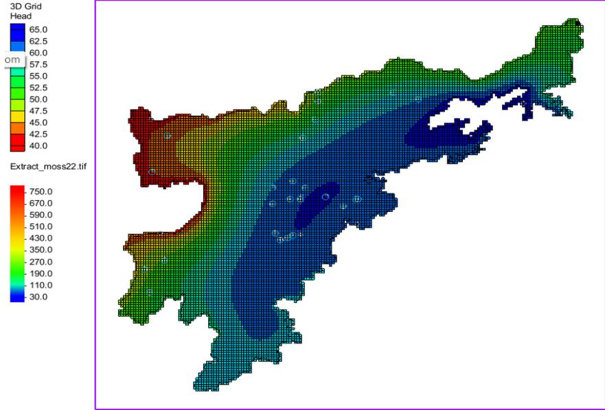
Fig 8.2 – Ground water flow model of Nagaon district using MODFLOW.
