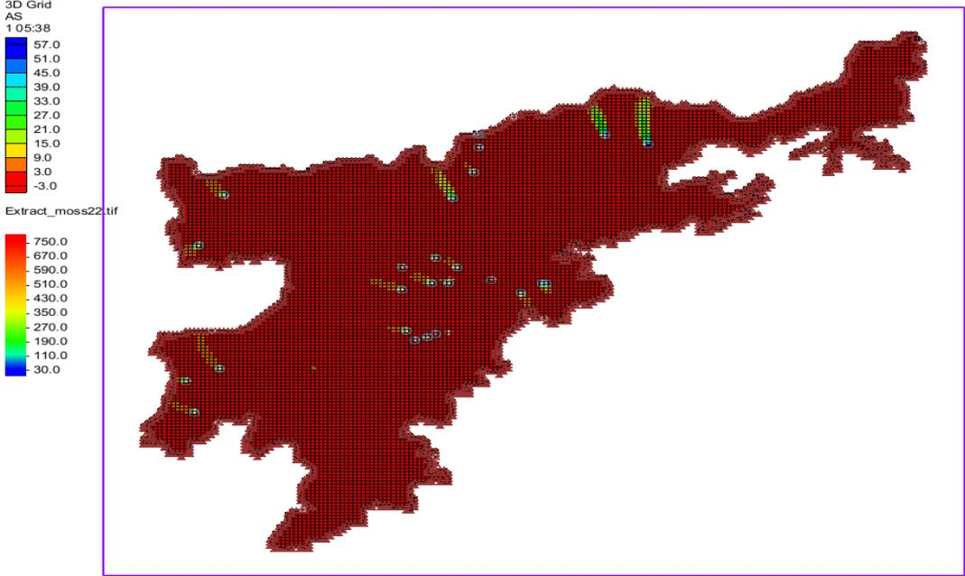
Figure 8.17: Transport of arsenic over a 270-day period simulated using MT3DMS in Nagaon
