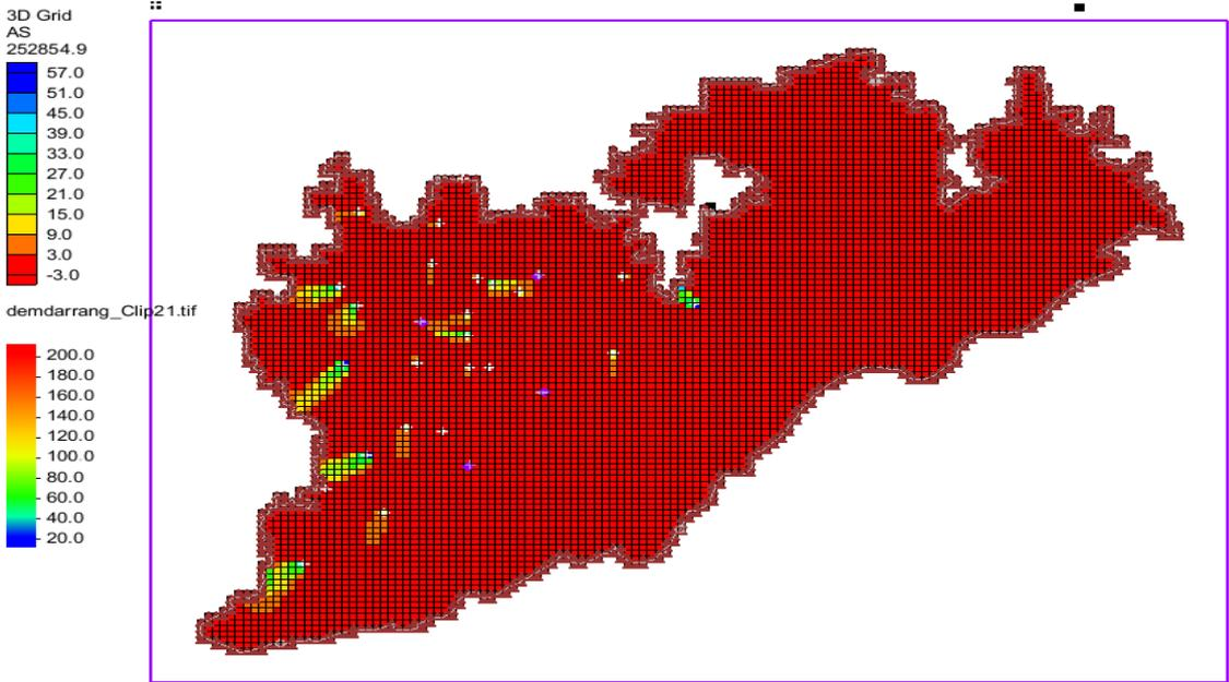
Figure 8.10: Transport of arsenic over a 540-day period simulated using MT3DMS in Darrang
