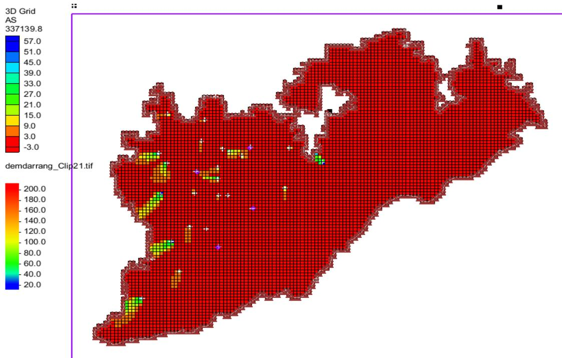
Figure 8.12: Transport of arsenic over a 720-day period simulated using MT3DMS in Darrang
