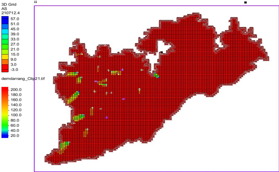
Figure 8.9: Transport of arsenic over a 450-day period simulated using MT3DMS in Darrang
