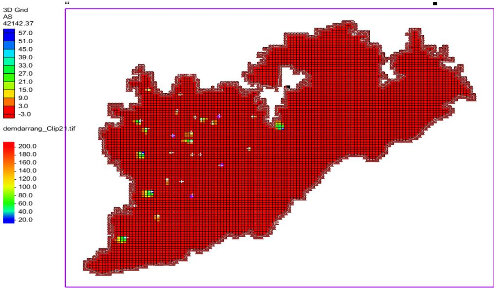
Figure 8.5: Transport of arsenic over a 90-day period simulated using MT3DMS in Darrang.
