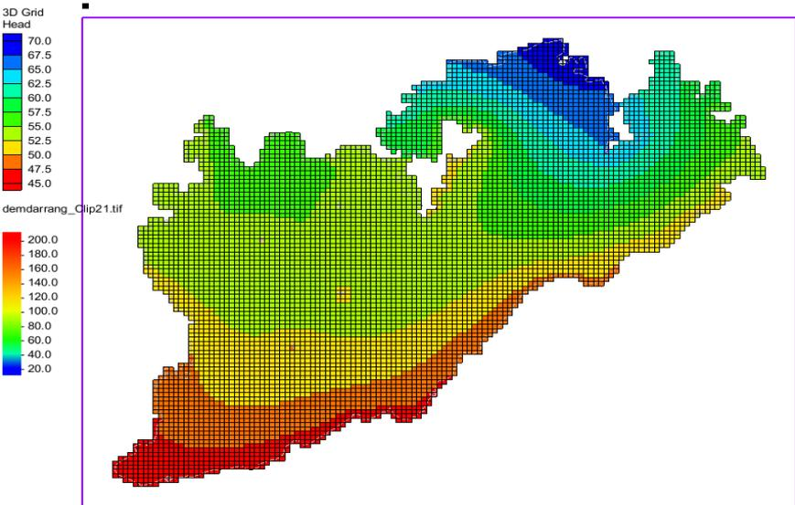
Fig 8.1 – Ground water flow model of Darrang district using MODFLOW.
