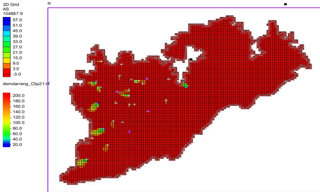
Figure 8.7: Transport of arsenic over a 240-day period simulated using MT3DMS in Darrang
