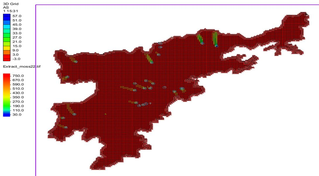
Figure 8.18: Transport of arsenic over a 360-day period simulated using MT3DMS in Nagaon
