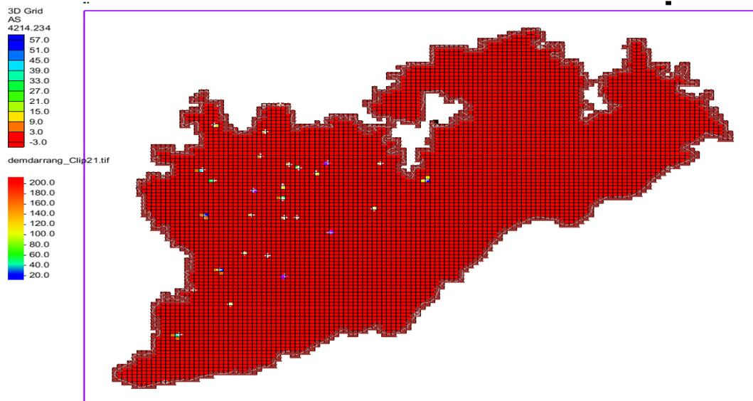
Figure 8.4: Transport of arsenic over a 9-day period simulated using MT3DMS in Darrang
