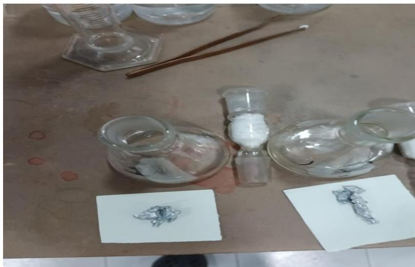
Fig -4.8 Scrubber tube and Absorber tube is prepared and glass wool is impregnated.
