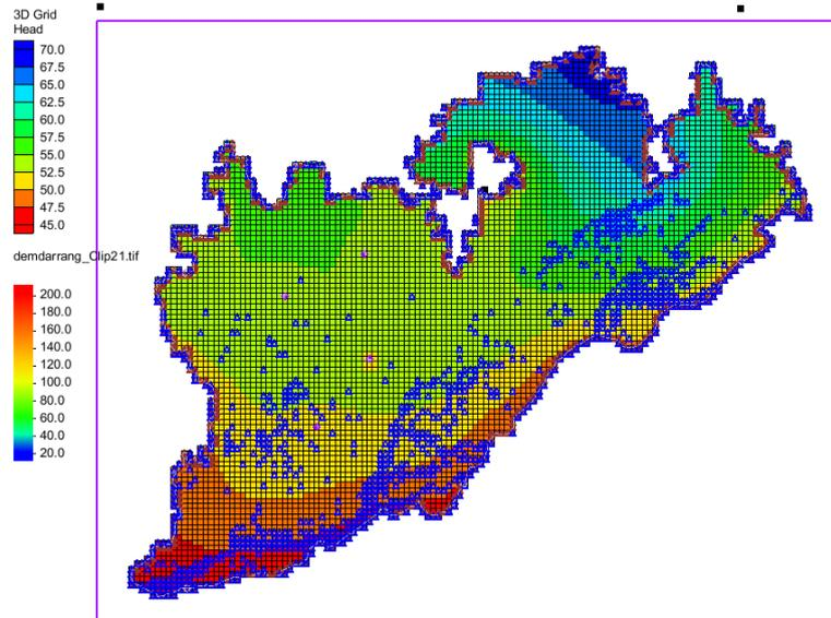
Fig 8.3 MODFLOW simulated model of study area – Darrang.
