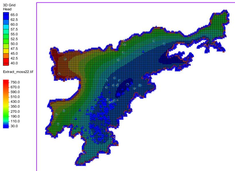
Fig 8.13 MODFLOW simulated model of study area – Nagaon
