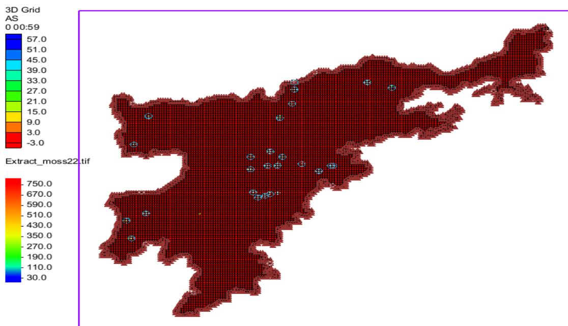
Figure 8.14: Transport of arsenic over a 9-day period simulated using MT3DMS in Nagaon
