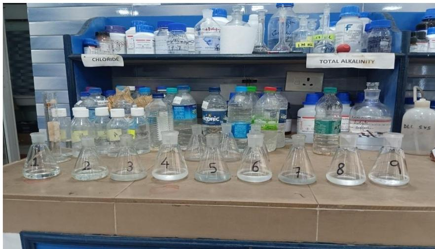
Fig - 4.7 35ml of water sample in 100ml of conical flask.
