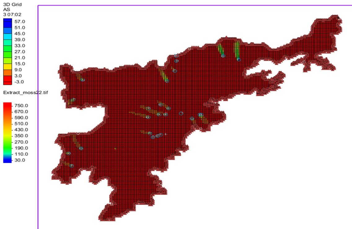
Figure 8.22: Transport of arsenic over a 720-day period simulated using MT3DMS in Nagaon
