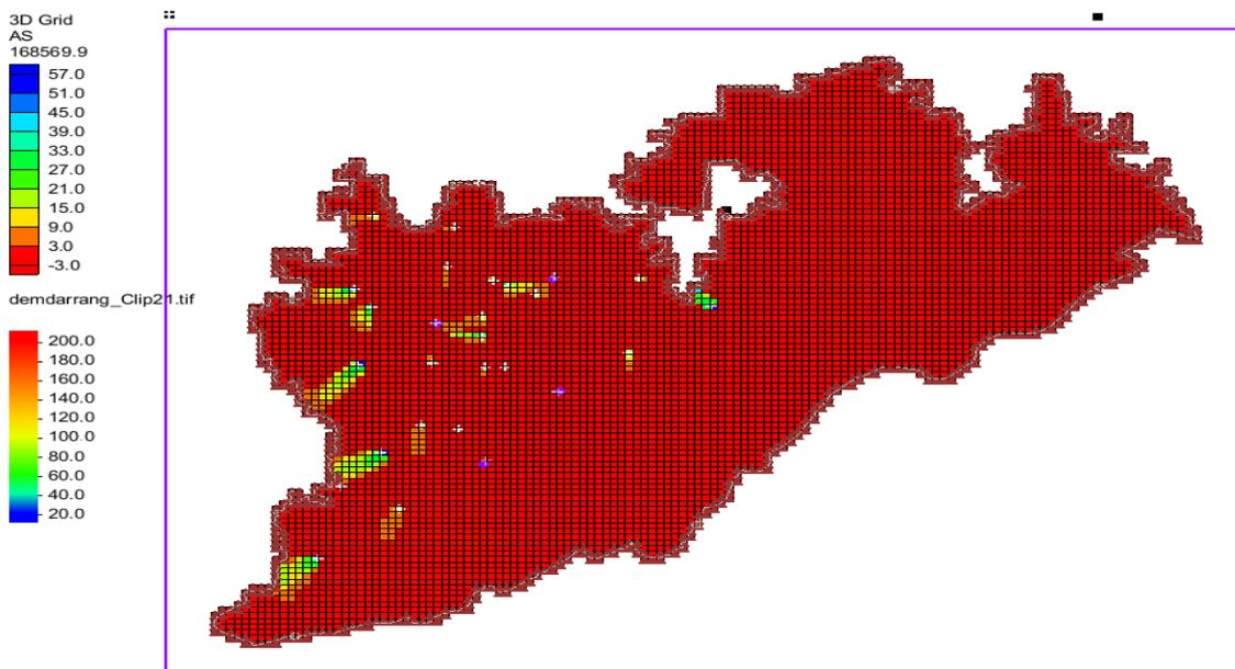
Figure 8.8: Transport of arsenic over a 360-day period simulated using MT3DMS in Darrang.
