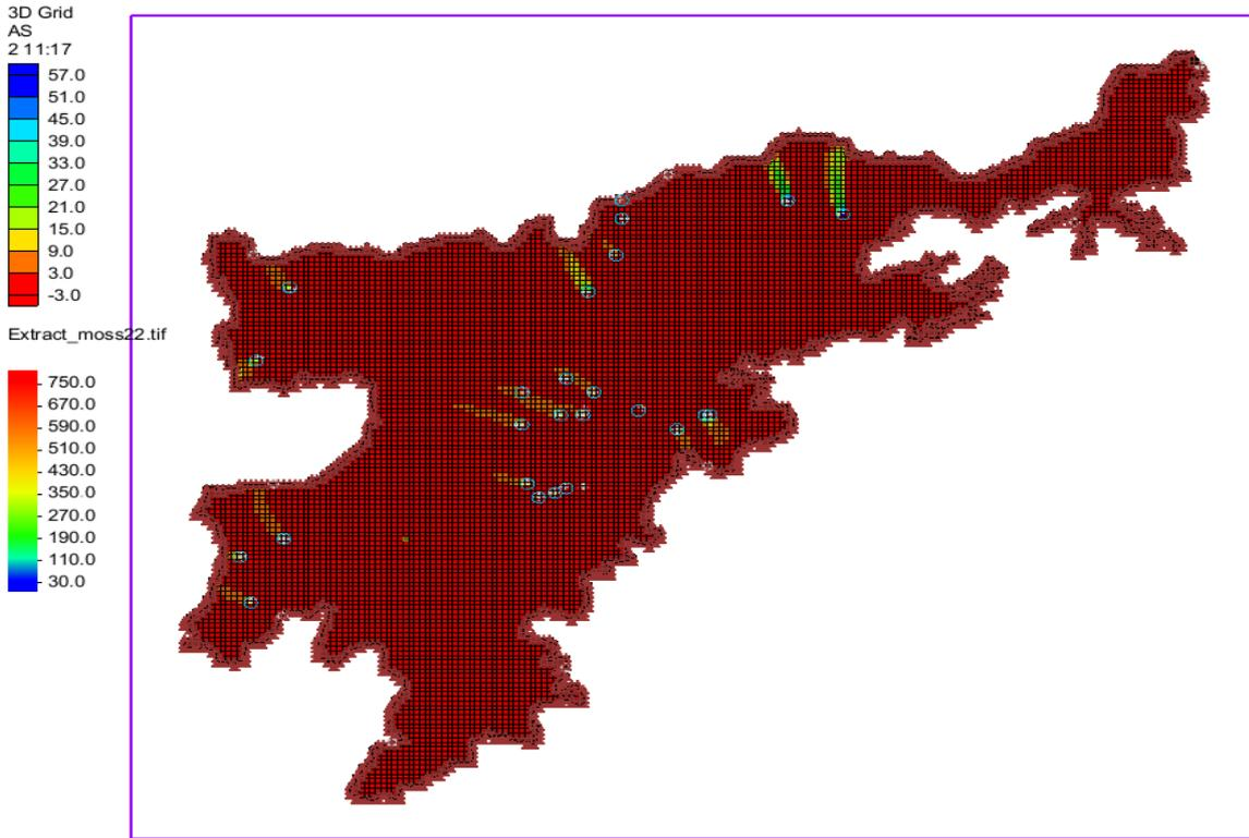
Figure 8.20: Transport of arsenic over a 540-day period simulated using MT3DMS in Nagaon
