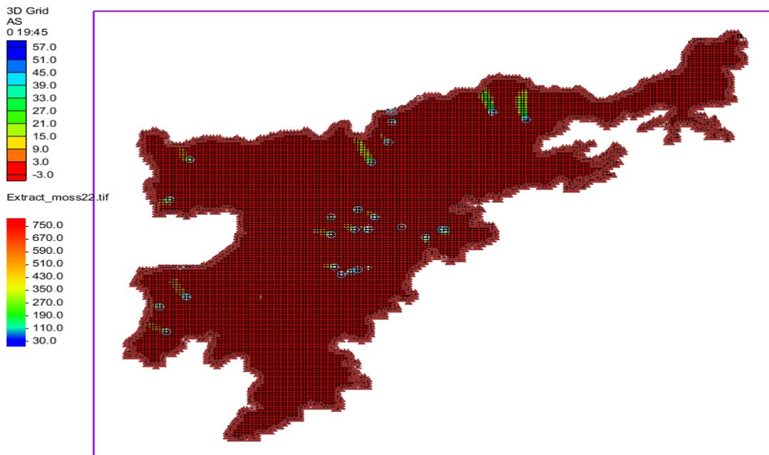
Figure 8.16: Transport of arsenic over a 180-day period simulated using MT3DMS in Nagaon
