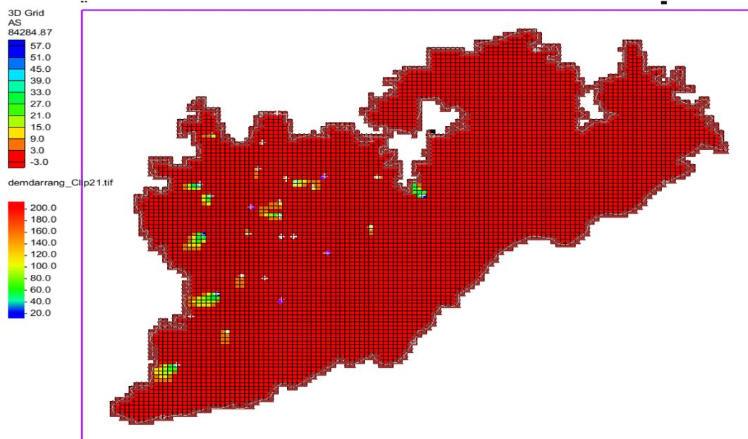
Figure 8.6: Transport of arsenic over a 180-day period simulated using MT3DMS in Darrang.
