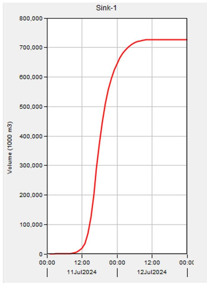
Fig 5.2: Cumulative outflow at the Sink (U/S of the study area) obtained from HEC HMS
