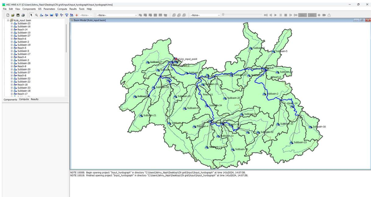
Fig 4.9: HEC HMS interface showing Sub Basin & Junctions
