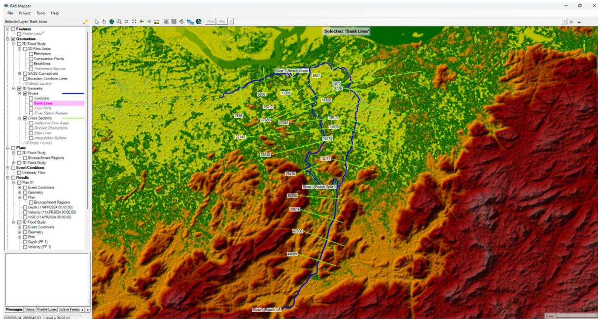
Fig 4.12: Marking Bank Lines, Flow Paths and cross sections in the RAS Mapper
