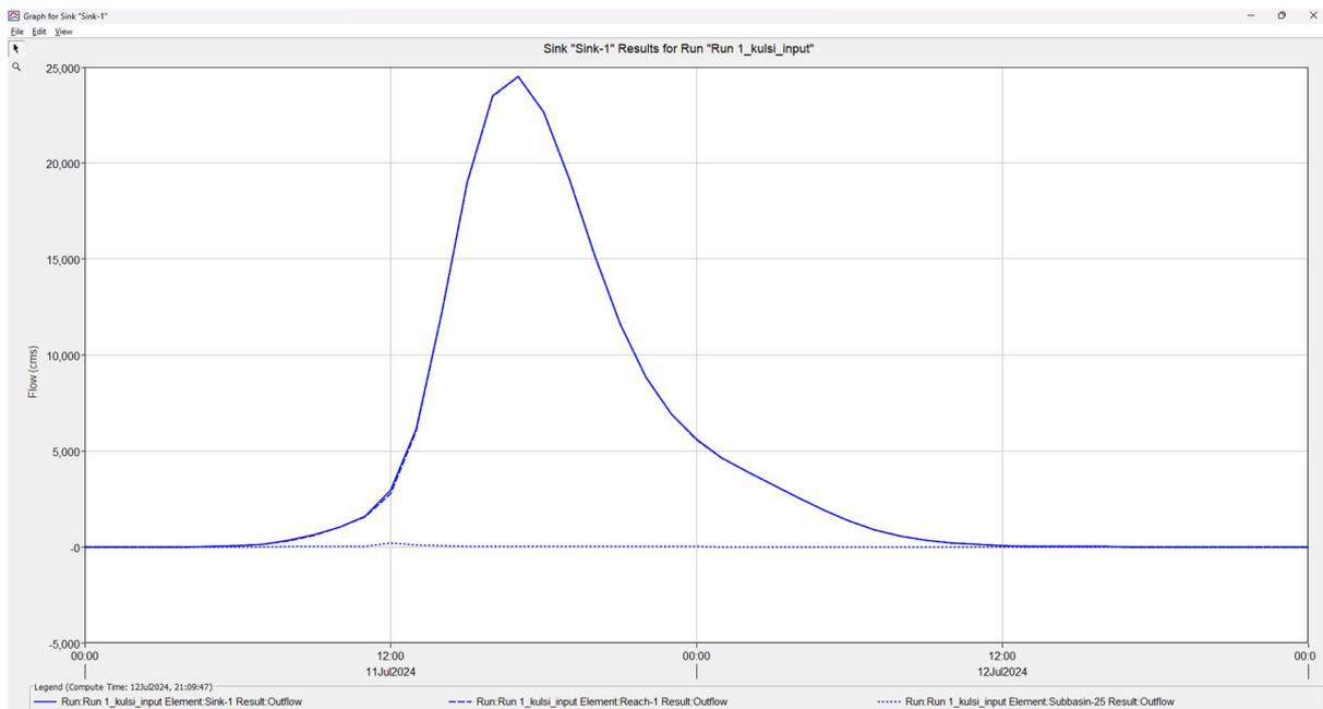
Fig 5.1: Hydrograph of Sink (U/S of the study area) obtained from HEC HMS
