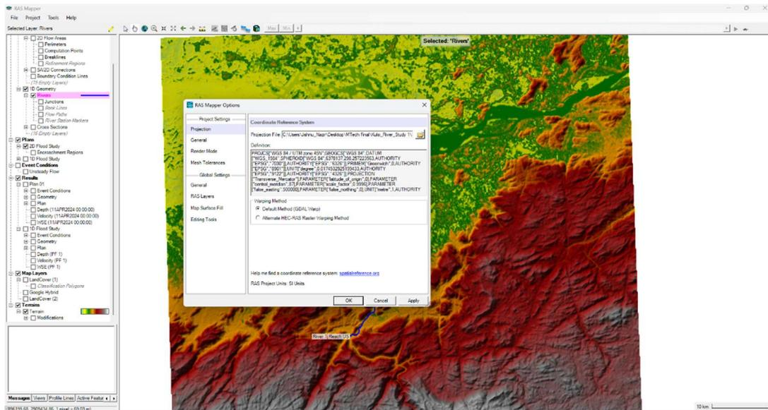
Fig 4.10: Applying Projection to the Terrain in RAS Mapper
