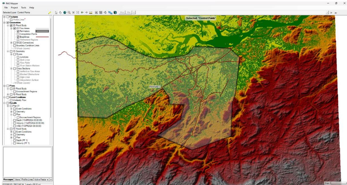
Fig 4.19: Adding breaklines to the Geometry
