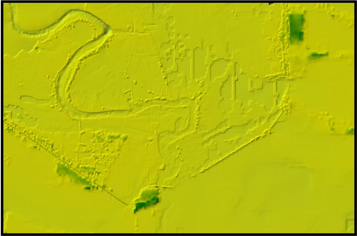
Figure 6.5 High resolution DEM of the area prepared using LiDAR and Eco-Sounding data
