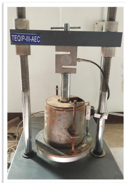
Fig 4.12 CBR Test Apparatus
