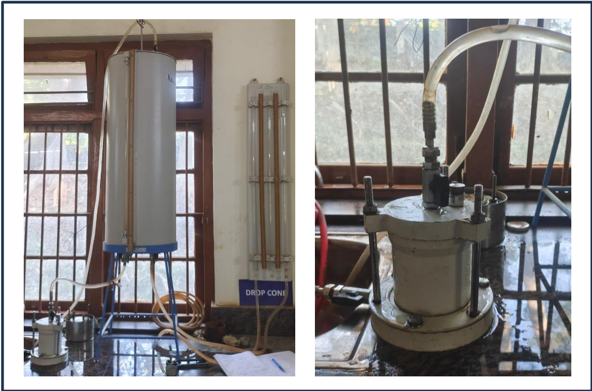
Fig 4.11 Constant Head Permeability Test Apparatus
