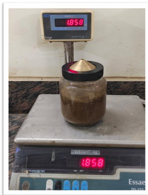
Fig 4.1 Specific Gravity using Pycnometer
