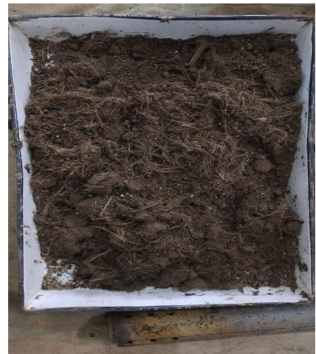
Fig 3.10 : Jute fiber mix with soil
