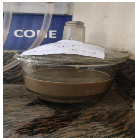
Fig 3.4: Sample placed for wet sieve analysis
