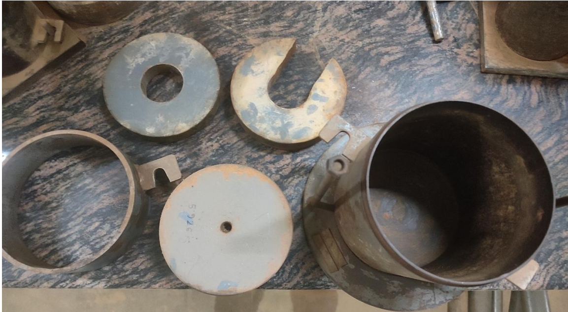
Fig 3.5 : Base plate, collar, spacer disc, mould , 2.5kg surcharge load used in CBR test
