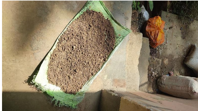
Fig 3.2 : Air drying of soil sample
