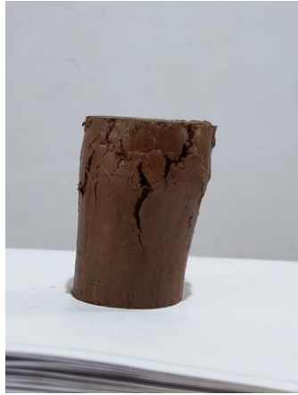
Fig 20: Failure sample (soil + 0% fiber)
