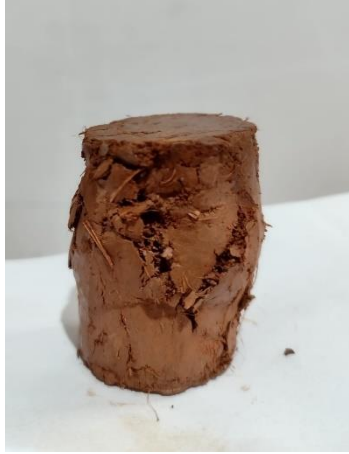
Fig 30: Failure sample (soil + 1% fiber)
