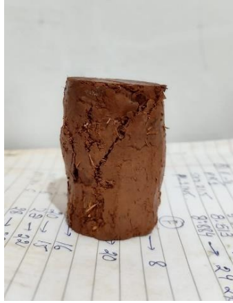
Fig 28: Failure sample (soil + 0.8% fiber)
