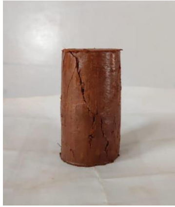
Fig 22: Failure sample (soil + 0.2% fiber)
