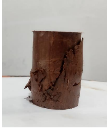
Fig 24: Failure sample (soil + 0.4% fiber)
