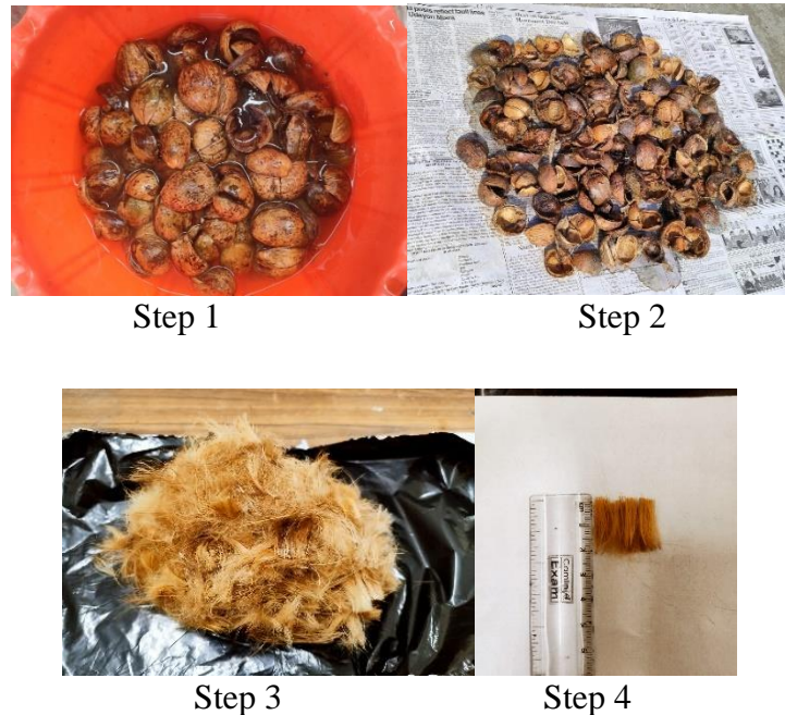
Fig 9: Fibers prepared for testing
