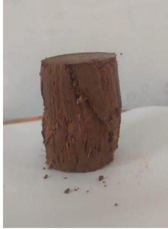
Fig 26: Failure sample (soil + 0.6% fiber)
