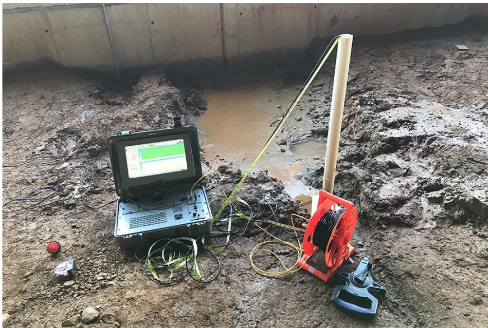
Fig 2.6: Parallel Seismic Test Equipment Setup (Source:
