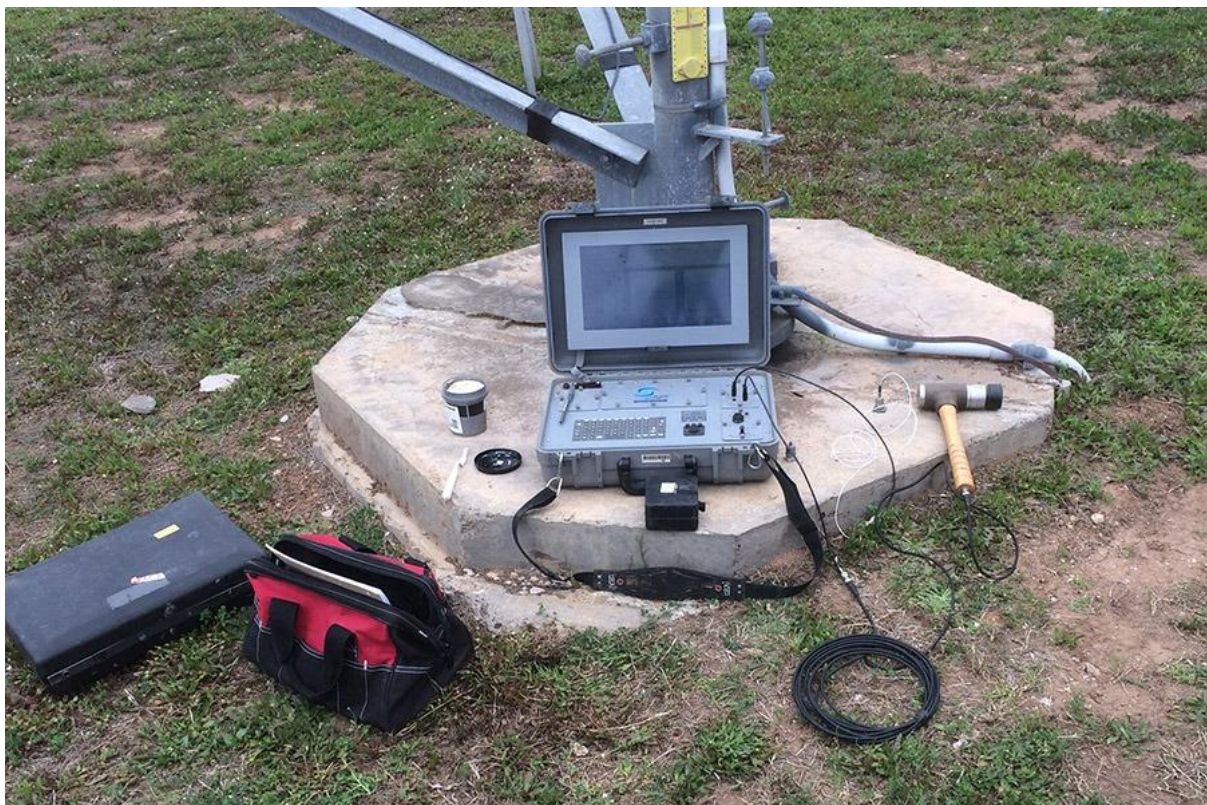
Fig 2.1: Pile Integrity Test Equipment
