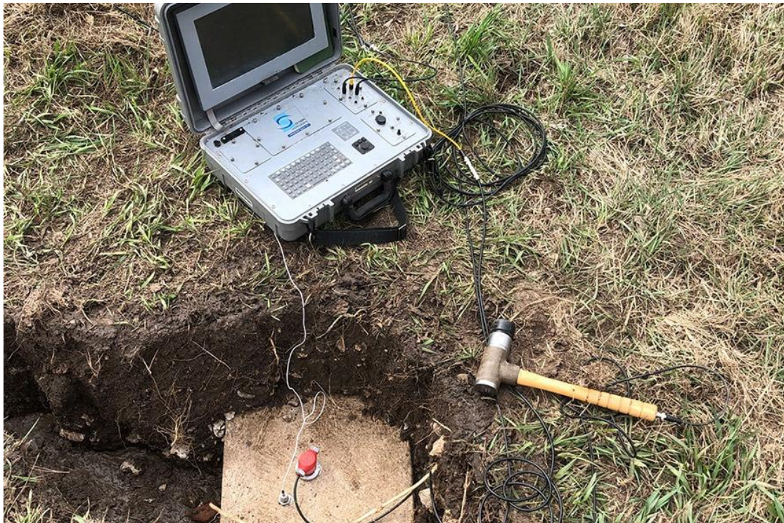
Fig 3.1: Pile Integrity Test Instrument Setup (Source: https://olsoninstruments.com/wp-content/uploads/seir_field2.jpg )
