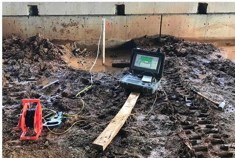
Fig 3.11: Borehole for Parallel seismic test setup
