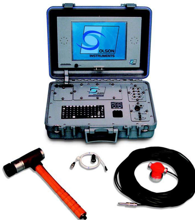
Fig 2.3: OLSON Instrument for Pile Integrity Test (Source: https://olsonengineering.com/ )
