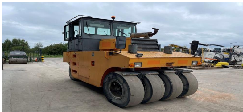
Fig 5: Pneumatic tired Roller (sources: www.wotol.com )
