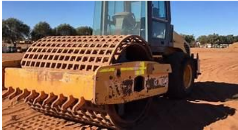
Fig 4: Grid Roller ( sources: engineeringlearn.com )
