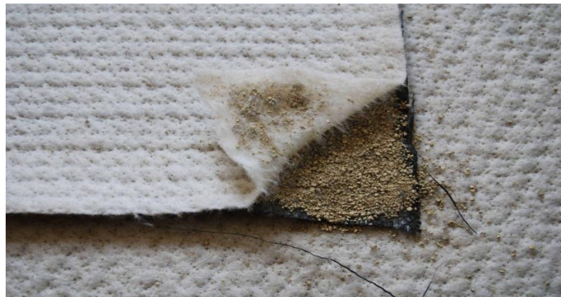
Figure 4.3: Geosynthetic Clay Liner
