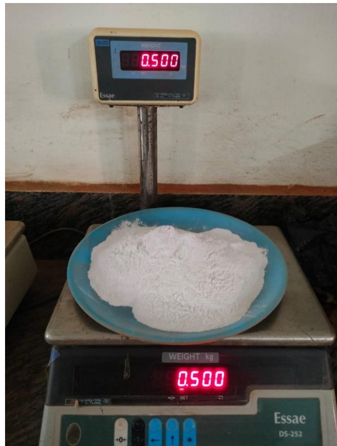
Fig 3.12: Egg shell powder being weighed for sieve analysis test.
