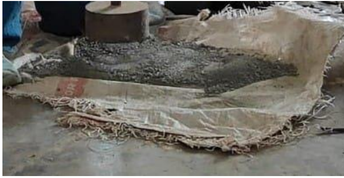
Fig 3.2: Collected soil sample being air dried in laboratory
