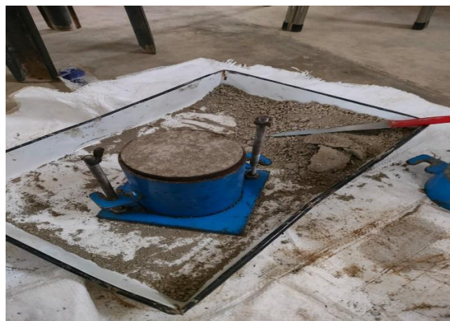
Fig 3.8: Standard Proctor test being performed.
