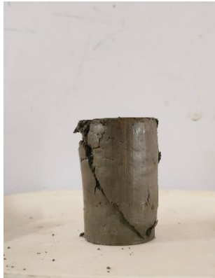
Fig 3.9: Sample after failure at UCS test
