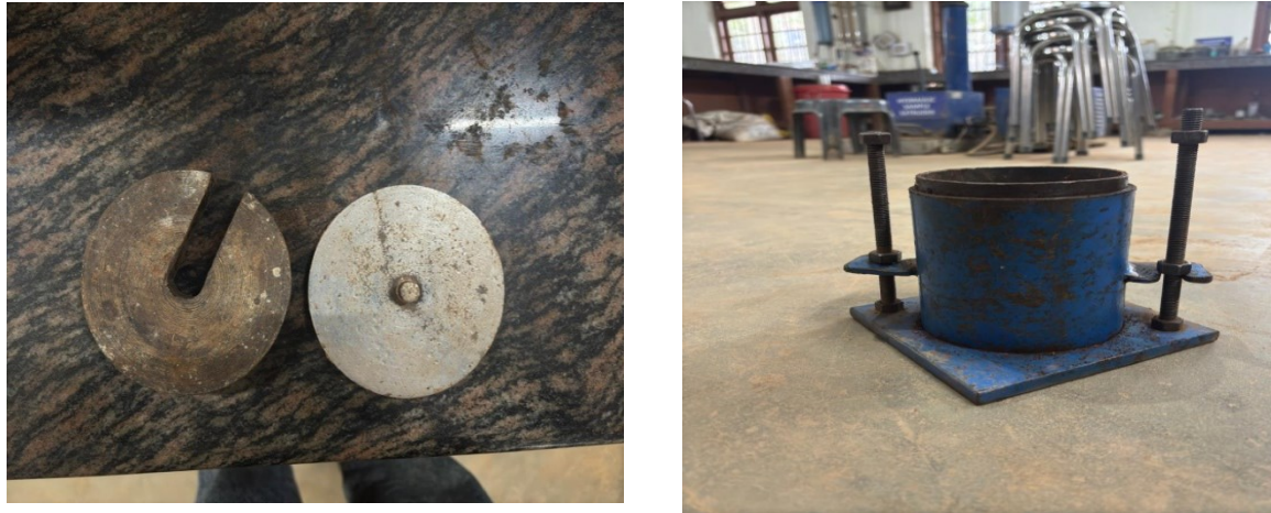
Fig 3.1: Two metal plate and Mould used in Static Compaction
