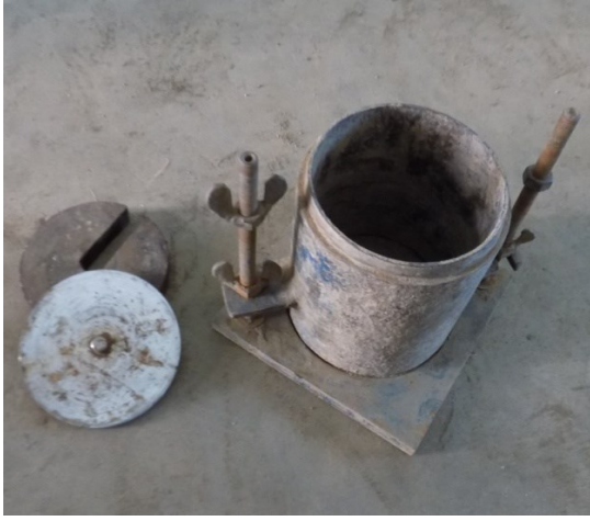
Figure 3.2: Static compaction mould with two base plates
