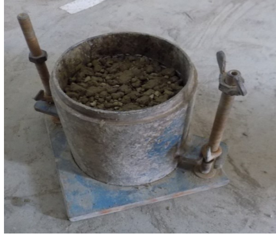
Figure 3.3: Filling the soil into the mould upto 100 mm height
