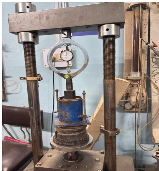
Figure 3.6: The static compaction test apparatus along with the mould
