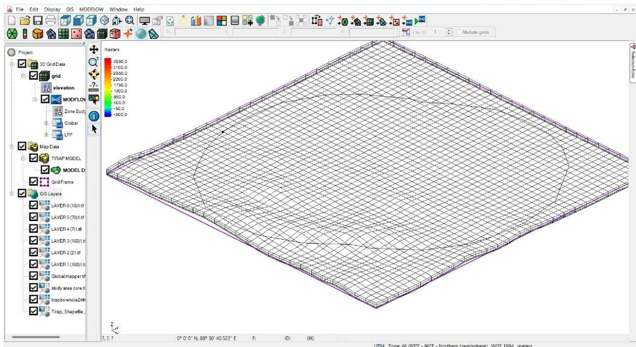
**Fig 3.3:** 3D grid with 6 layers and Model Boundary.
