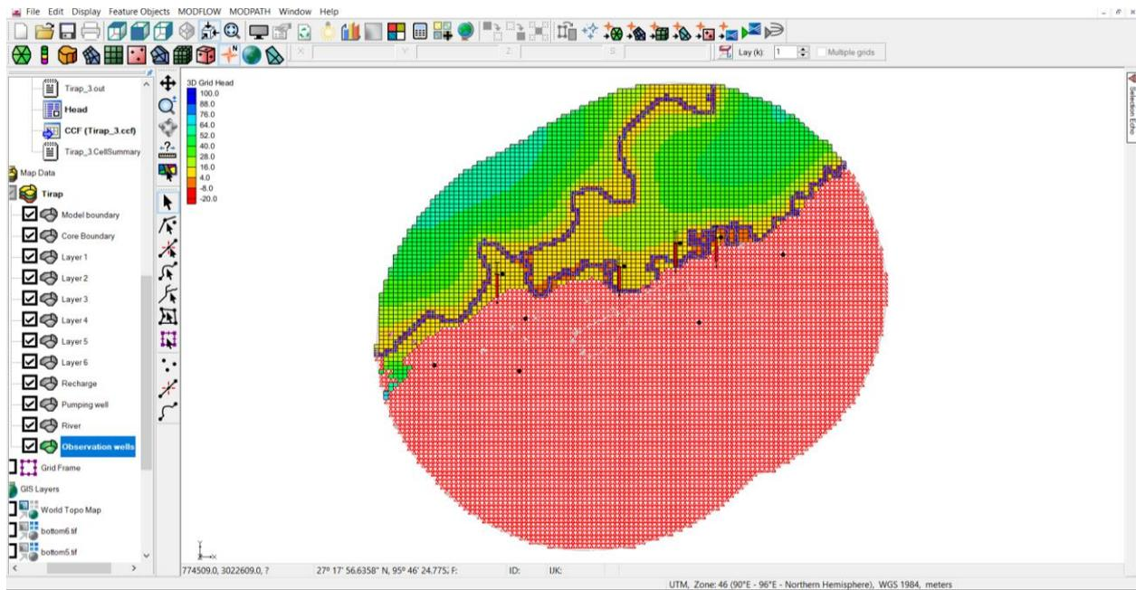
**Fig 3.8:** Calibration of Steady State Model using observation wells.
