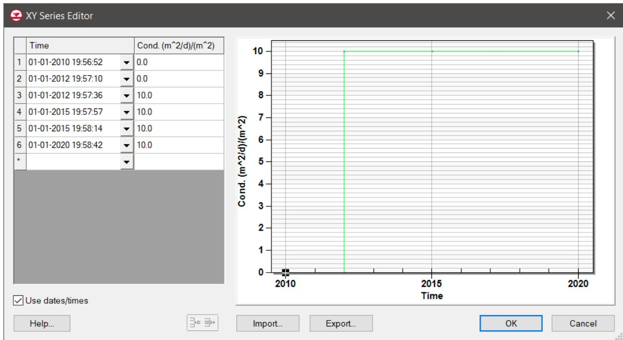
**Fig 3.13:** Drain boundary condition for the mine site.
