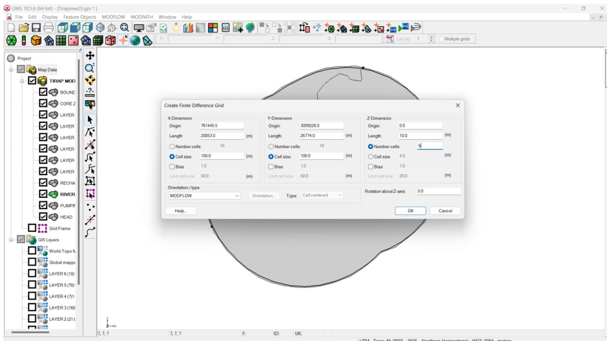
Fig 4.4.3 Creating 3D grid and new modflow simulation
