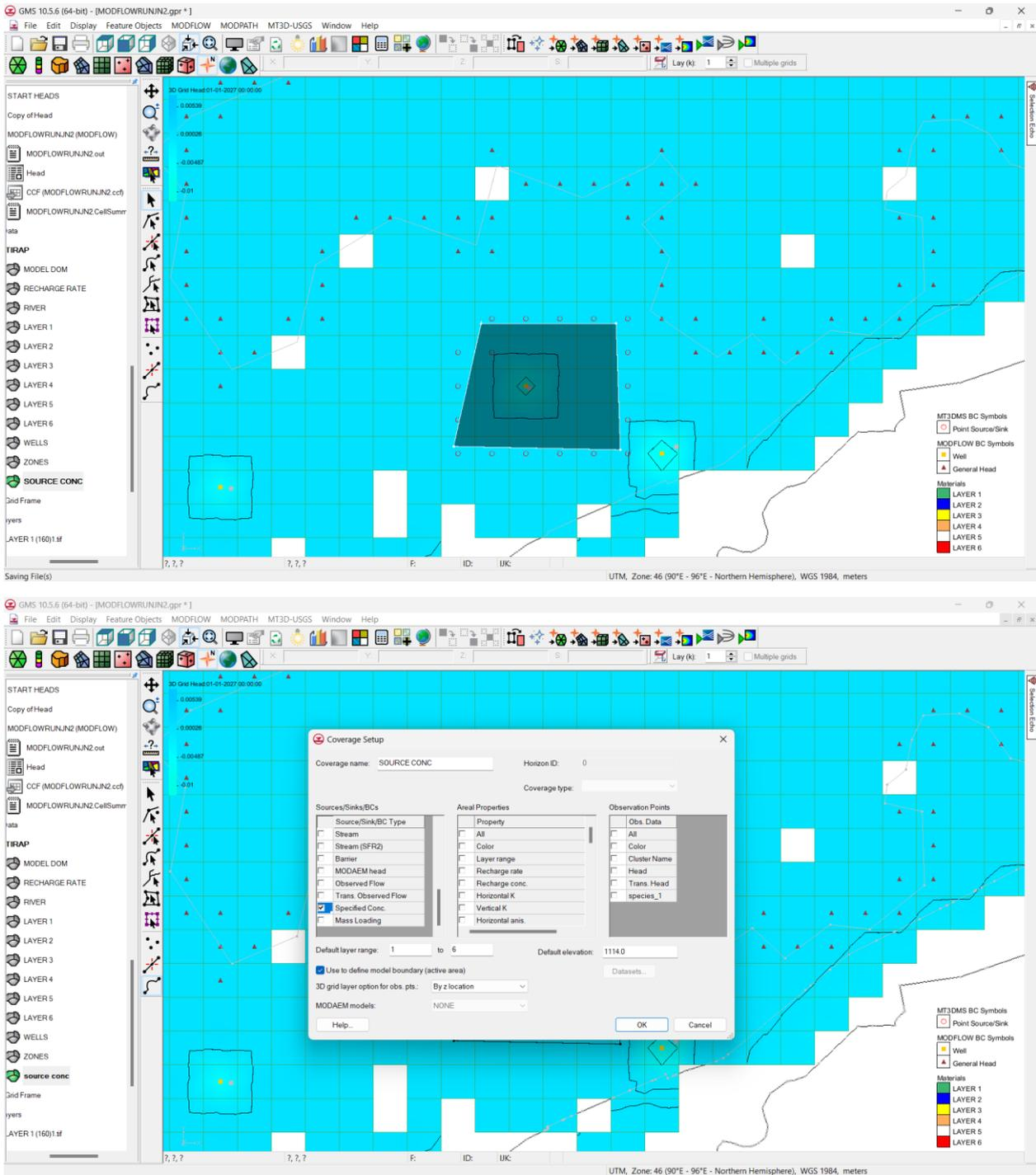
Fig 4.4.22: New polygon created for Source Concentration.
