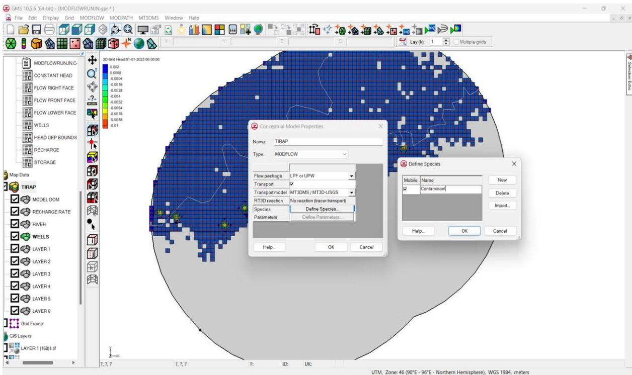
Fig 4.4.21: Assigning properties in Tirap
