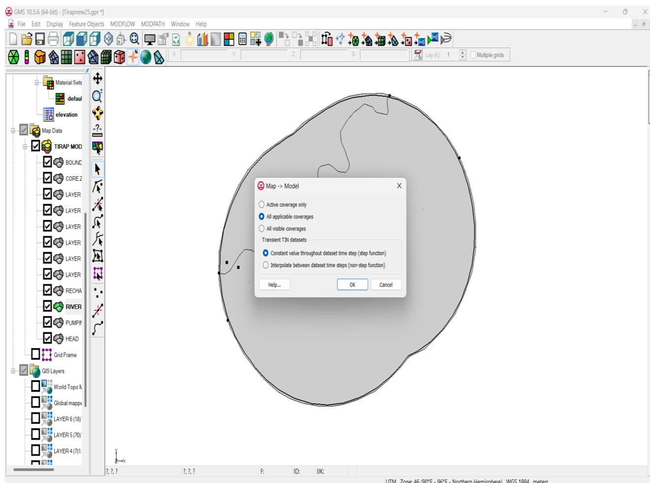
Fig 4.4.8: Map all the applicable coverages made to Modflow.
