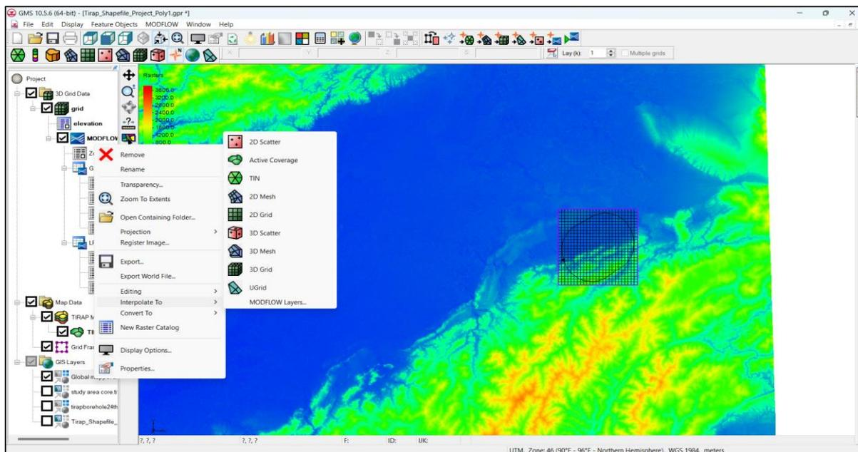
Fig 4.4.5 Interpolate DEM FILE TO MODFLOW Layer
