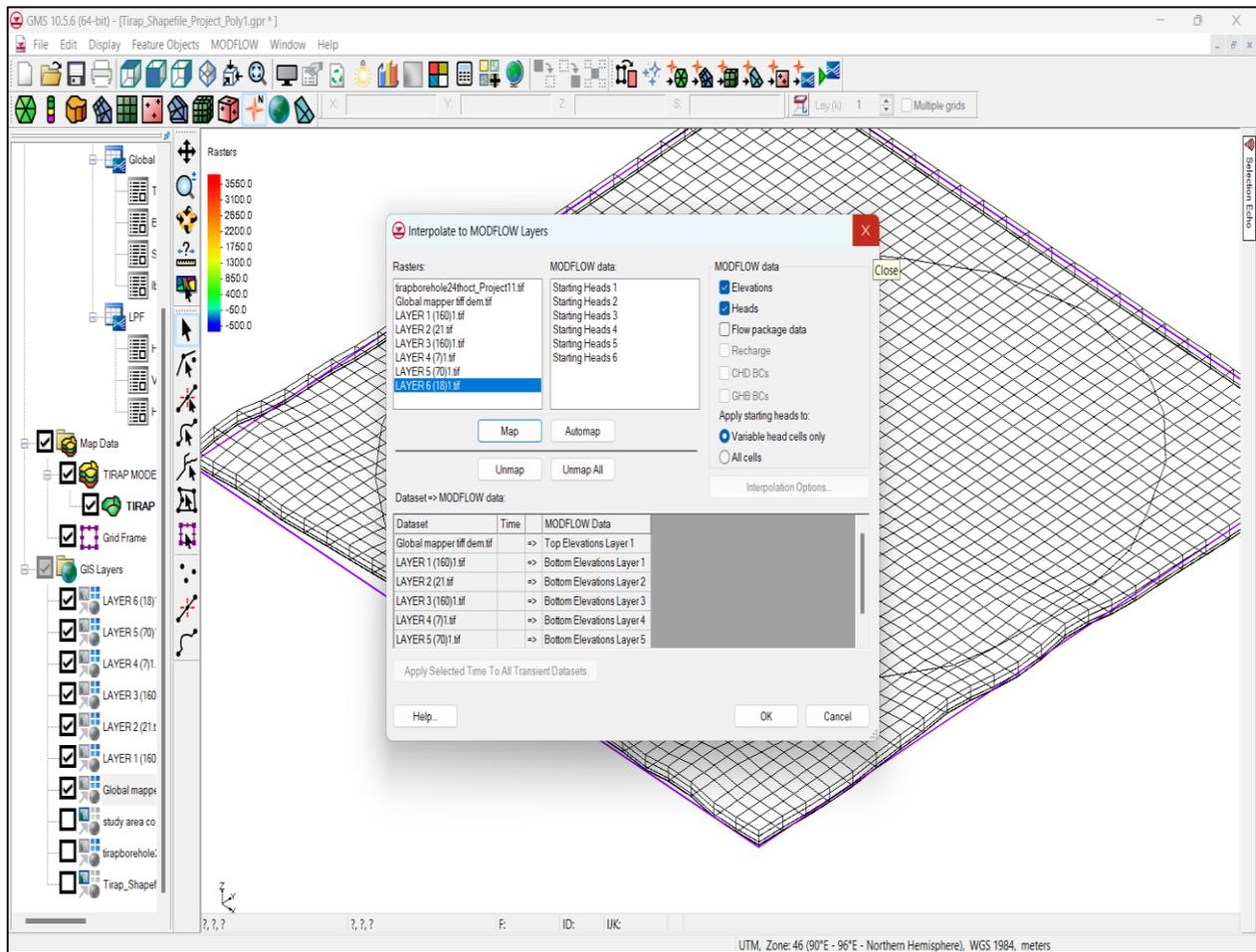
Fig 4.4.6: Interpolation of Raster to Modflow by Layers
