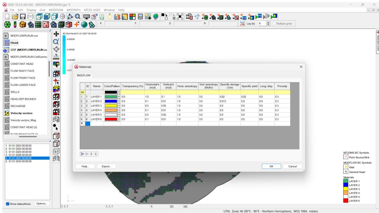
Fig 4.4.12: Assigned Layer Properties
