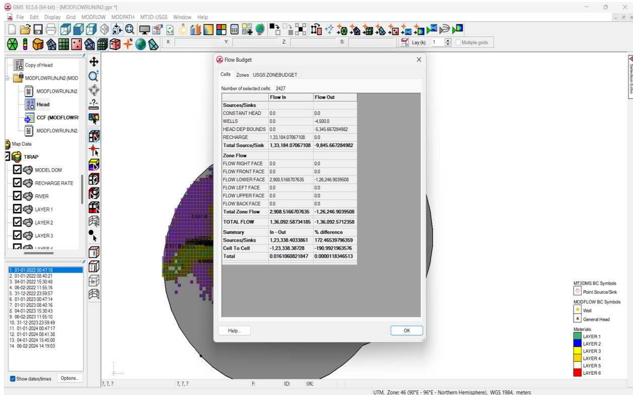
Fig 5.3 Layer 1 flow budget of calibrated model
