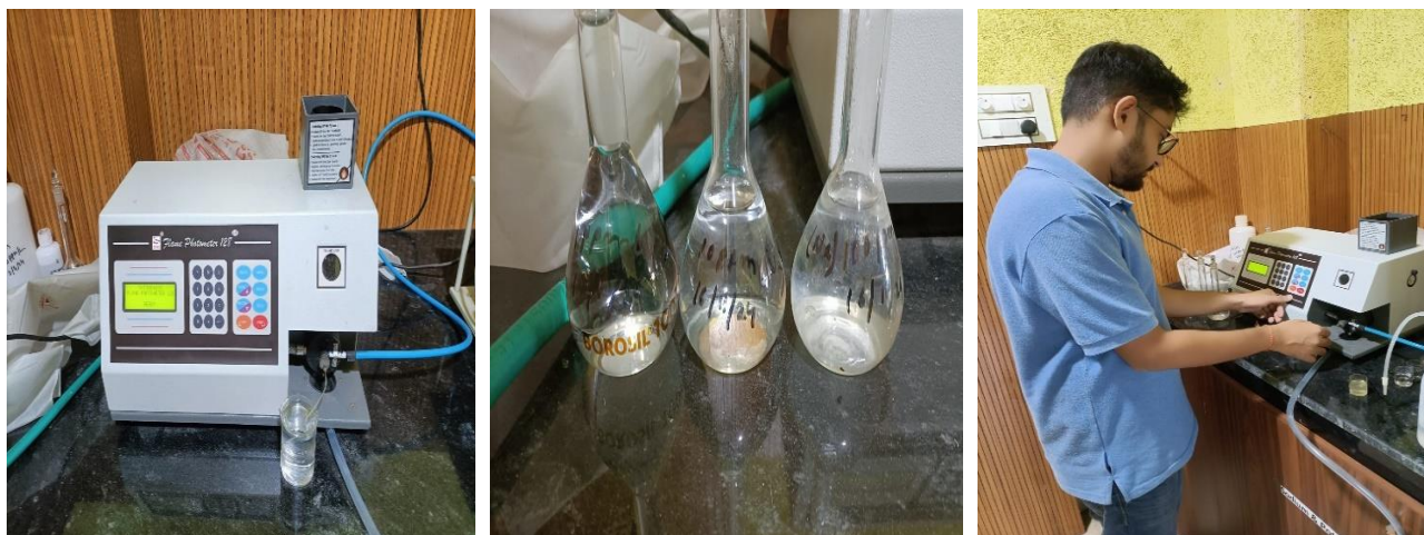
Fig 5.5 (a) Flame photometer, (b) Stock solutions of sodium of 1, 10 and 100 ppm, (c) A moment while conducting flame photometer test
