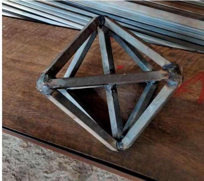
**Fig 3.1:** Octahedron made of MS Rod
