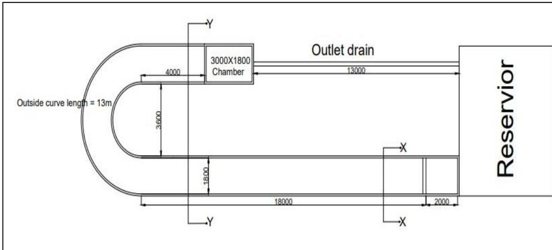
**Fig.3.2:** Experimental channel
