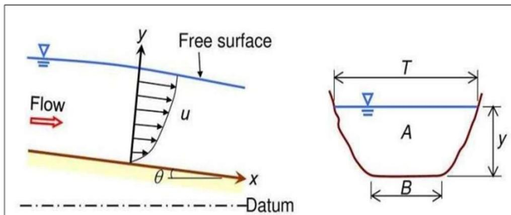
**Fig 1.2:** Open Channel Flow with hydrostatic pressure distribution.
