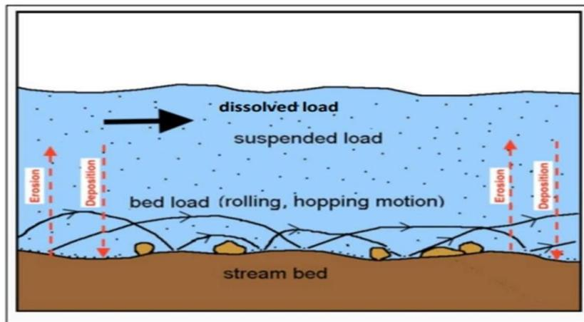
**Fig.1.3:** Sediment transport process
