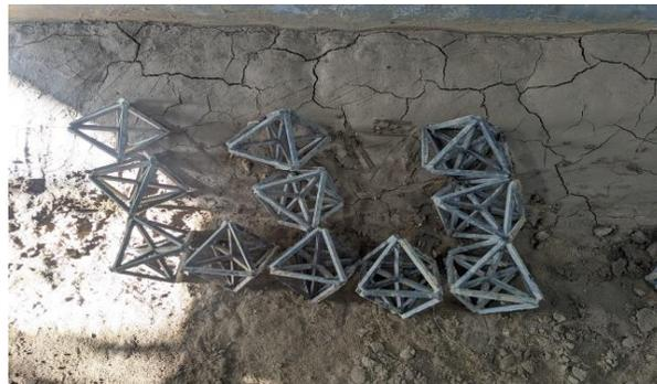
**Fig 4.4:** octahedron field for arrangement 1, set1, before experiment, (Medium depth)
