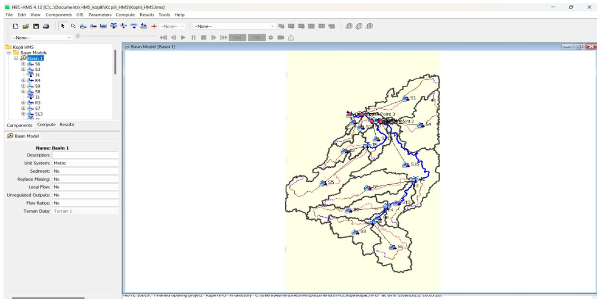
**Fig 4.7: HEC-HMS interface showing sub-basins and junctions**
