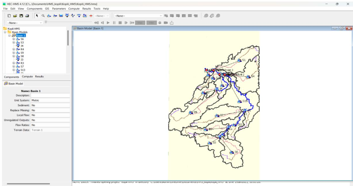
**Figure 5.4:** Dividing the watershed in to different subbasins, drainage parameters and watershed boundaries.
