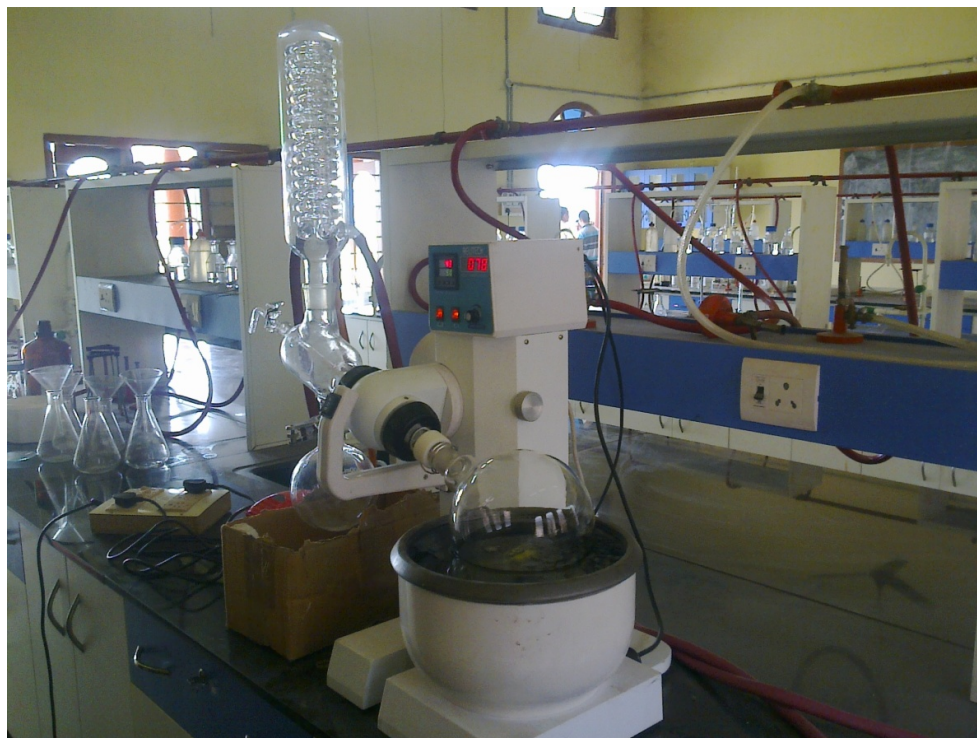
Fig.3.9 Solvent removal (Rotary Vacuum Evaporator)
