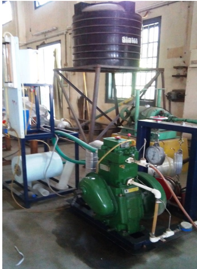
Fig. 3.29 Set up of Single Cylinder Four Stroke Diesel Engine Test Rig (With Rope Brake Dynamometer)
