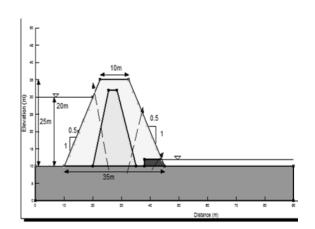
Fig. 1 Dam section having slopes 0.5H:1V
