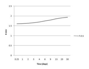
Fig. 5 Factor of safety during all stages of drawdown for the section having side slopes 1H:1V
