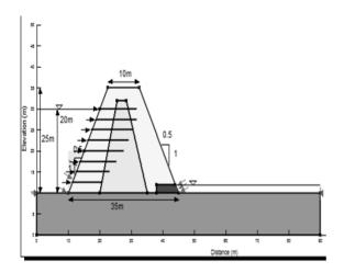
Fig. 3 Dam section having slopes 0.5H:1V reinforced with geosynthetic material
