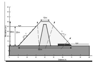
Fig. 2 Dam section having slopes 1H:1V
