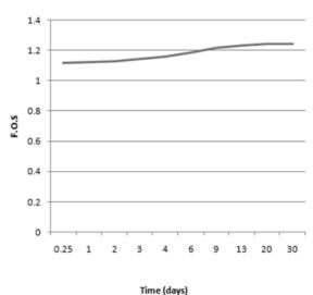
Fig. 4 Factor of safety during all stages of drawdown for the unreinforced section having side slopes 0.5H:1V
