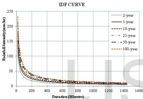
Fig. 1. Intensity Duration Frequency Curve
